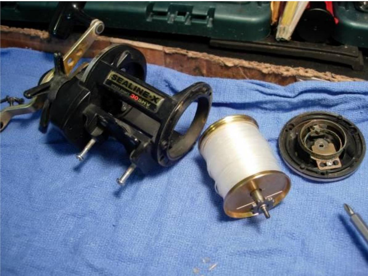
if this reel is going to be used for distance casting and you will be servicing the bearings frequently, then let's remove all of the hardware covering/protecting the left spool bearing (key #9) to allow easy access. otherwise, let's leave it covered and just lube it up.
