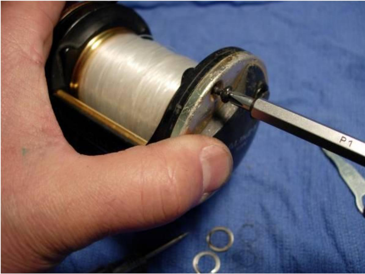
now, for the right side plate assembly. first, let's remove the handle nut plate (key #78) by pushing on two small tabs underneath the handle arm.
