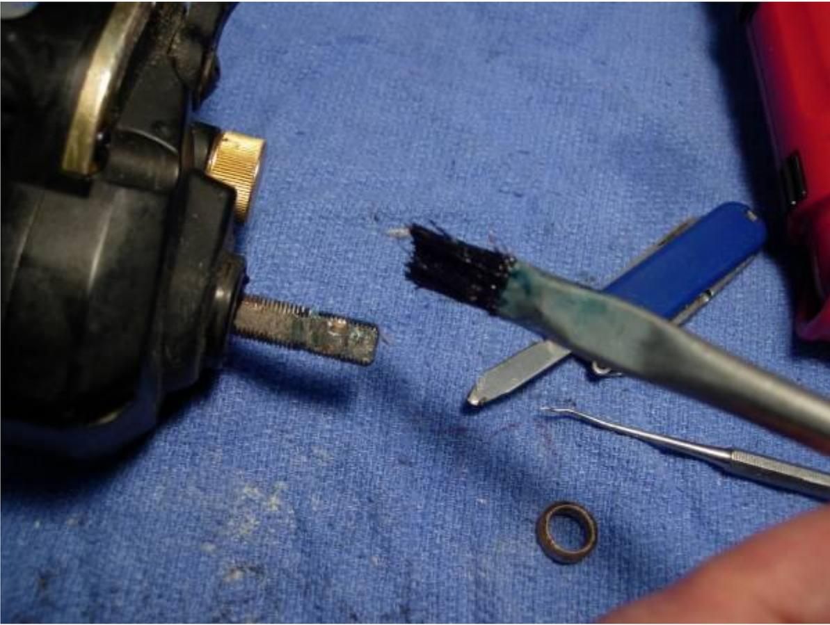
install the bearing washer B (key #72) and the drag spring washers (key #73) oriented "()".
