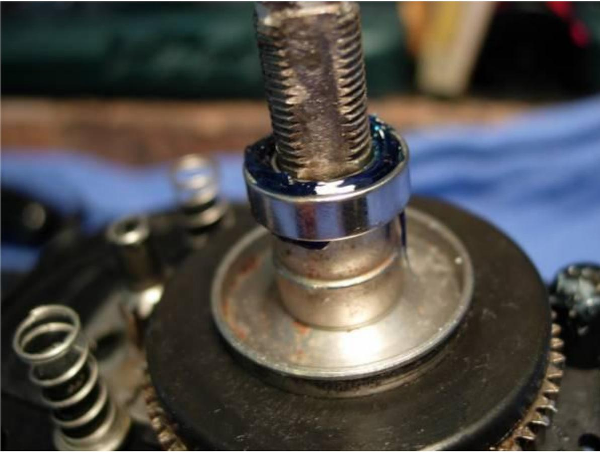
let's install the side plate (key #41). first, the round peg on the clutch cam (key #39) has to match up with the oval hole of the yoke plate (key #28).
