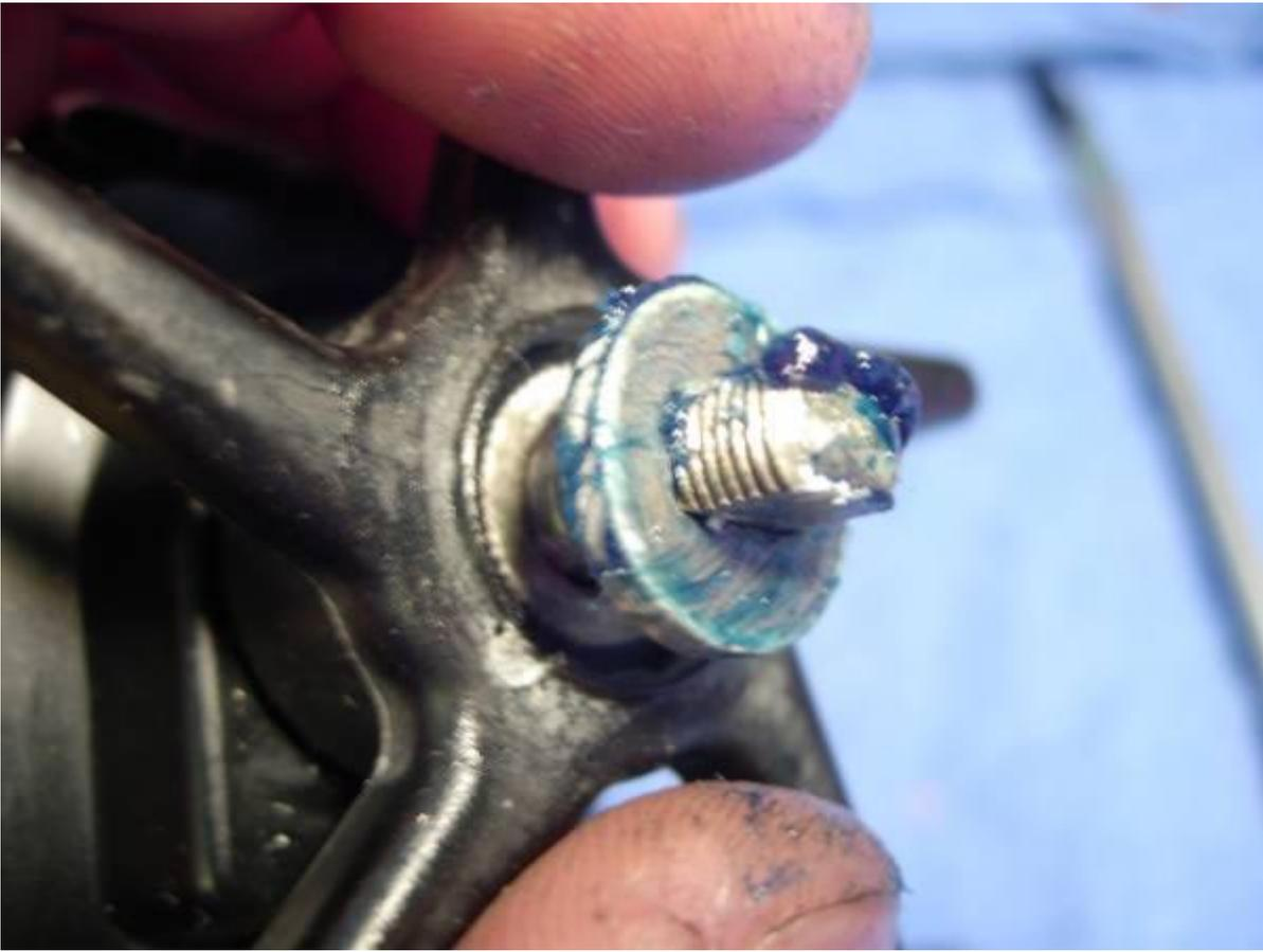
install the handle (key #76), the handle nut (key #77), paint on a little extra grease and then install the handle nut cap (key #78).
