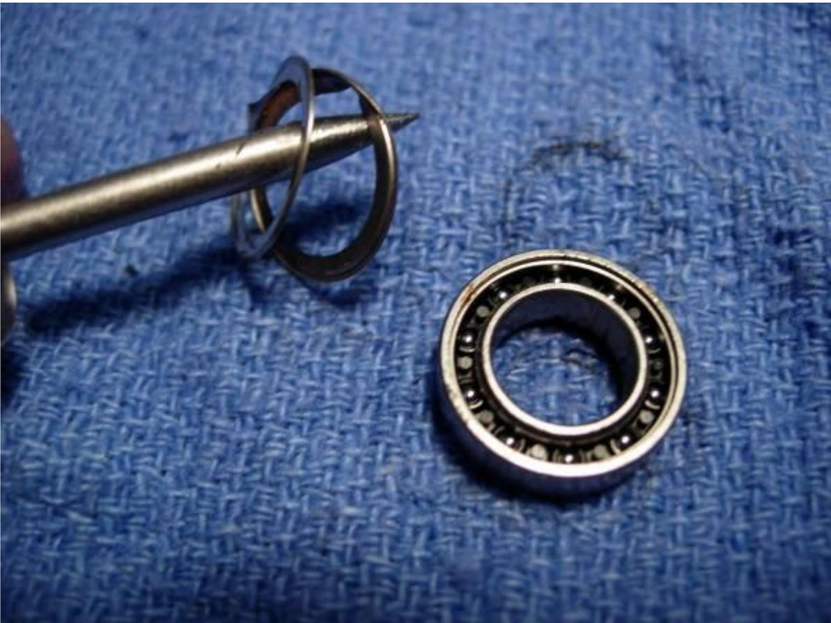
i've opted to clean this bearing and lube it with corrosion x. if casting was not an issue, you could pack the bearing with grease as discussed in the bearing post.
