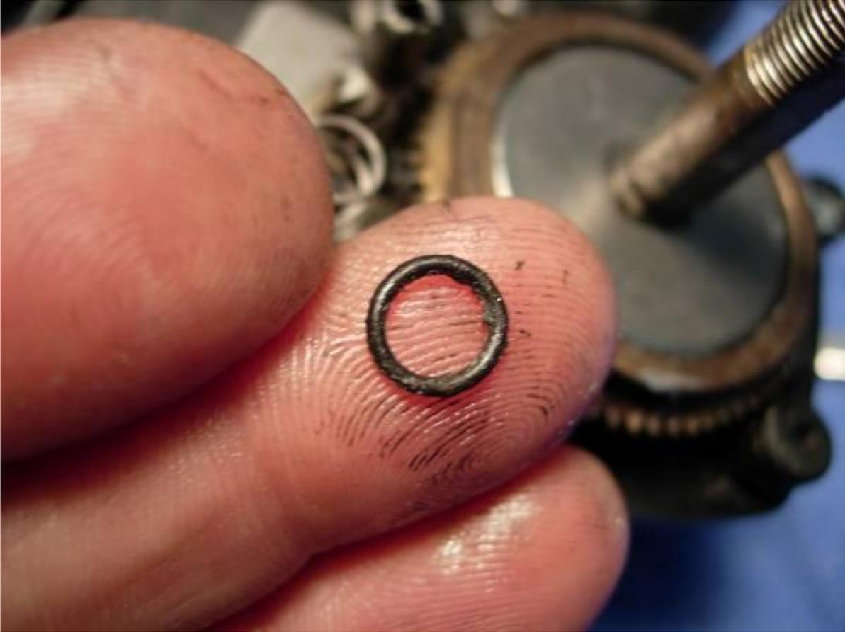
replace collar A (key #69) and the water shield (key #68).
