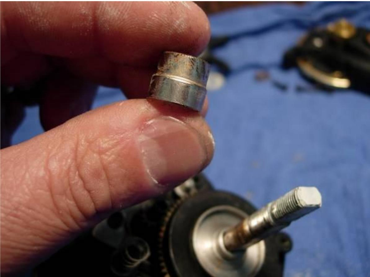
remove collar A (key #69) and the water shield (key #68).
