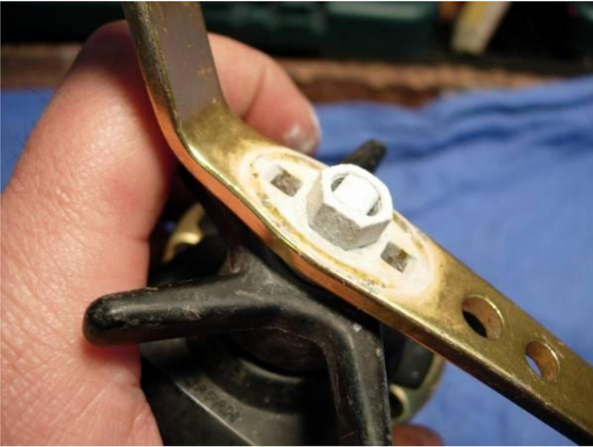
see, i told you it would work!!!!!! now, remove the spacing sleeve (key #75) and the star drag (key #74).
