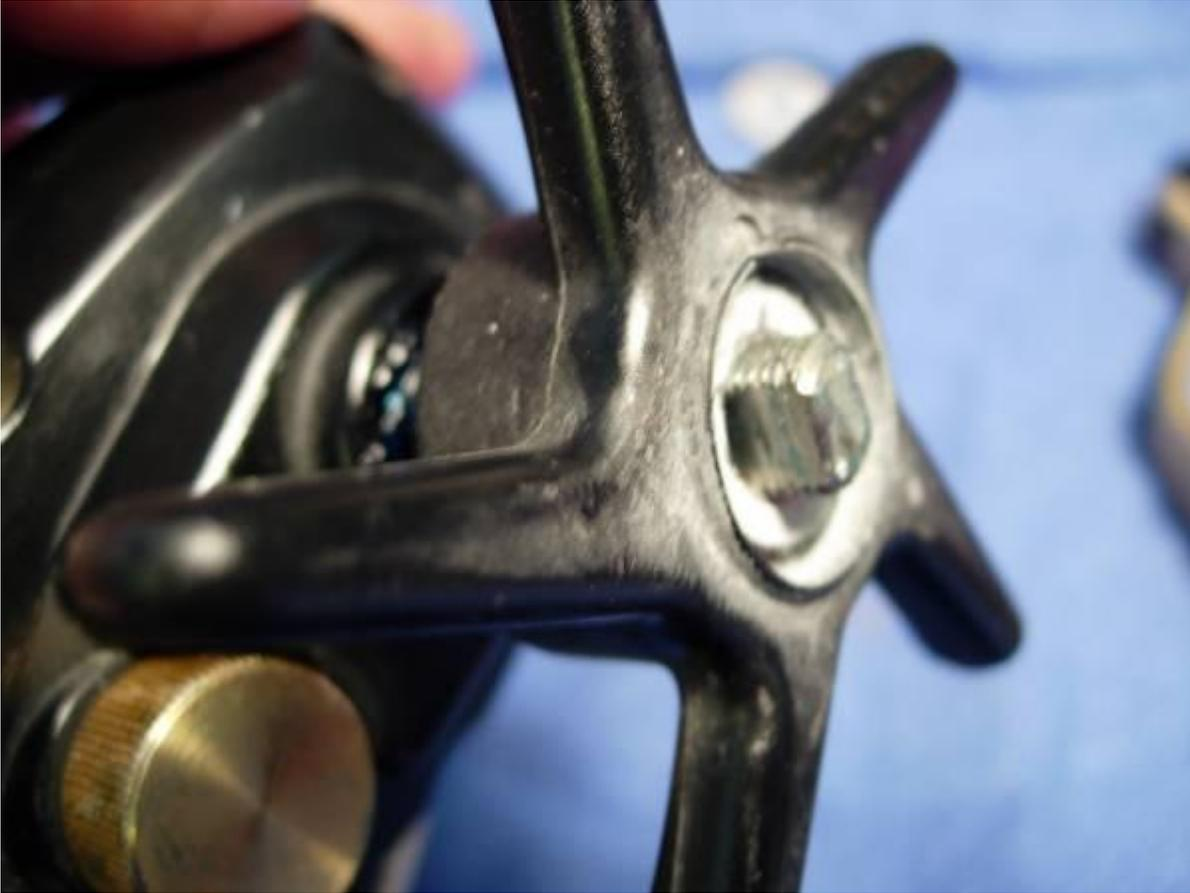
**paint a little grease on the spacing sleeve (key #75) and install it.**
