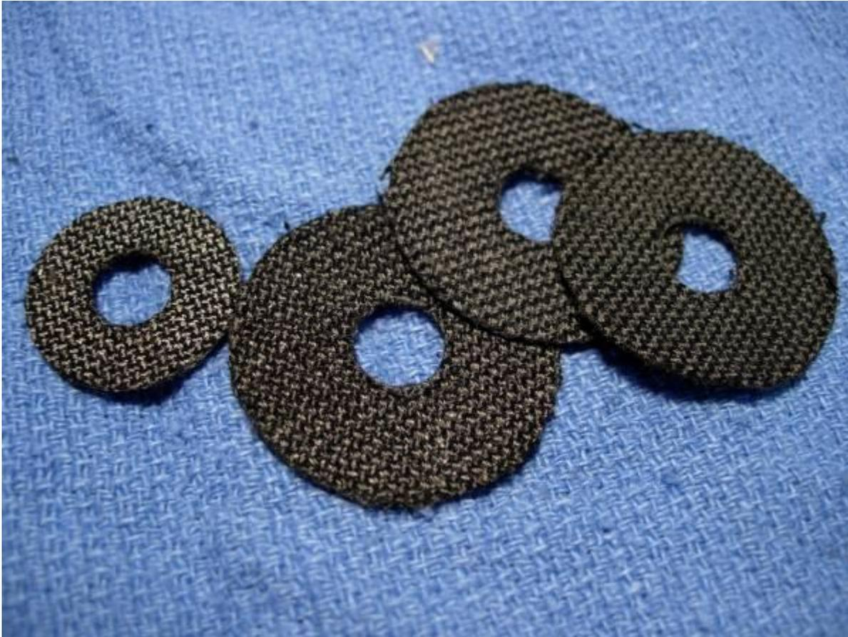
slap a thick coat of shimano or cal's drag grease on the drag washers. let the excess ooze out the sides.
