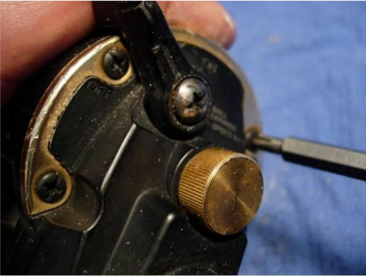
remove the right side plate assembly (key #41). it will lift off cleanly. note that the bearing (key #71) stayed with the side plate. pull it out and set it in line with everything else, or just leave it there for now.
