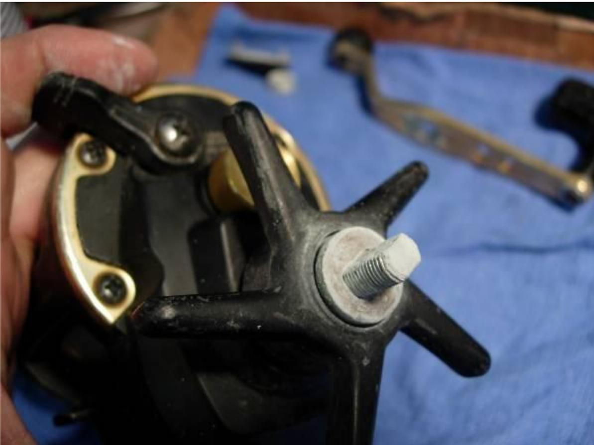
remove the drag spring washers (key #73) and bearing washer B (key #72). note that the spring washers are cupped "()" .
