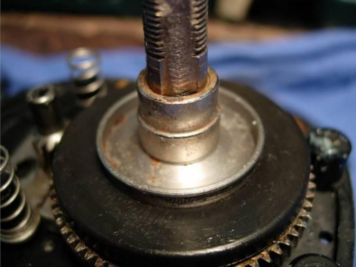
now, about that bearing (key #71). sorry, it's toast. it's a very common problem. and don't be disappointed. not a single reel manufacturer anywhere, from accurate to zelina, will take the time to adequately pack these drive shaft bearings with grease.
