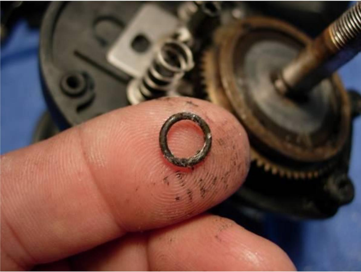
when you bolt down the handle, a small burr forms on the drive shaft (key #59). to make it easier to remove the metal drag washer and the main gear, let's take a flat file and file off the burr.
