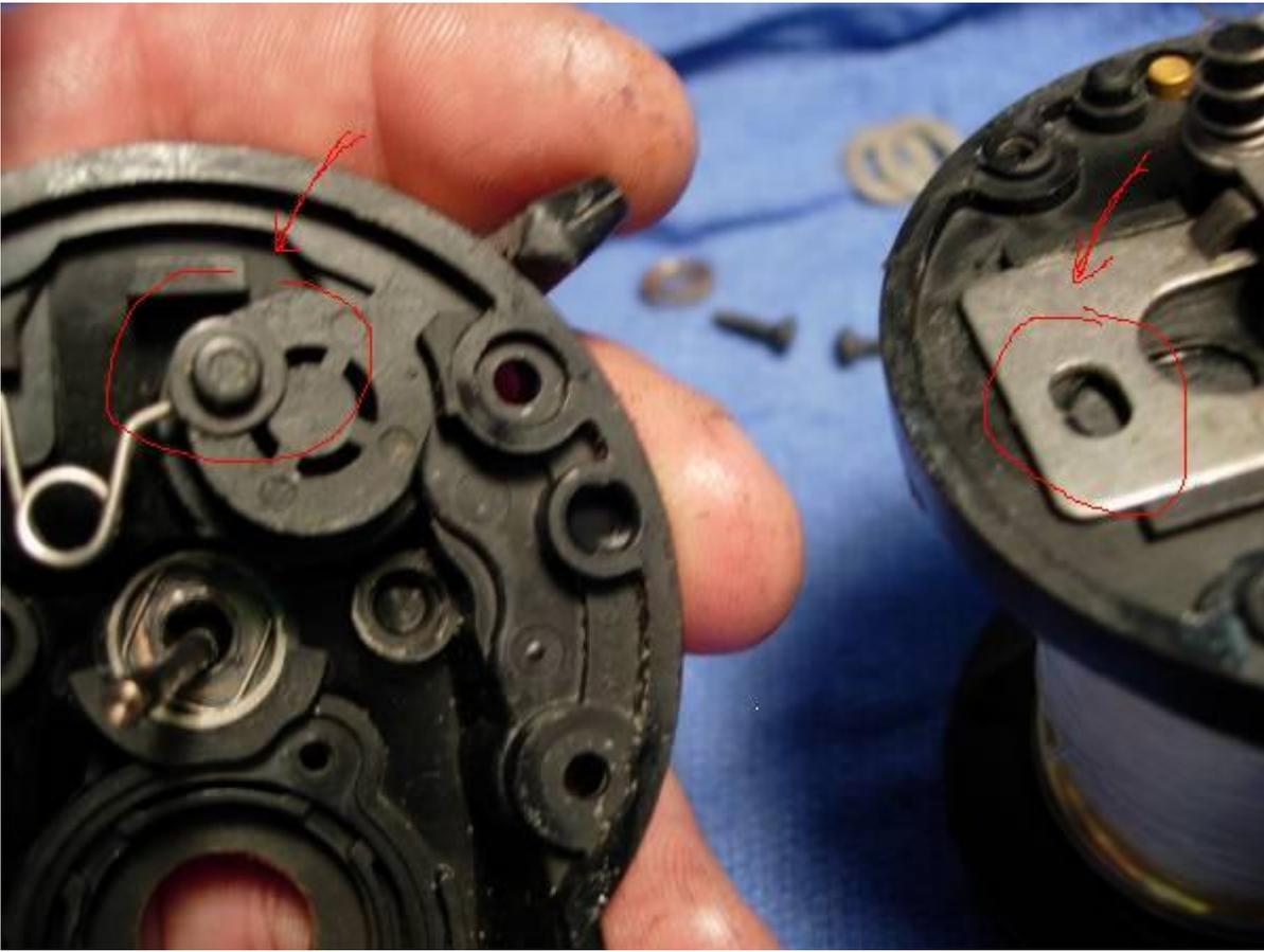
second, the point of the pinion shaft (key #49) has to match up with the hole in the pinion gear (key #32).
