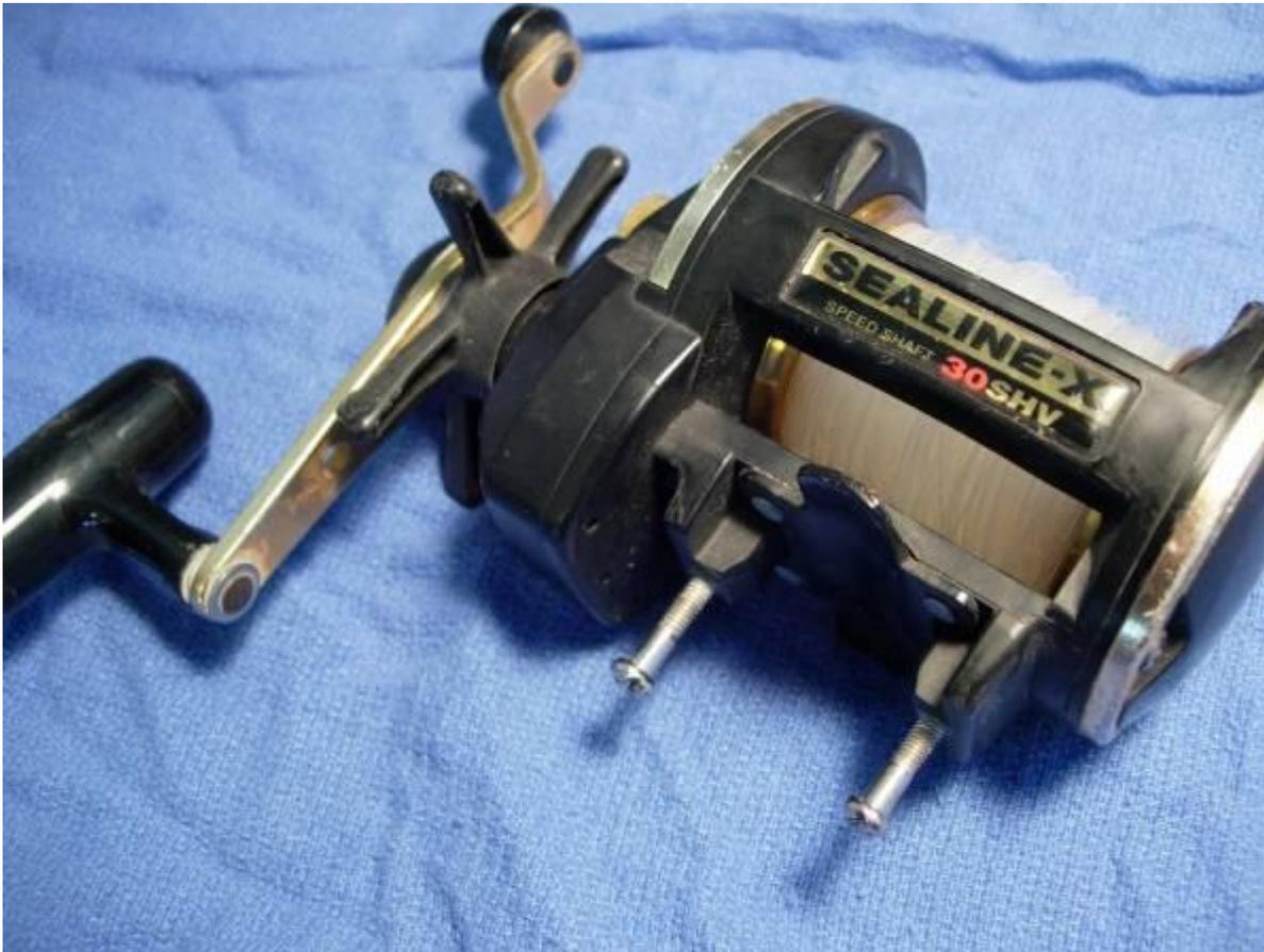
this is a casting reel. for now, and in the future, we can service the bearings by pulling just the left side plate and spool. nice design. remove the three left side plate screws (key #1).
