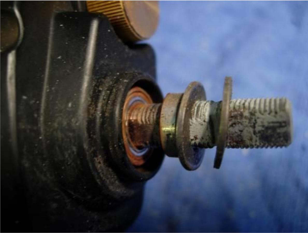
now for the right side plate. remove the four right side plate screw A's (key #46) and the two right side plate screw B's (key #47). take note, they are different. also, there is no need to remove the clutch lever (key #42) or the cast control cap (key #54), so let's leave them in place.
