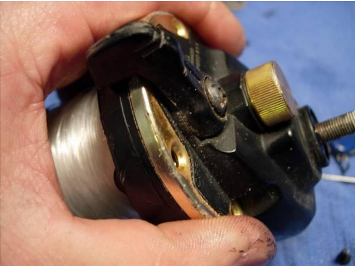
reinstall side plate screws A (key #46) and B (key #47).
