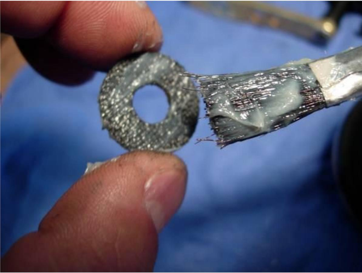
rebuild the drag stack and alternate the metal washers "keyed/eared/keyed."
