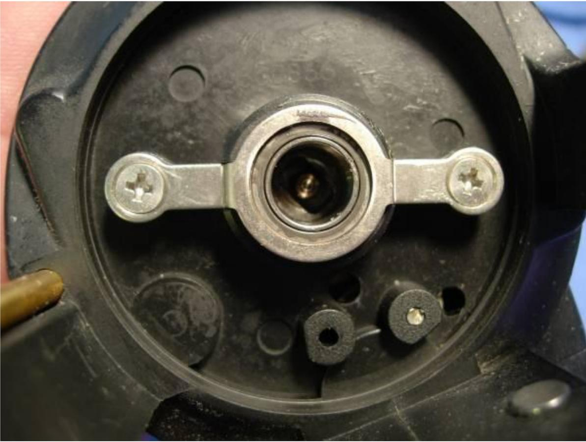
at the very least, let'd pull it out and remove the shields. remove both bearing retainer screws (key #20) and the bearing retainer A (key #19).
