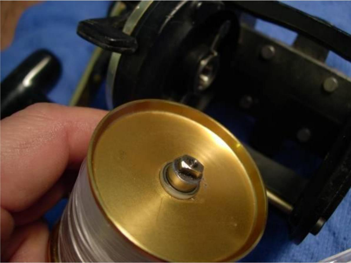
reinstall the left side plate assembly.
