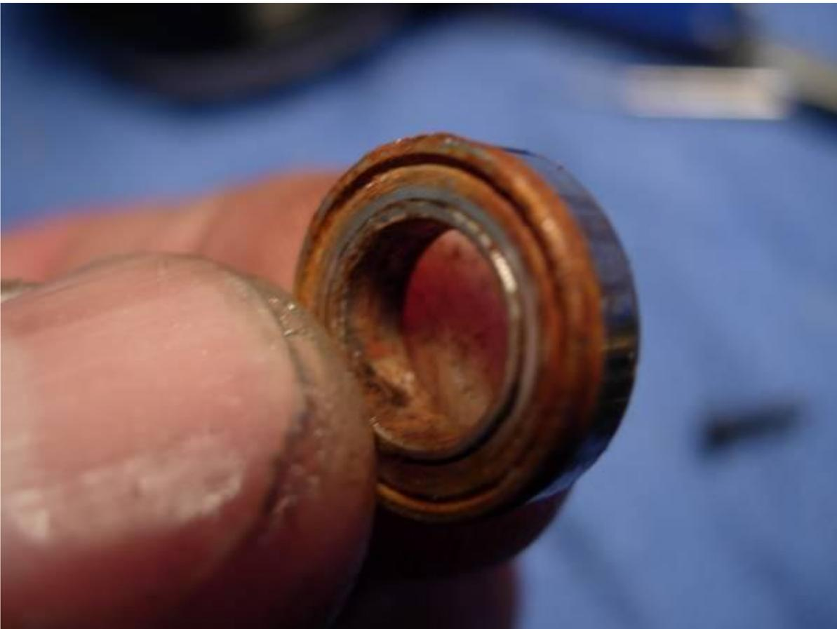
so let's replace it with a new bearing, pack that bearing with grease and put it back on the drive shaft.
