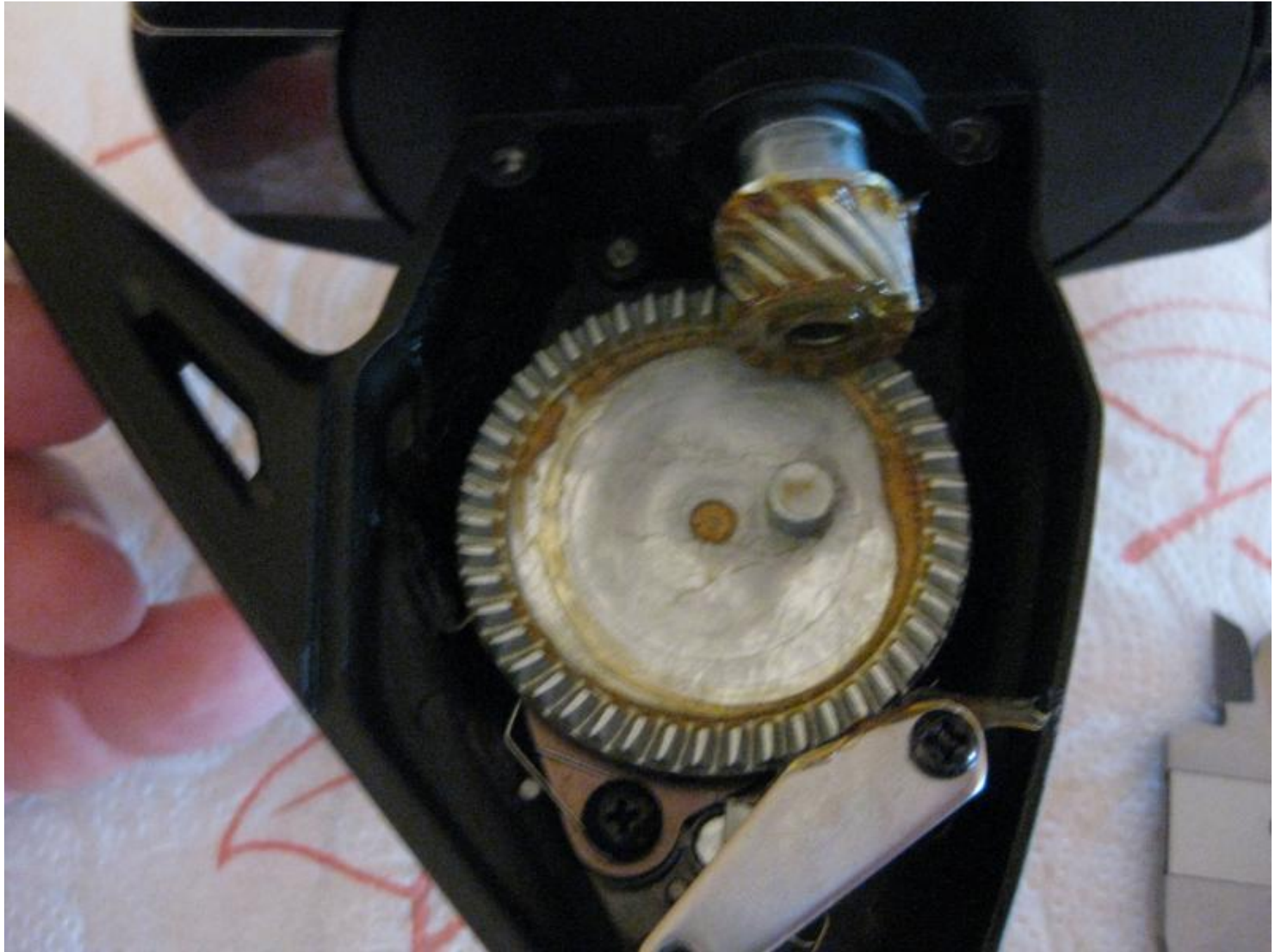
View with the removed axle and its drive
