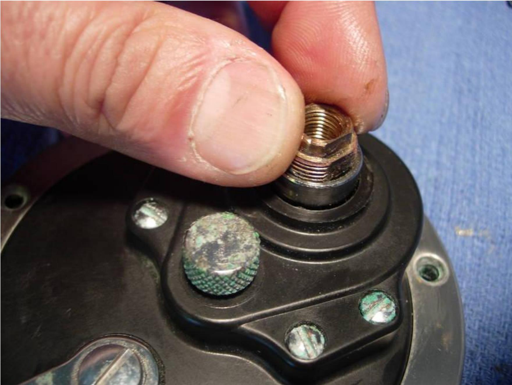
check the function of the eccentric lever assembly (key #21).
