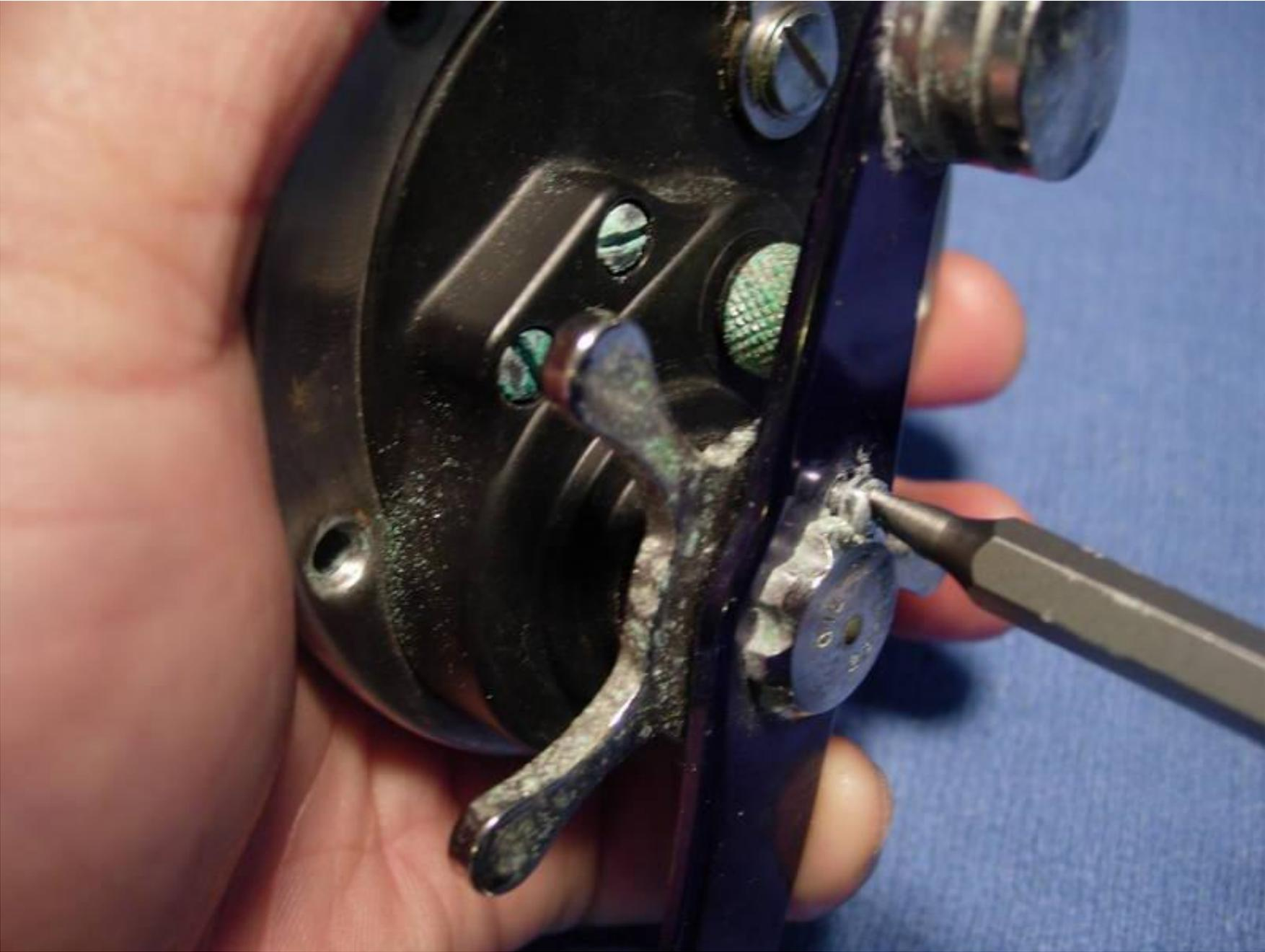
remove the handle assembly screw (key #23).
