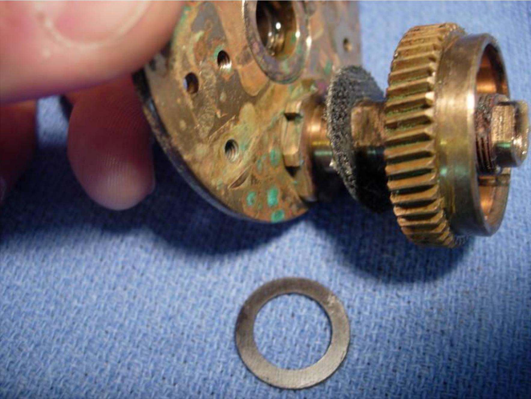
**slap a thick coat of drag grease on all the other carbon fiber drag washers and rebuild the drag stack.**
