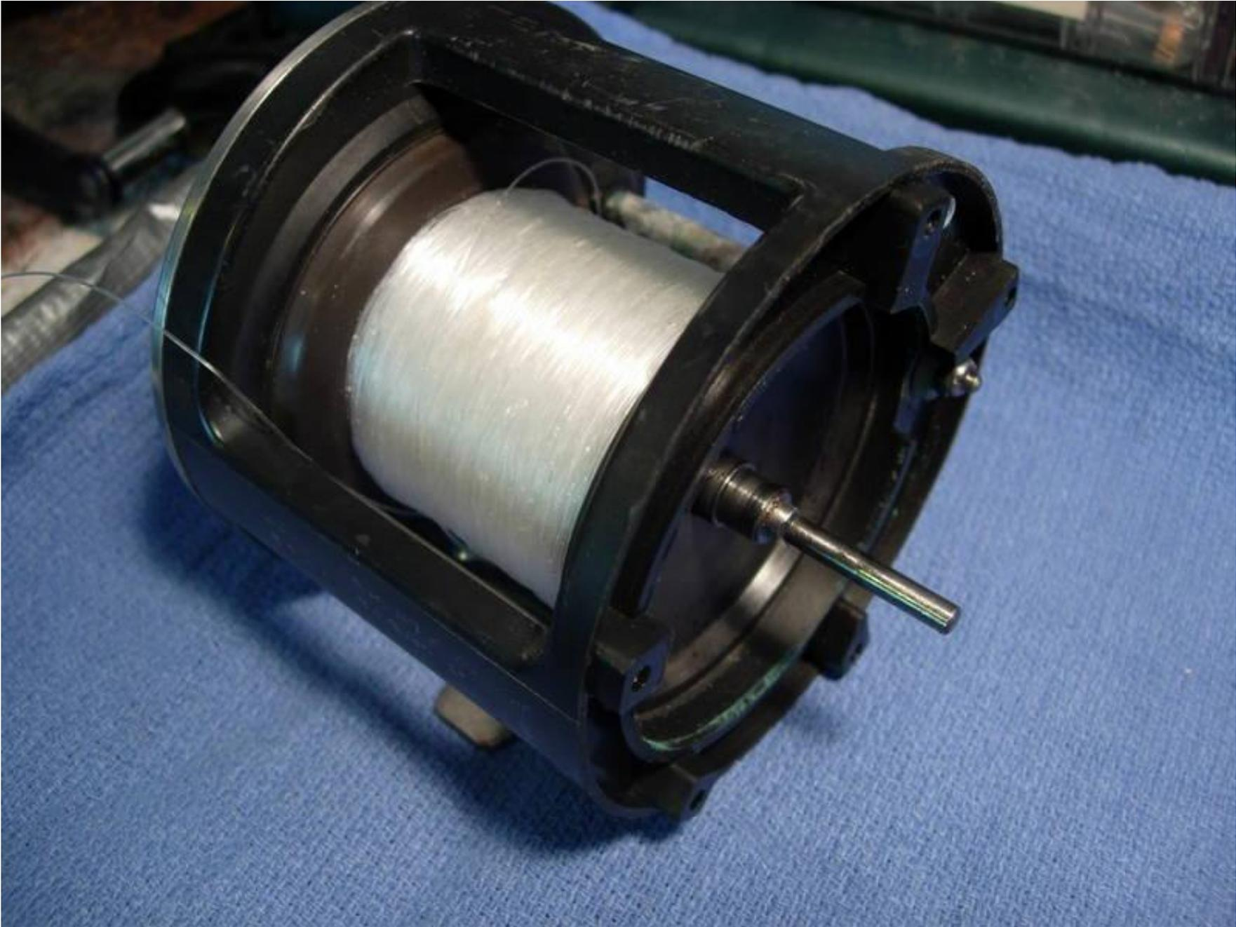
now for the right side plate assembly (key #1). remove the handle lock screw (key #23A).
