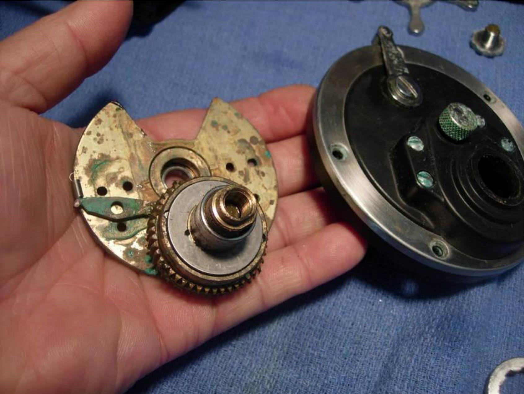
here is an exploded view of the bridge assembly (key #3) and main gear cluster (key #5).
