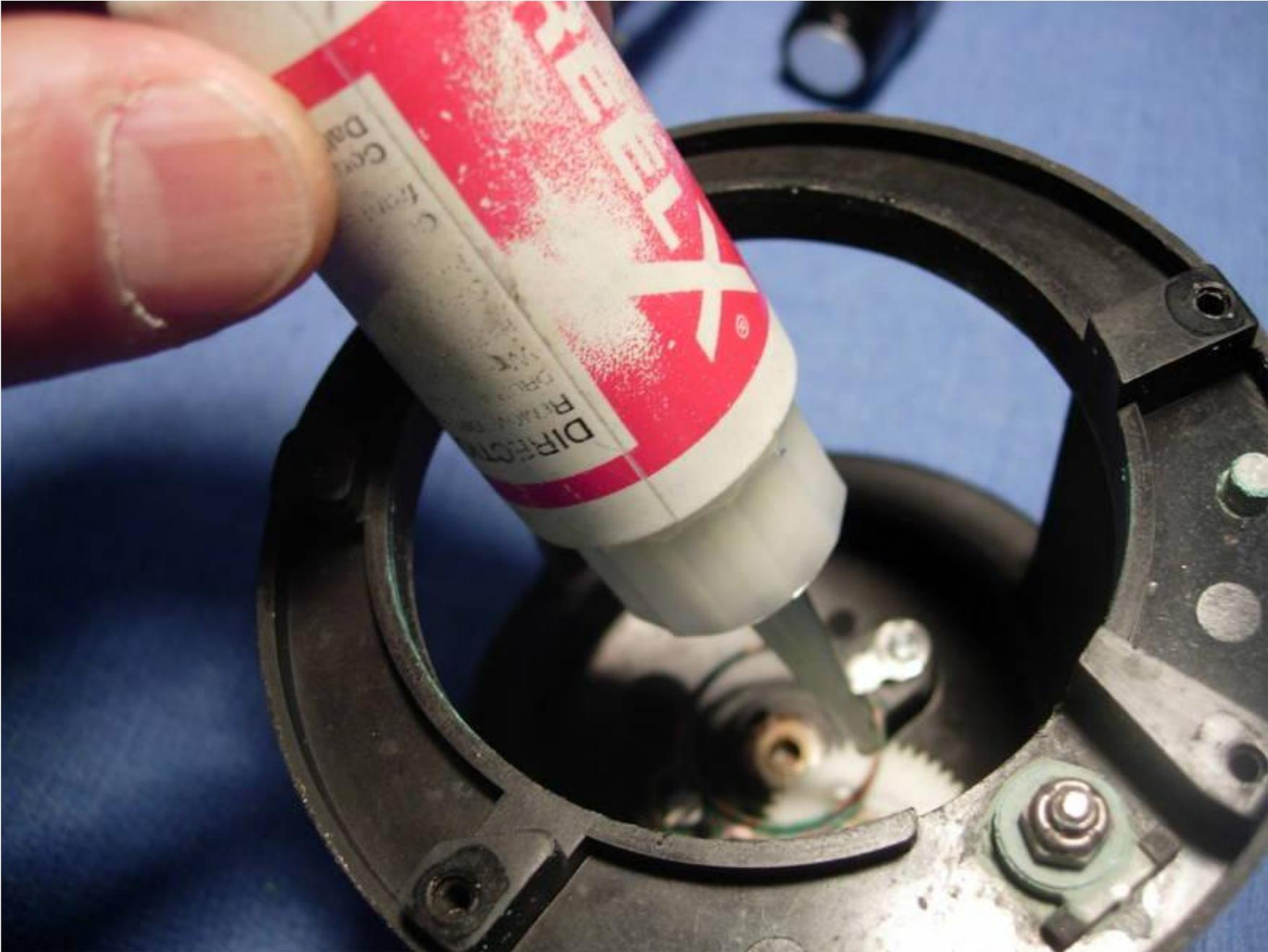
lube the worm (key #42) in the levelwind assembly.
