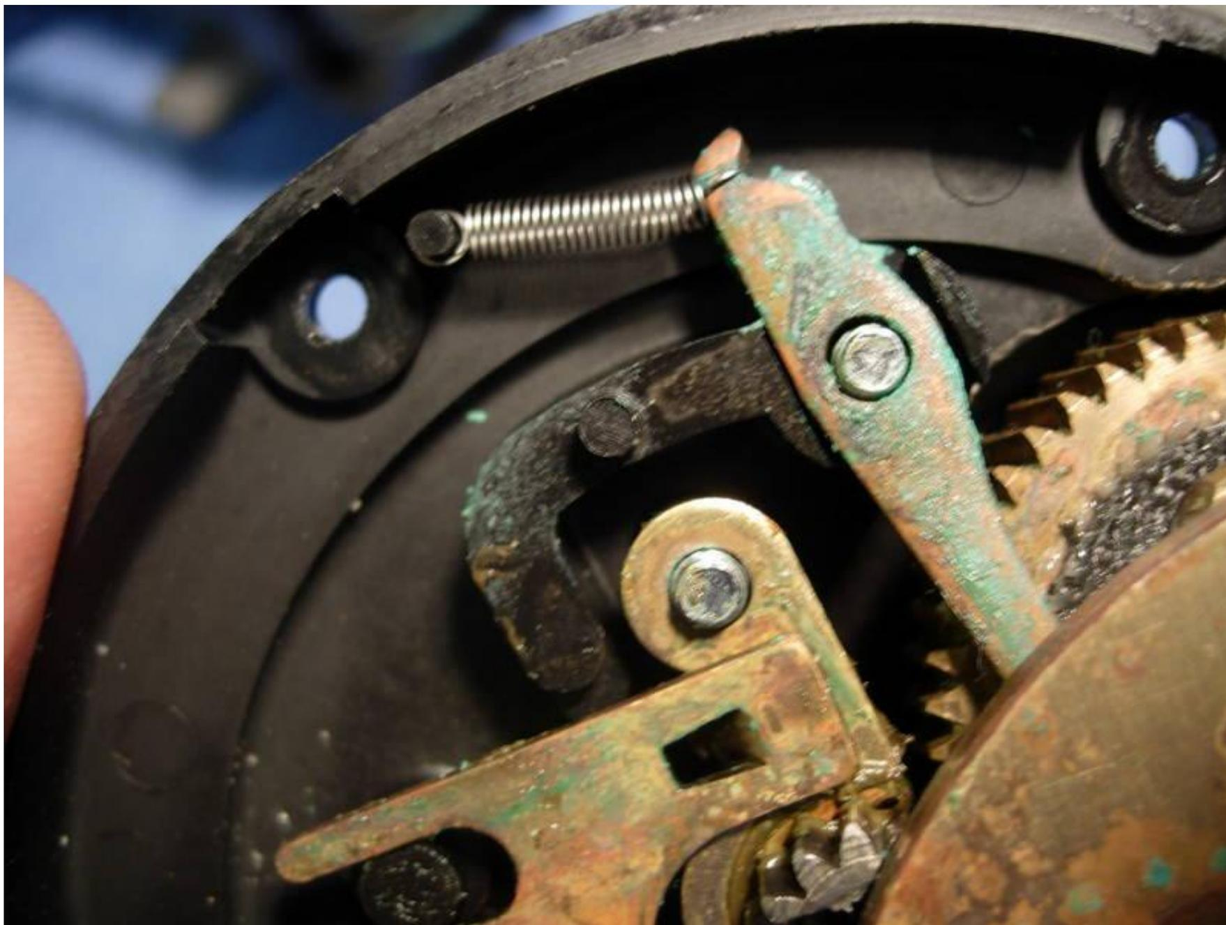
rotate the bridge (key #3) 90 degrees clockwise until the bridge plate seats properly.
