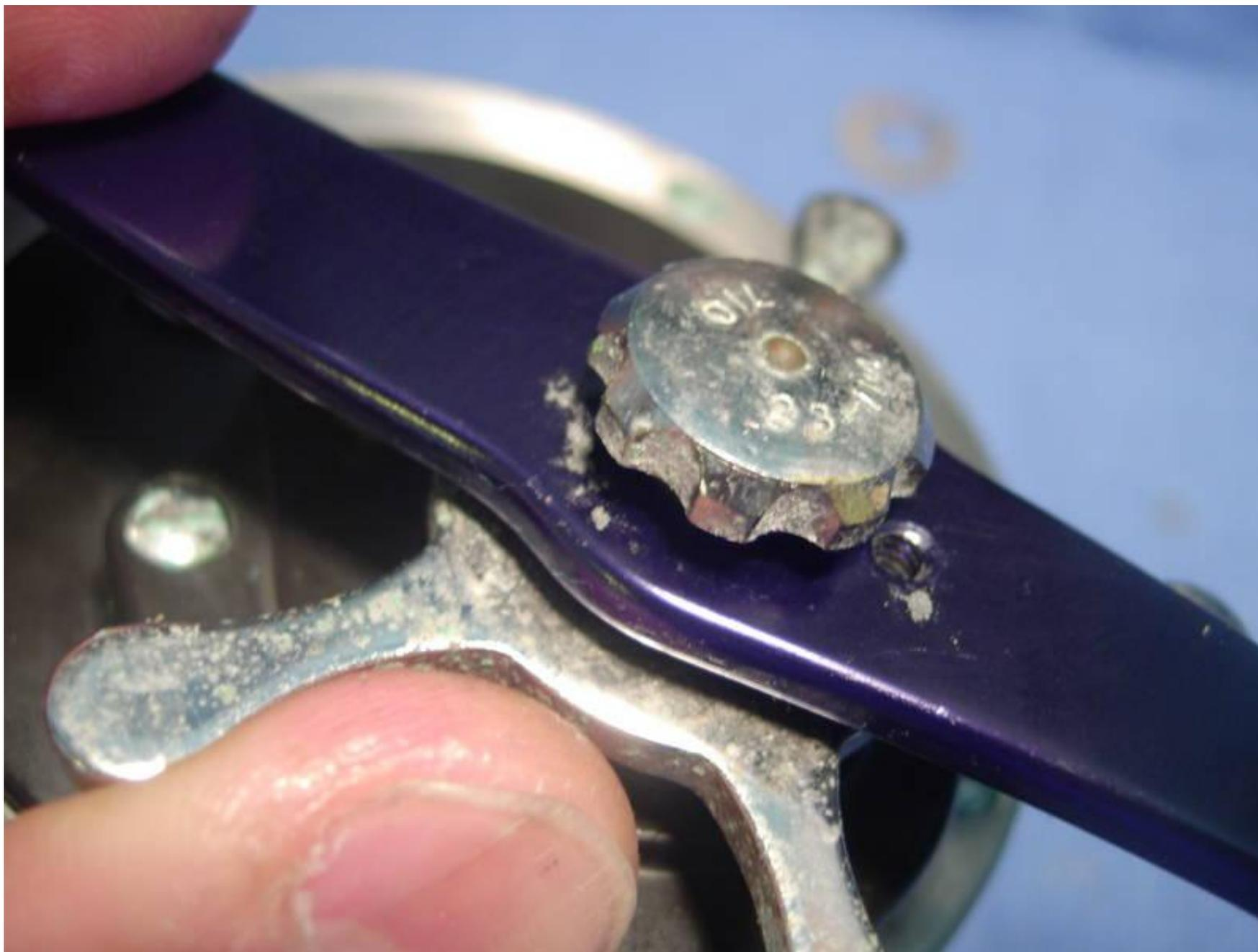
install the handle lock screw (key #23A).
