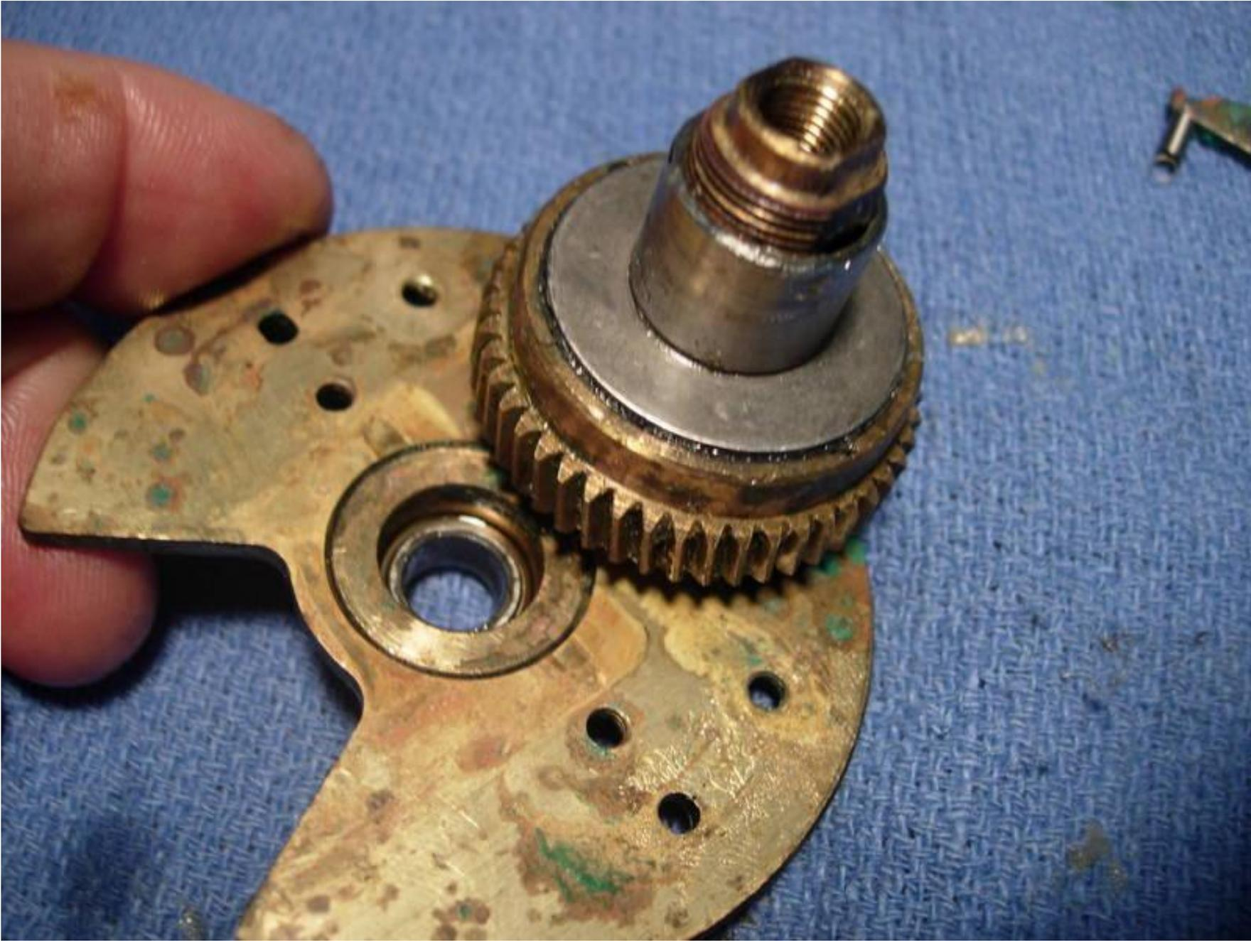
place your left and middle fingers over the bridge screws and lift up the right side plate.
