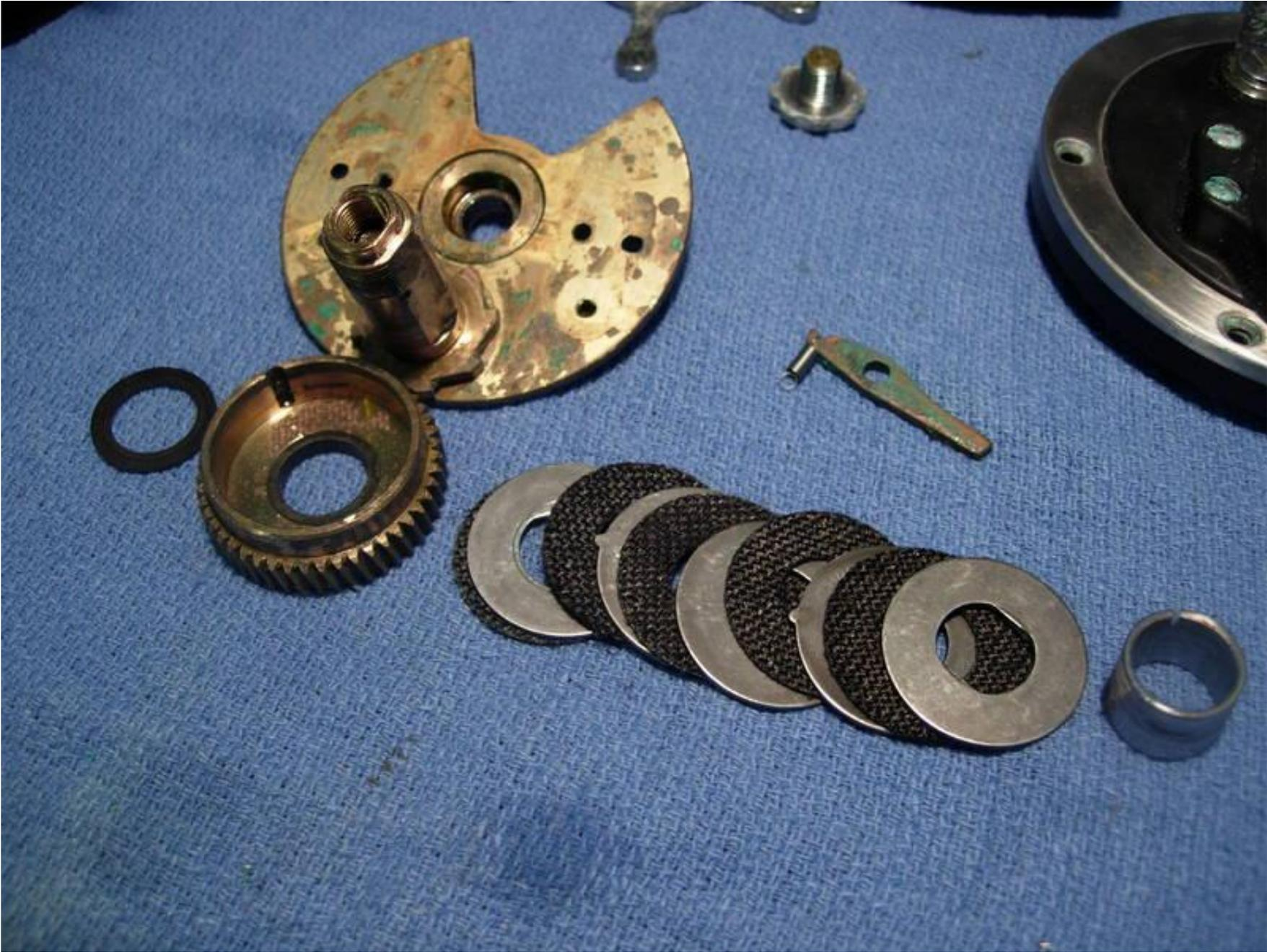
we're going to switch out the fiber washer (key #4) for a drag washer (penn part #6-875).
