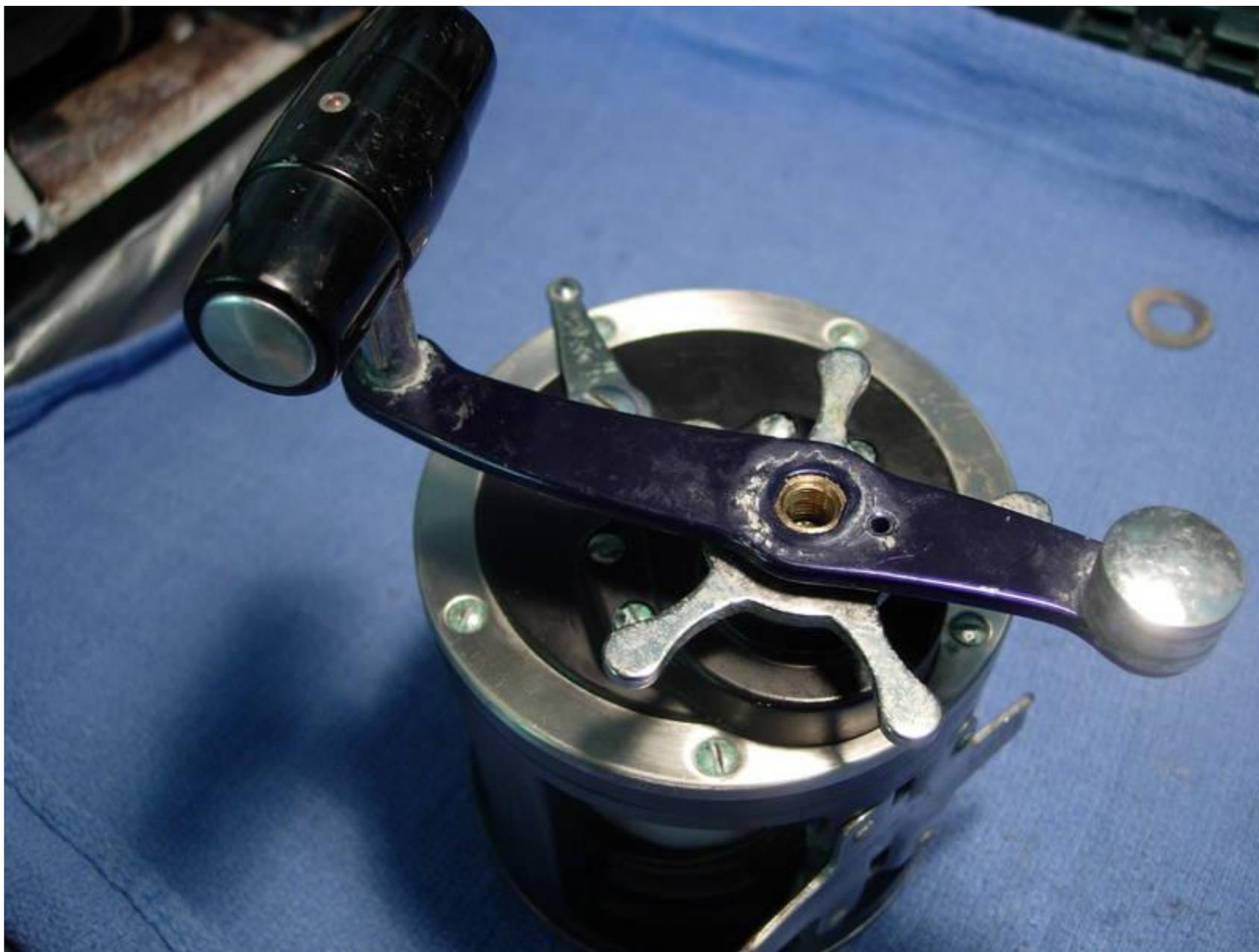
install the handle assembly screw (key #23).
