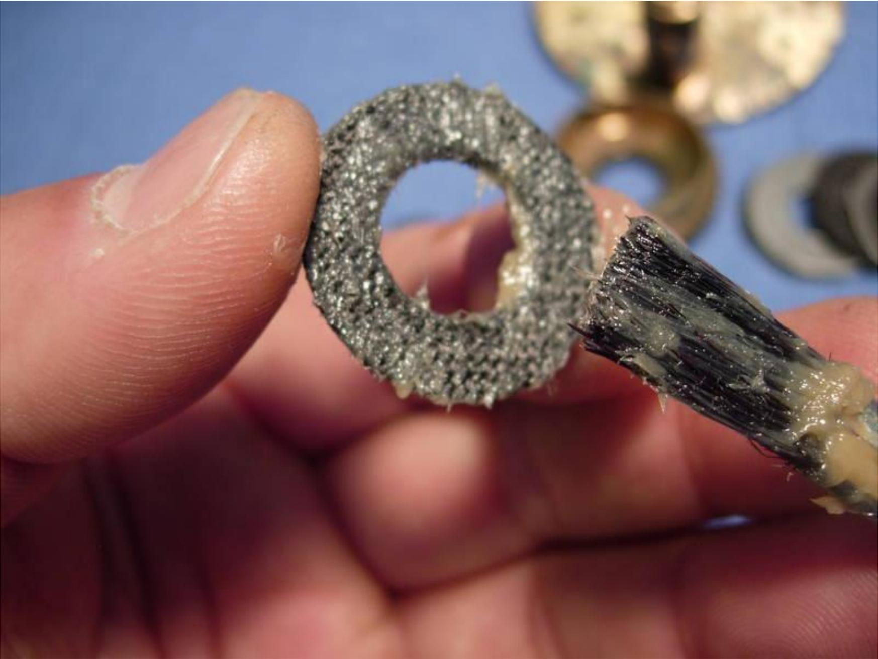
rebuild the drag stack, starting with the #6-875 washer underneath the main gear.
