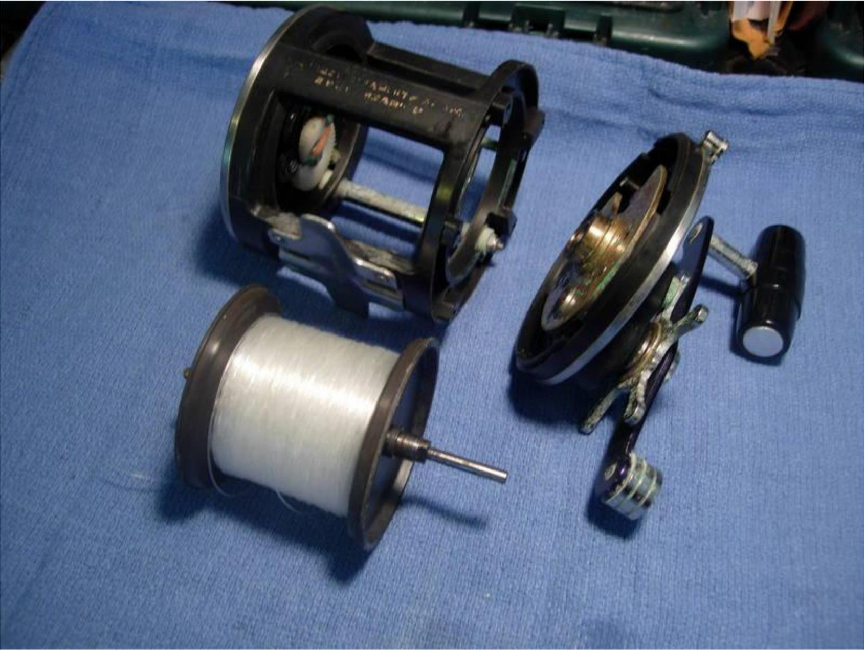
**lube the left side plate bearing (key #40).**
