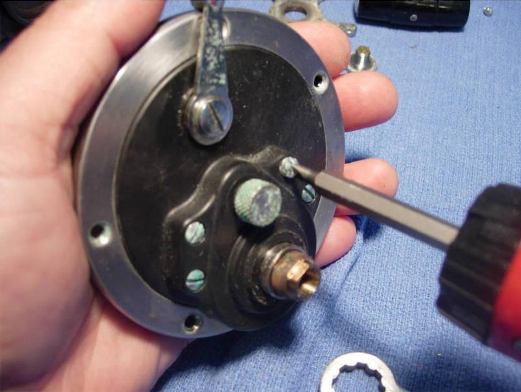
the bridge assembly (key #3) will fall out easily, so catch it without turning the right side plate (key #1) upside down.
