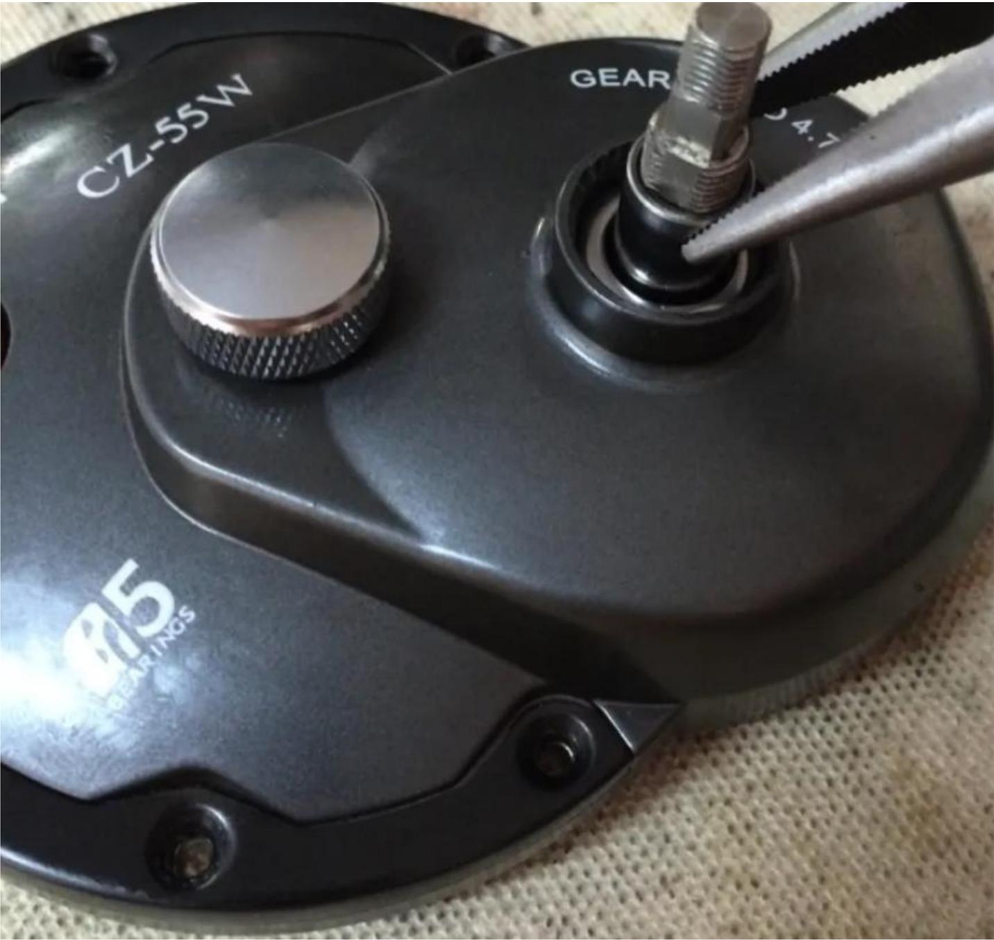
When pulling out the Spool Assembly (key# 400) from the Left Side Plate – Okuma calls this the Vice Side Plate (key# 300) be careful not to lose the Under Bearing Shim/Spacer/Washer (key# 302).
