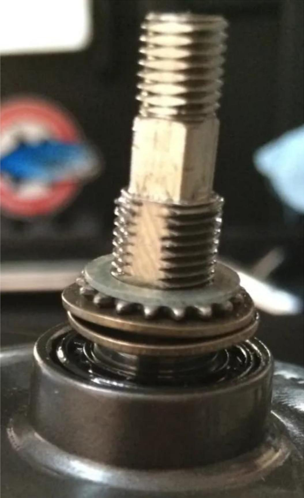
Remove the Spacing Sleeve – Okuma calls this another Drive Gear Shaft Bushing (key# 720)
