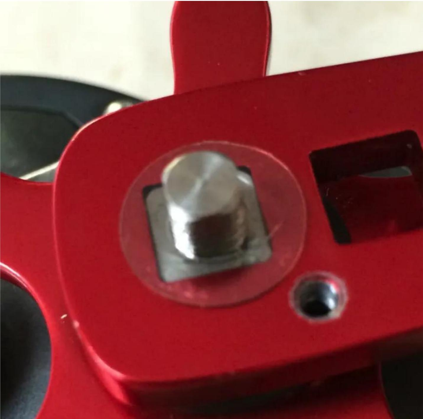
Lastly, install the Handle/Retainer Nut (key# 117) and Handle Screw (key# 515).
