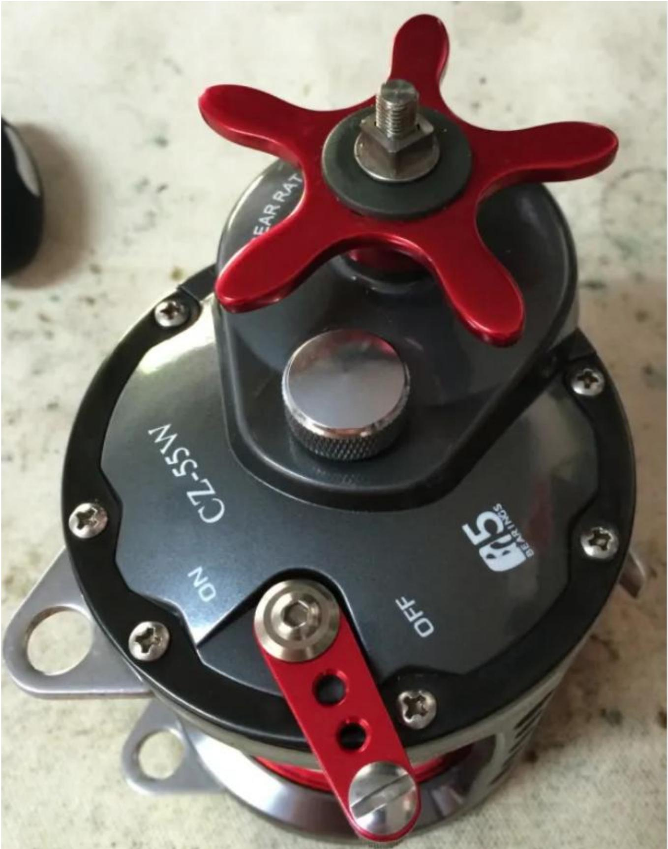
Now remove the Washer (key# 0920326), Click Gear (key# 401-2), Belleville Washers – Okuma calls these Drag Spring Washers (key# 609) & Drive Gear Shaft Bushing (key# 720-1)
