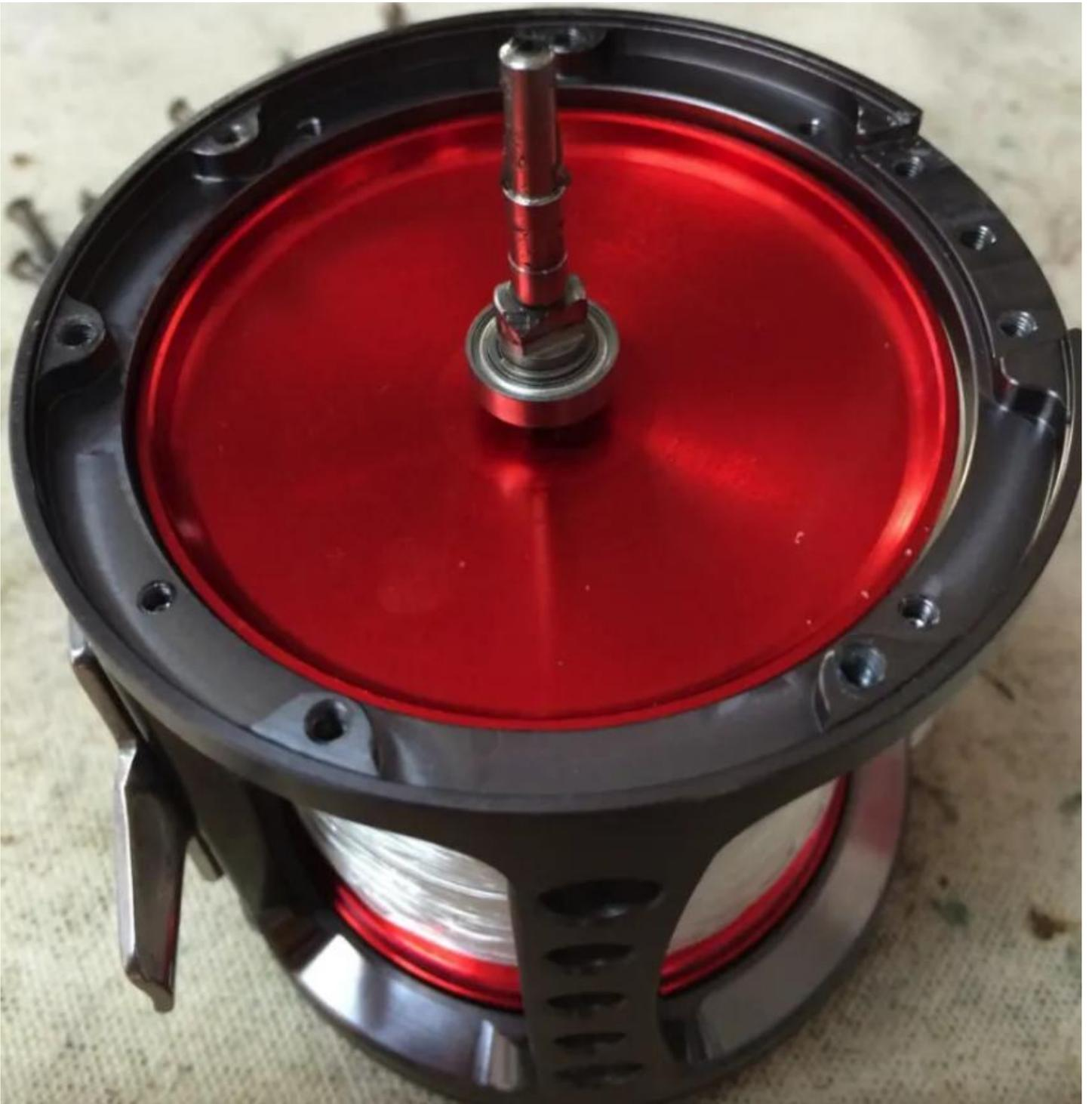
Notice the little knurl on the Handle Side Plate (key# 200), it tells you how to mate the Side Plate to the Frame/Main Body Assembly (key# 100). The knurl is where the Harness Lug/Hanger (key# 108) should go.
