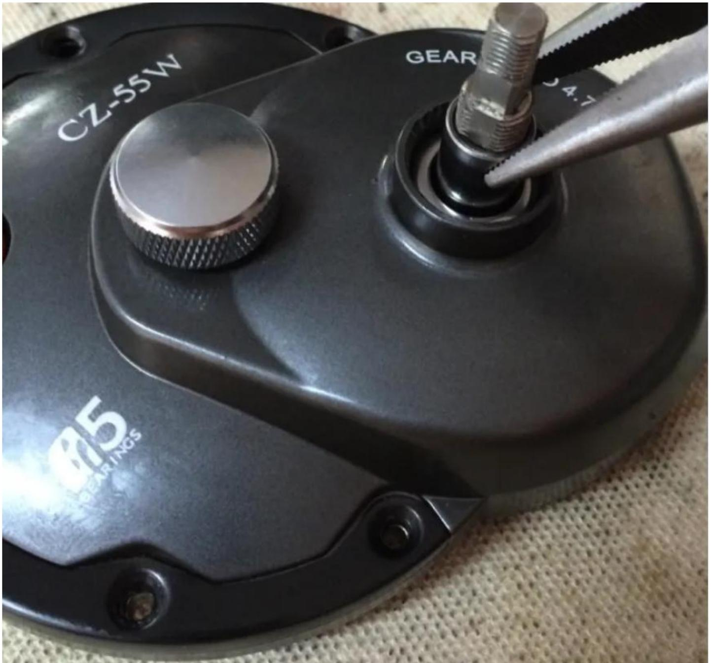
Now remove all 6 Screws (key# 09301224) which secure the Handle Side Plate (key# 200) to the Frame/Main Body Assembly (key# 100).
