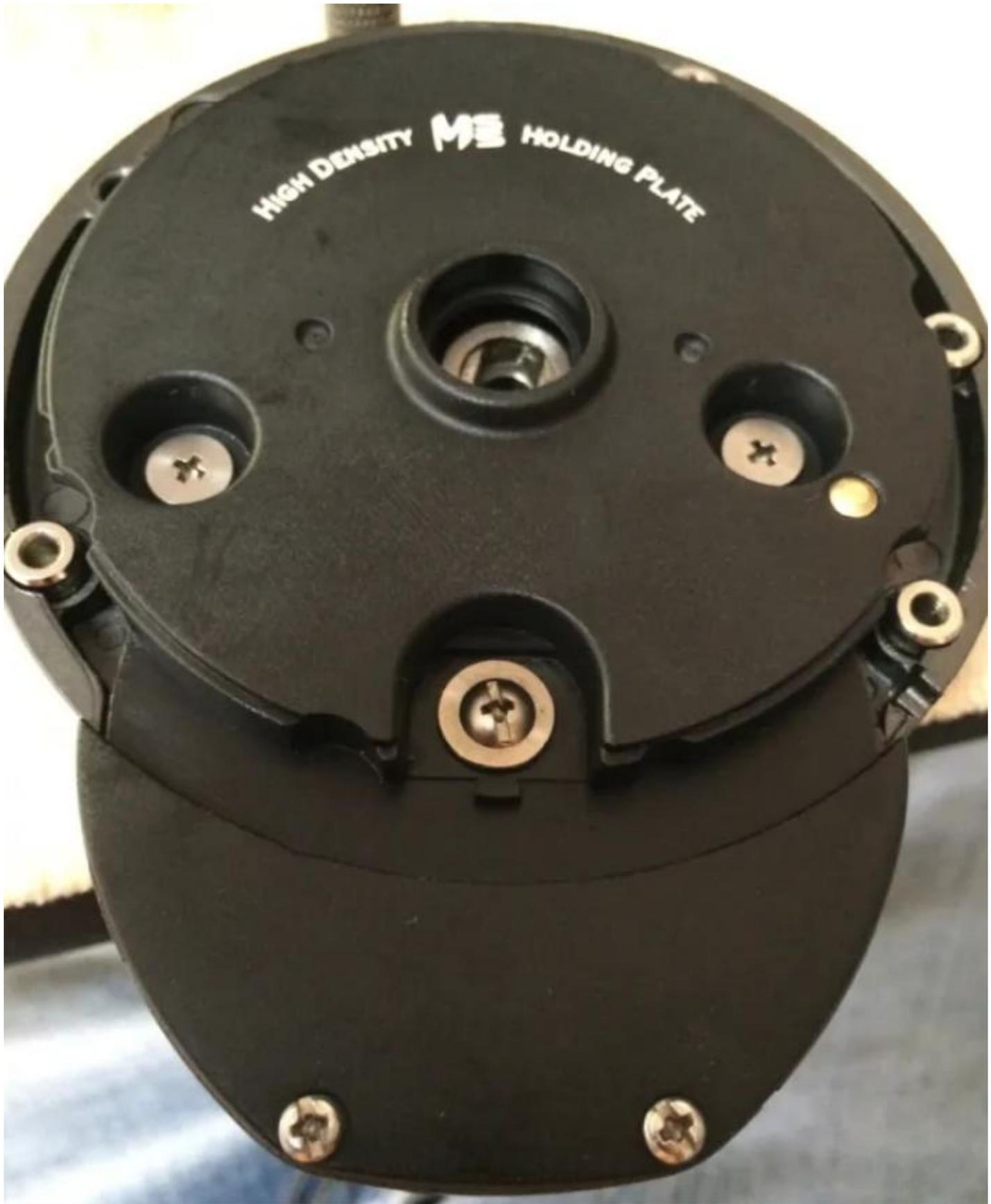
Turn the Handle Side Plate (key# 200) right side up and install the small Washer (key# 0920161).
