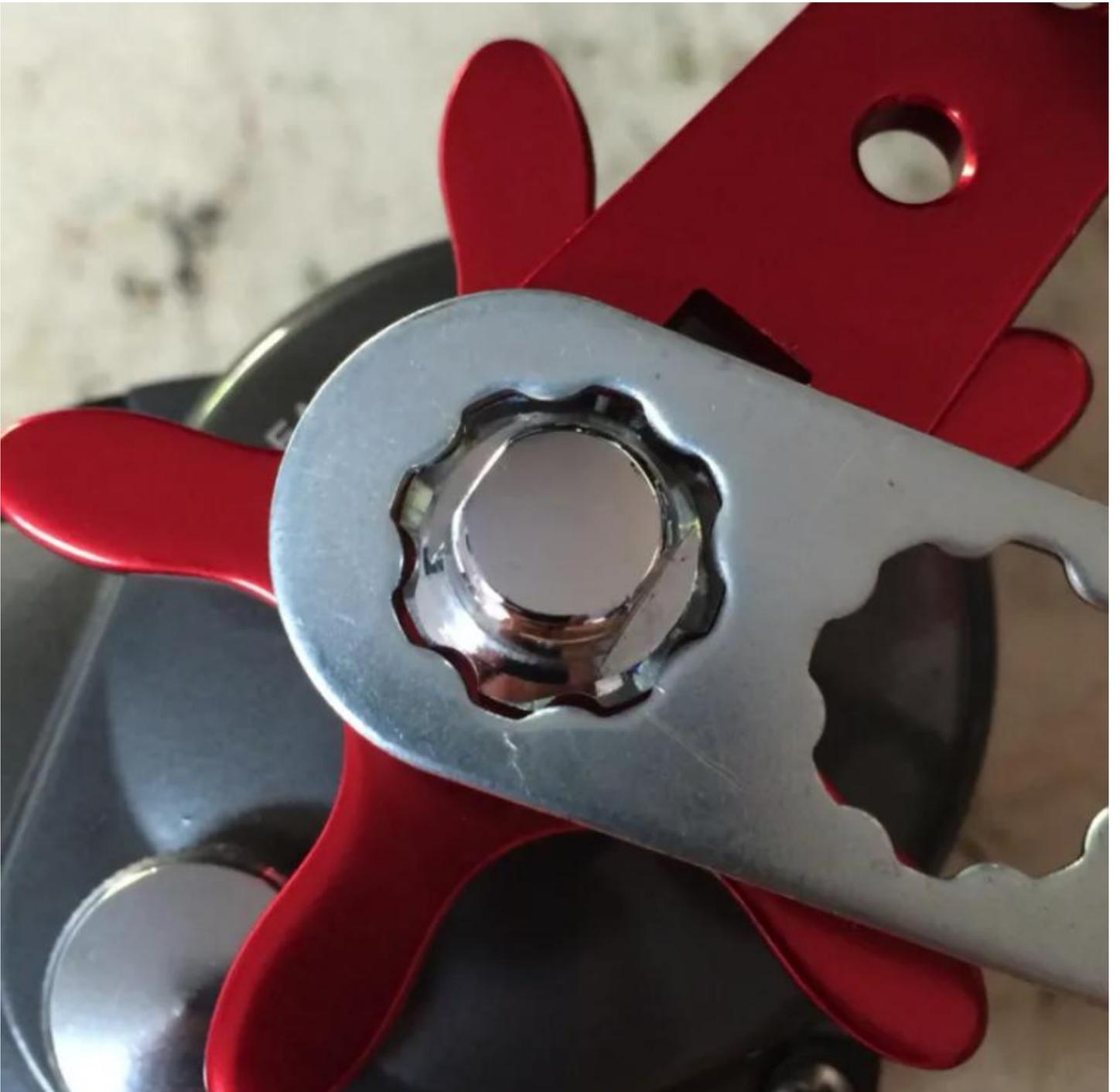
So, lacking the proper tool, I had to use Channel Locks to take the Handle Nut off. Make sure if you go this route, use some kind of material in between the handle nut and Channel Lock teeth to prevent marring. In this case, I just used a shop towel which seemed to do the trick.
