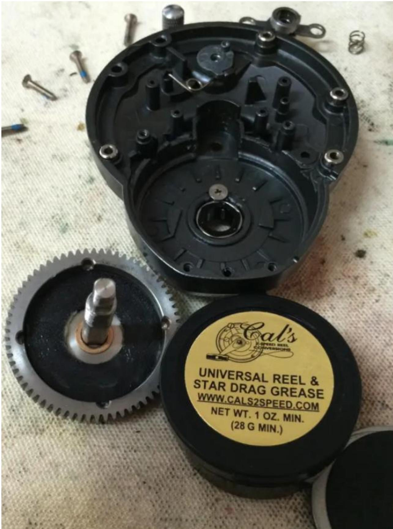
Notice the order of the Drag Stack - Keyed Drag Washer (key# 612-1), Small Hole Carbon Drag Washer (key# 610), Eared Drag Washer (key# 611), Small Hole Carbon Drag Washer (key# 610), Keyed Drag Washer (key# 612) & Big Hole Carbon Drag Washer (key# 610-1)
