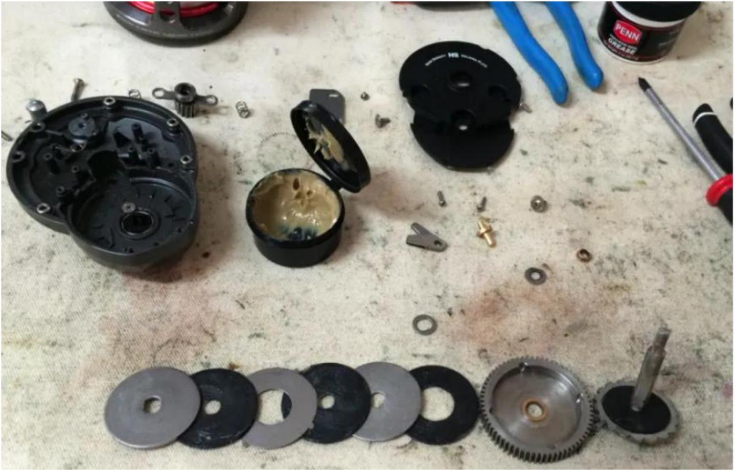
Now to reassemble..... Put the Under Drag Washer (key# 0920488), Main Drive Gear (key# 700) & Drag Stack – [(Top to Bottom) Keyed Drag Washer (key# 612-1), Small Hole Carbon Drag Washer (key# 610), Eared Drag Washer (key# 611), Small Hole Carbon Drag Washer (key# 610), Keyed Drag Washer (key# 612) & Big Hole Carbon Drag Washer (key# 610-1)] back onto the Drive Gear Shaft (key# 701) in the correct order and install it back into the Handle Side Plate (key# 200).
