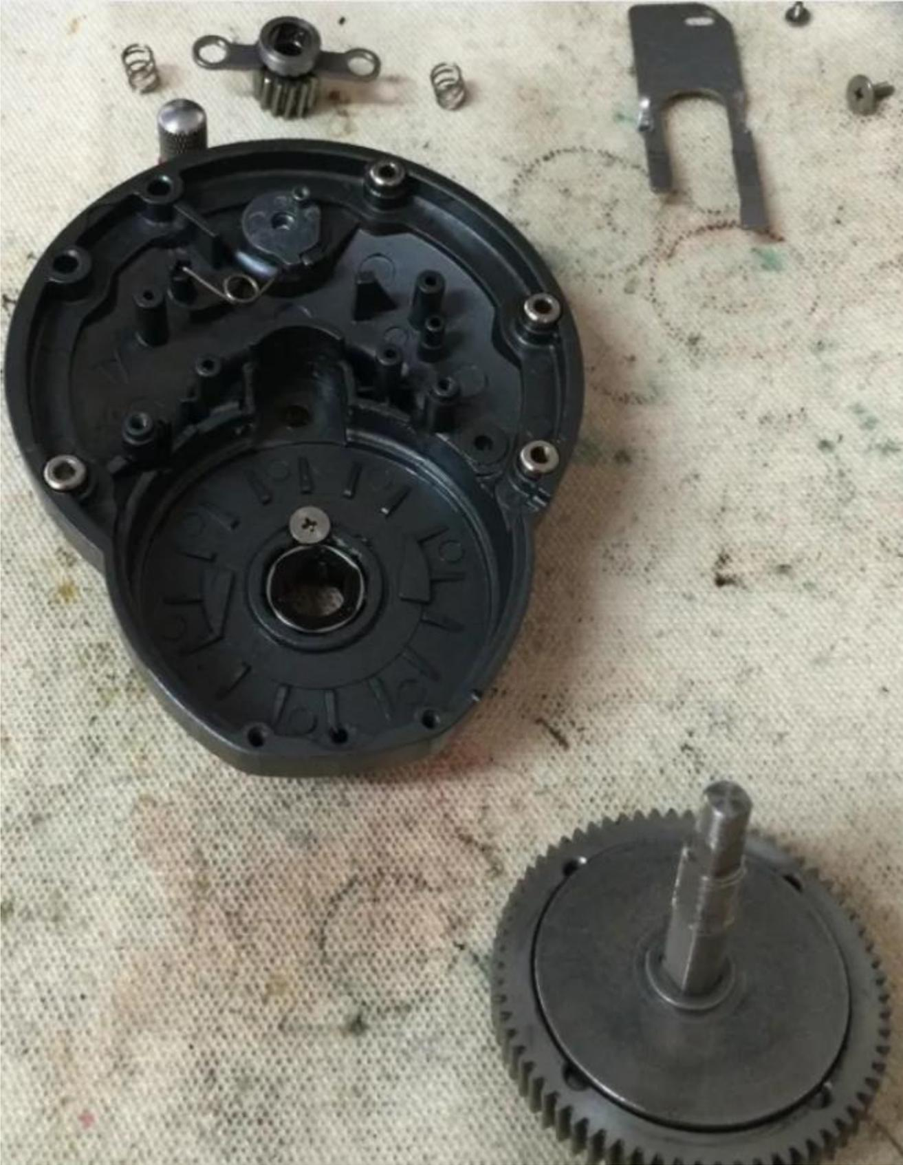
Take the Main Drive Gear (key# 700) off of the Drive Gear Shaft (key# 701) along with the Under Gear Drag Washer (key# 0920488). Then remove the Drag Stack (Keyed Drag Washer (key# 612-1), Small Hole Carbon Drag Washer (key# 610), Eared Drag Washer (key# 611), Small Hole Carbon Drag Washer (key# 610), Keyed Drag Washer (key# 612) & Big Hole Carbon Drag Washer (key# 610-1)) and Top Keyed Washer (key# 612-2).
