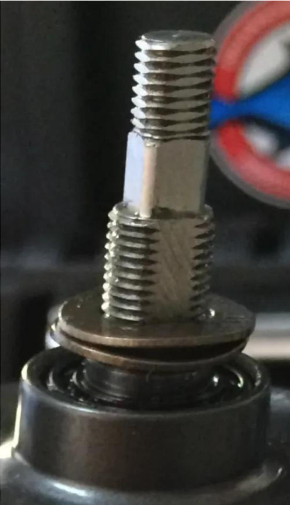
Install the Click Gear (key# 401-2) and Washer (key# 0920326)
