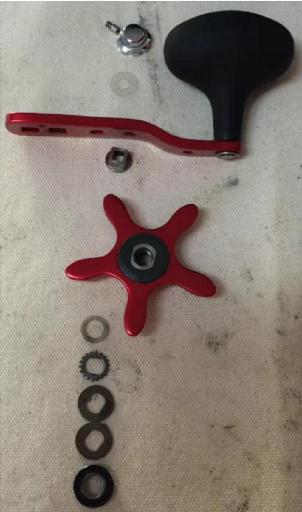
Install the Drive Gear Shaft Bushing (key# 720-1) then the Belleville/Drag Spring Washers (key# 609) – Notice the way the Bellevilles are positioned “()”.
