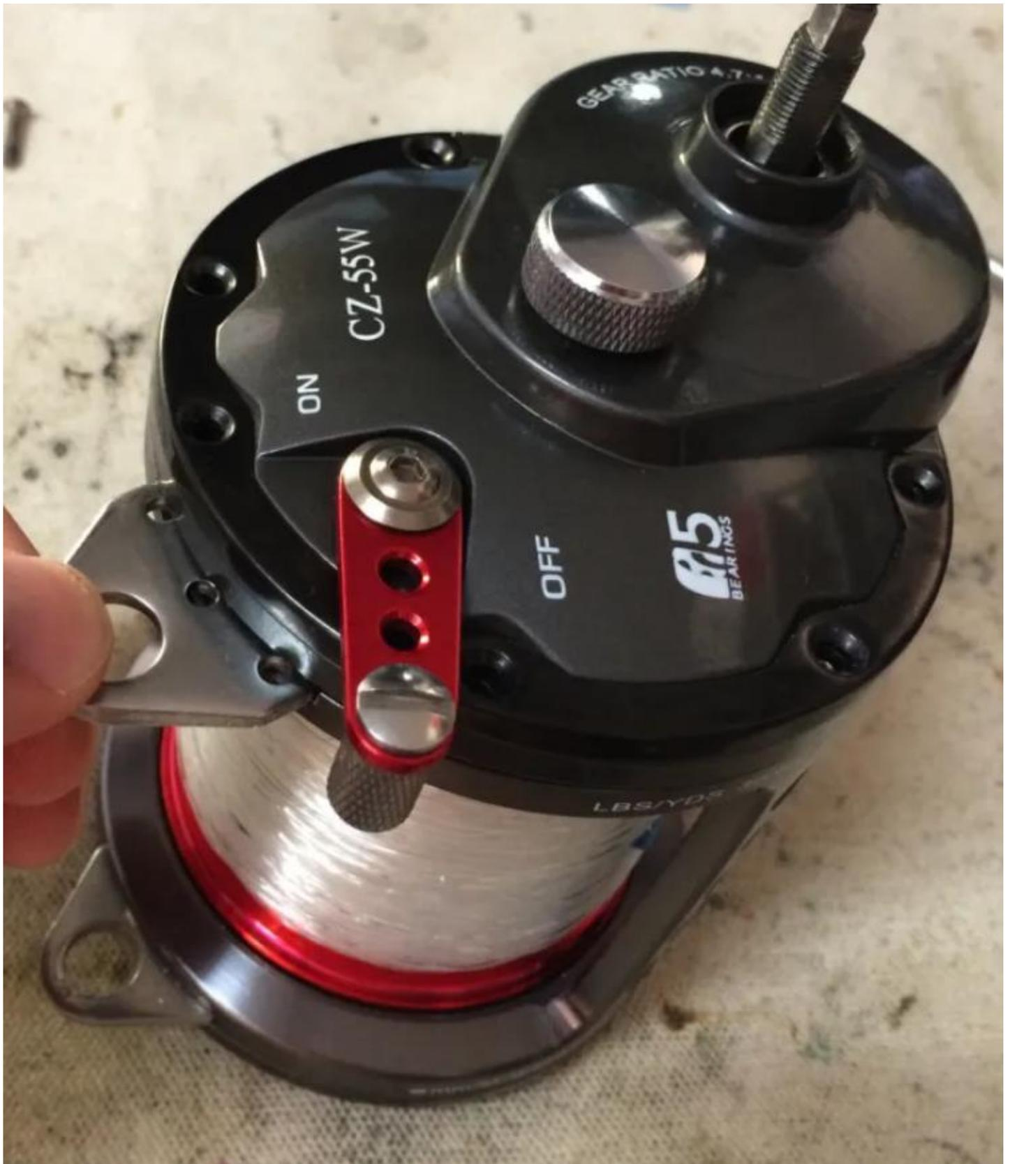
Just a pic of the High Density Holding Plate aka Holded Plate (key# 207) in Okuma lingo, which holds all the internals together so be careful when removing it.
