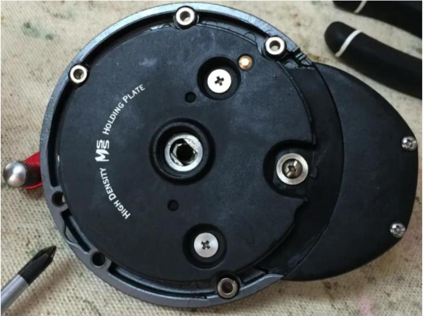
Install the Handle Side Plate (key# 200) back onto the Frame/Main Body Assembly (key# 100) with the 6 Screws from earlier (key# 09301224) taking note of the Harness Lug/Hanger (key# 108) position.
