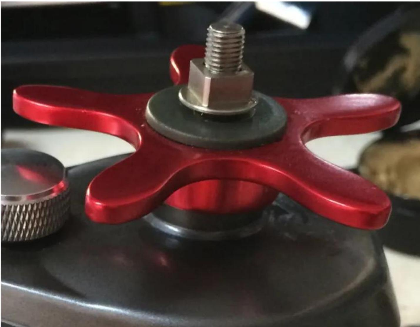
Install the Handle Assembly (key# 500) and Plastic Washer (key# 0920133).
