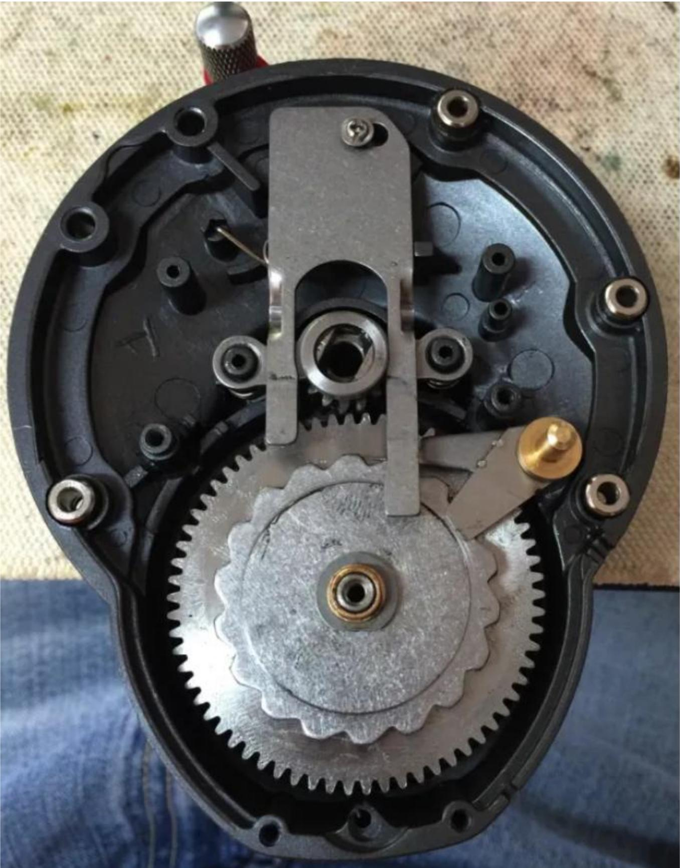
Remove the Eccentric Jack Screw/Clutch Slider Screw (key# 0930194) & Eccentric Jack – Okuma calls this a Clutch Slider (key# 804).
