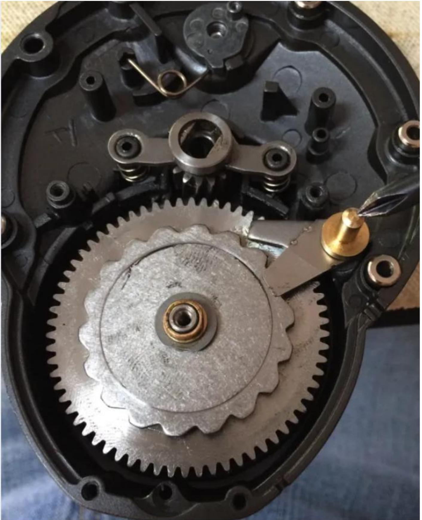
Remove the Pinion Gear Assembly (key# 702), Pinion Gear Yoke (key# 805) & Yoke Springs (key# 806), Main Drive Gear (key# 700) & Drive Gear Shaft (key# 701).
