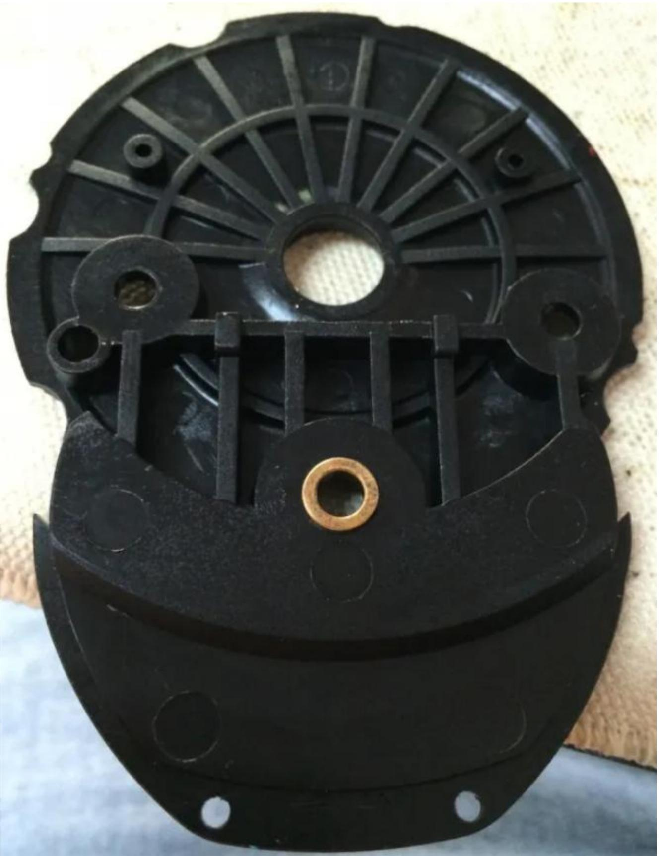
Put the Holded Plate (key# 207) back onto the Handle Side Plate Assembly (key# 200). Make sure everything lines up.
