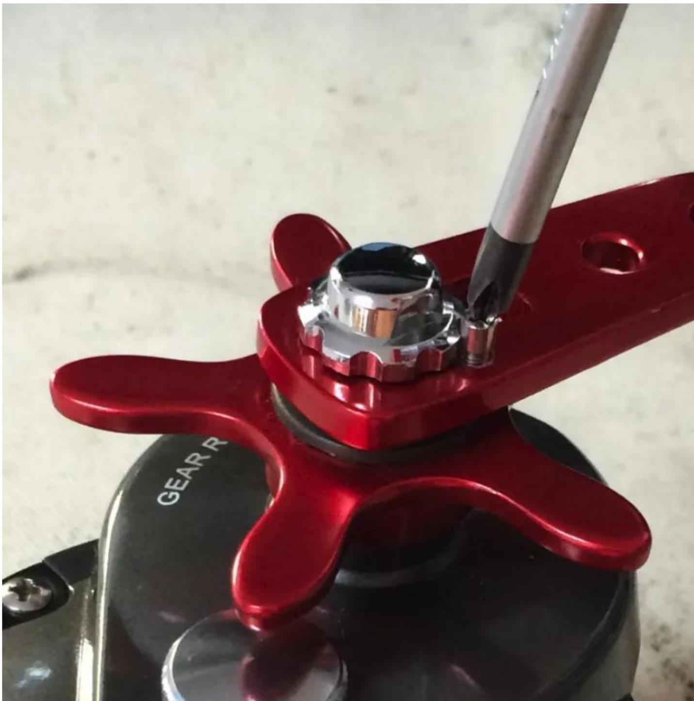
DONE! I didn't show pictures of it but during reassembly I put a thin layer of grease between the Frame, Sideplates & Frame Rings – Okuma calls these Side Plate Covers (key#'s 208 & 311) on both sides as well as some grease in all of the screw holes.
