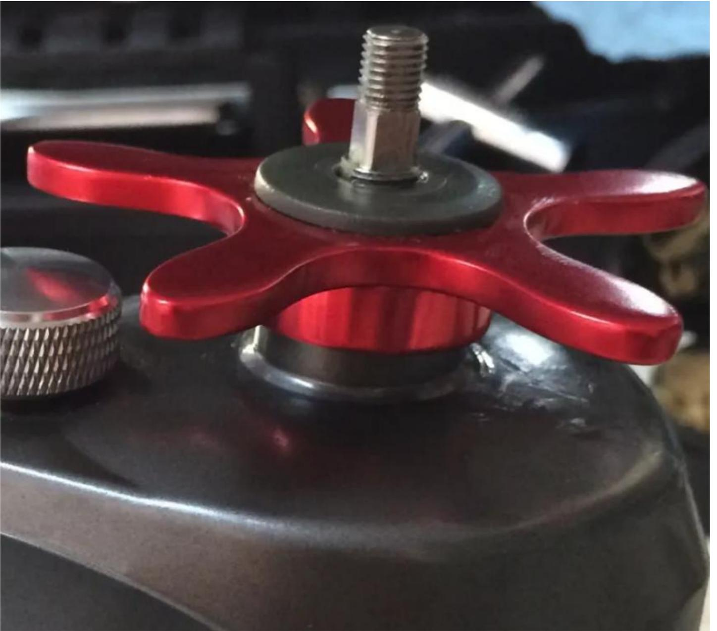
Install the Keyed Handle Bushing/Drag Washer (key# 520).
