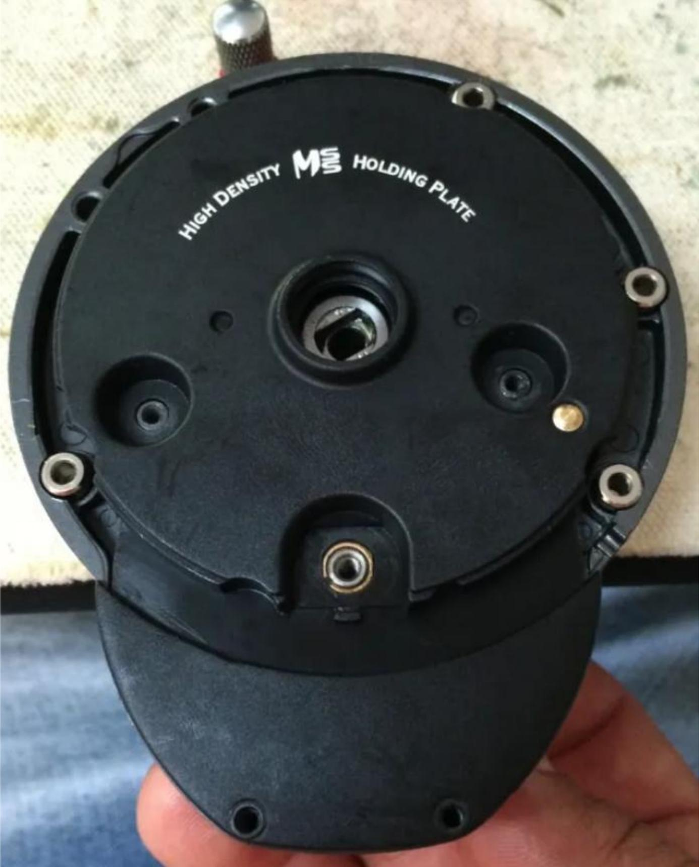
Take the 5 Screws from earlier [(2x key# 0930060)(2x key# 0930651) & (1x key# 0930202)] and lock down the Holded Plate (key# 207) & Drive Gear Shaft (key# 701). You may need to install the Handle Bushing/Drag Washer (key# 520) and Handle Assembly (key# 500) to lock down the Drive Gear Shaft Screw (key# 0930202).
