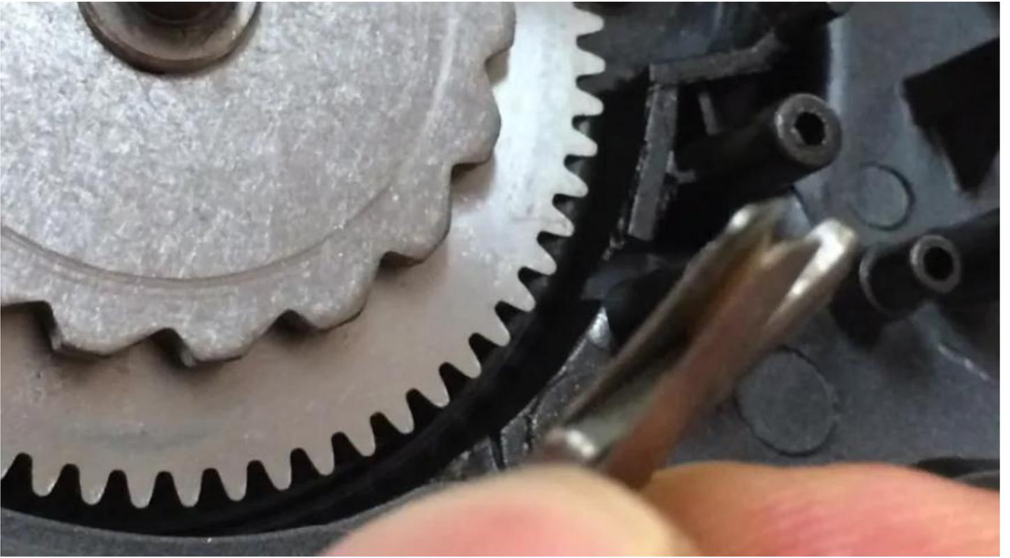
Install the Yoke Springs (key# 806), Pinion Gear Yoke (key# 805) & Pinion Gear Assembly (key# 702).
