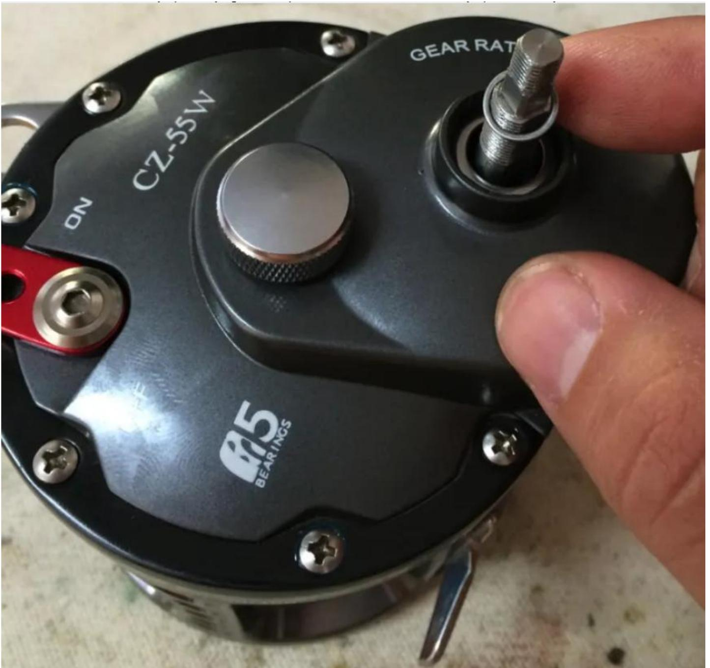
Install the Spacing Sleeve/Drive Gear Shaft Bushing (key# 720).
