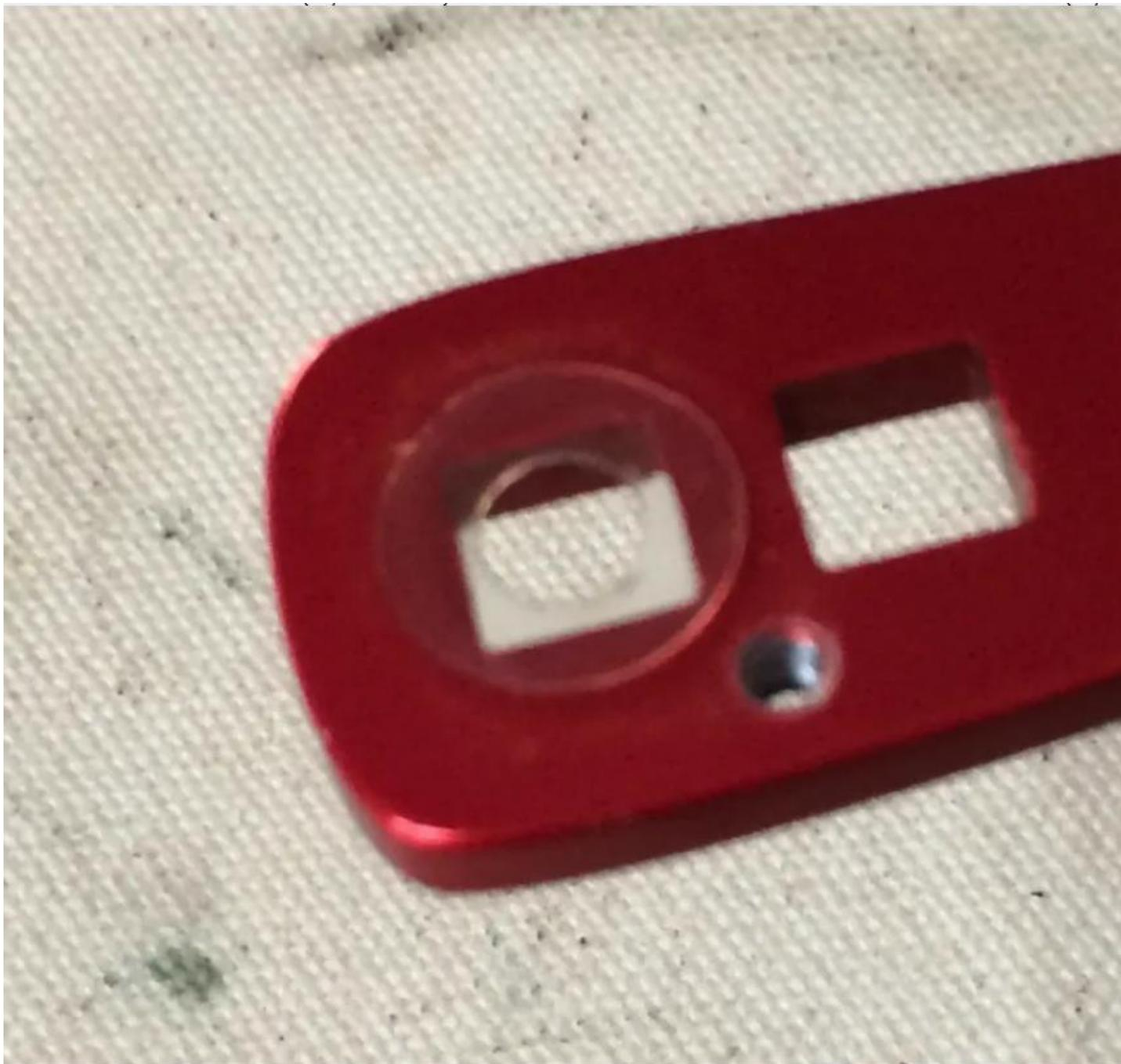
Next remove the Keyed Handle Bushing - Okuma calls this a Drag Washer (key# 520) and Star Drag Assembly (key# 615)
