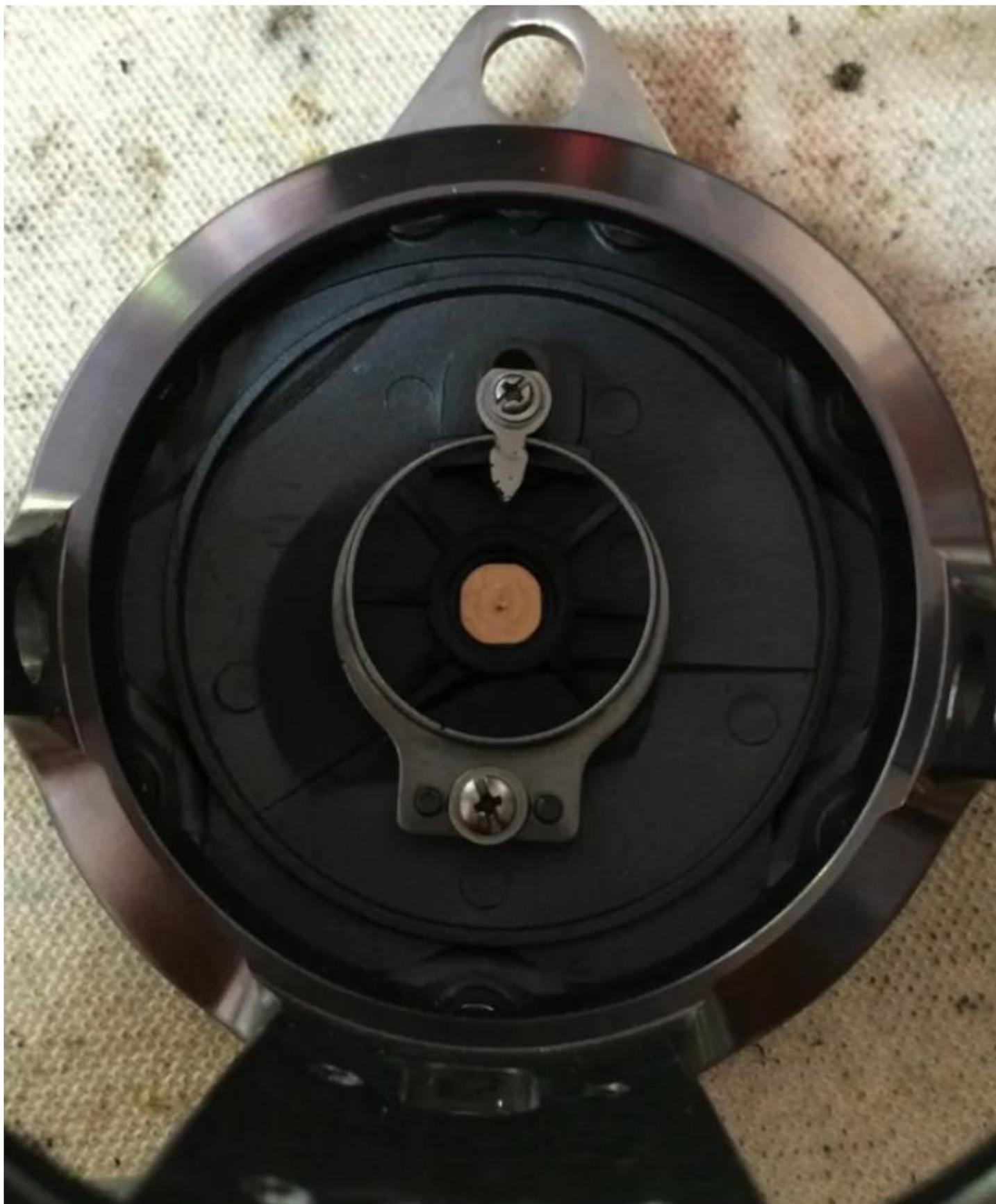
Just a pic of the Spool Shaft with its Bearing (key# 0910278).
