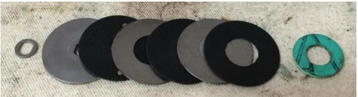
Since the Drag Washers were out anyway, I figured I'd just grease them up with some Cal's. Don't forget to put some grease on the Anti-Reverse Bearing (key# 0910153).
