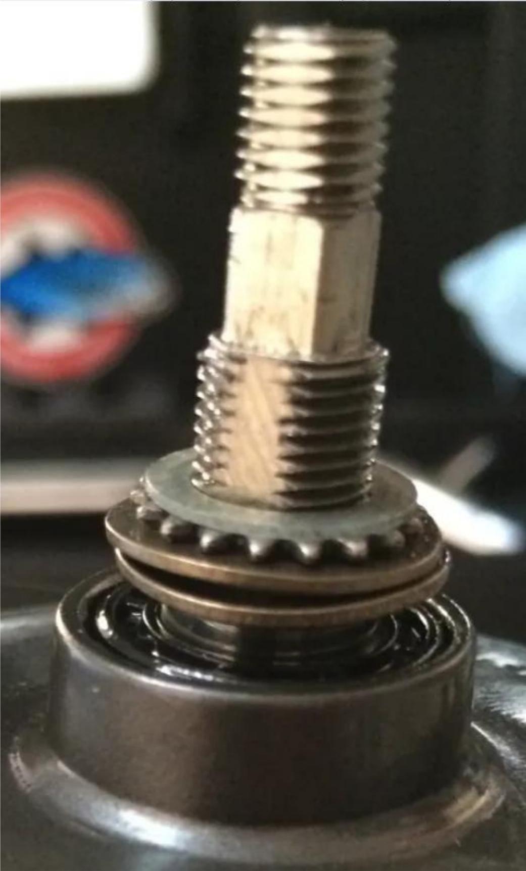
Install the Star Drag Assembly (key# 615).
