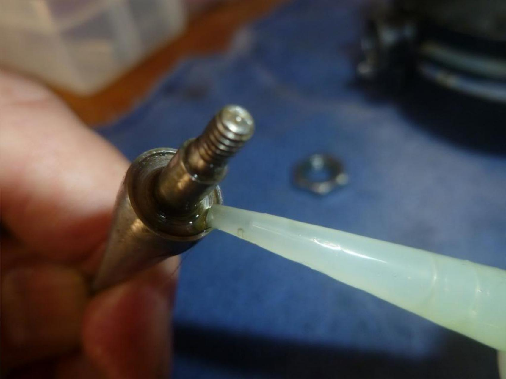
The other end of the Bail Arm is straightforward and similar to replace. Both have to have their springs compressed to allow replacement of their Bail Arm Screw. It's really the only "fiddly" bit on the whole reel. I found it slightly easier if you remove the Bail Release Arm (28) first and the whole removed assembly is shown for your reference. The Arm itself sits in the Bail Release Saddle (28A), pivoting on the Bail Release Pin (29) with the action provided by the Bail Release Spring (30):
