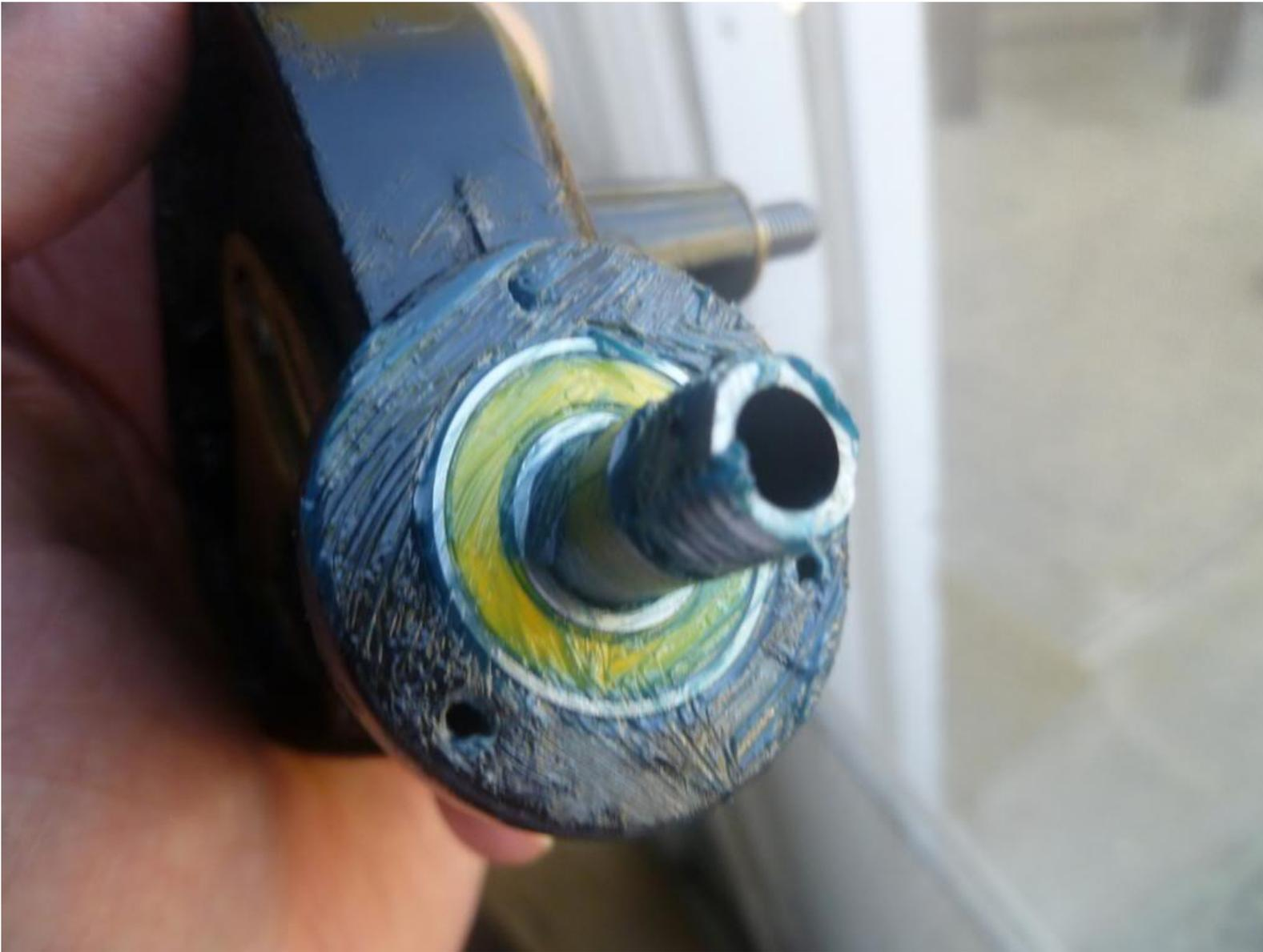
Then replaced the Retainer and Brake. This did not photograph well with a flash but the retainer is well cleaned up with Brasso and a tooth brush and very superficial tarnish remains. It was all replaced well greased:
