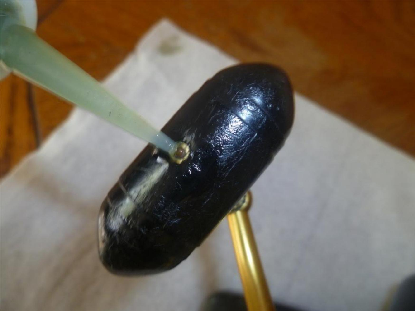
Lastly, we have the Spool (47) with the drag stack removed. This was cleaned then re-lubed with Cal's Drag Grease:
