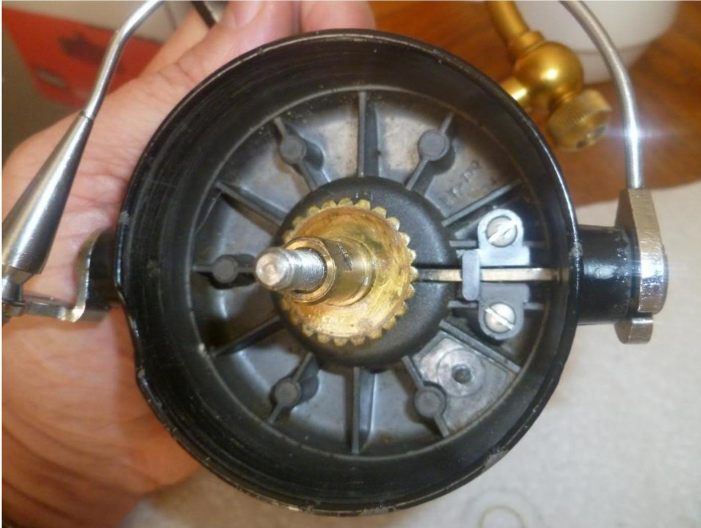
Hmm, looking good...but to remove the Spool Shaft we have to crack the body via the Housing Plate (45) and it's 3 Housing Plate Screws (46):
