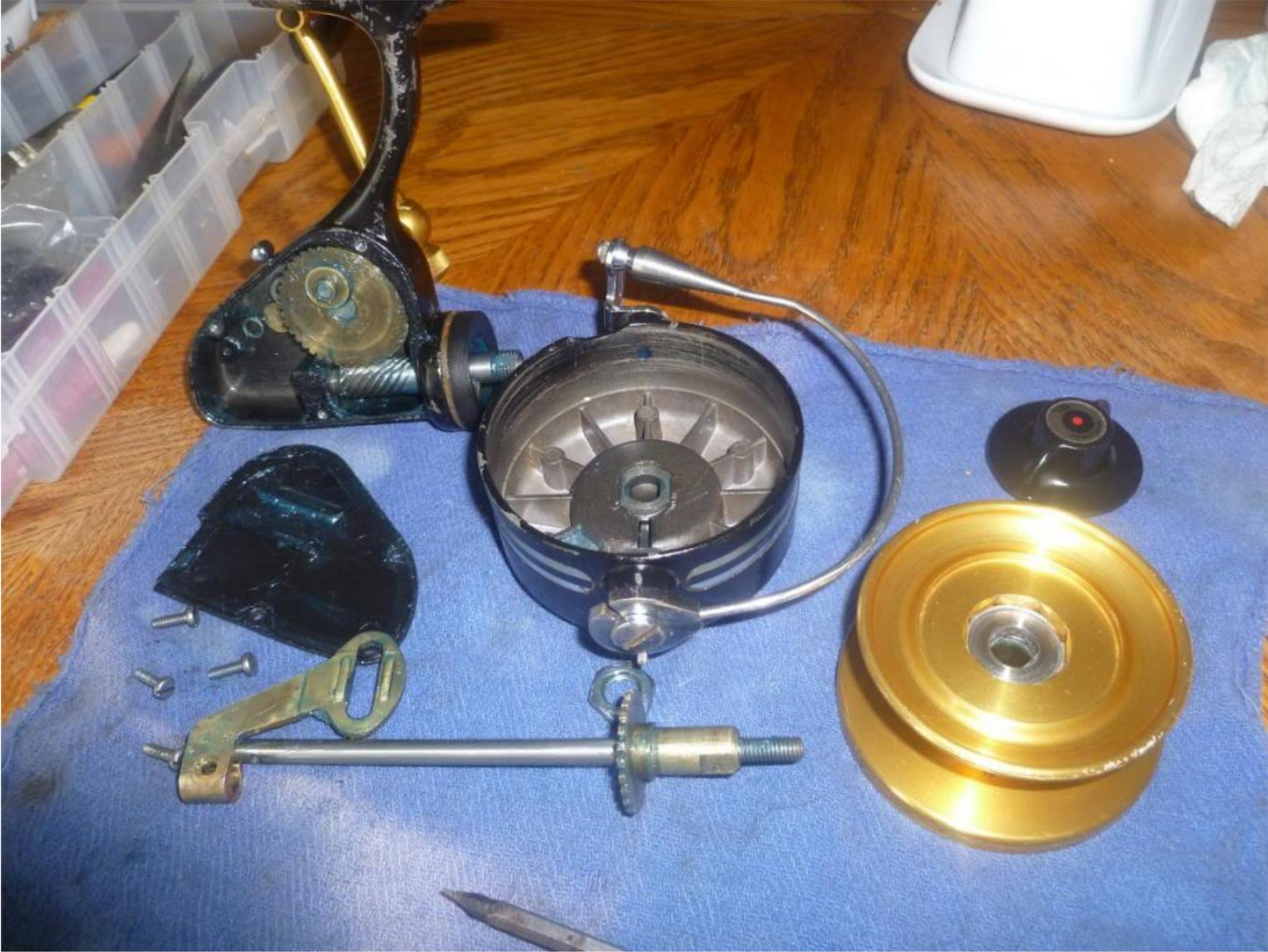
Let's start with the Rotor Cup. Needless to say this is an older design that predates carbon fiber rotors and skirted spools. We can start with the Bail Assembly by servicing the Bail Arm (34) by removing the Bail Arm Screw (31):
