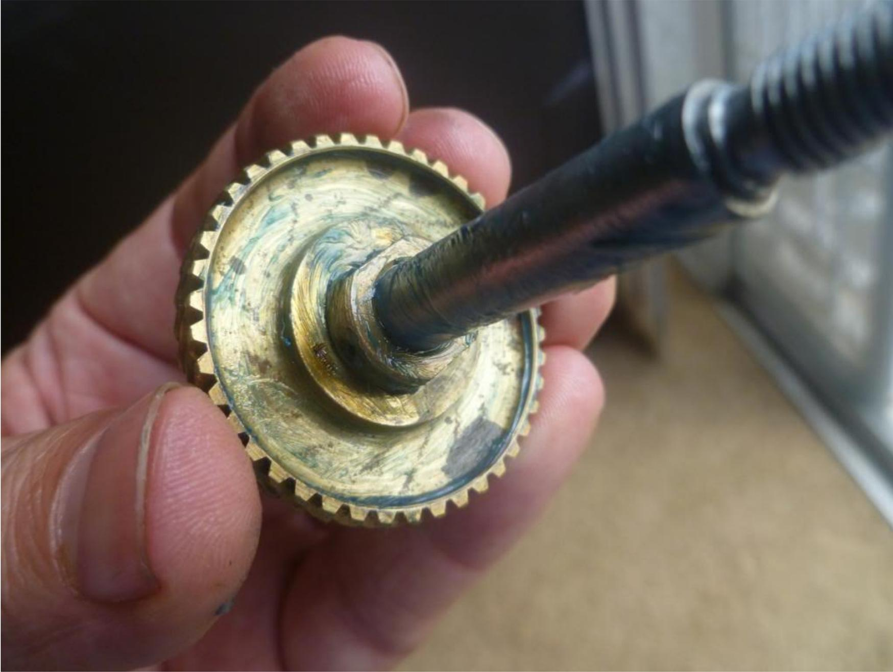
This is the Housing with the old grease cleaned out showing the Eccentric (21) assembly. It was in perfect working condition so did not remove it and all it got was a scrubbing with a toothbrush saturated with Corrosion-X. This image is all you should need for assembly. From L to R we have the Eccentric Spring (6D) in proper position leading to the Eccentric (21) with its Eccentric Liner (6D, underneath), the Eccentric acts on the Dog (4) which rests on its Dog Spring (5):
