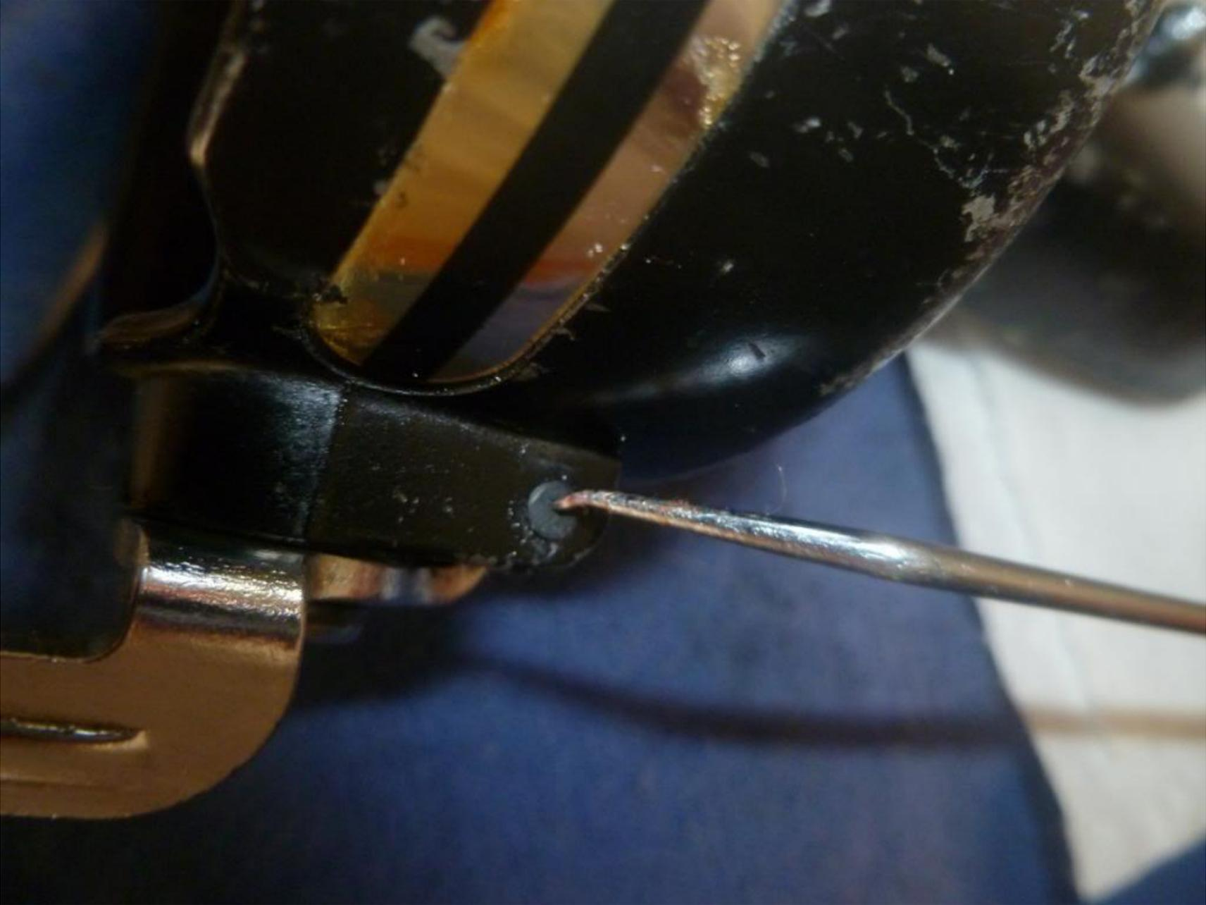
The Line Roller (35) is simplicity itself, removed via the Bail Lock Nut (36) finding the tiny Roller Sleeve (35A) inside:
