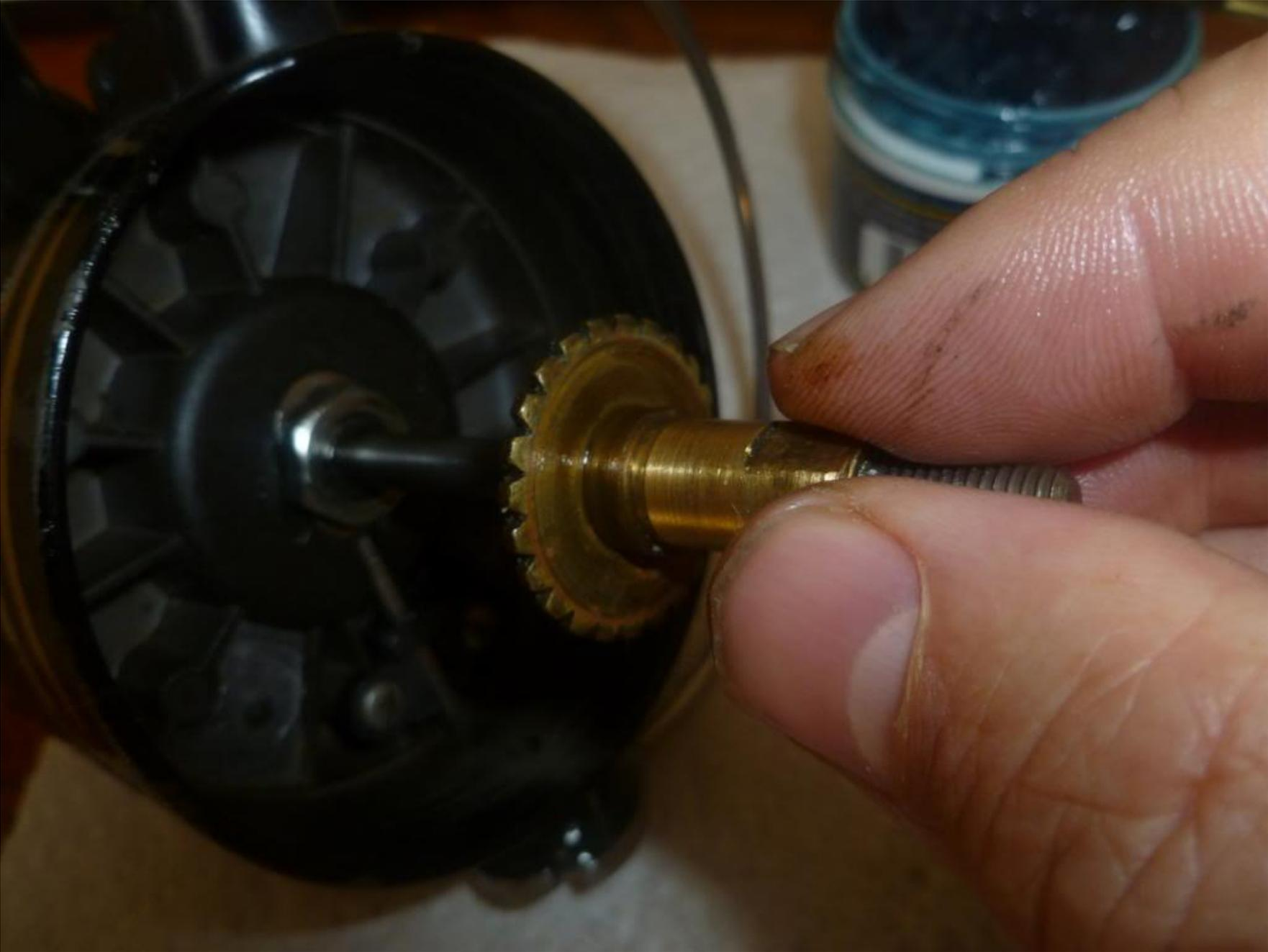
Which gives us access to the Rotor Cup Nut (38) with the Rotor Cup Washer (37) underneath:
