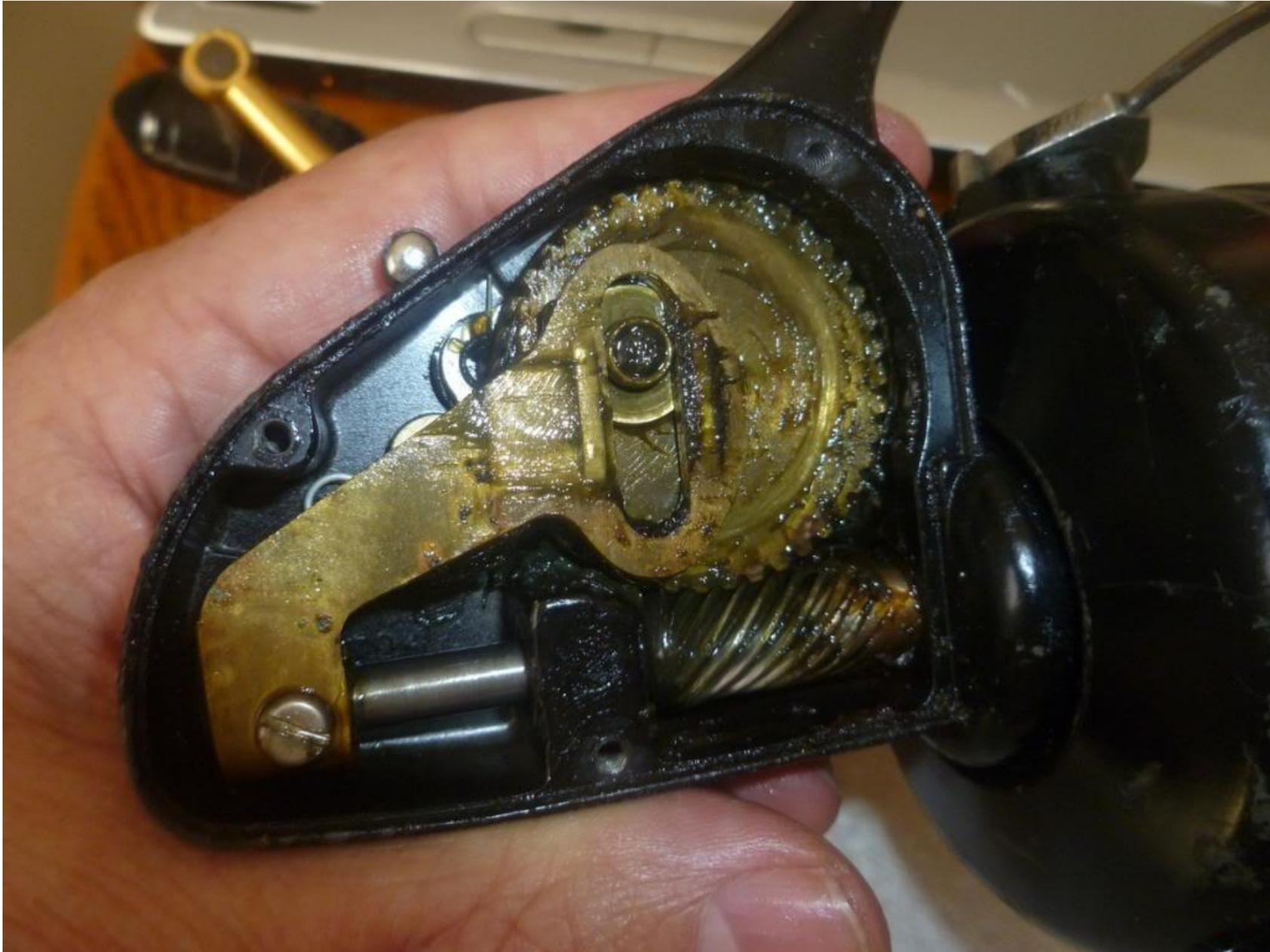
Then, the Spool Shaft disconnects from the Crosswind Arm (43) via the Crosswind Arm Screw (44):
