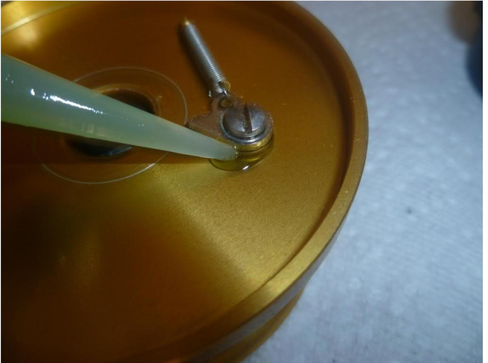
Nothing to take apart in this older style knob. A touch of oil for corrosion resistance is all that is needed. I believe that the newest style has increased water resistance to keep the stack dry:
