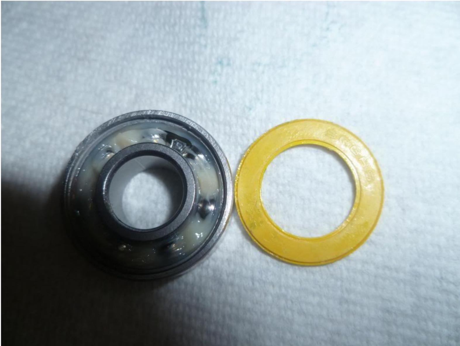
So I repacked it properly. Ceramic balls will not rust, but we want to protect the stainless races/cage and not create a path for saltwater to flow into the body.
