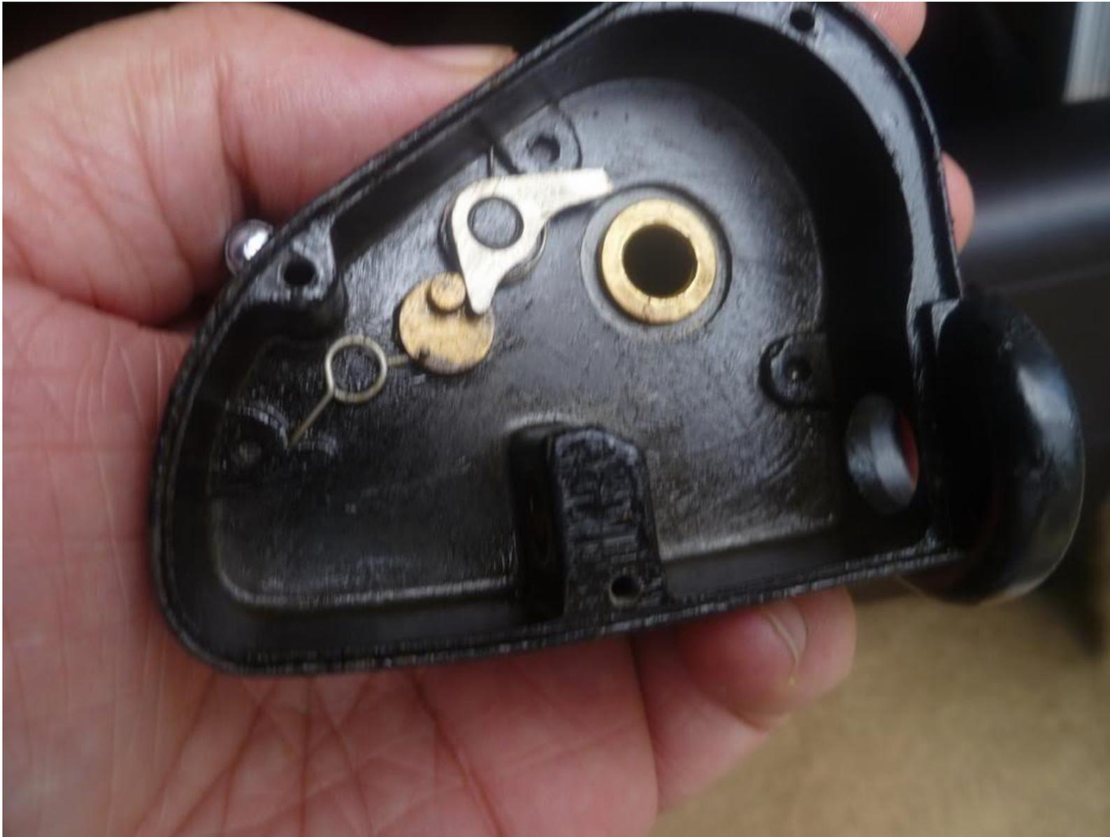
To the right of all of that above is one of the brass Bushings (2) that support the handle shaft which had not the slightest wear. I believe these are pressed in the Housing and should rarely need anything more than lube.
