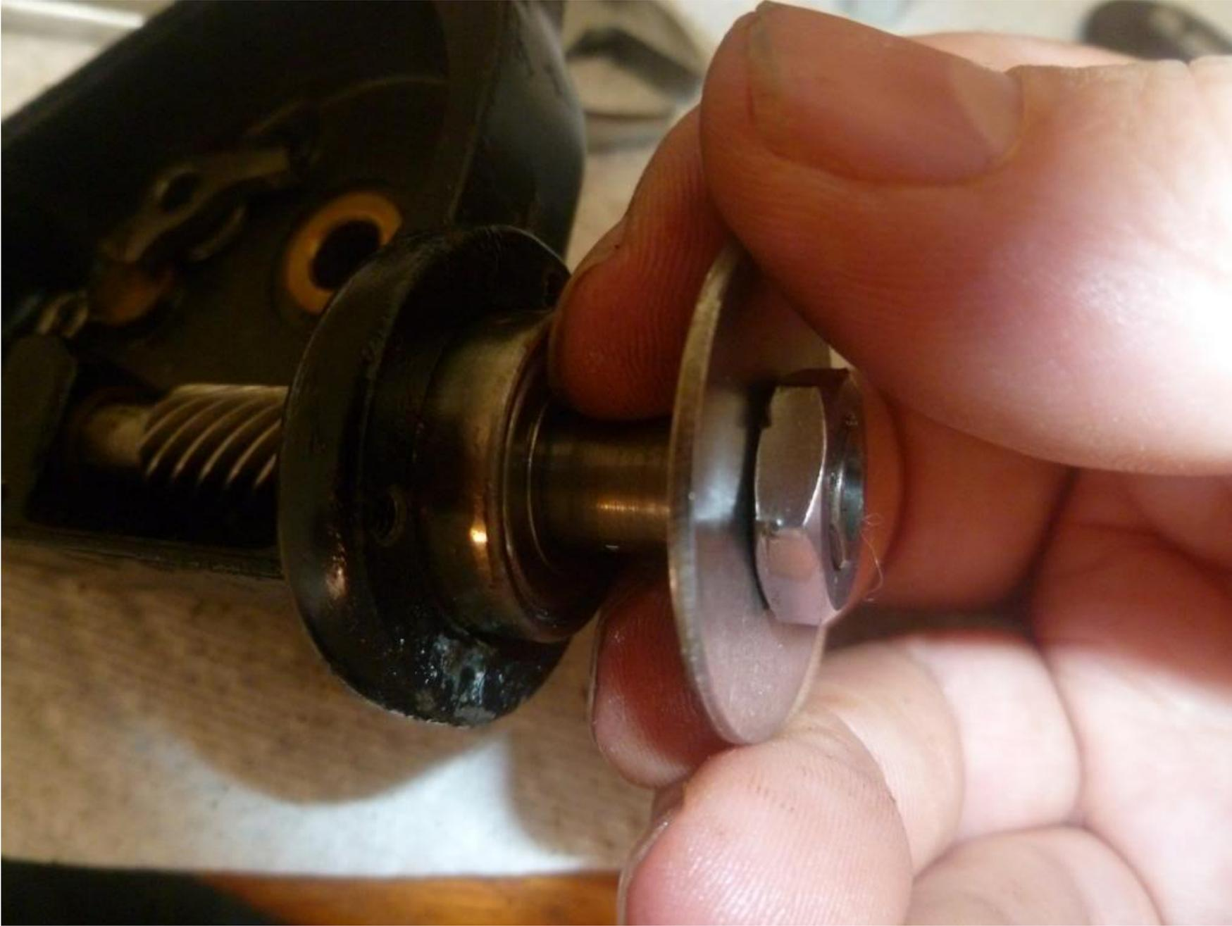
The inner race was frozen and the bearing destroyed, but I was curious so I pulled the shield:
