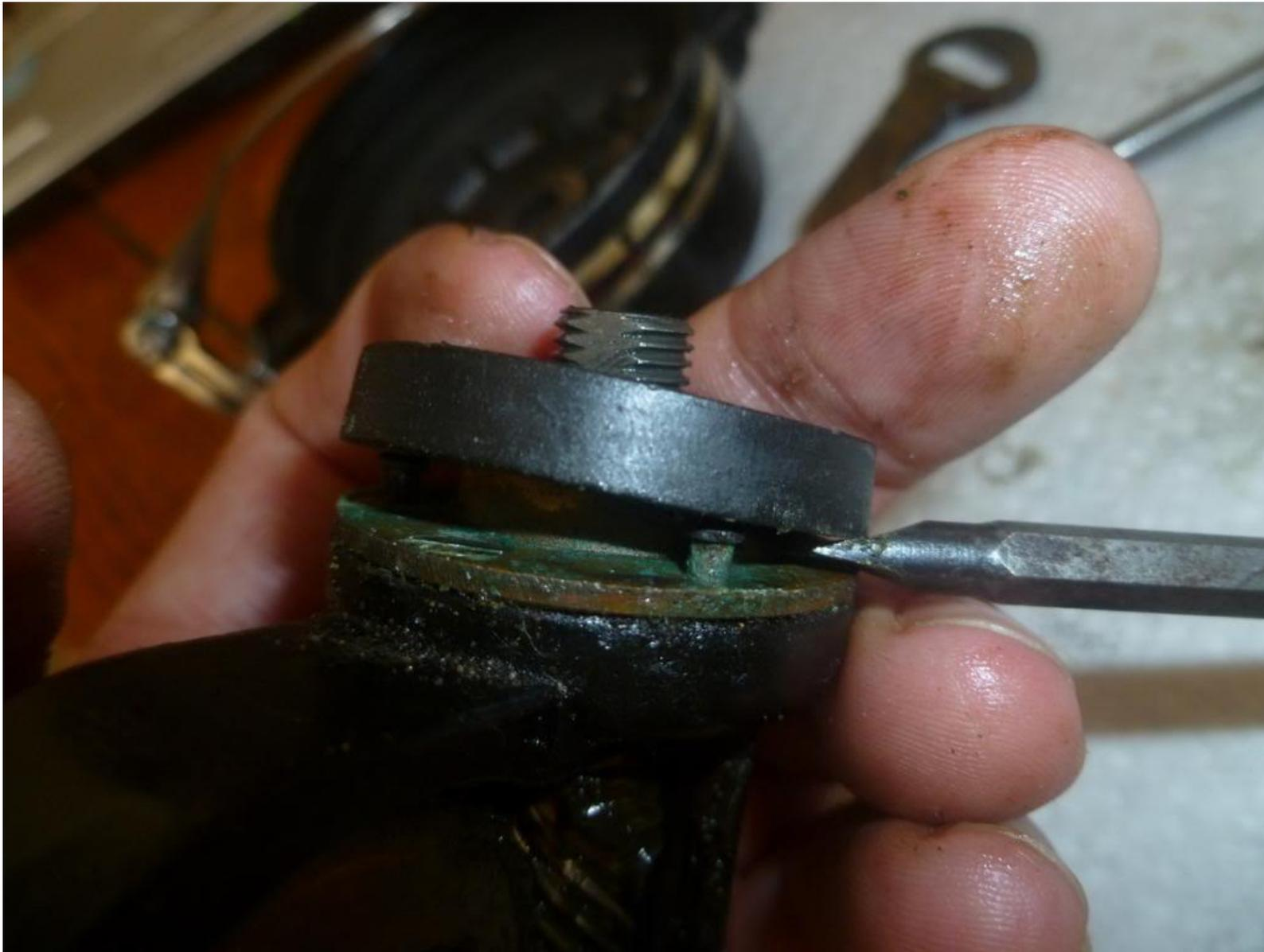
Revealing the pinion Bearing Retainer (21A):
