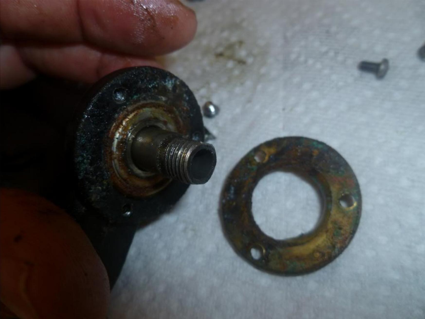
A washer for the 3/8" diameter pinion and replacing the Rotor Cup Nut helped me get a grip on it as it was frozen in its receptacle:
