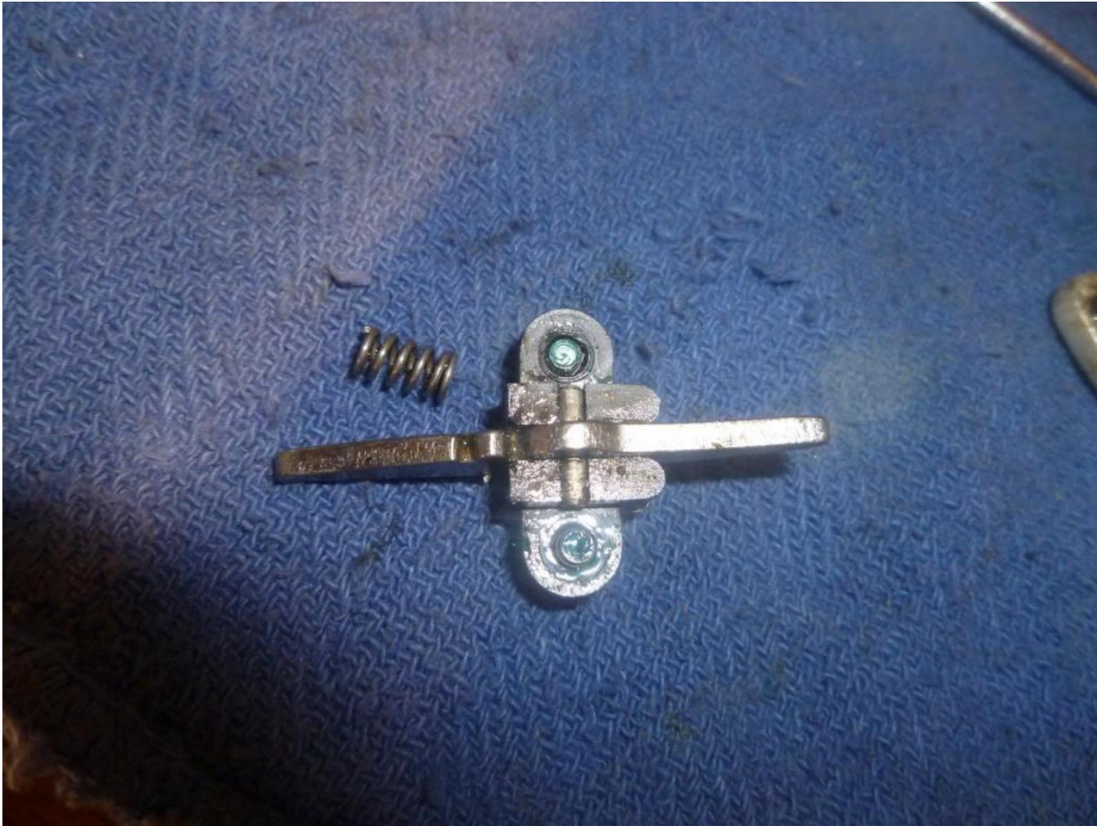
Once you remove the Release Arm you'll find a natural spot to collect dirt and sand. Note the little post in the Rotor Cup that supports the Bail Release Spring when you re-assemble:
