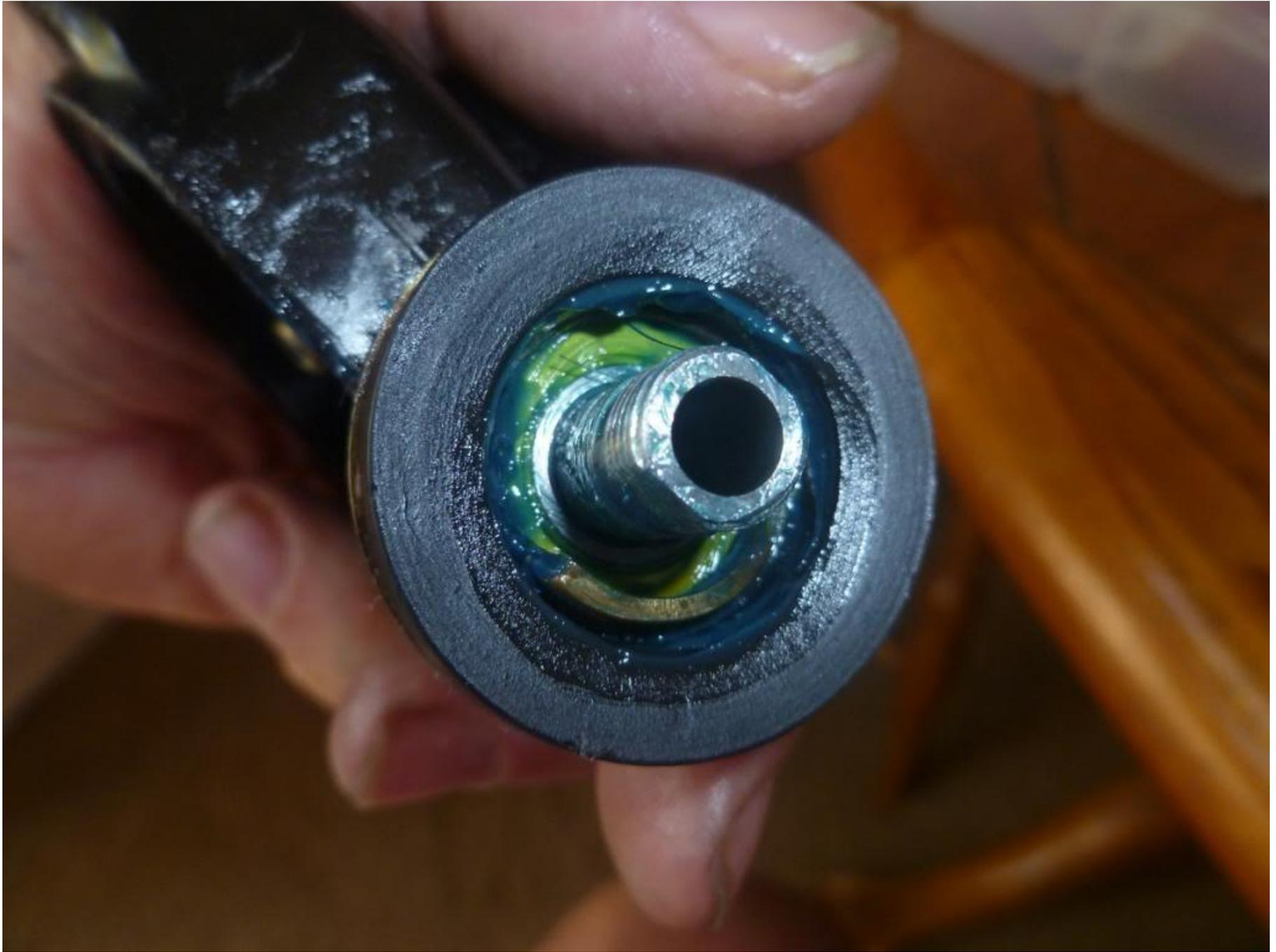
On the other side We can easily pull out the Main Gear 😊, Ratchet (10) and Main Gear Thrust Washer:
