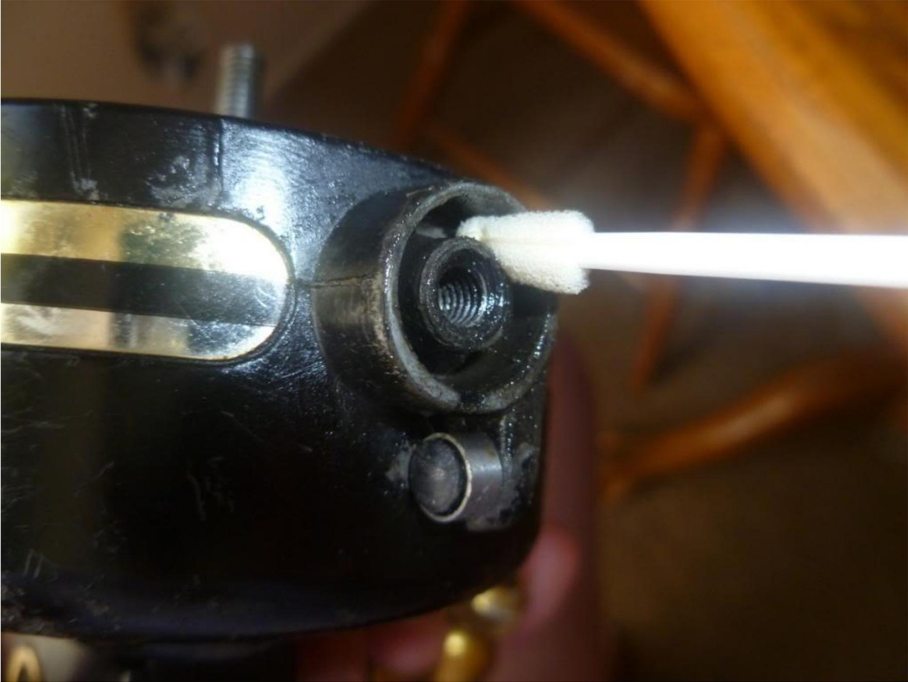
Beneath the foam “q-tip” is the Bumper (33) and its cup. If yours is beat up it simply pokes out from the other side with a probe then can be replaced (this one I did):
