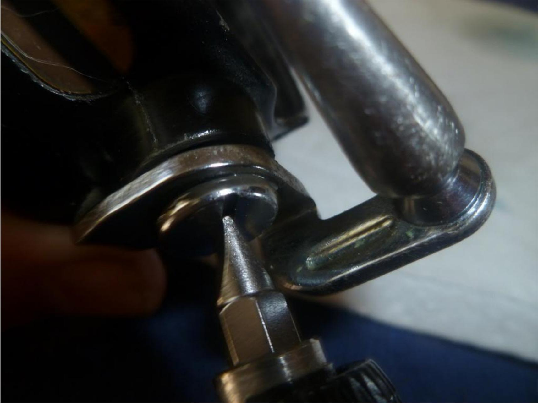
Finding the Bail Spring (32) below. Usually you will find that the Spring will come off with the Arm and with one of its ends in the tiny hole in the Arm, but I show the Spring in its proper position for your reference:
