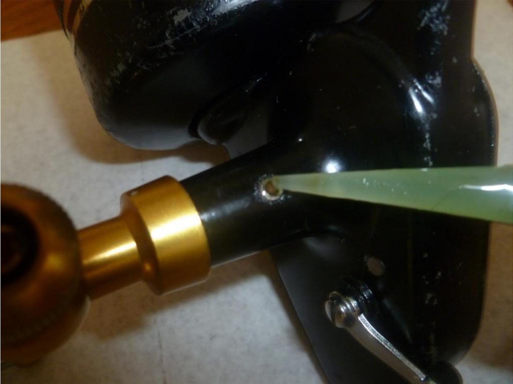
The handle needs a little (very little) attention. Just make sure that the Handle Washer (17) and threads on the end of the shaft connecting to the Main Gear get some marine grease, the threads and articulating surfaces of the Handle (14) get Corrosion-X.
