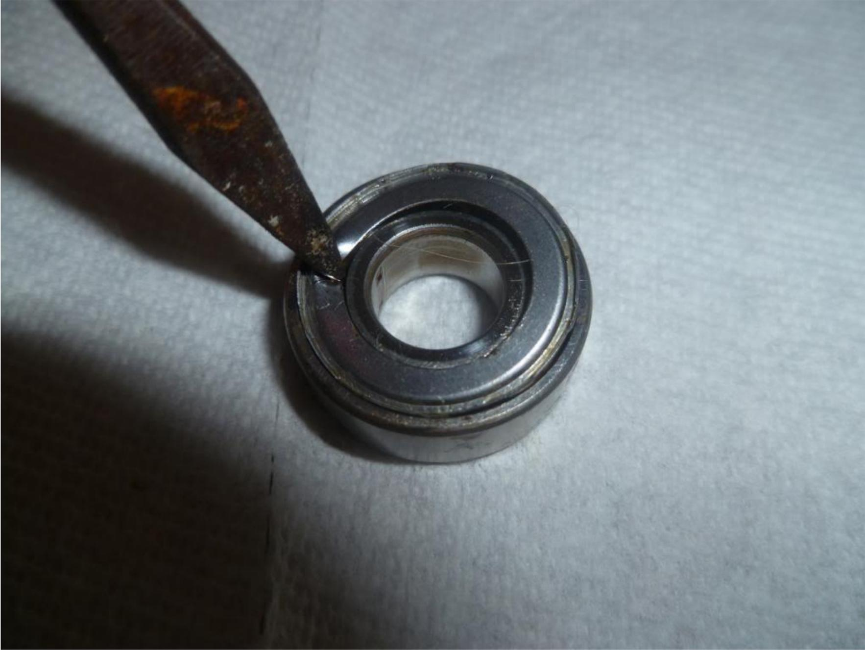
**This image is after attempts at reconditioning it. No go for sure, frozen with rust. It is worth noting that the pinion itself still turned smoothly with the bearing acting more like a bushing:**
