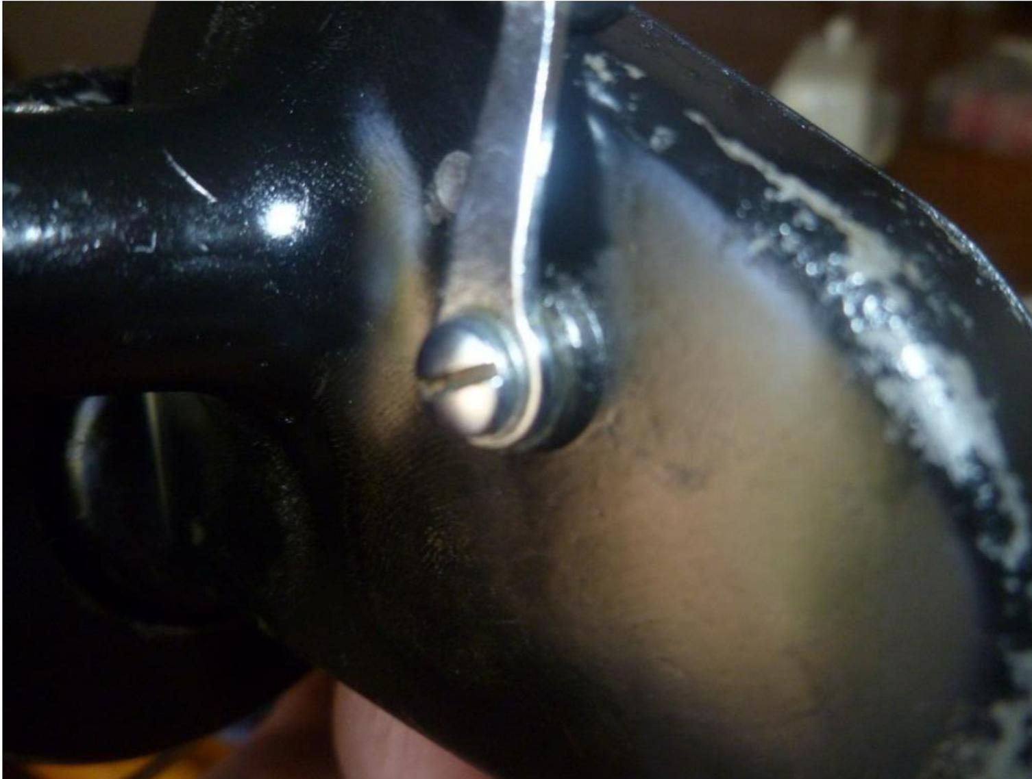
The grease fitting on the handle stem. Firmly depress the "stopper" and give a little squirt. I prefer a light oil.
