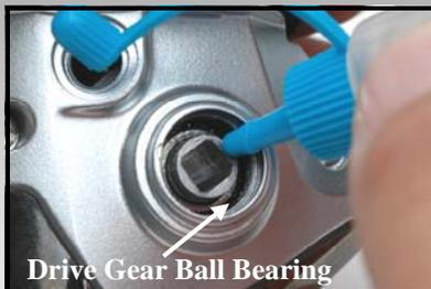
Oil drive gear bearing (s) . Bearings are visible with the handle assembly removed . Some reels also have an additional drive gear bearing on the right hand side.
