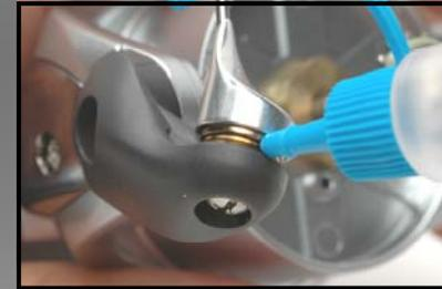
Lightly oil line roller assembly using Shimano® Bantam™ Oil. Regular oiling (after every fishing trip or two) will greatly increase the life expectancy of the line roller bearing.
