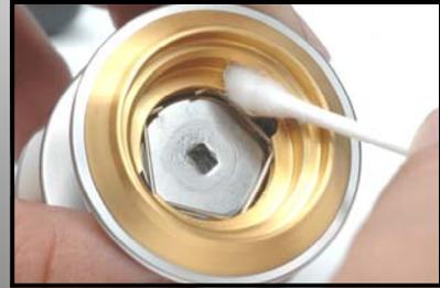
Inspect spool assembly for damage. Pay special attention to the spool lip, as damaged or chipped spool lips will consequently cause premature wear on fishing line.
