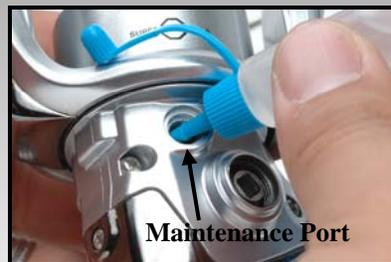
On reels that are equipped with a **Maintenance Port**™ apply one or two drops of Shimano® Bantam™ Oil. Do **not** use **WD-40**® or any degreaser, as it will cause premature wear and tear on the internal parts of your reel.
