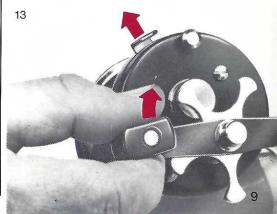
Changing the spool Unscrew the case cover like shown in figure 10. Pull off the spool and insert the new spool (Pict. 14).
