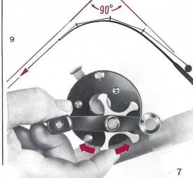
Step 3 con't: Centrifugal brake For novices it is advisable to use the two large centrifugal weights that are inserted in at the factory. Experienced anglers should try the smaller weights. To change the weights, remove the cover cap like shown in figure 10, change the weights, replace the cover cap.
