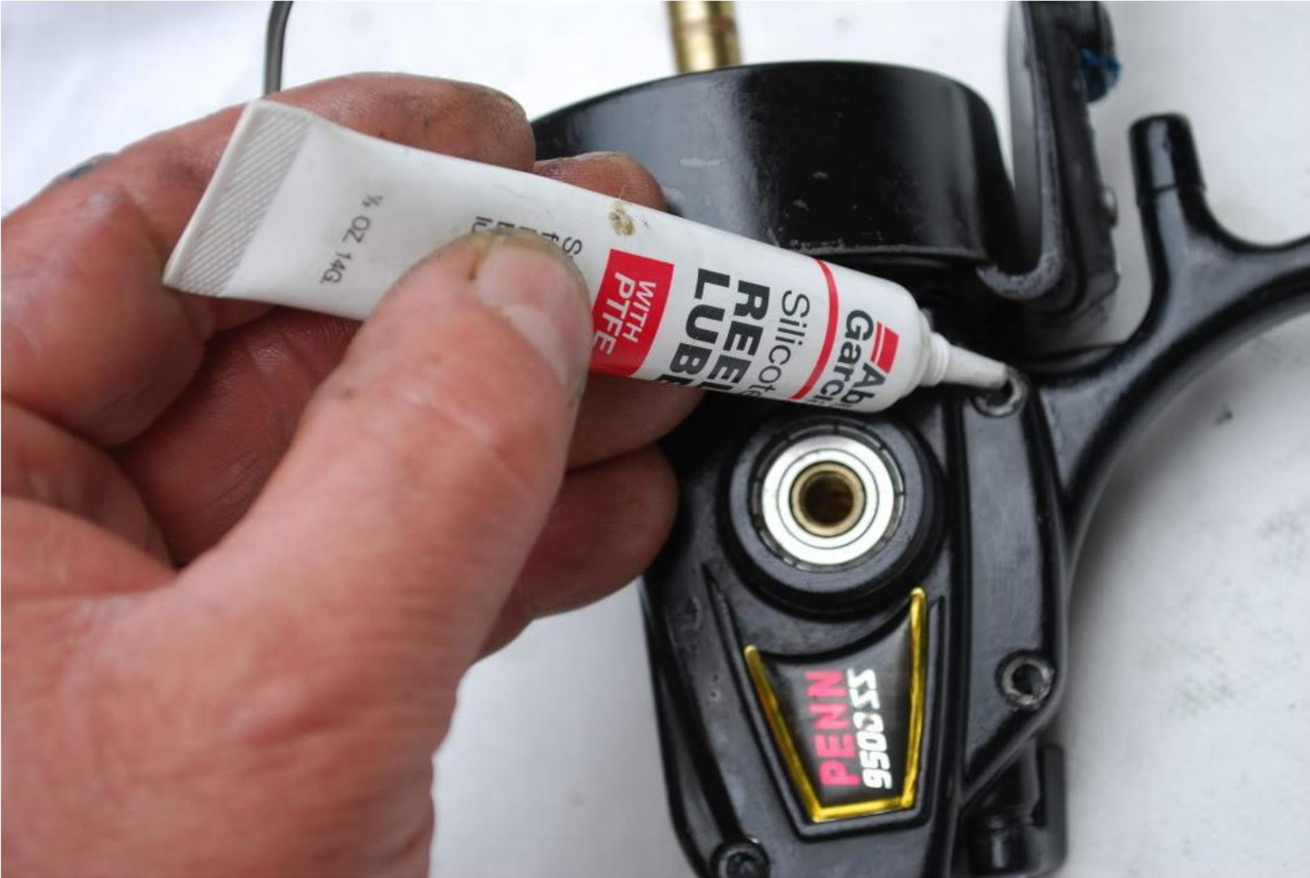
I then put the handle back. I put a drop of oil on the joints and knob (#15).
