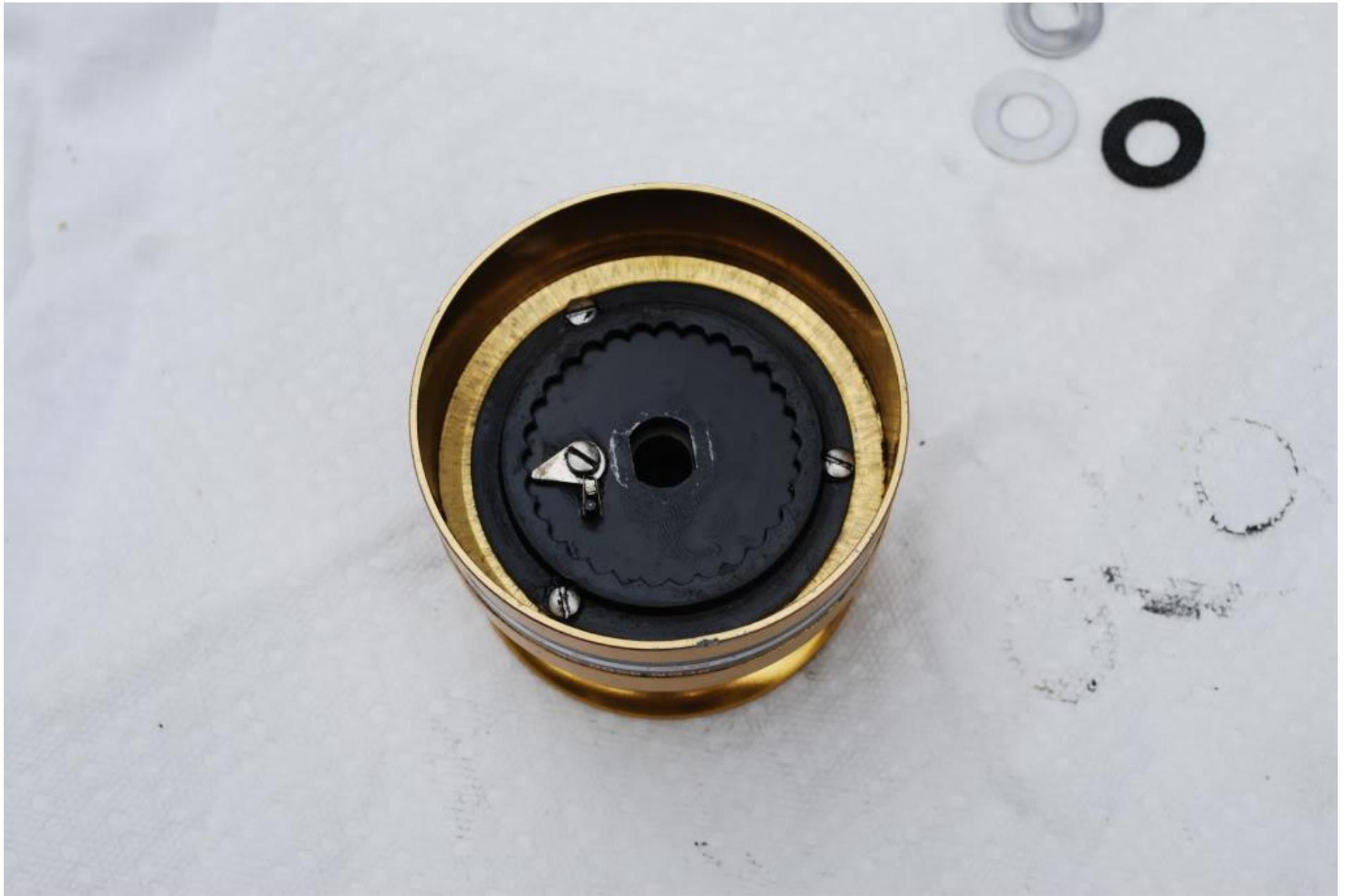
I then removed the plate and pulled the main gear out, key #8. I also removed the spool shaft, #39.
