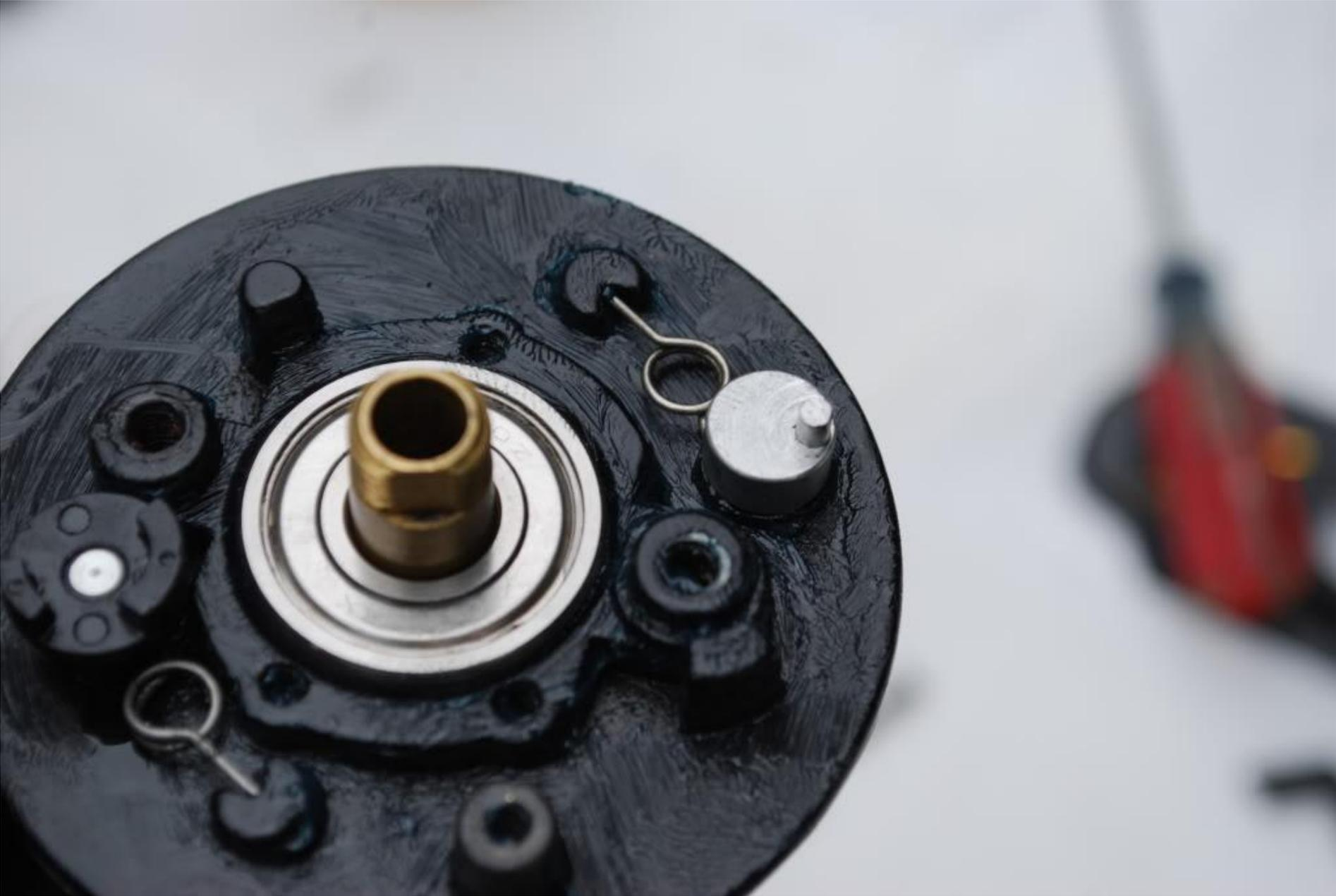
Then I installed the dog, the bearing cover, the pinion spacer, the ratchet, the silent dog, and the transfer lever (key #4, 21, 19a, 10, 4a, 224)
