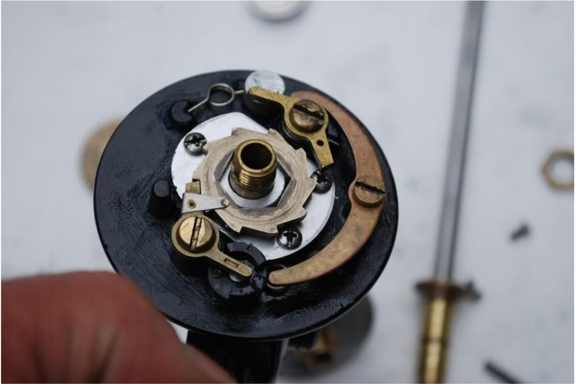
Then I removed the bail wire, key #24. I cleaned the line roller, #35, and the line roller bearing, #35a and reinstalled them.
