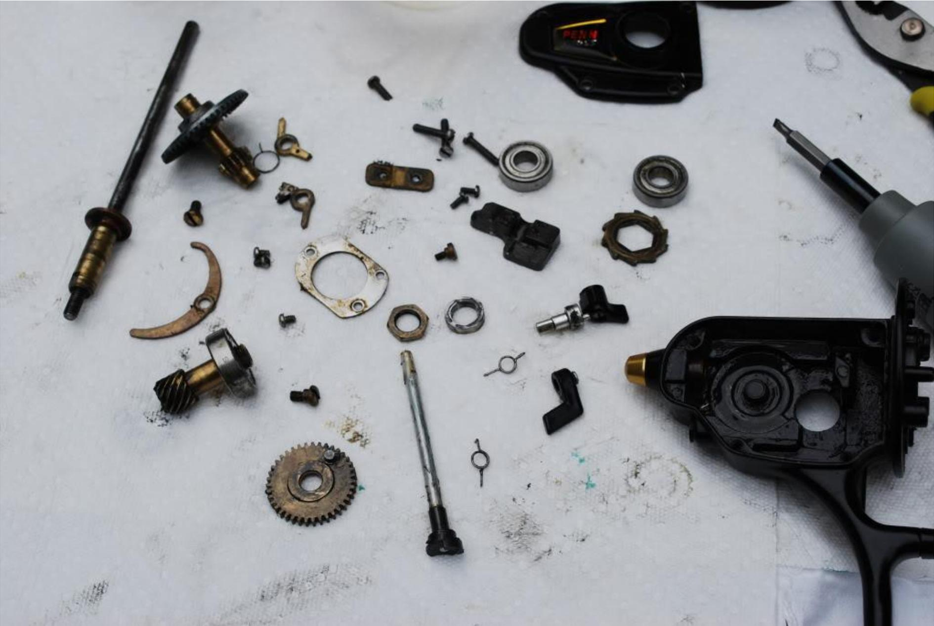
The silent dog needed to be replaced, along with the spool block, key #4a and 43.
