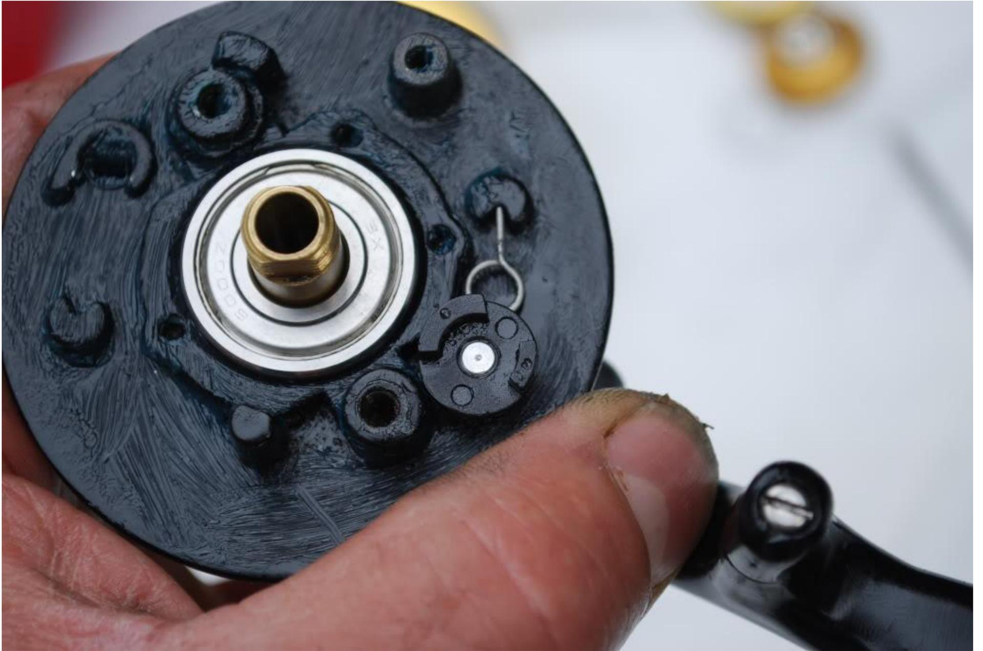
Then, I installed the silent eccentric, key #6L.
