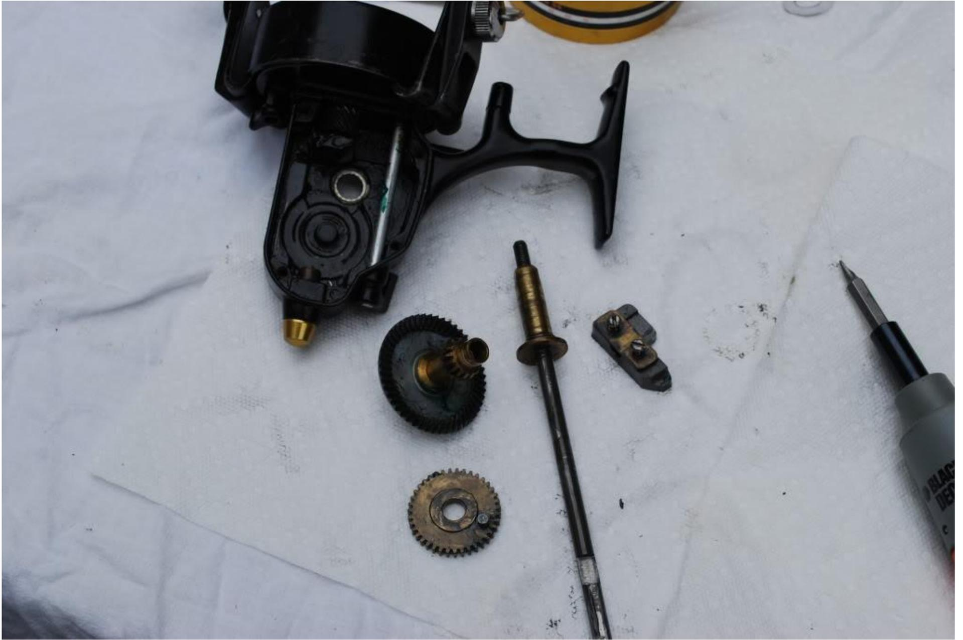
I then removed the transfer lever, the dog, and silent dog, key #4 and 4a. I also removed the bearing cover, the upper eccentric, and the silent eccentric, key #21, 6a, and 6l.
