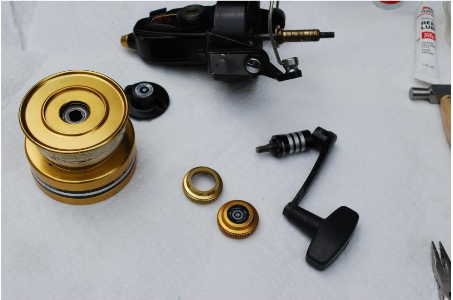
I then checked the drags. The drag washer and drag plate looked good, key #117. I replaced the Teflon washer (key #56t) with a carbon washer.
