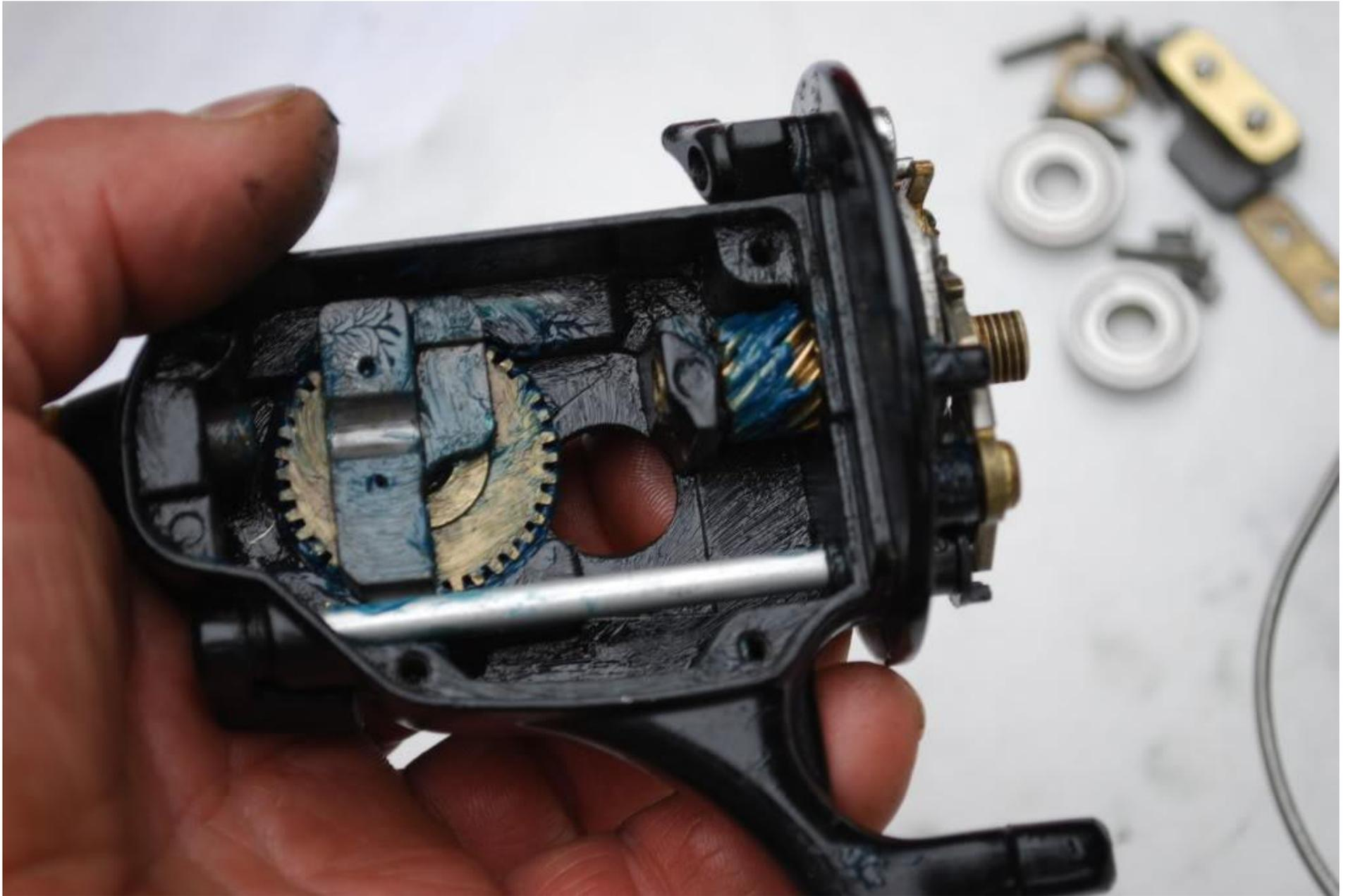
I greased the spool shaft and set it in place, key #39.
