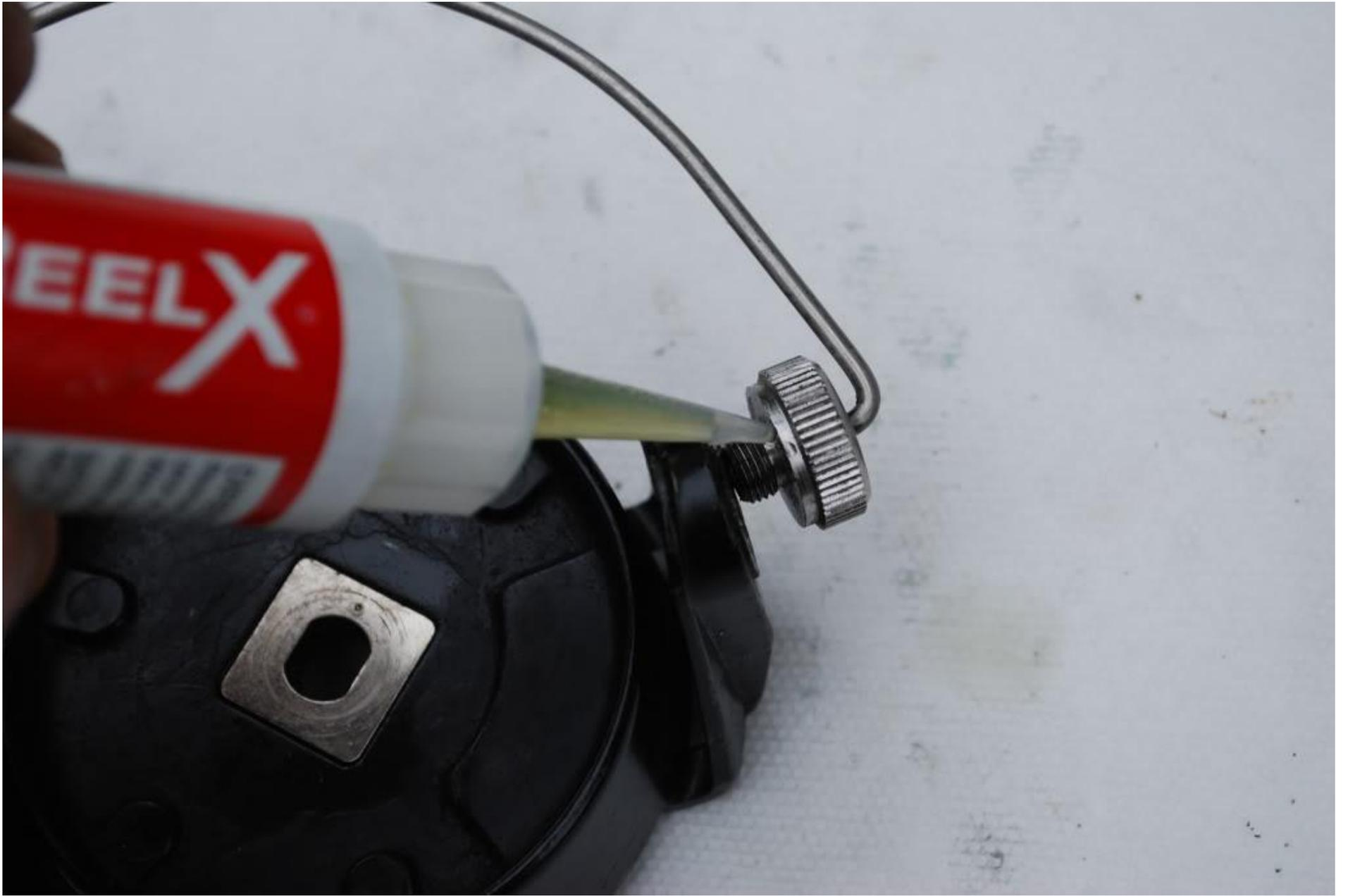
I also removed the bail spring cover, checked the spring, and applied some grease to it.
