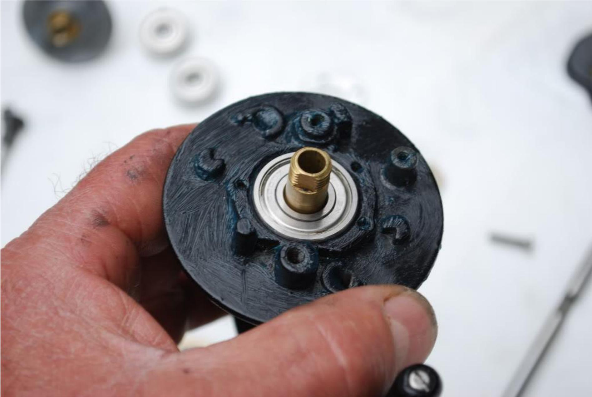
While putting back the upper eccentric, I noticed that it was chipped, so I also replaced this part (key # 6a)
