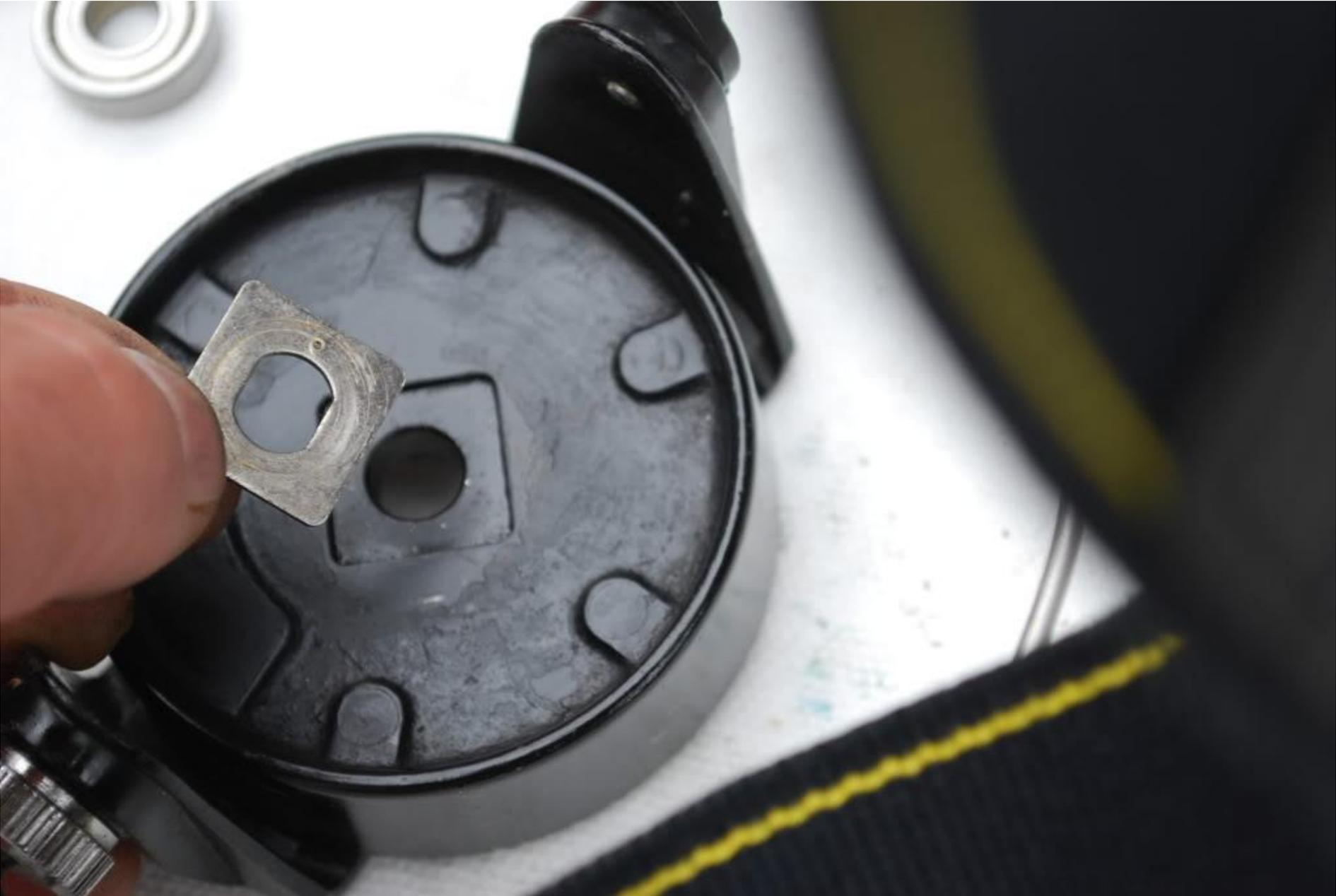
I put the crosswind gear back in place (#231), along with the spool block (#43).
