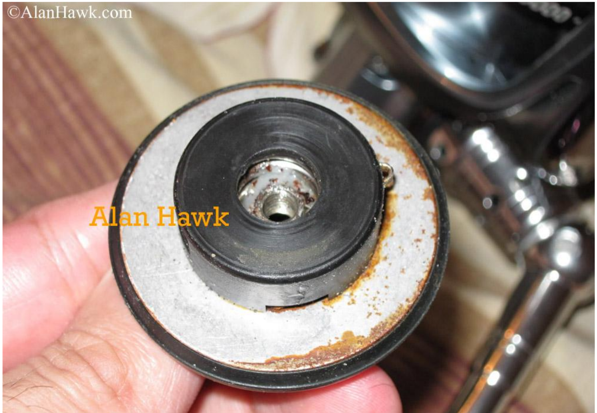
Corrosion in the flange of the drag knob, and inside in the nut and spring.
