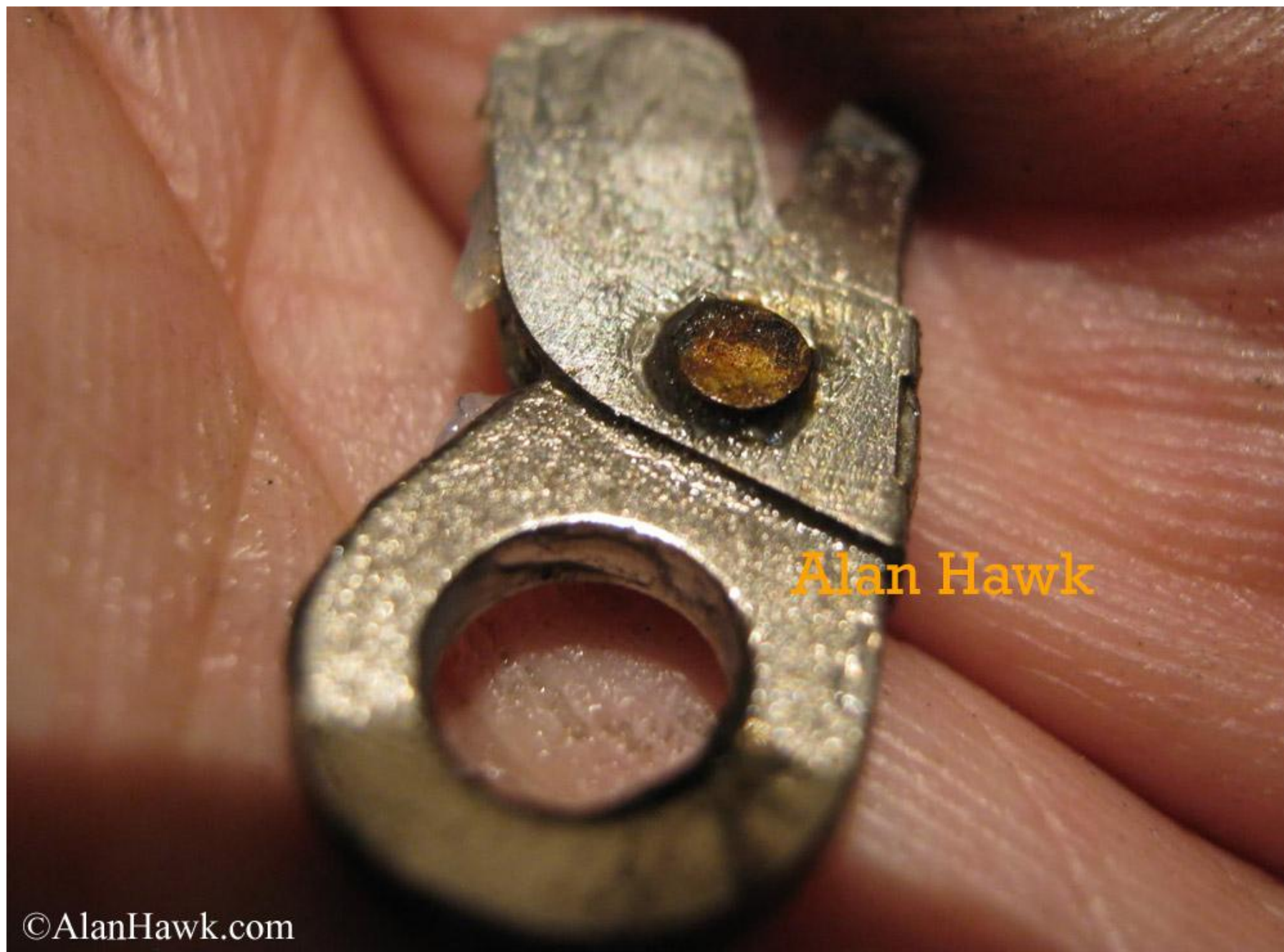
Even deep inside the gearbox, the pin of the backup anti-reverse dog rusted.
