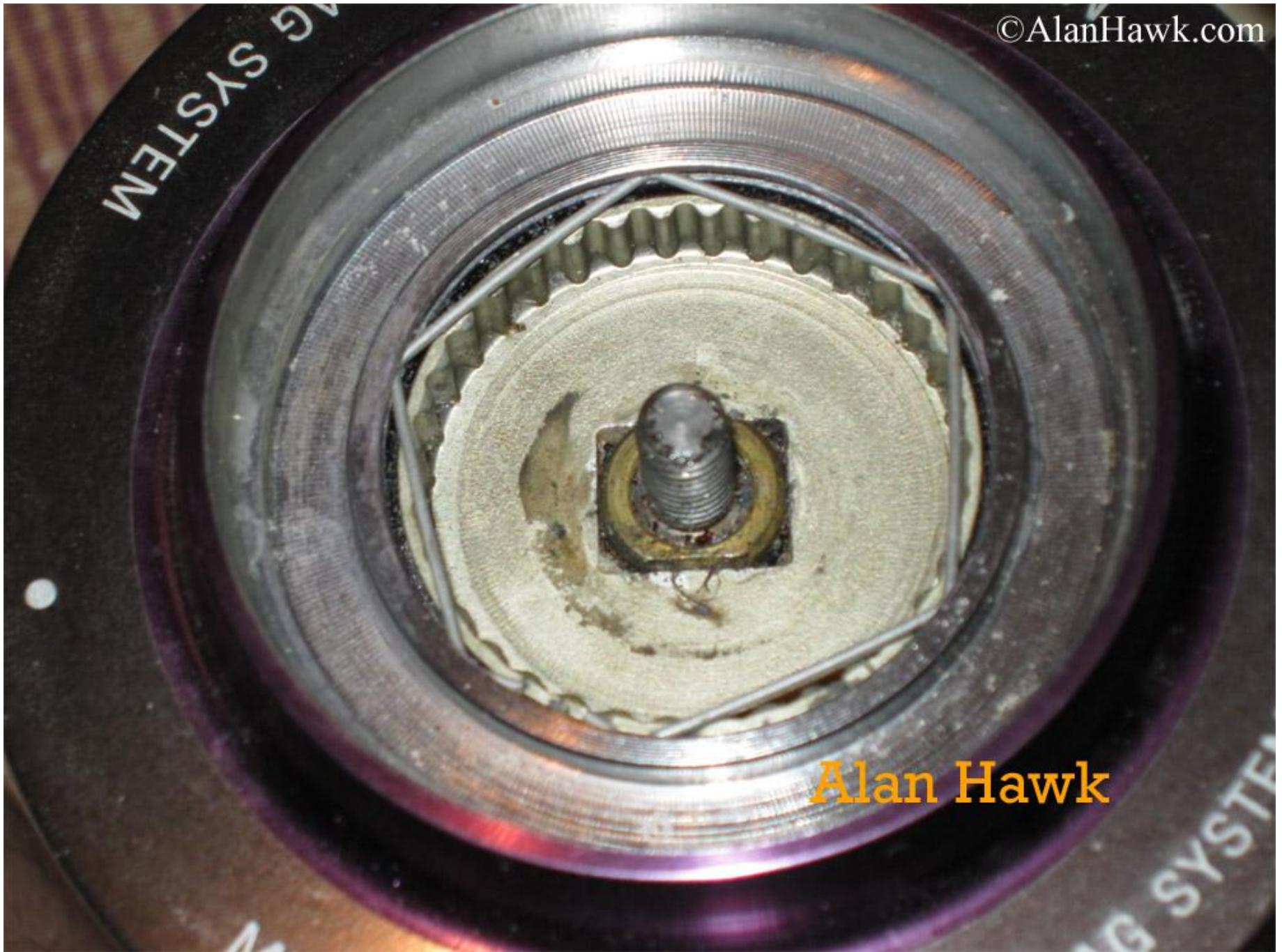
Corrosions in the top drag plate.
