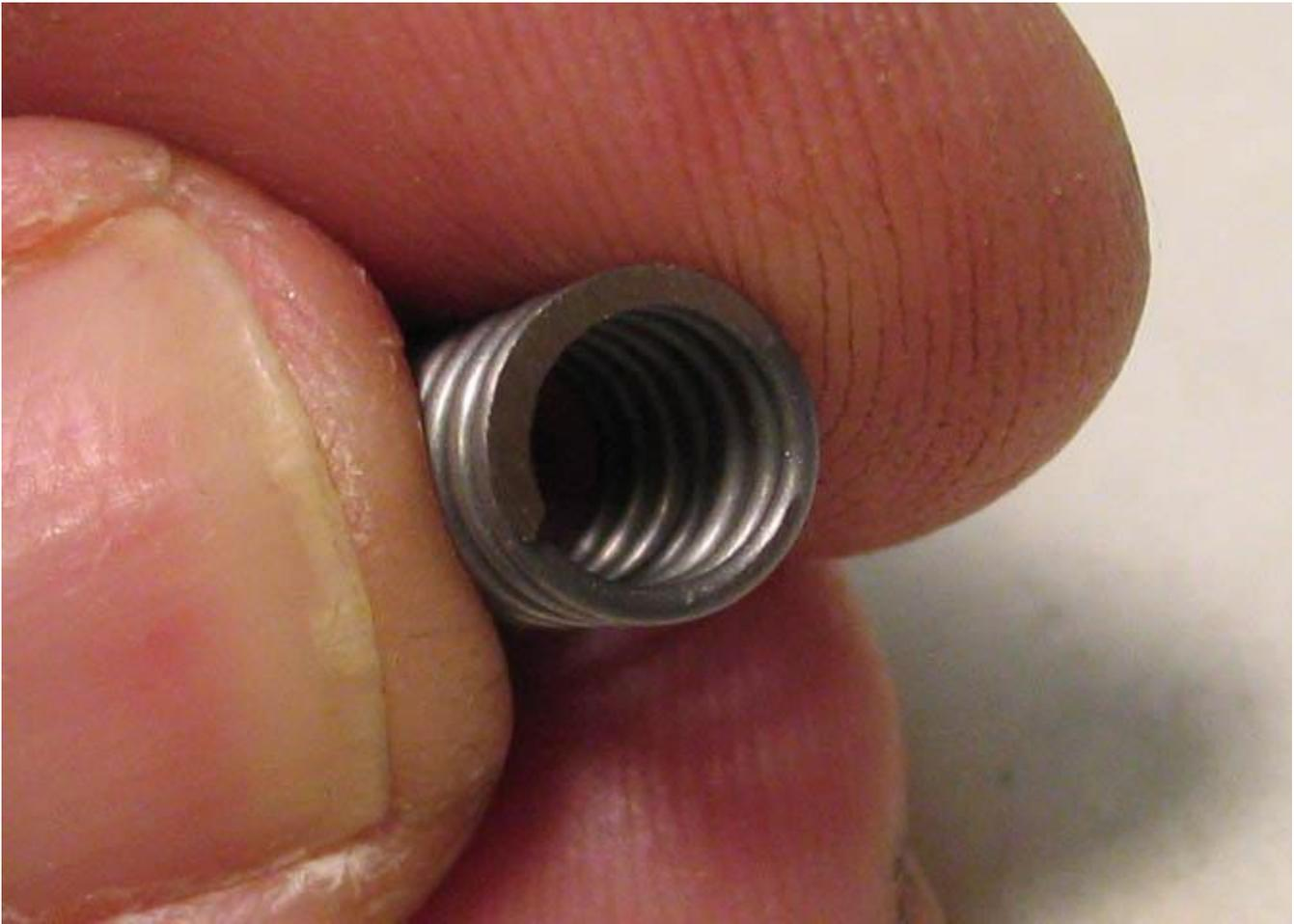
**You can see how it came out, here. The last coil now has a flat end. If I'd left a little more of that coil, like I said to do, the flat would go almost 3/4 of the way around the end of the spring.**
