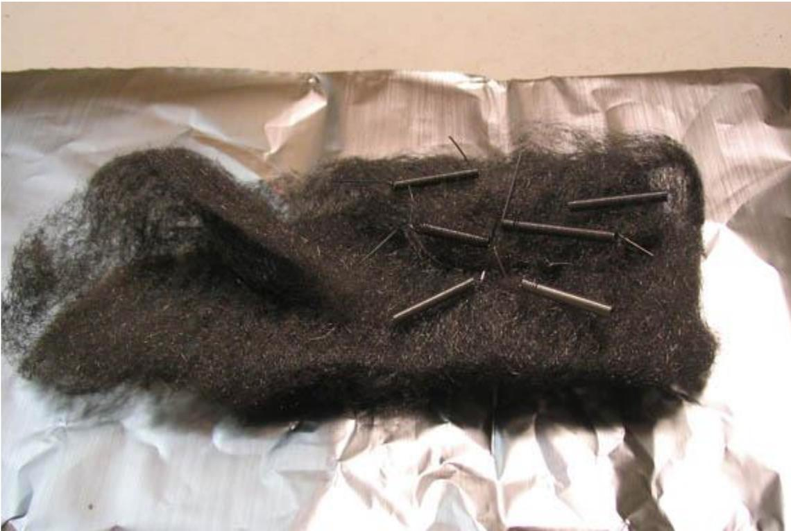
**This next bit, including the following few pictures show the method I use to heat the springs. They have to be stress relieved after the winding process, or they won't hold their shape well. If you don't do this step, the springs won't be as springy as they should be, and can easily be stretched out of shape.**
