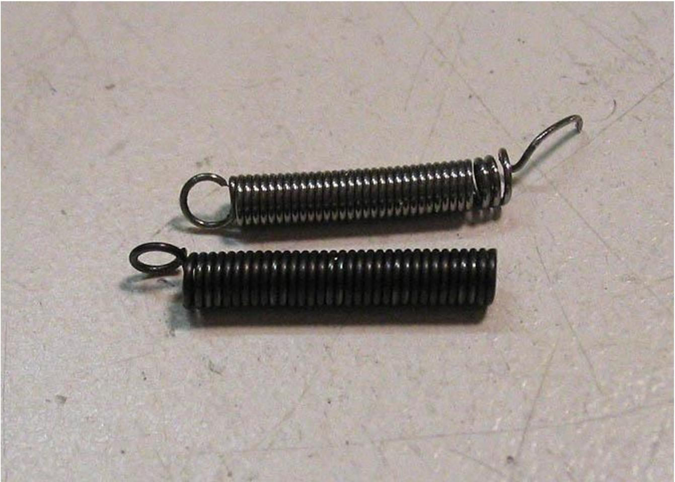
Here's the new spring, and the old one. In this shot, I'm just getting a sense of the position for the second eye needed on the other end. The eye pulling process is repeated.
