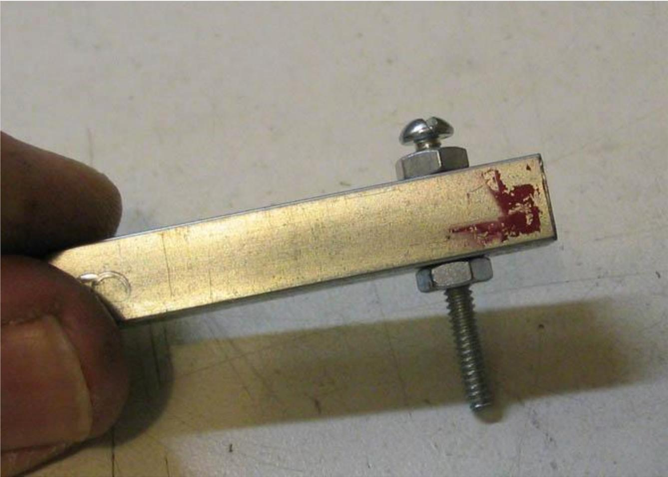
**Here's a closer shot of the working end. This one will make springs using wire up to about 1/16", which would make a fairly stout spring if it was of small dimension.**
