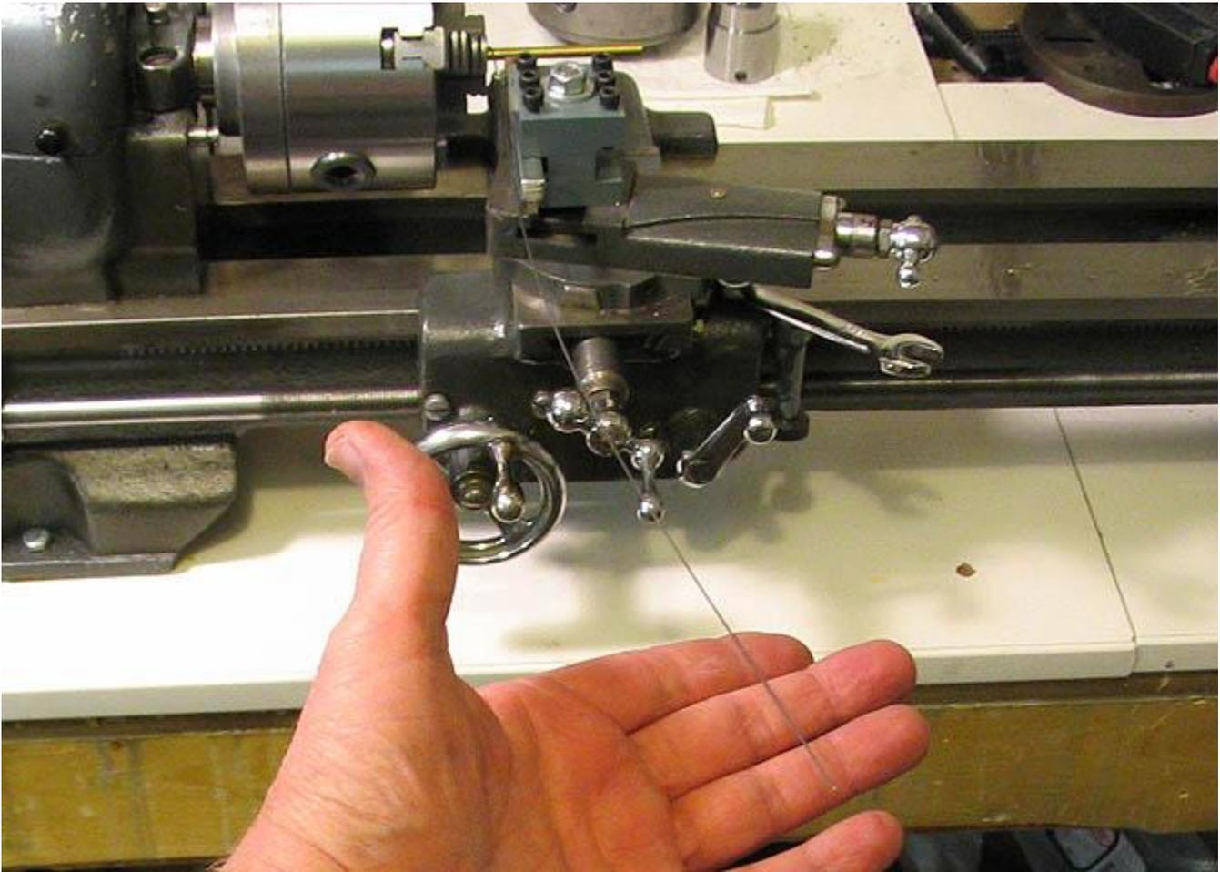
**Here, you can see how the wire hangs off the end of the cross slide. Have a care about it as it sets there. It's small wire, and you can lose it in the background and forget it's there as you are making the spring. Don't put your face in that area.**
