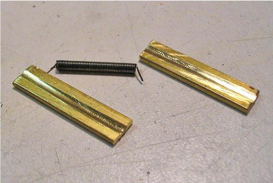
**Here's one of the heat treated springs, ready for the final sizing and pulling out the eyes.**
