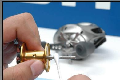
Inspect and clean spool assembly. Clean spool shaft and oil spool bearing or bushing if applicable.
