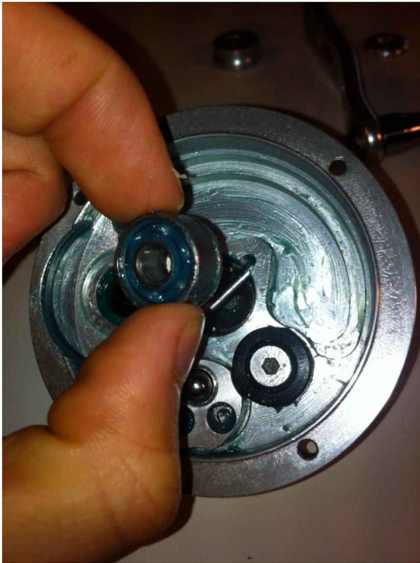
Now the shields cannot be replaced so the bearing has to be left open for now. I actually found a shield and a retainer from another bearing which I used to hold the grease inside the bearing. I faced the shielded side of the bearing towards the inside of the drag cam.
