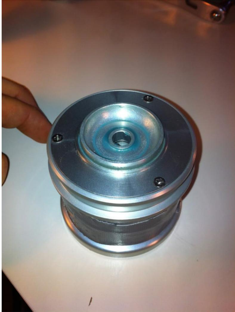
The drags are glued on carbon fibre. The drags are bone dry. I will apply drag grease on on the washers.
