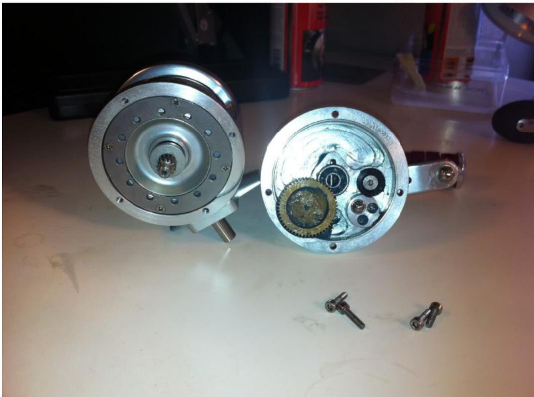
here you can see the alignment of the handle which attaches to the main gear, you have to use the end screw on the handle side and screw it inside the main gear sleeve and then tap it with a semi hard object. I used the plastic handle of a wrench) The main gear will then have to be carefully pulled out of the anti reverse bearing. This way you can access the AR bearing and the right side plate bearing.
