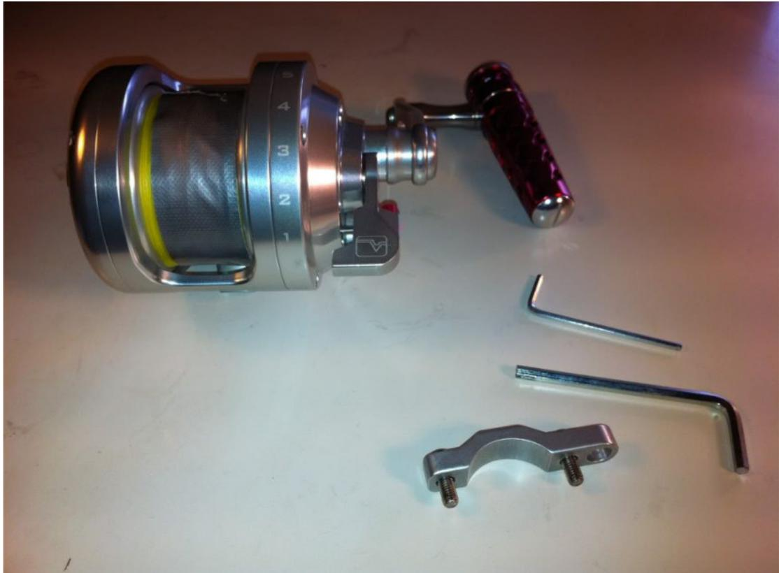
The right side frame goes off in one piece (four umbraco screws) leaving the spool and left side plate and the spool pinion and pinion gear. As you can see there is a big clicker mechanism which they have used a stainless steel chrome ball that will slide over the engraved clicker bracket attached to the spool. (this clicker is much more stabile and works much better than the plastic clicker that is often used in small reels, the same clicker is used in many international reels)
