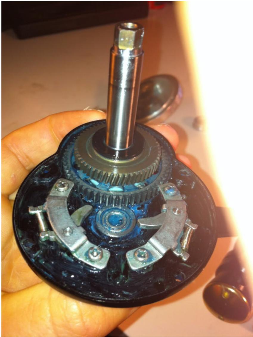
As the main gear is pulled out you can access the right side plate bearing. (The bearing has a metal spacer inside the cam to fit the housing of the reel) The bearing was pretty good greased up but I will remove it with carb. cleaner and pack it completely with yamaha marine grease. (you have to remove the pressed in metal shield. (see alantani's sticky bearing thread for instructions removing pressed in shields) the Bearing measures: ID:8mm, OD: 16mm and Height: 5mm
