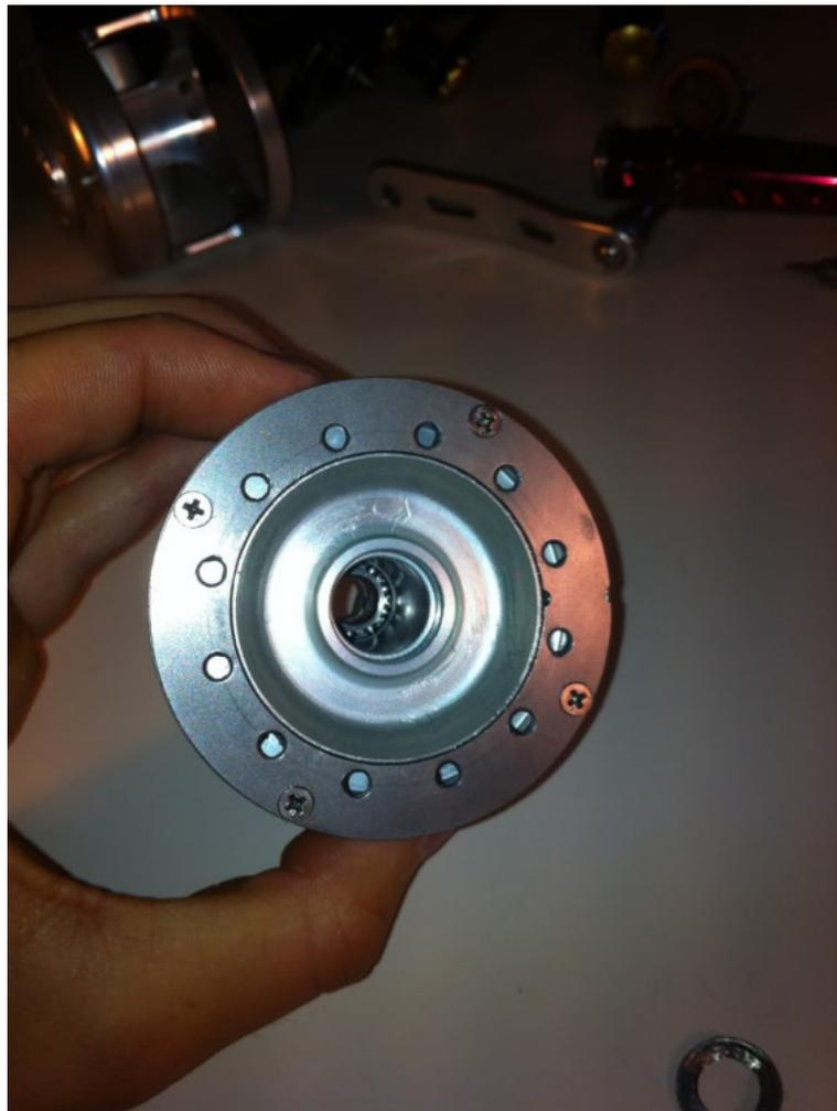
On to the left side of the spool is a machined housing which holds the whole drag assembly and works as a shield. This is not watertight though... The drags are enclosed by three screws.
