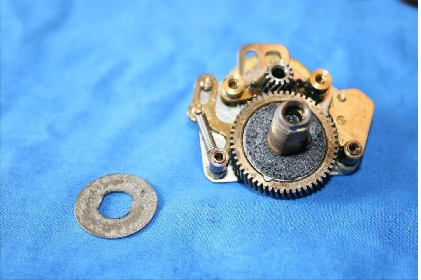
Again, installation is a reversal of the removal procedure with note to the following points: Make sure that these two pins align in their respective slots...
