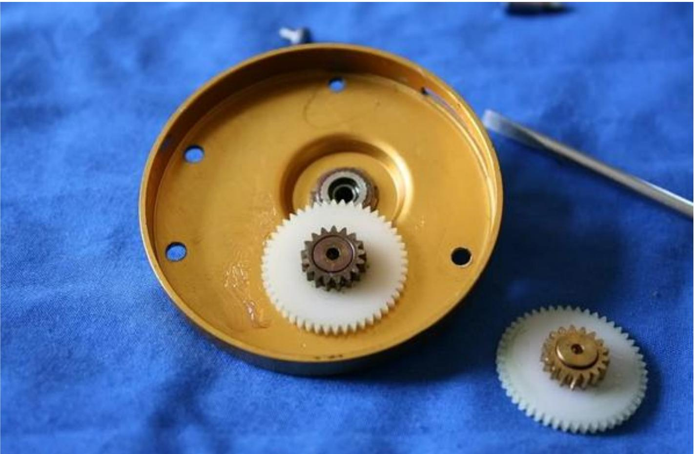
I was replacing the level wind worm, idler gear, the idler shaft and the bearing as I was having a couple of small issues with the level wind from time to time. Refer the pictures for the parts involved and the worm can be removed by (carefully!) removing the small circlip on the end of the shaft.
