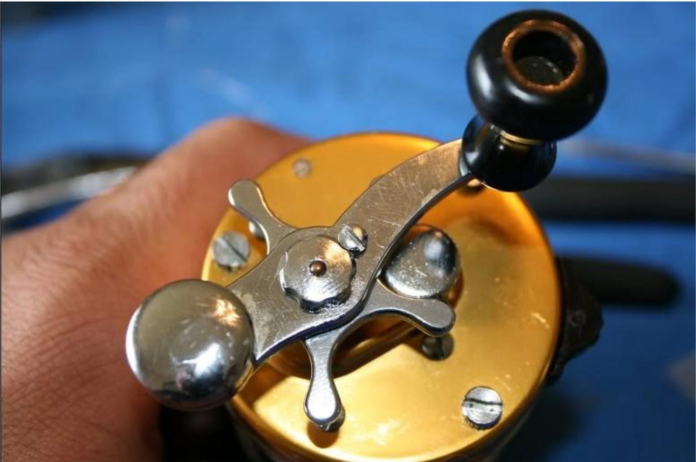
**Nip it up just firm and insert and tighten the grub screw.**
