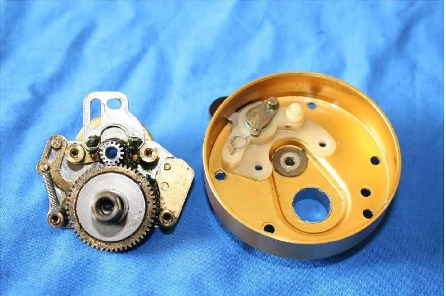
This shows the HT-100 washer that sits under the main gear. You'll note I have plans to replace the sleeve next time I strip the reel down as you can see the salt water is starting to get to it. A quick and gentle clean up with steel wool was the go here this time....
