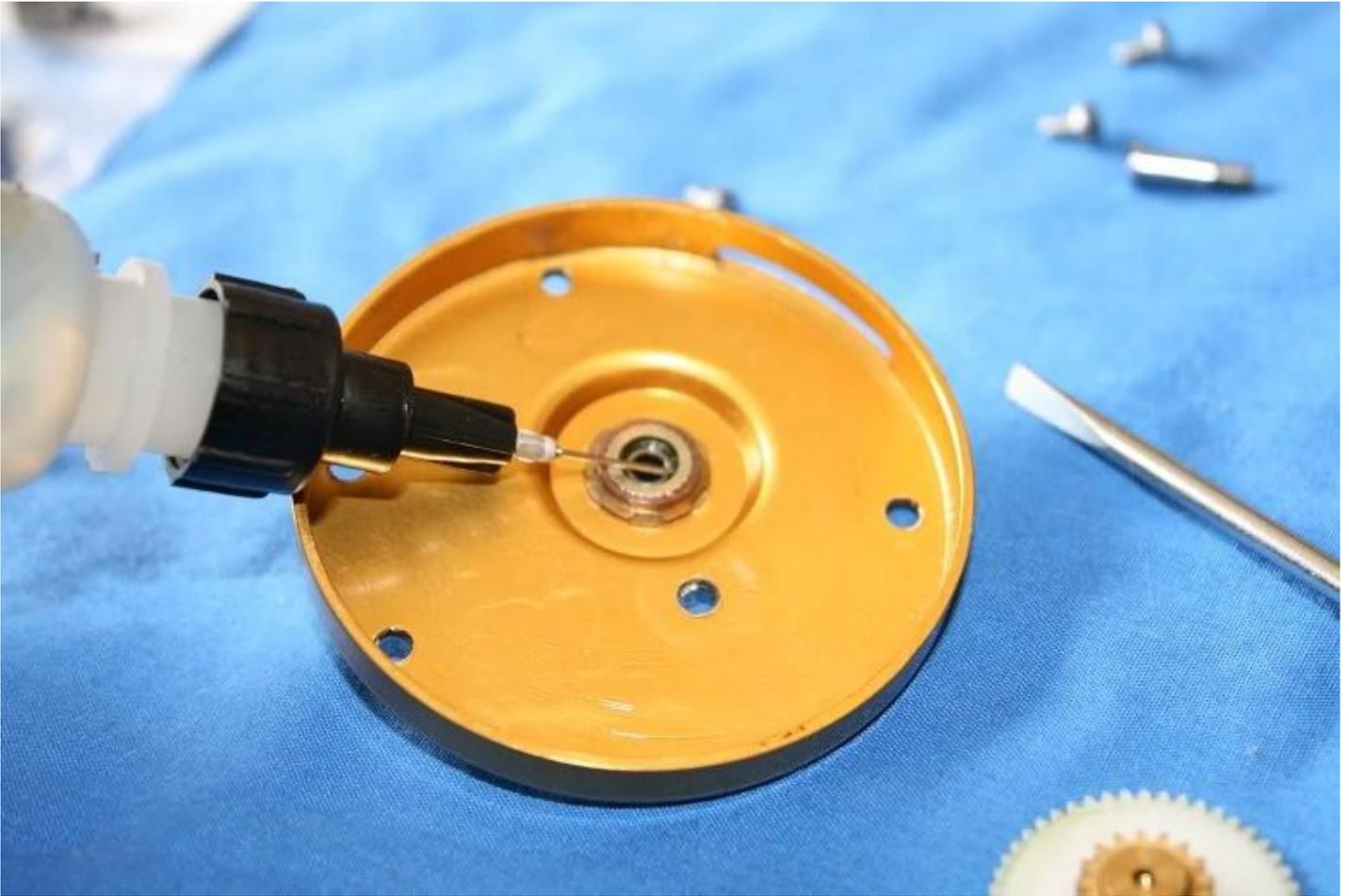
Remove the nut holding the slotted line guide onto the right side inner ring. This one was just starting to corrode again slightly from a drop of salt water under where the nut seats despite being fastidious when cleaning my reels after use (this one had not been apart for probably 6-7 fishing trips in the salt but had been cleaned in warm soapy water after every trip).
