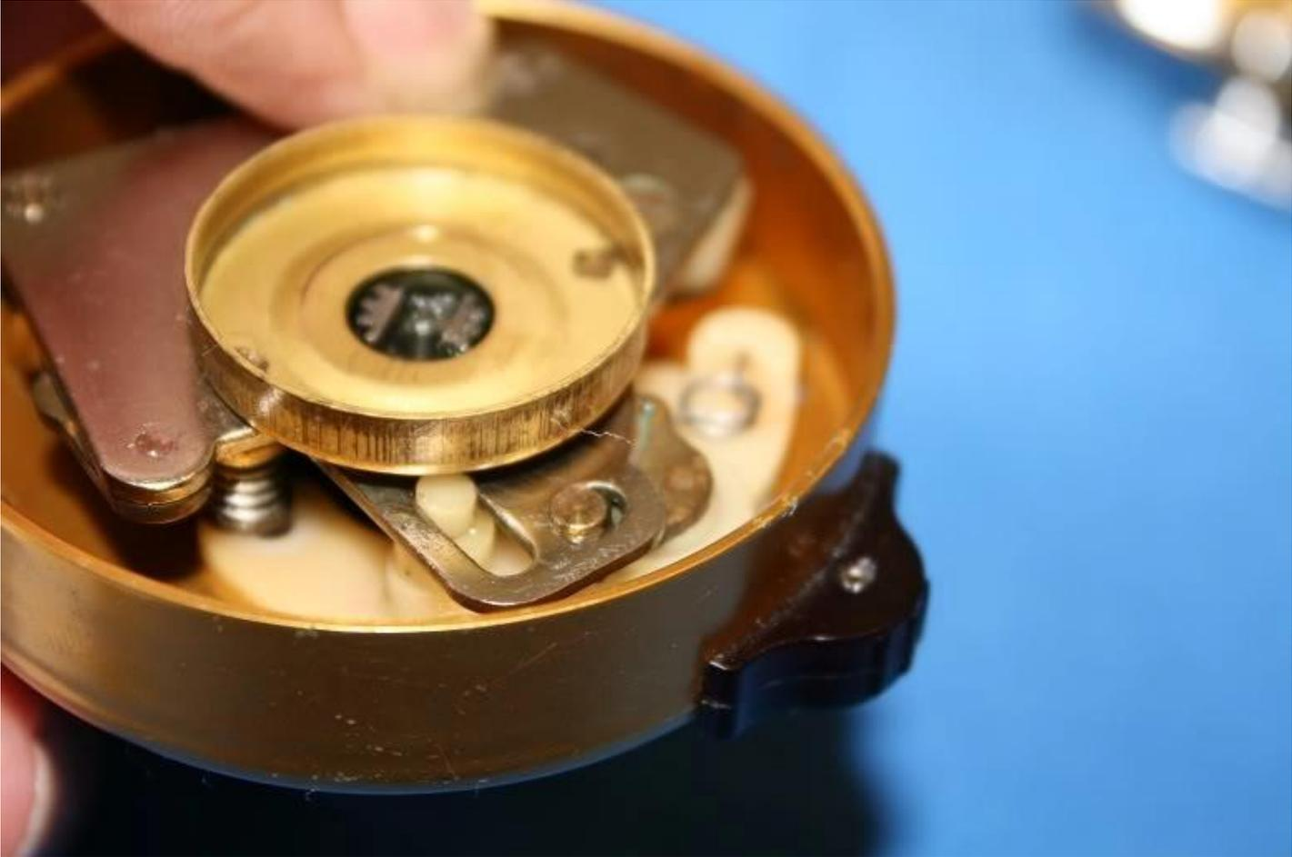
Ensure that BEFORE you put the bridge screws back in that the plastic (neoprene?) hole guides align in the side plate correctly prior to inserting the screws and that the chromed sleeve is inserted prior to fitting the wave washer and star wheel.
