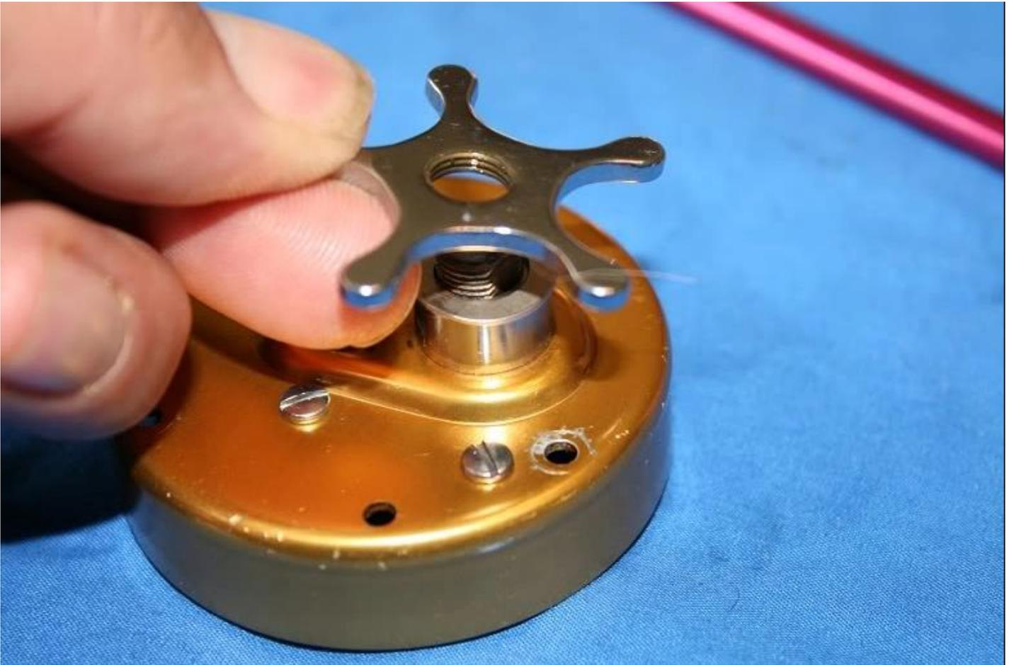
A small drop of Metoil on the bearing and the drive unit is ready to be refitted to the rest of the reel taking note of the correct alignment of the dowel to the side plate and that you have nipped the retaining nuts up snugly and in the right position. Also ensure that the spool brakes ( if you need them ) are in-situ.
