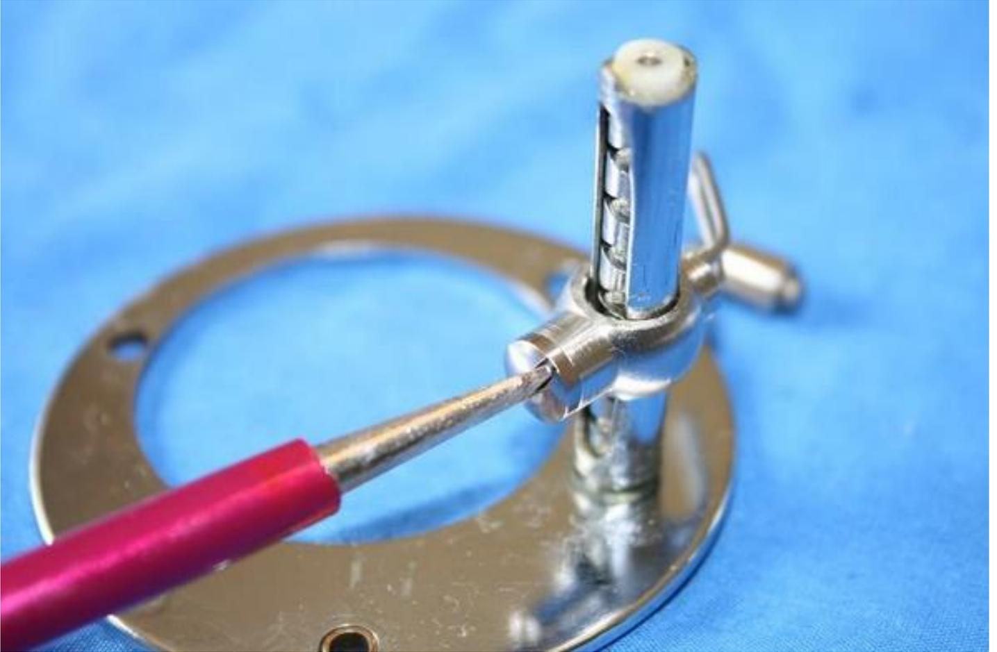
The disassembled line guide.
