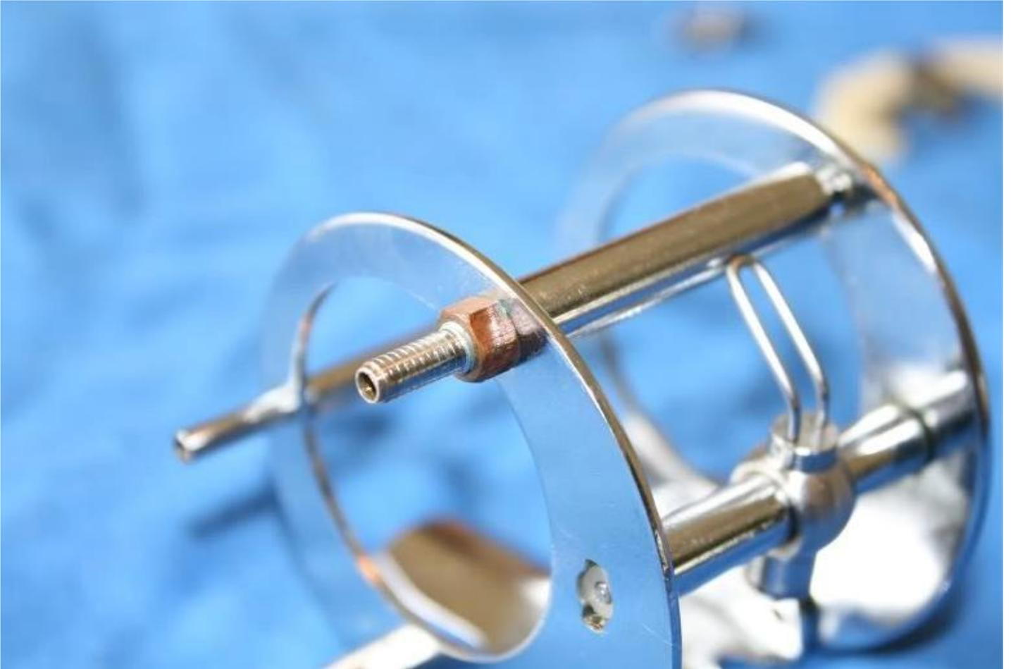
You can now disassemble the line guide being careful not to force any of the parts. You can see here that I should have used a slightly larger screwdriver!
