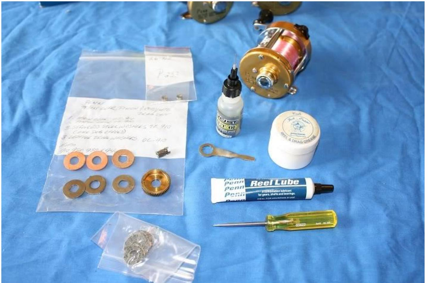
Remove the handle lock retainer and handle screws from the reel. The handle will just lift off, leaving the star drag wheel to spin-off anticlockwise.
