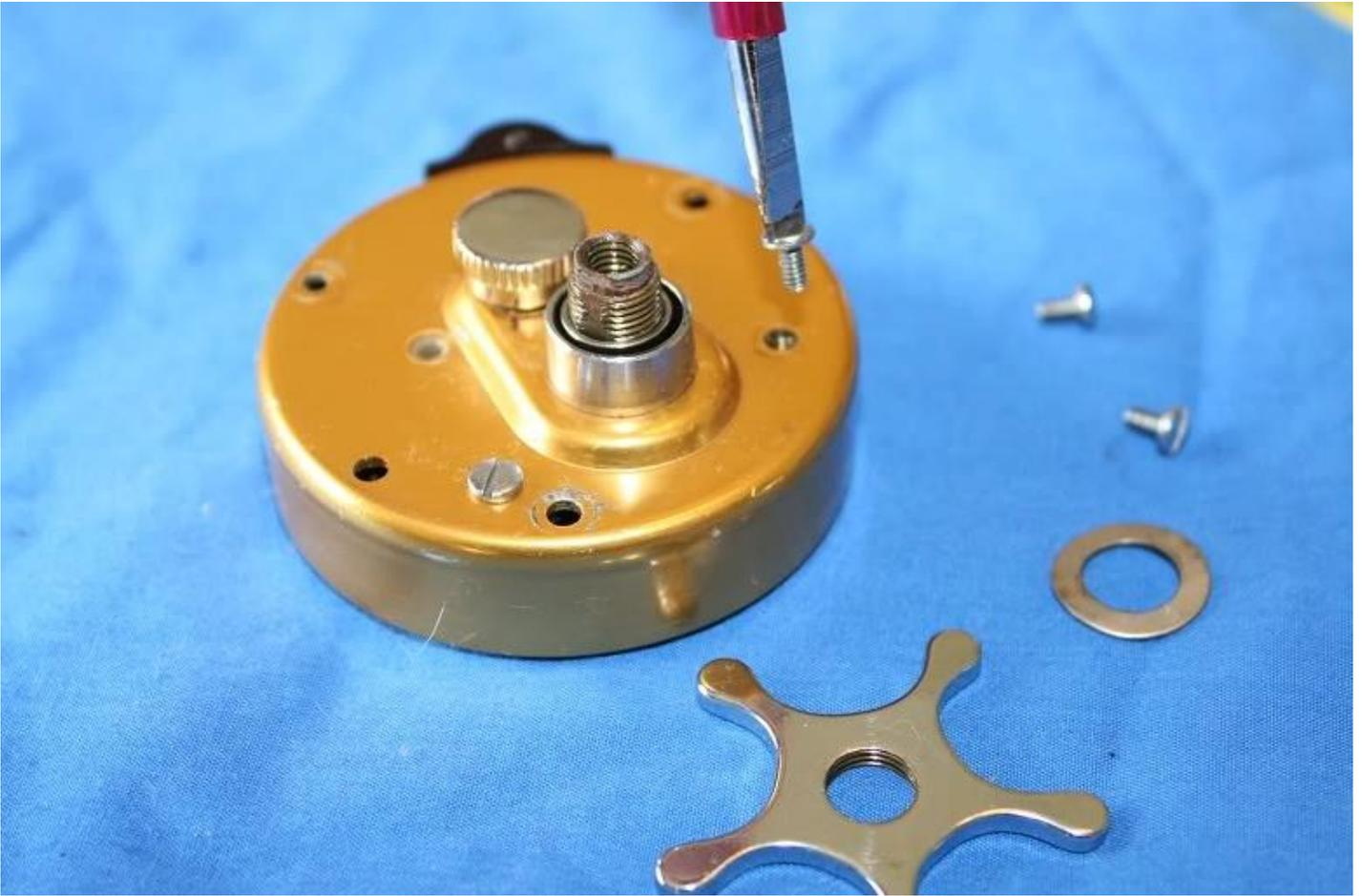
The bridge assembly will come out as a unit reel exposing the drag washers and gears. I had no reason to strip the reel any further down than this to do what I needed to (replace the drag washers), but a general clean-up in solvent (of your choice, I tend to use carby cleaner being careful not to use so much as to melt any plastic parts) and re-grease is always in order.
