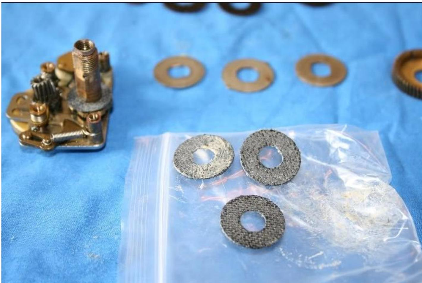
The new HT-100 drag washers that replaced the leather originals. The residue on the stainless washer is actually Cal's as I had fitted the washers then realised I hadn't taken a photo!
