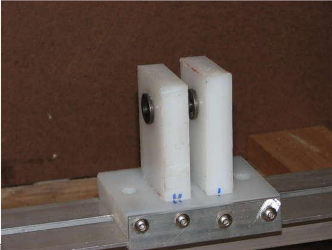
It is a good idea to use the finished headstock to help finish the tailstock. I removed the chuck, so the end of the shaft was now exposed again. On the tailstock, I mounted two pieces of UHMW vertically. Two pieces because they should keep whatever tailstock accessory aligned better than just one piece.
