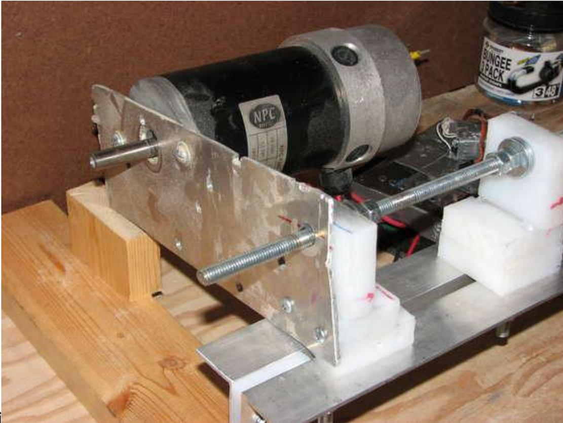
I will not go into excessive detail here because everyone's motor setup will vary. The main thing is to make sure your motor can spin with both a lot of speed and a lot of power. For a wood lathe, a 1/2 horsepower motor should be enough. Mine is a 10 pound, 1.25 horsepower motor and it has never slowed down while I am turning something. I decided to use this motor because I had the motor and a fully variable speed controller just sitting around.
