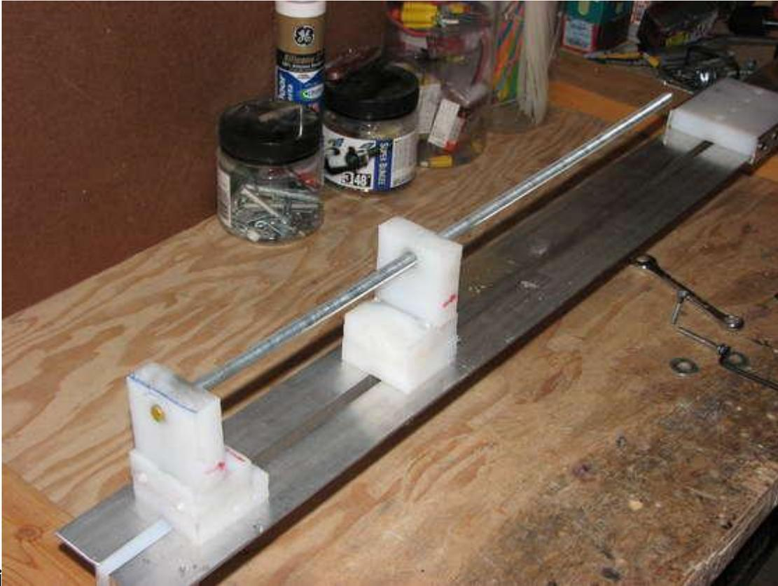
Next I aligned the two supports I created. I pushed a long threaded rod through both of the supports, and fiddled until the rod lined up perfectly with the bed. I had to remake the supports several times until I got the shaft to line up nicely, but it is worth a little extra work to have a well aligned shaft. When you are happy with the alignment, tighten down the supports extremely tightly because they wont be moving.
