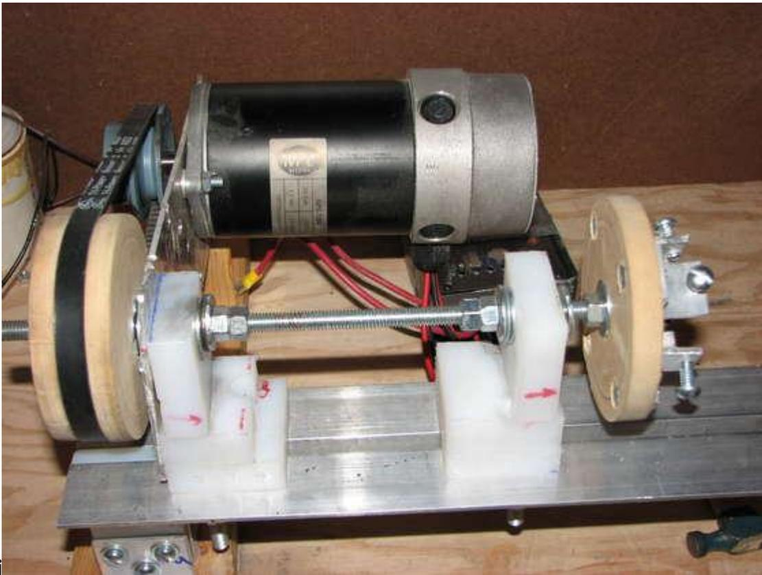
At this point, you should be able to turn on the motor and have the chuck spin reliably. Start at a low speed and ensure the chuck is balanced and that everything is secure. Now is a better time to find any problems with things before you start spinning chunks of wood.
