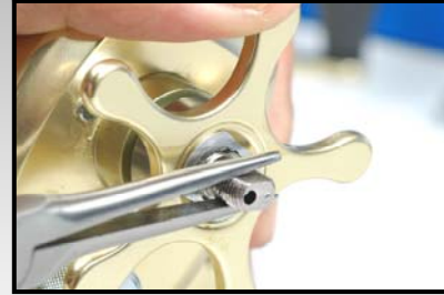
With the click pin held in place by the star drag washer, spin the star drag onto drive shaft. Use pliers to hold the shaft from spinning.
