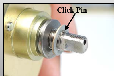
After removing star drag, exercise caution, as the drag clicker pin may pop-out.
