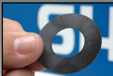
Lightly apply Shimano® Drag Grease on drag washers. Excessive grease will adversely affect maximum drag pressure.
