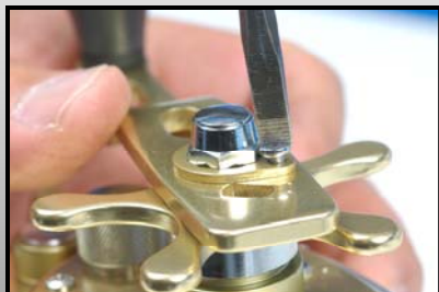
Use a small Phillips or flathead screwdriver to remove handle as-
