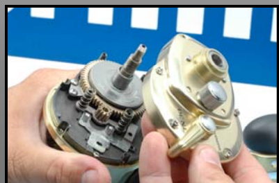
Remove right side plate. Be careful not to lose yoke springs as they may fall out.
