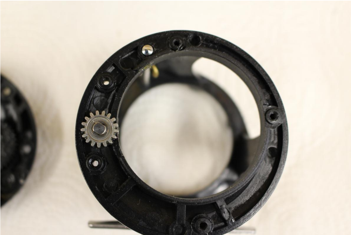
The reel frame viewed from the left side, showing the Levelwind mechanism.
