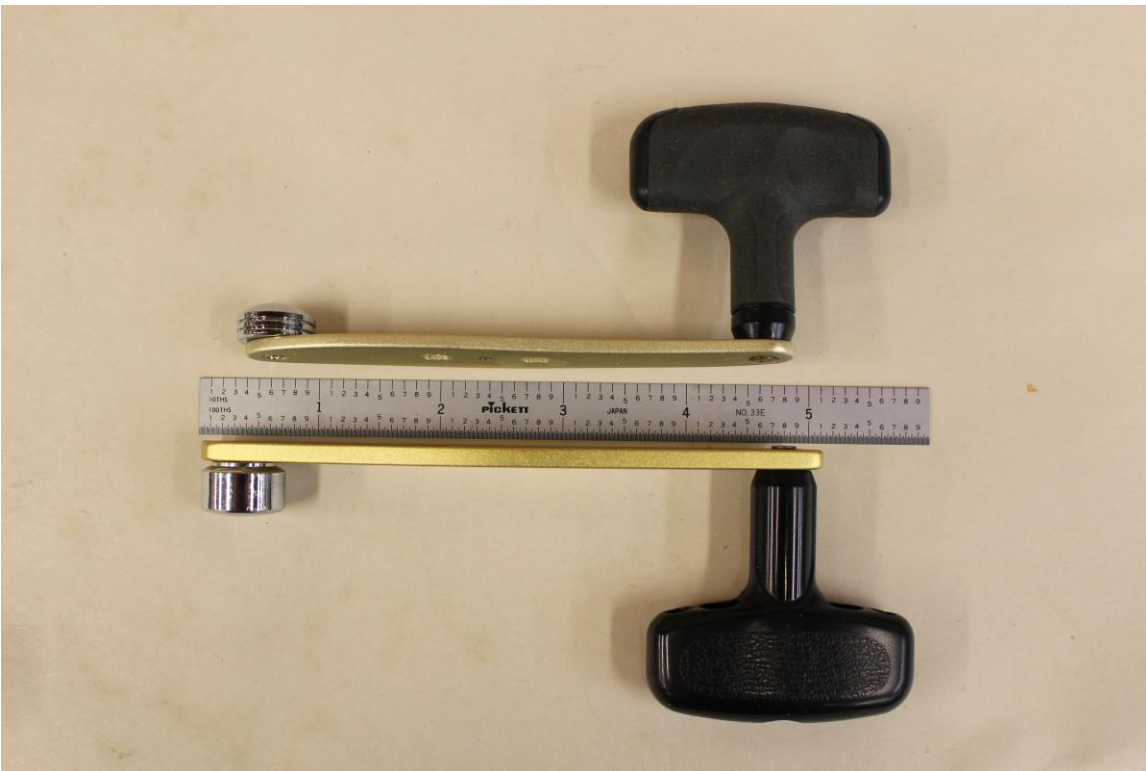
Side views of the original Cabela's handle (top) and the Power Handle (bottom) with the mounting holes aligned with the 2 inch mark on the ruler.
