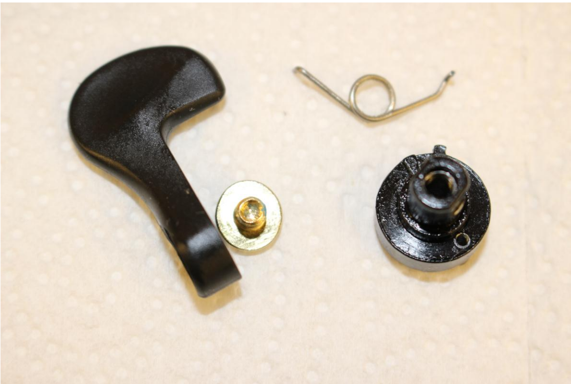
Photo showing the Clutch Cam assembly parts.
