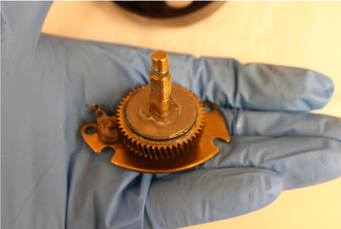
The Hold Plate assembly after removal from the side plate.
