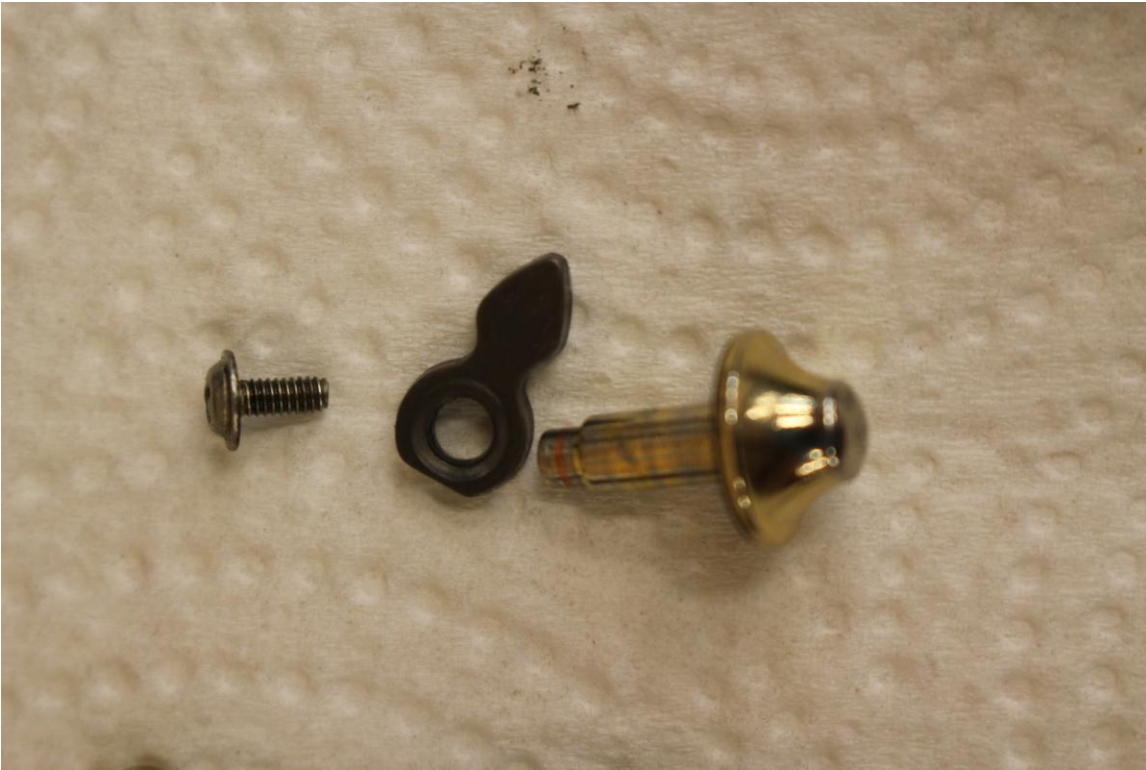
The Click Pawl, Click Button, and Click Pawl Screw shown after removal. (DM30)
