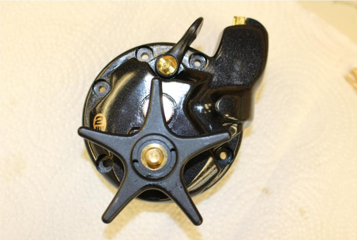
Assembly of the Right Side is complete. The handle will be installed after the side plates are assembled onto the reel body.
