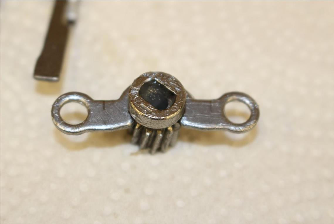
Grease the Pinion Gear and Pinion Gear Yoke then slide the Yoke onto the Gear as shown.
