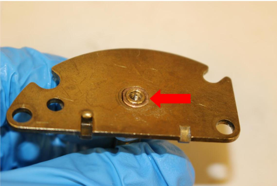
Grease the bottom surface of the Hold Plate and install it on the Drive Shaft Bushing.
