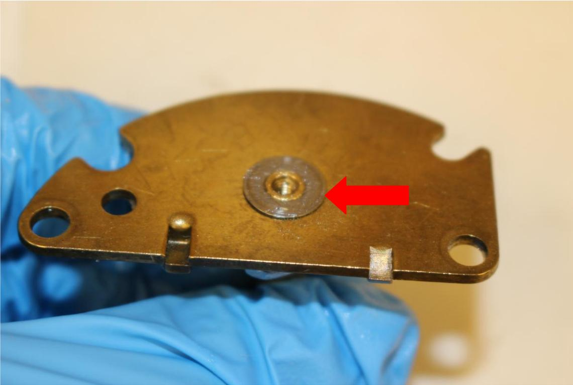
Grease and install the Washer and Drive Shaft Screw onto the Drive Shaft Assembly.
