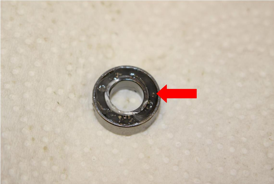
Pack the Ball Bearing with grease. I used Silicote grease because it comes in a tube with an applicator tip which is a convenient size for applying the grease. Super Lube would work just as well for greasing Ball Bearings. Try not to get lots of grease on the outer race of the Ball Bearing; we don't want the race to spin in the side plate.
