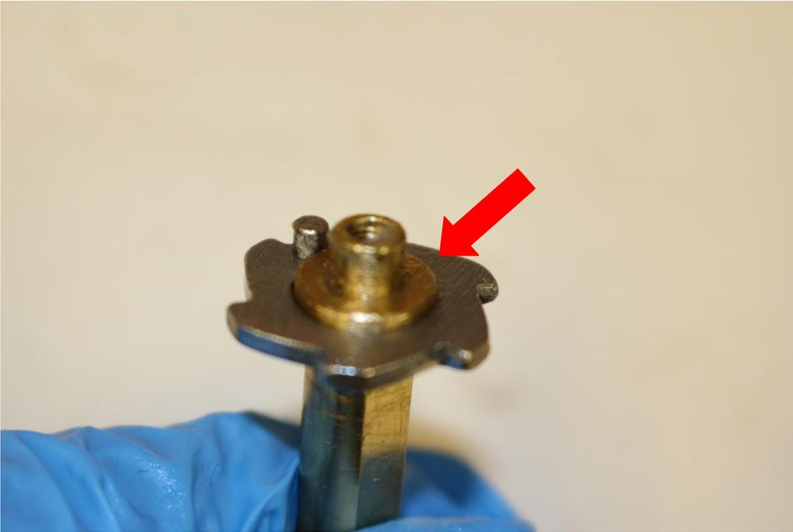
Grease the bottom of the Drive Shaft Assembly.
