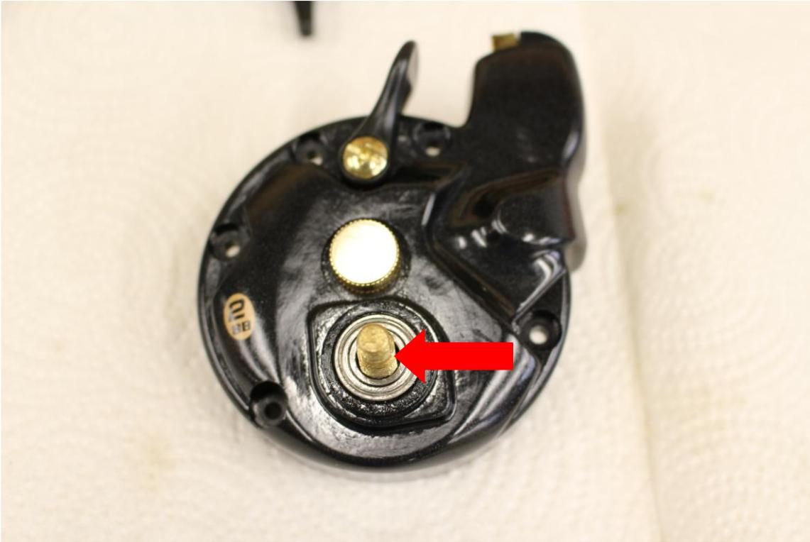
Install the Star Drag knob on the Drive Shaft, tightening it only until you feel resistance. The Star Drag does not need to be tight.
