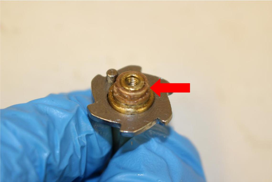
Grease the Drive Shaft Bushing and install it on the bottom of the Drive Shaft Assembly.
