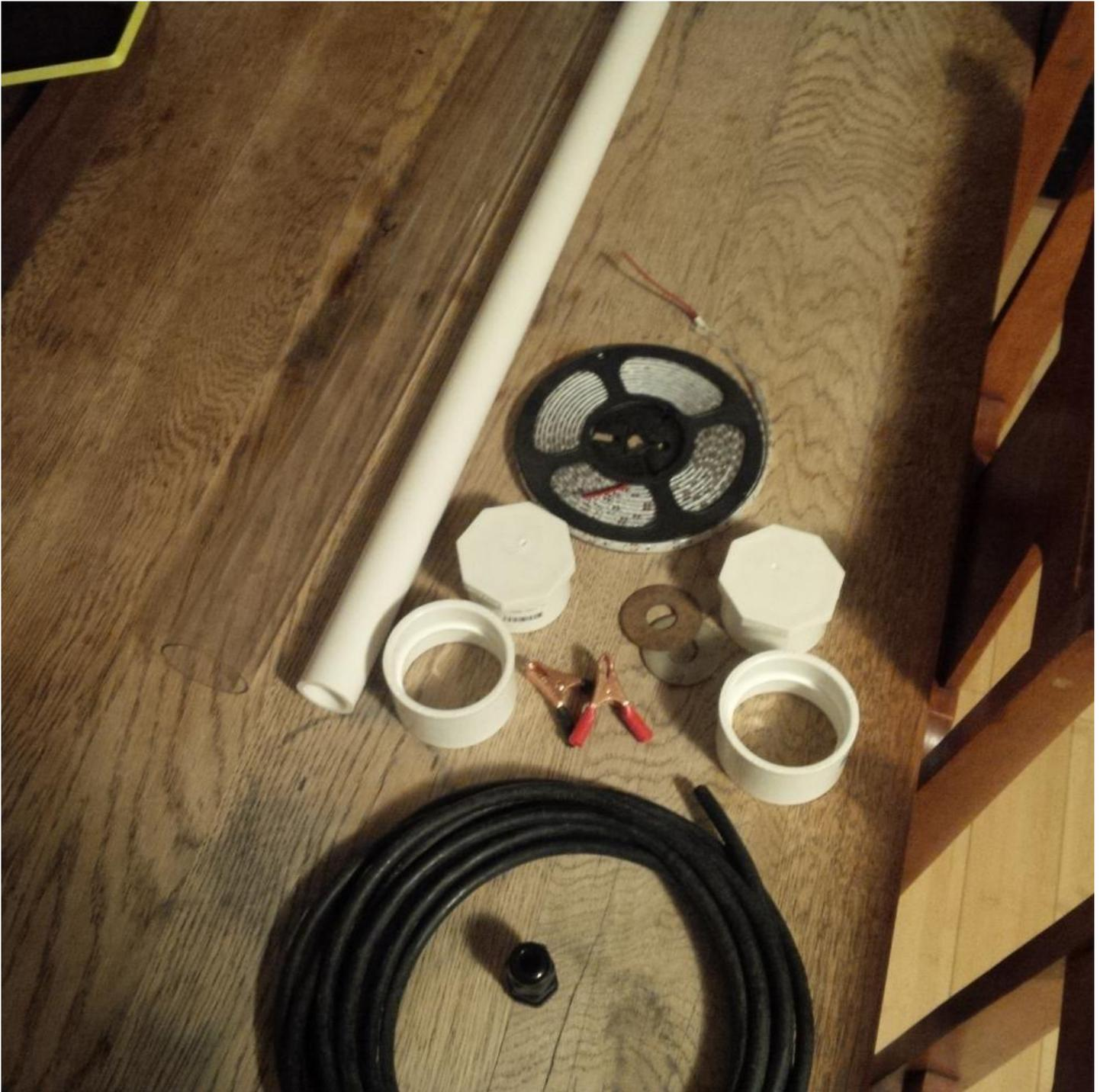
Minus those couplings in the pic that I didn't use, the parts are simple and there are many ways to build it. Amazon has the led light strips and the acrylic tube. In all it can be built for under \$50. Light strip is 16' wrapped around 1" pvc then secured inside clear tube using large washers glued on the 1" pvc pipe ends. I used a plastic epoxy from loctite for the joints. Used a waterproof cable gland on the end cap, epoxy inside and out.
