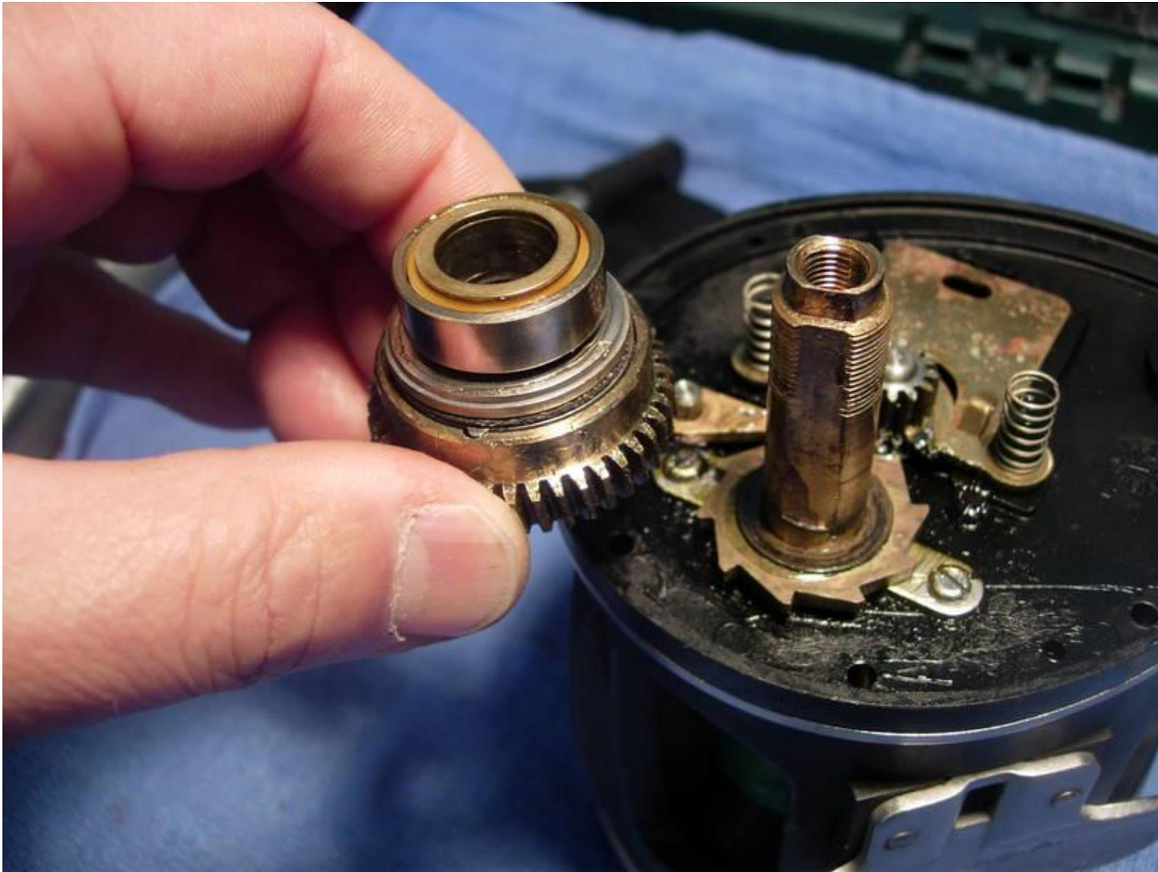
here is an exploded view of the gear cluster. going top left to bottom right, you have a fiber washer (key #4A), the 113h main gear (key #5), five 113h carbon fiber drag washers (key #6), five 113h metal washers (key #7), a belleville tension washer (key #18), a bearing washer (key #4), a bearing (key #55A), and another bearing washer (key #4).
