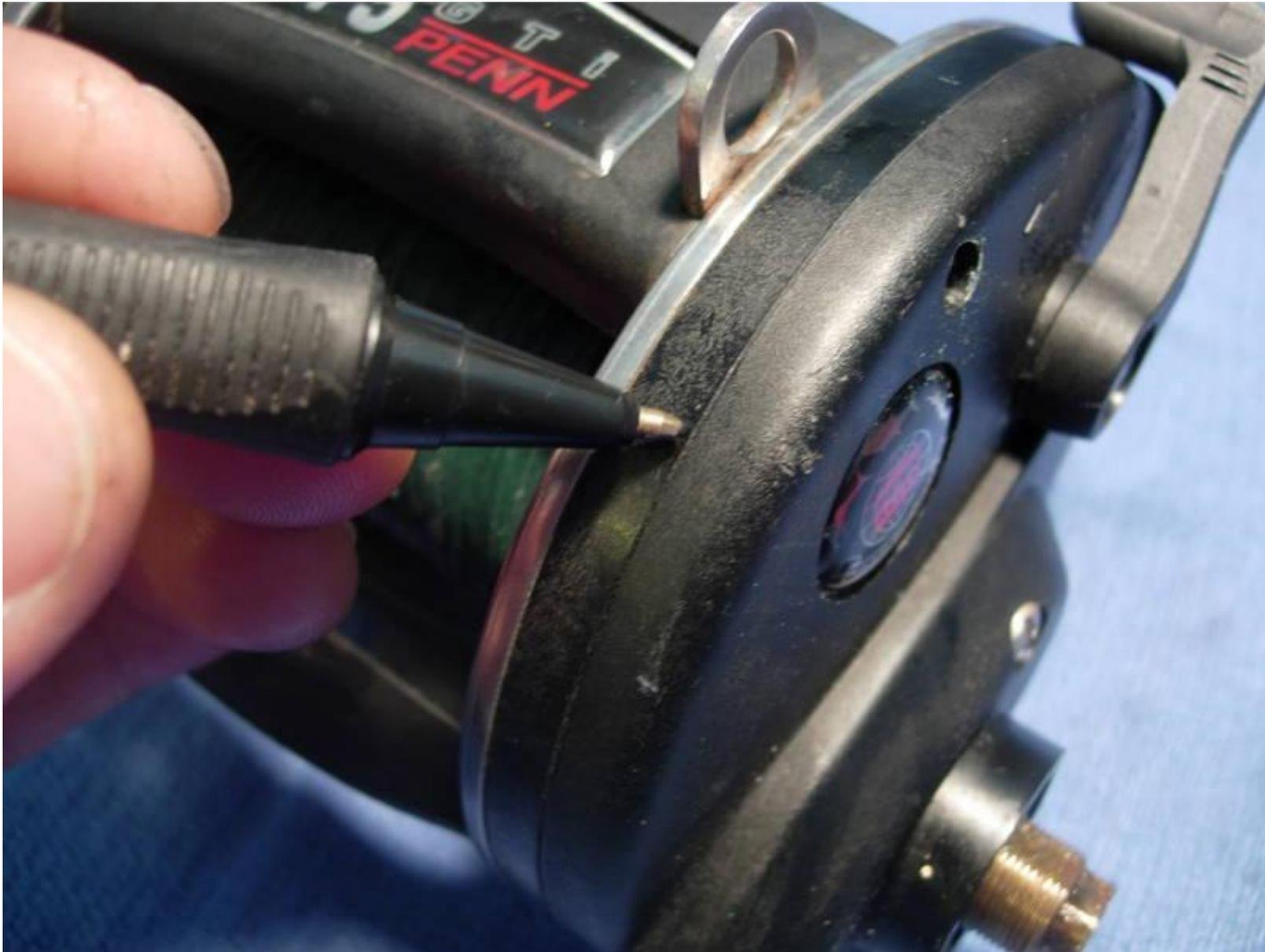
remove the two long (key #31) and three short (key#38) right side plate screws. do not remove the spool tension control screw (key #26B) in the center or the eccentric screw (key #22).
