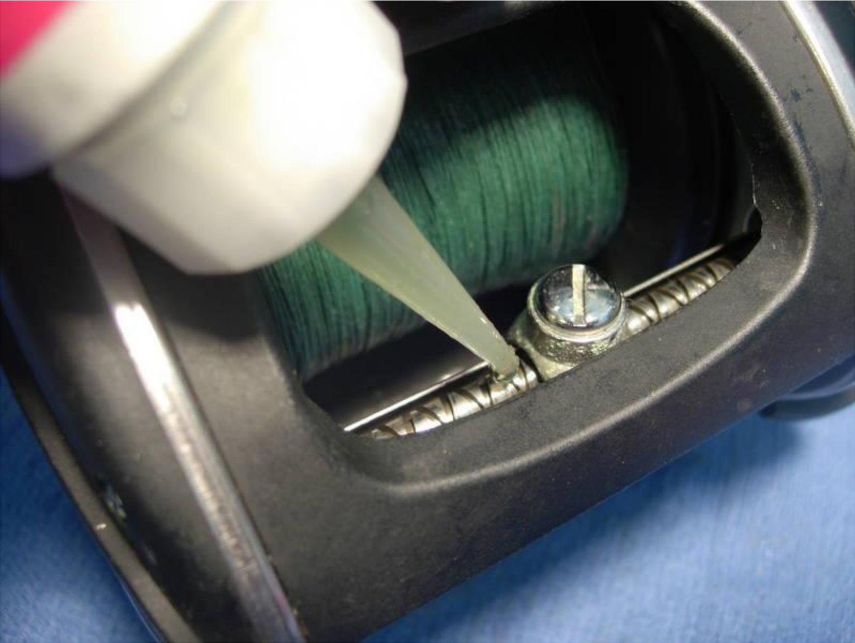
now, for the right side plate. remove the handle lock screw (key #110).
