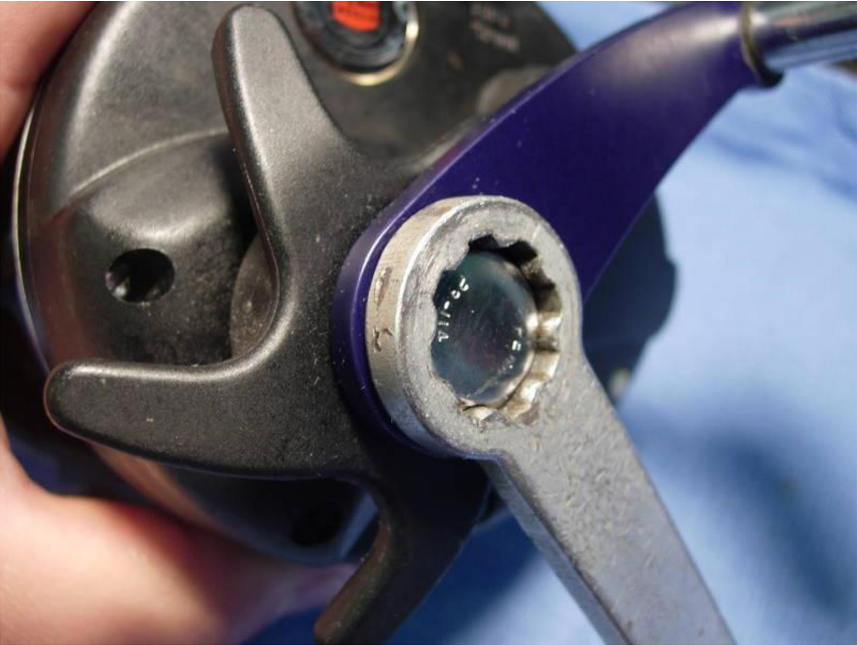
remove the handle assembly (key #24).
