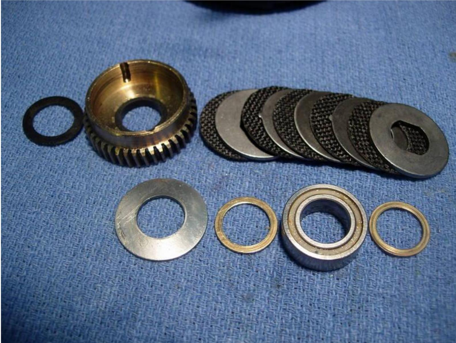
to eliminate the sticking caused by the fiber washer (key #4A), we are going to substitute a penn ht-100 drag washer (part #6-855). i have noted that these washers will soon be in short supply. there is no problem using a #6-113H washer. and honestly, if you don't need the drag to be super smooth, you can even leave the original fiber washer in.
