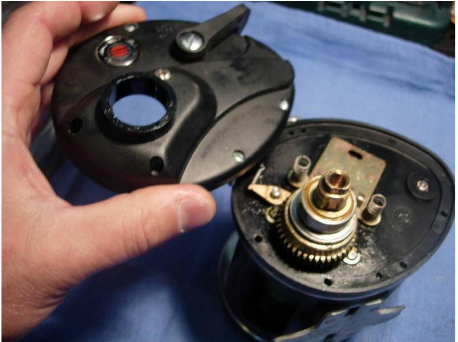
if the gear sleeve (key #98S) is not badly burred, you can lift the gear cluster off in one piece. otherwise, you may have to pull the pieces off one at a time.
