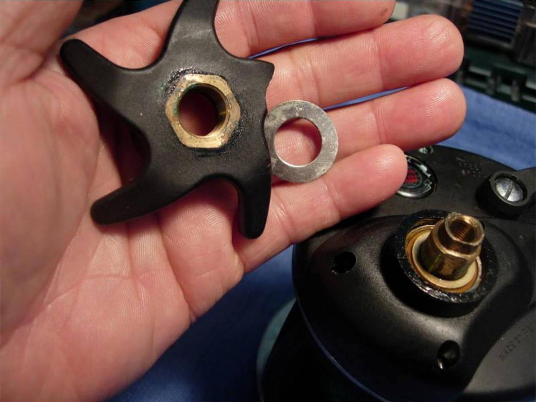
ok, now this is important. see the gap here? the right side plate is actually two pieces, a right side OUTER plate (key #1) and a right side INNER plate (key #1B). to service the right side plate, you need to remove the outer plate and leave the inner plate in place. got it? good! ok, let's start!
