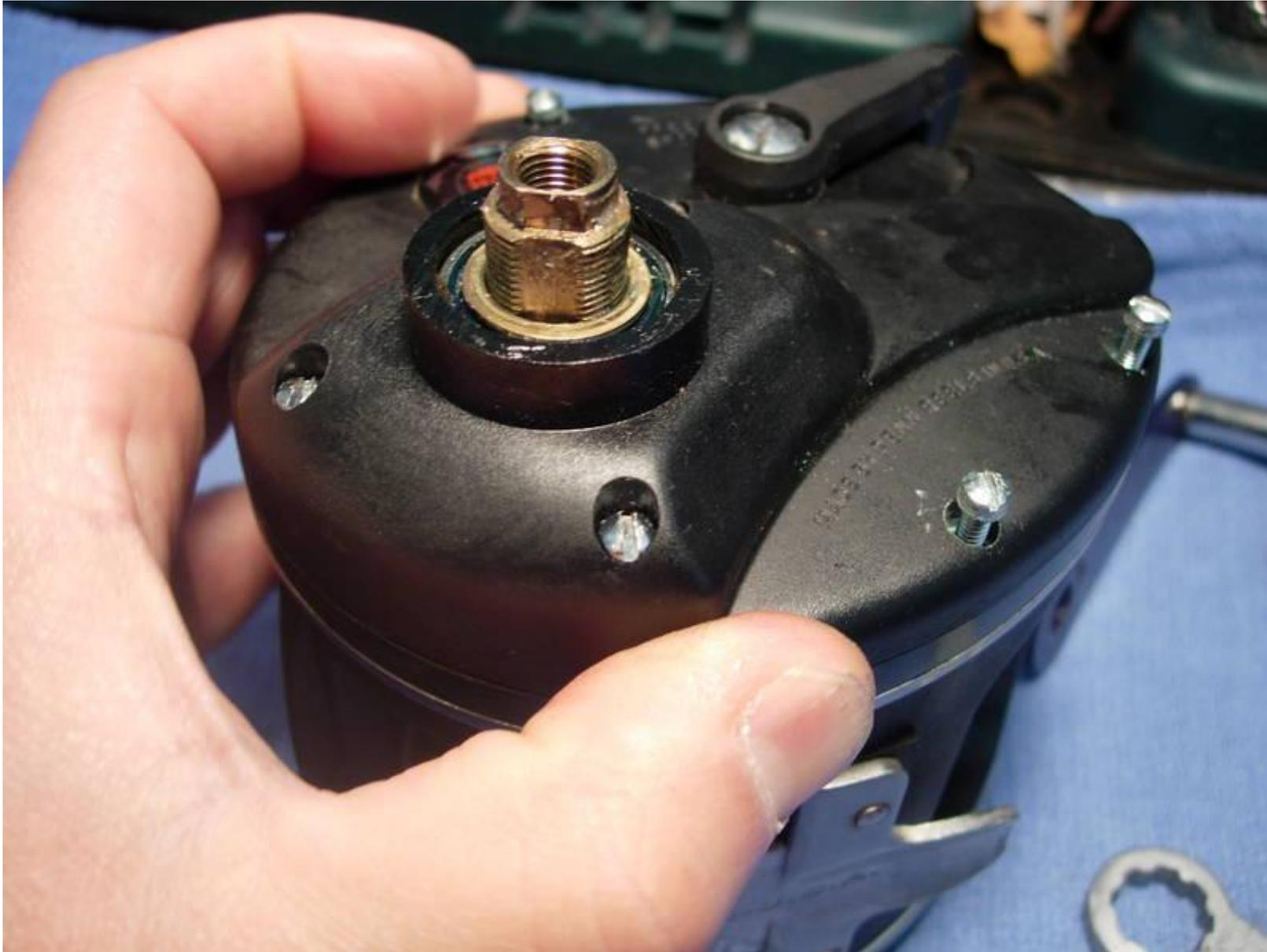
replace the long (key #31) and short (key #38) right side plate screws.
