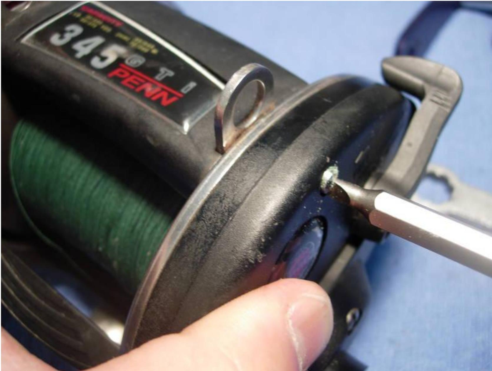
carefully separate the outer plate from the inner plate.
