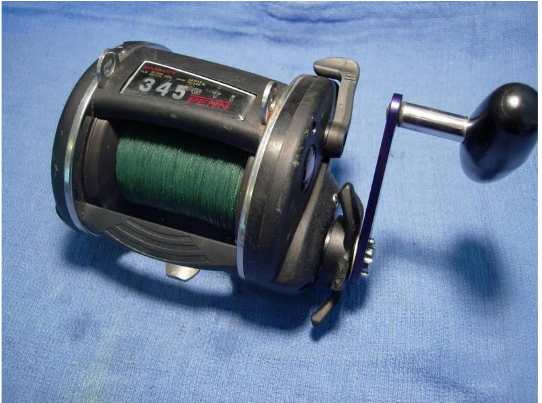
we are going to start by backing out all of the left side plate screws (key #'s 16 and 16A).
