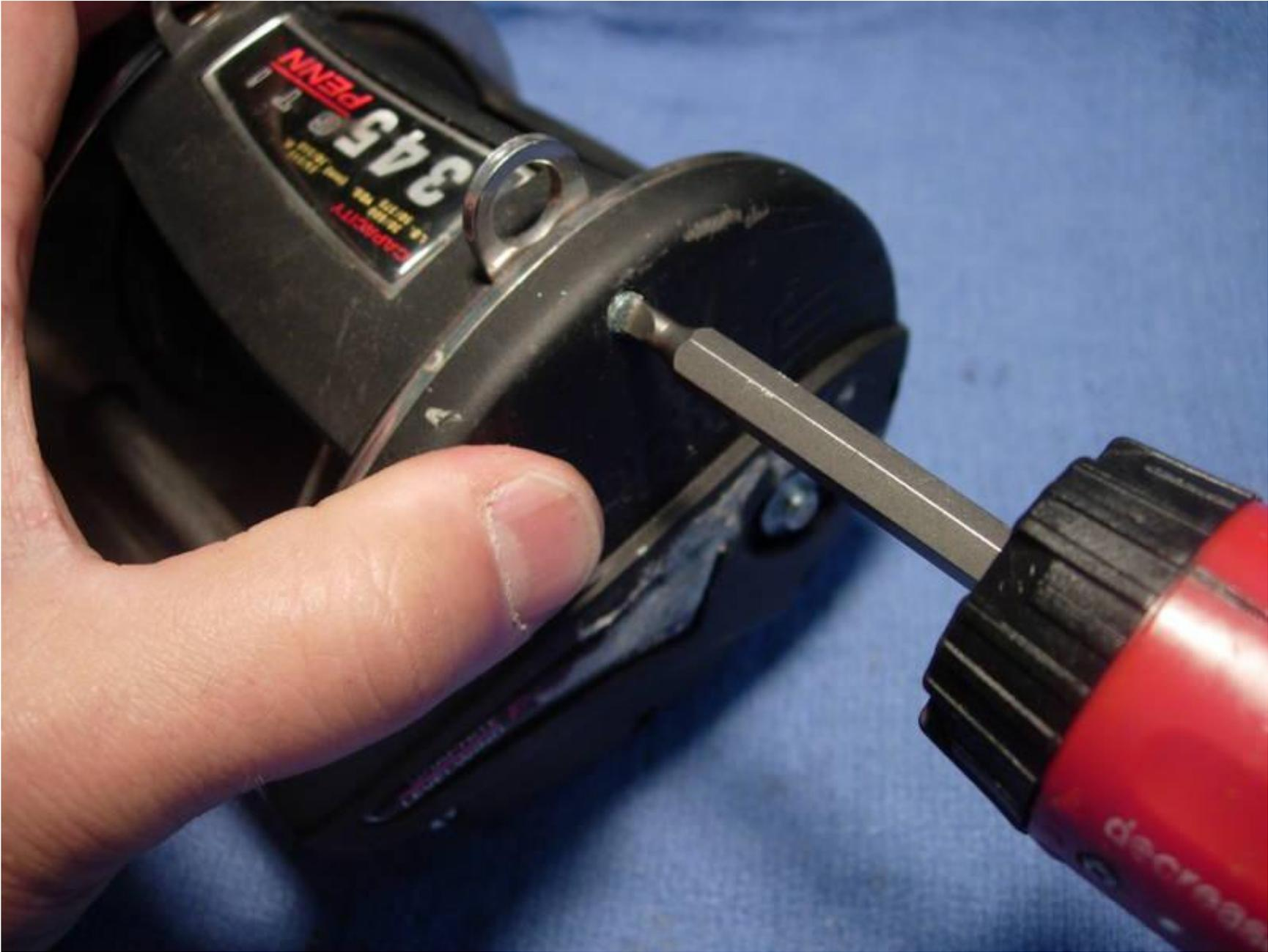
carefully remove the left side plate (key #27), leaving the levelwind assembly in place.
