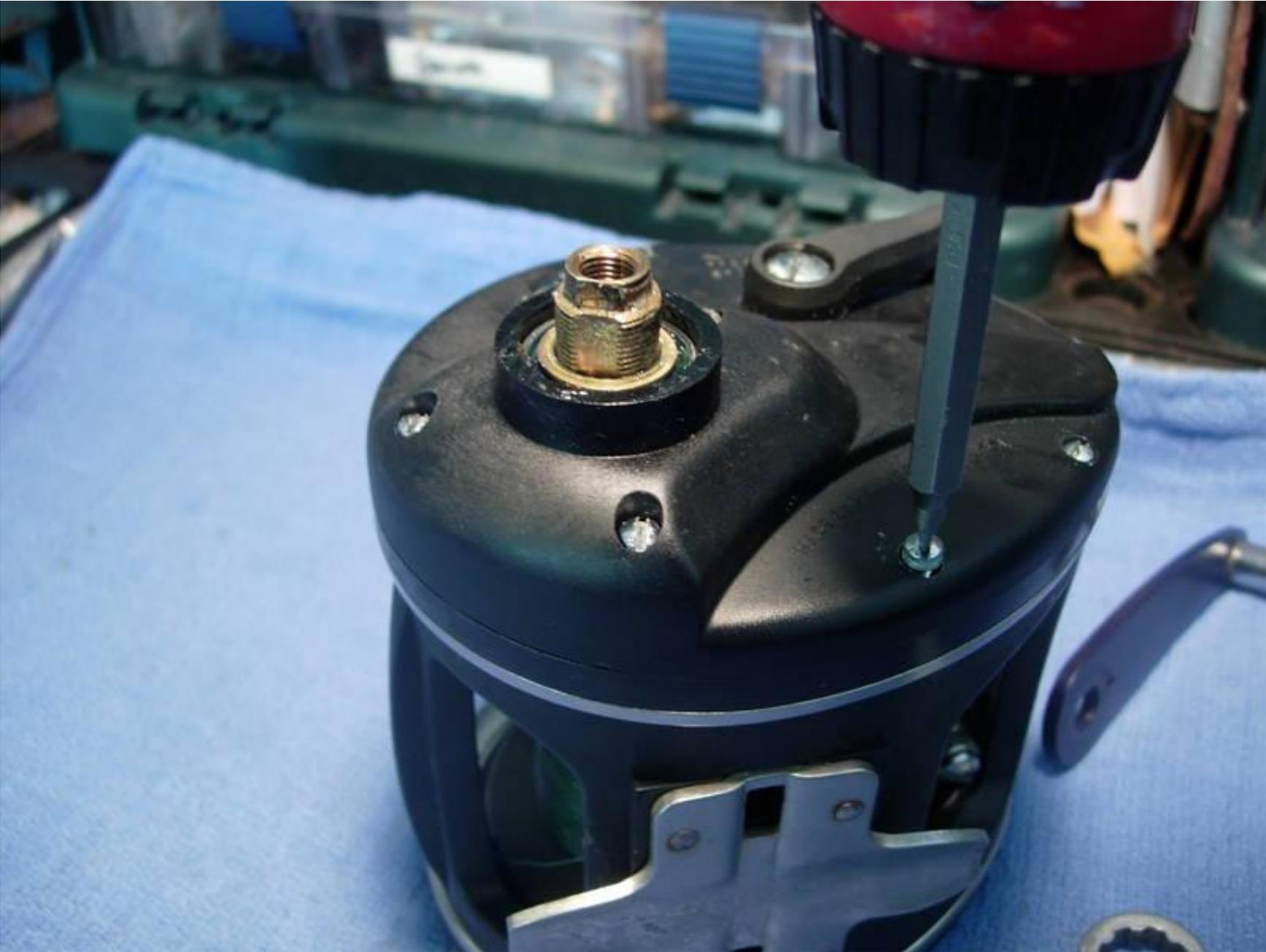
**install the star drag (key #10) and turn it down until it clears the shoulder of the gear sleeve (key #98S) to properly install the handle assembly (key #24).**
