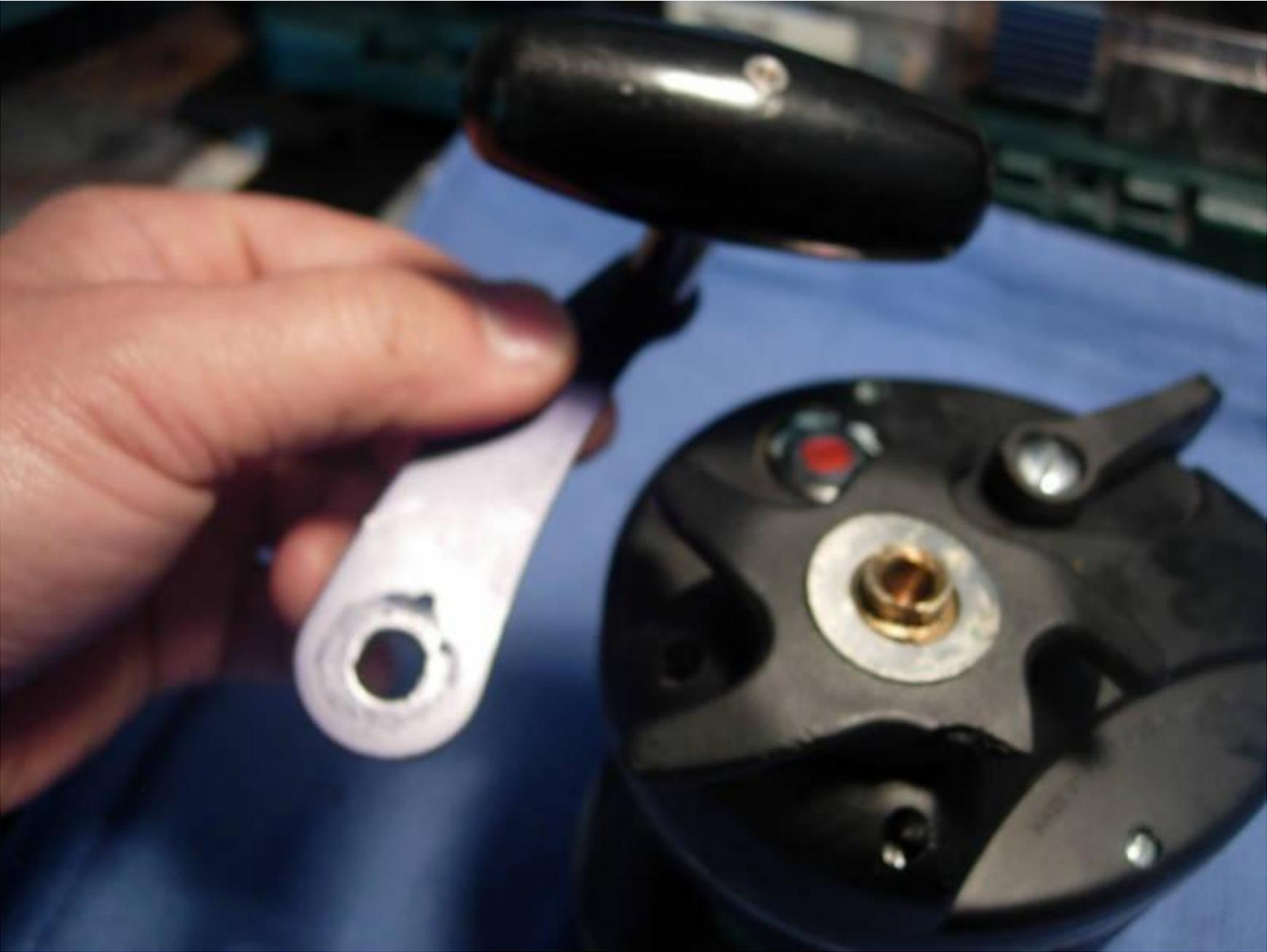
remove the tension spring (key #8) and star drag (key #10). i typically discard the spring.
