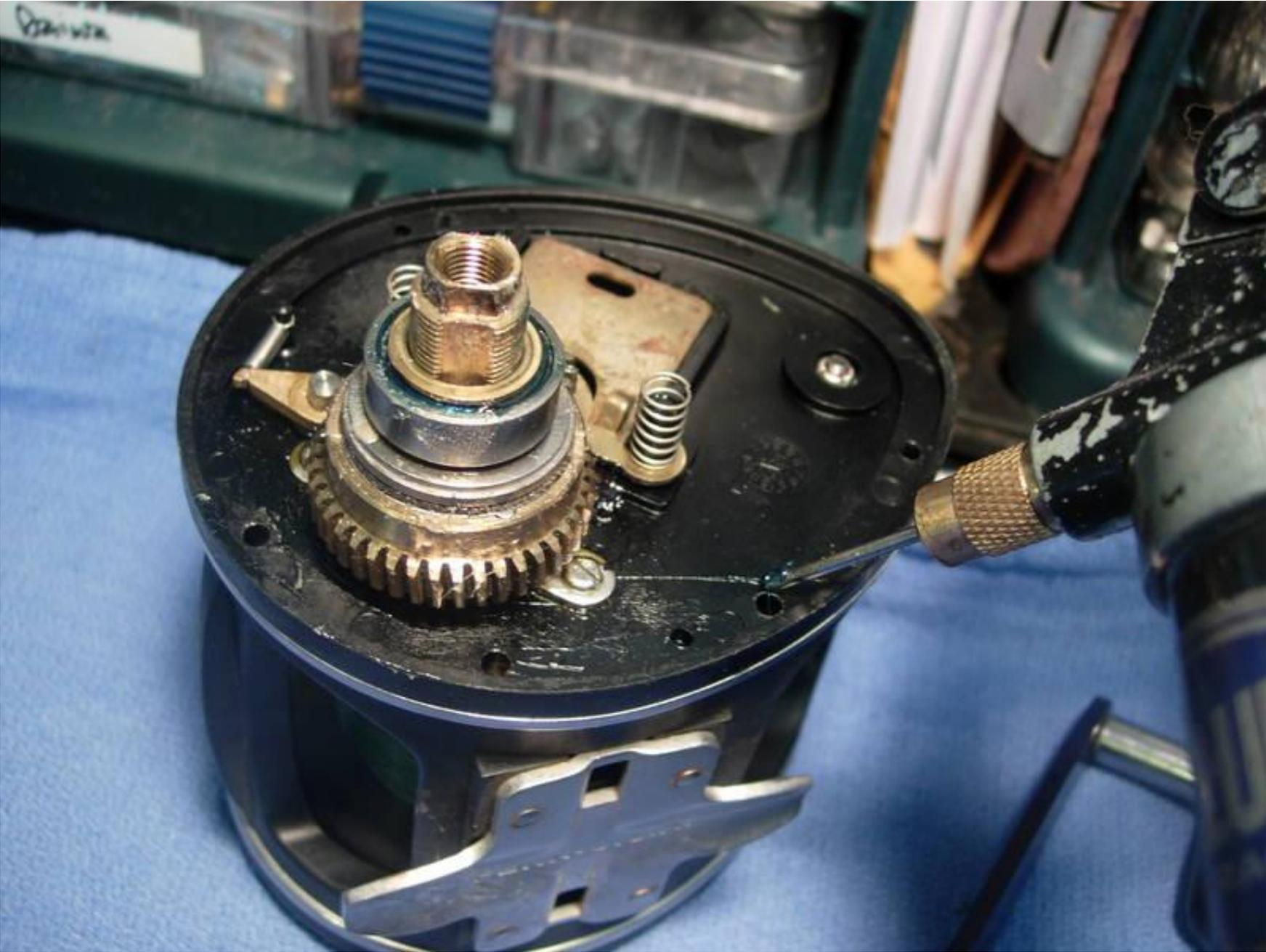
carefully replace the right side outer plate (key #1) with the eccentric jack (key #11) in the "up" position and the eccentric lever (key #21) in the "back" or "free" position (not the "forward" or "in gear" position shown in the photo).
