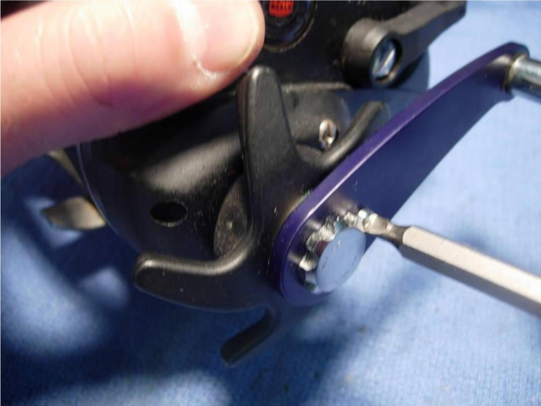
remove the handle assembly screw (key #23).
