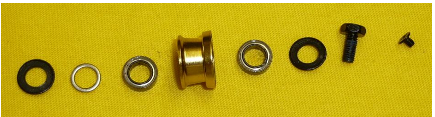
bearing dimensions 5x8x2,5mm
