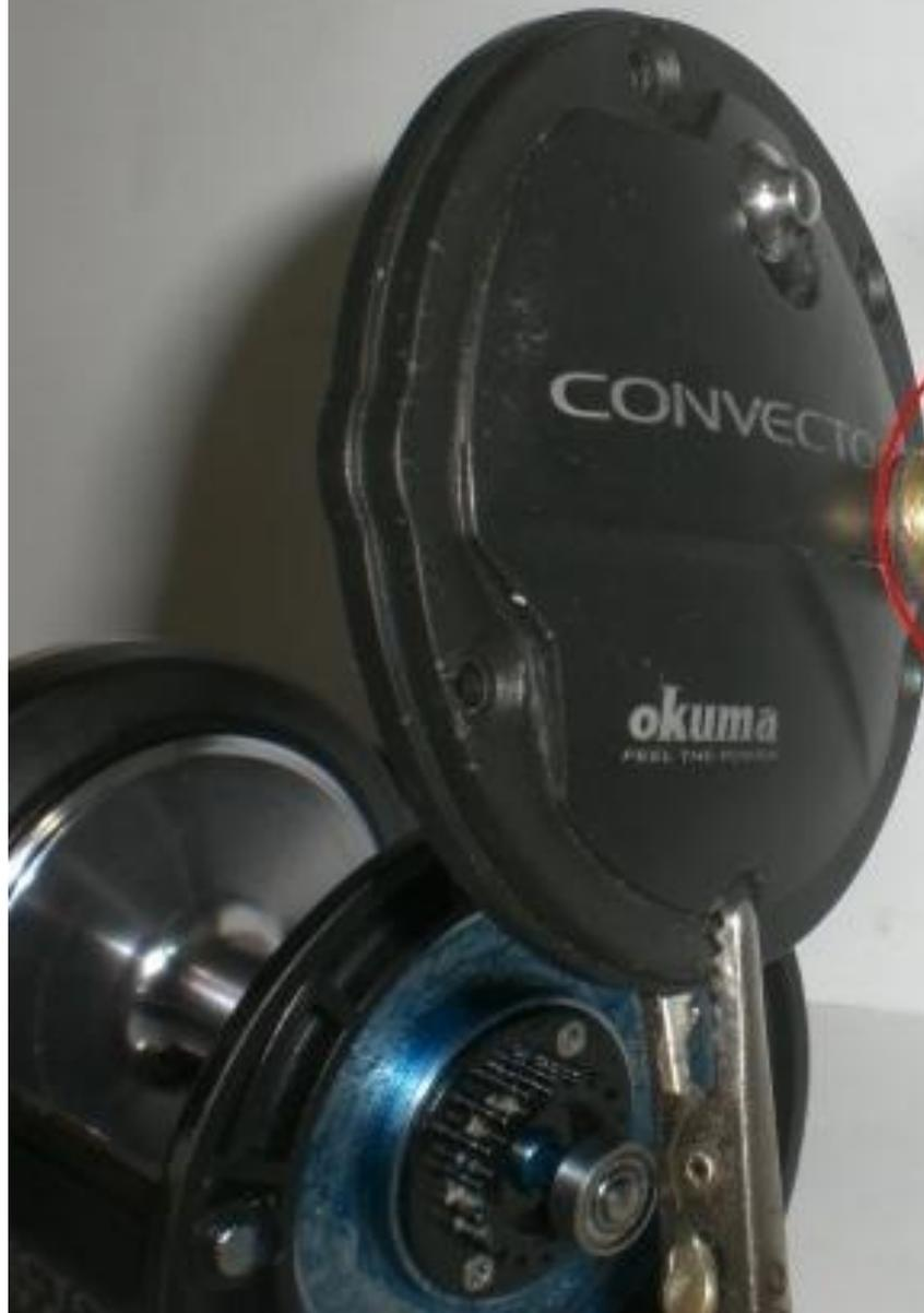
Width has been taken right down to 1mm. Note more space has been created along the bolt shaft.
