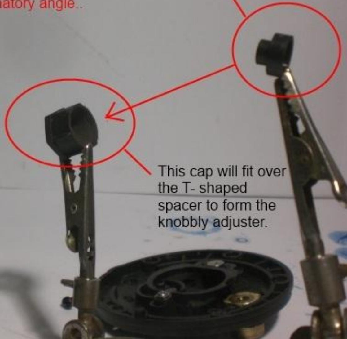
This cap will fit over the T-shaped spacer to form the knobby adjuster.
