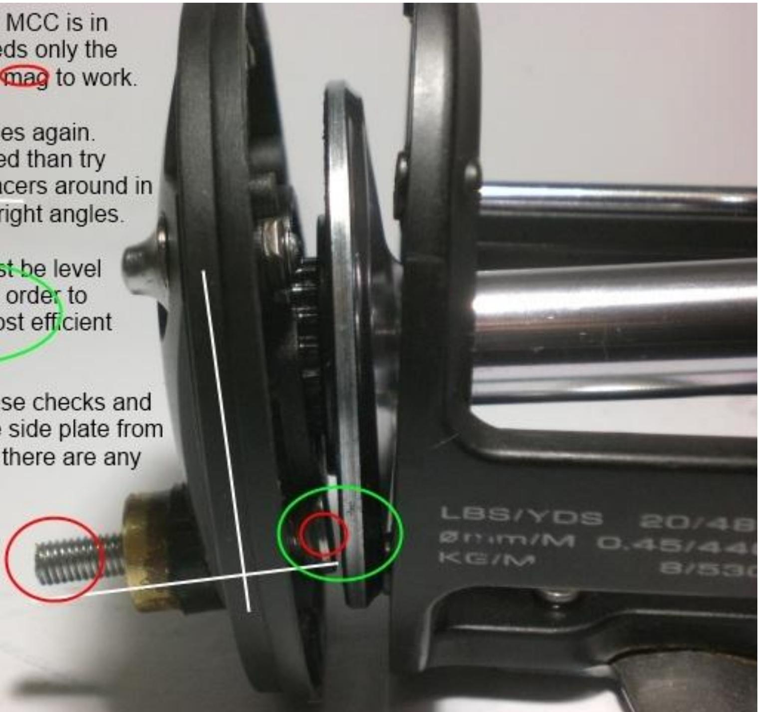
Remove the bolt from the unit completely. Select a magnet that is 5mm wide x1mm or 2mm thick.
