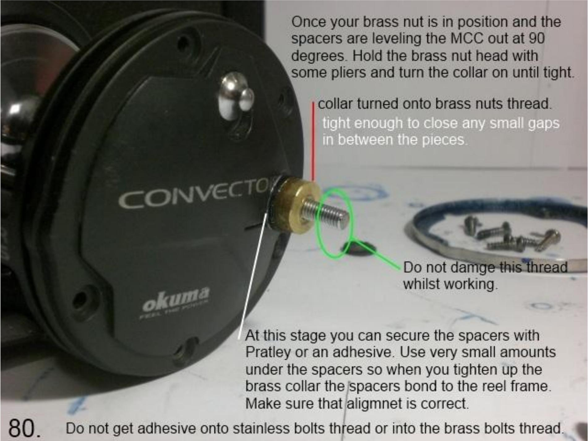
Once your brass nut is in position and the spacers are leveling the MCC out at 90 degrees. Hold the brass nut head with some pliers and turn the collar on until tight.
