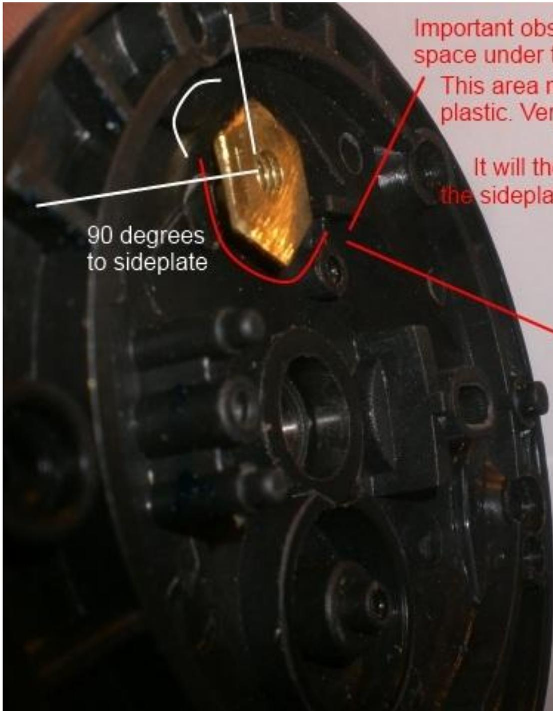
Important observation - Note the size and shape of space under the bolt head.
