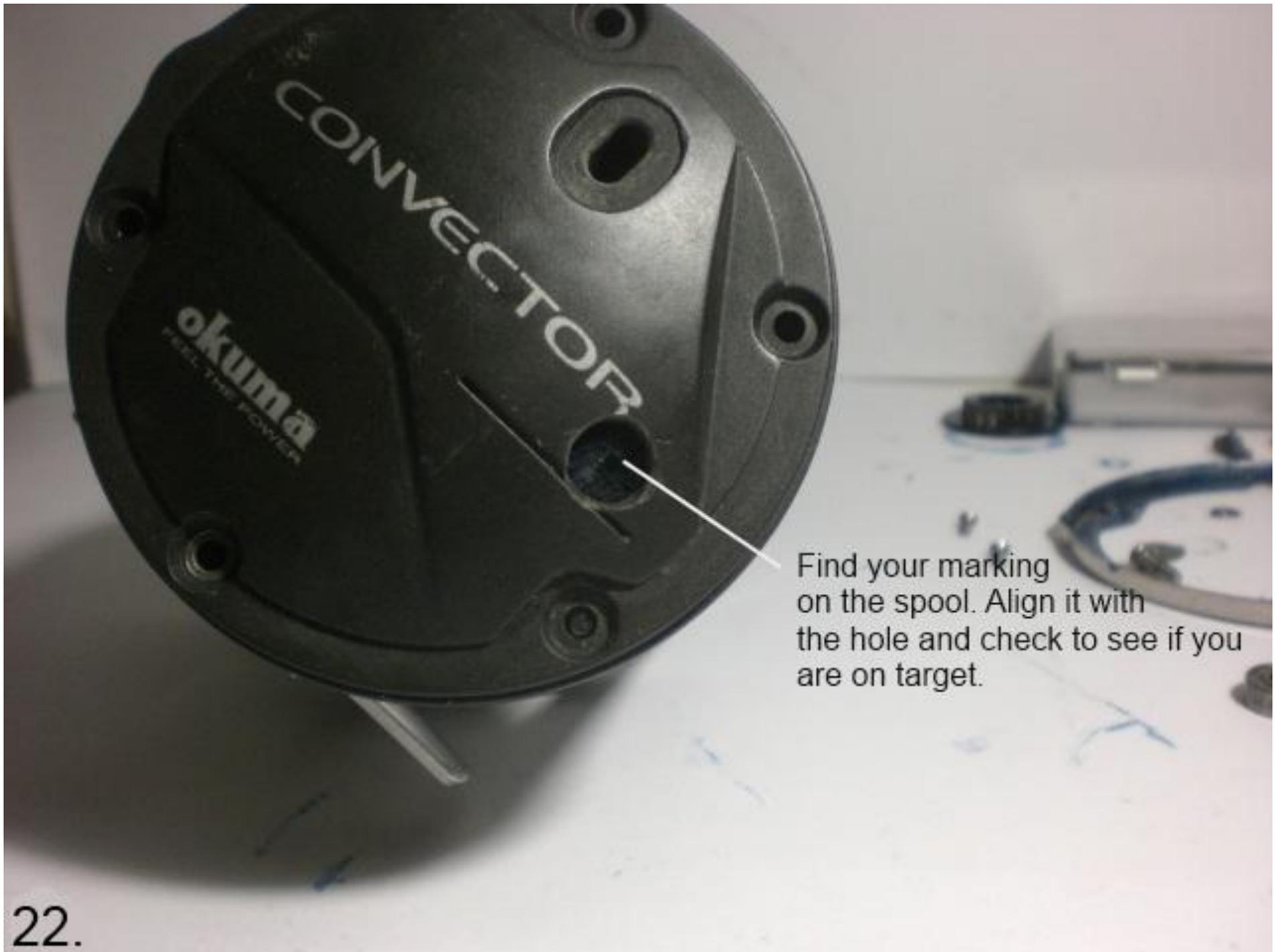
Find your marking on the spool. Align it with the hole and check to see if you are on target.
