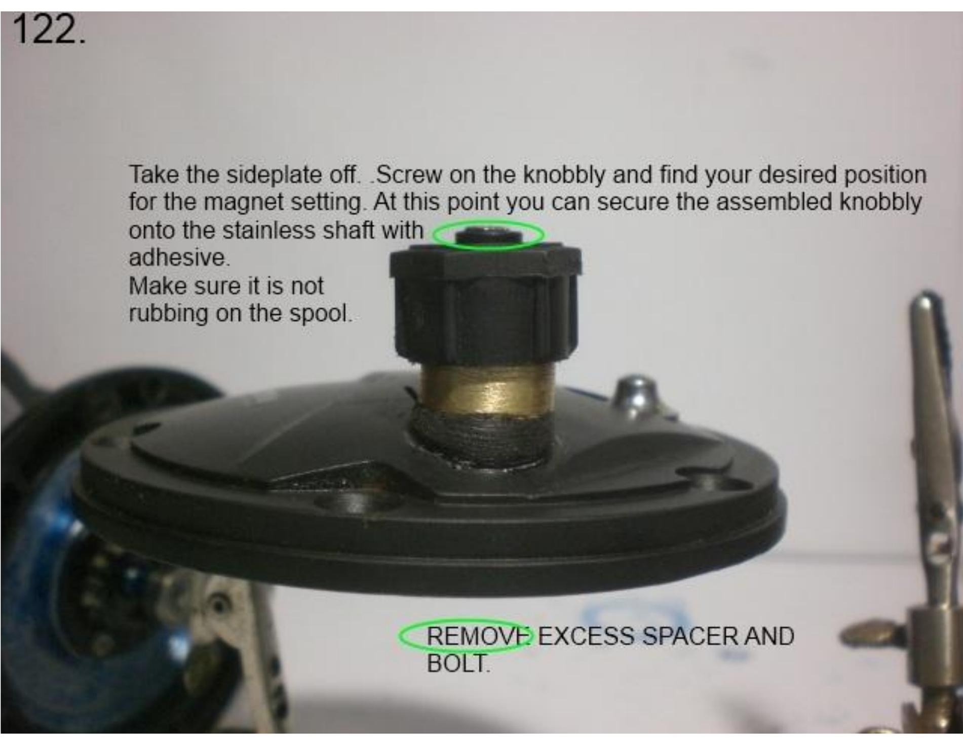
~~REMOVE~~ EXCESS SPACER AND BOLT.
