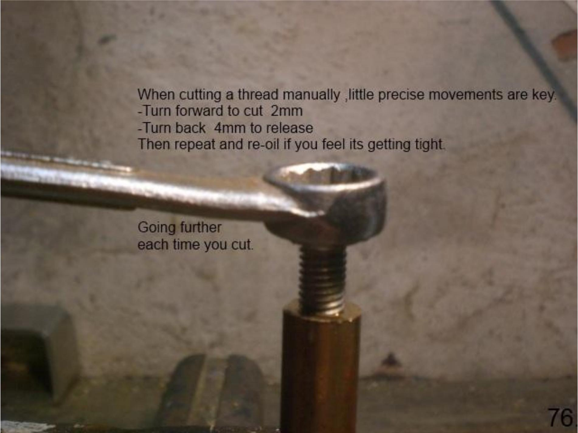
When cutting a thread manually ,little precise movements are key.
