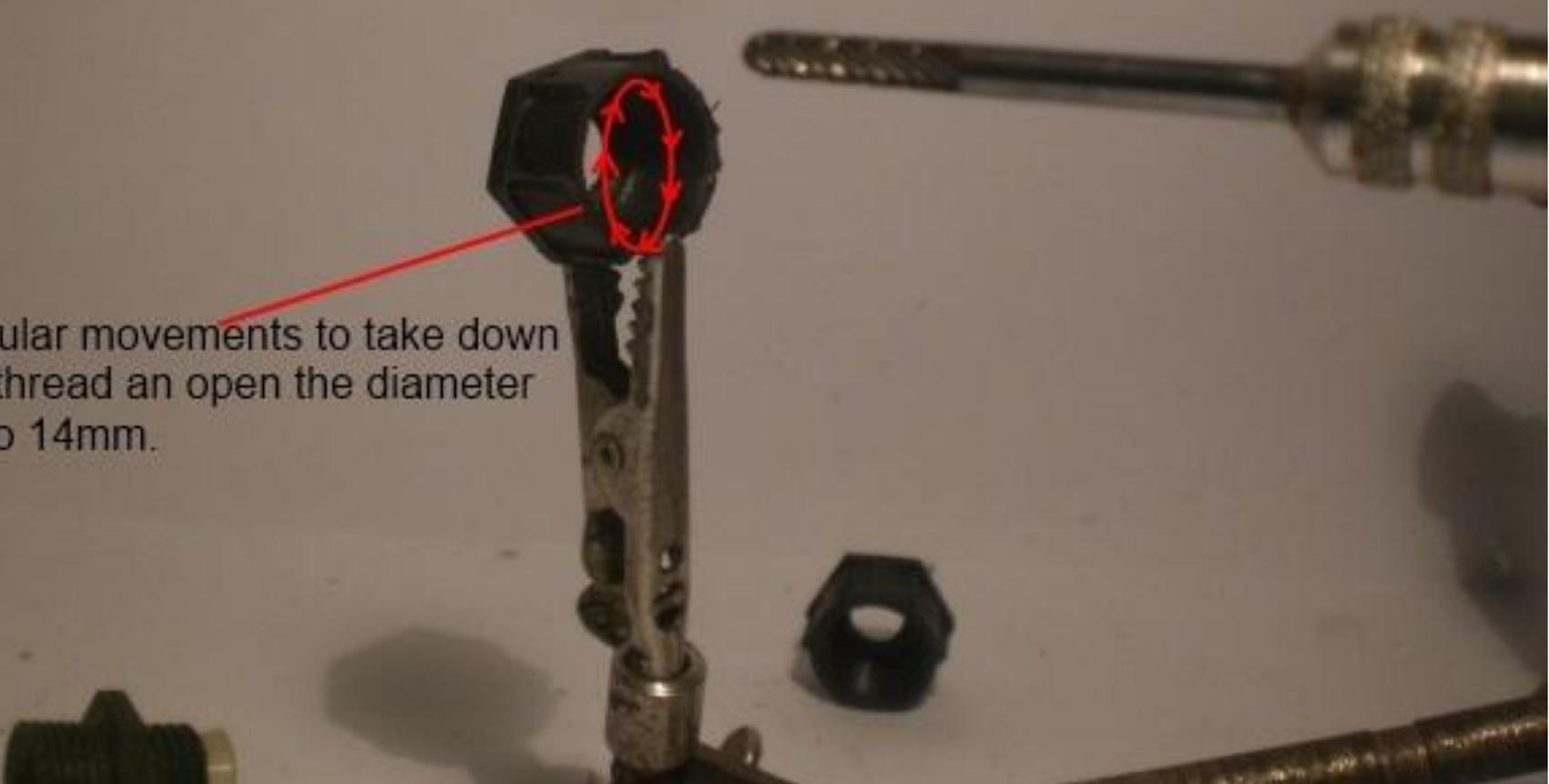
Circular movements to take down the thread and open the diameter up to 14mm.
