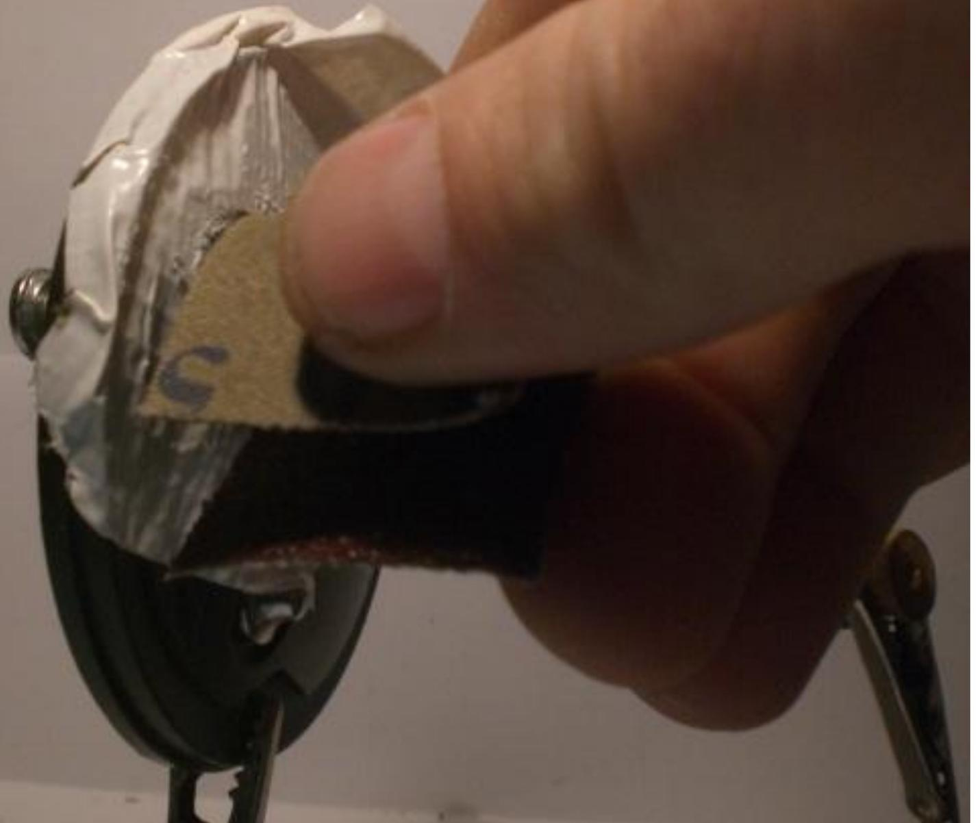
Once it has been sand and cleaned properly remove the tape.
