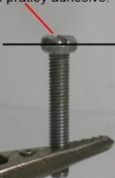
Some reels have very little space to operate a mag break. Grinding this bolt head down to a platform of 1mm thick will help the issue.
