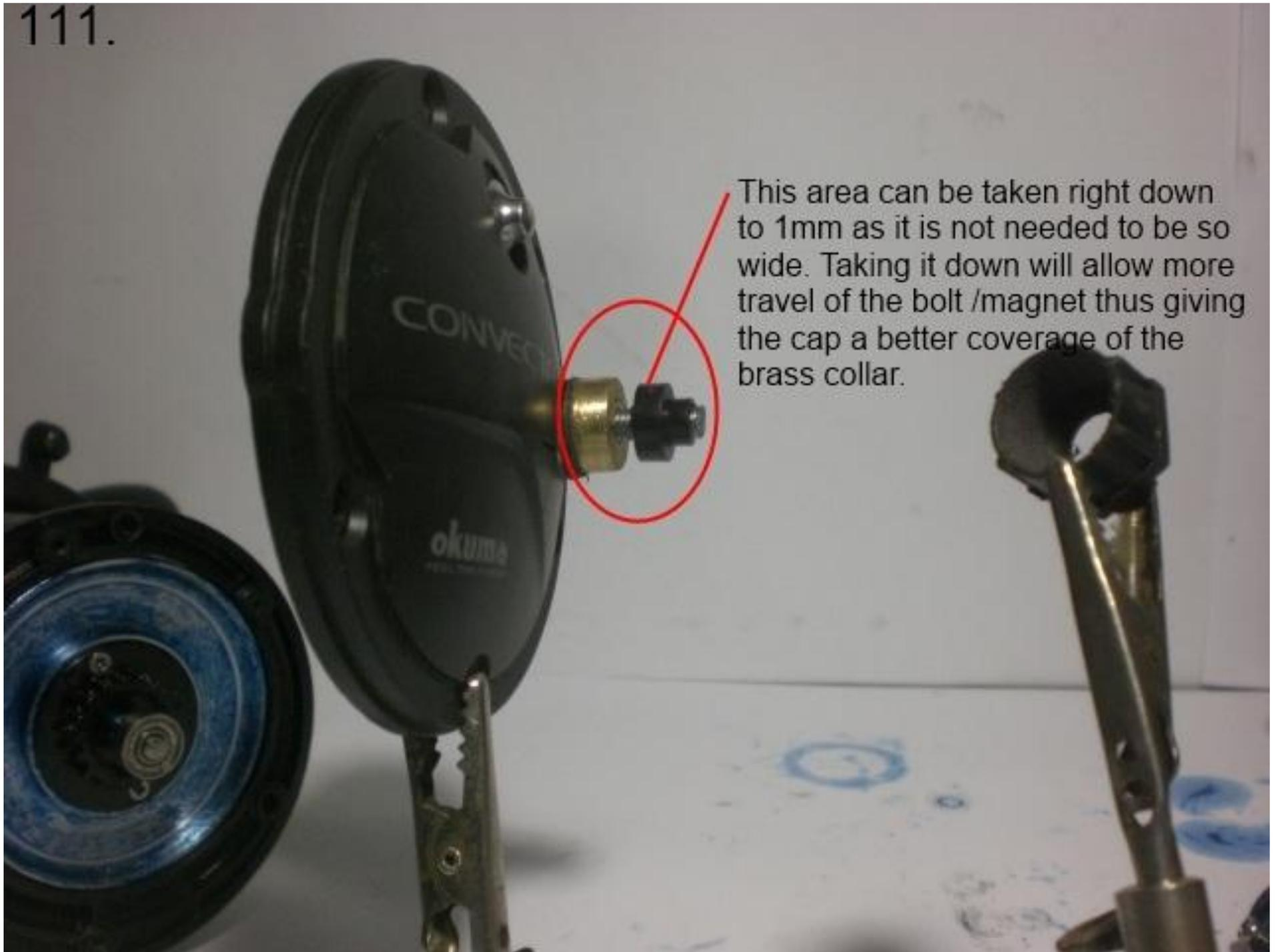
This area can be taken right down to 1mm as it is not needed to be so wide. Taking it down will allow more travel of the bolt /magnet thus giving the cap a better coverage of the brass collar.
