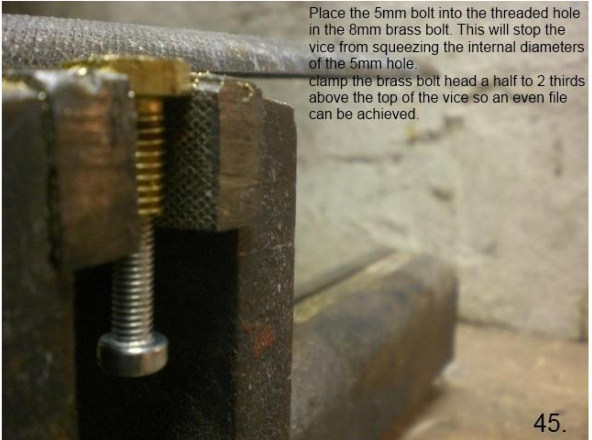
Place the 5mm bolt into the threaded hole in the 8mm brass bolt. This will stop the vice from squeezing the internal diameters of the 5mm hole.
