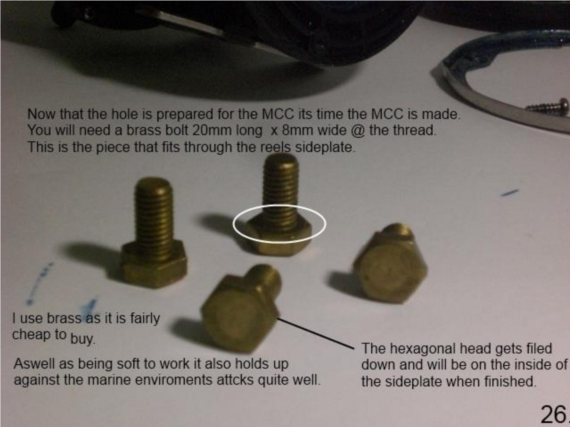
Now that the hole is prepared for the MCC its time the MCC is made.
