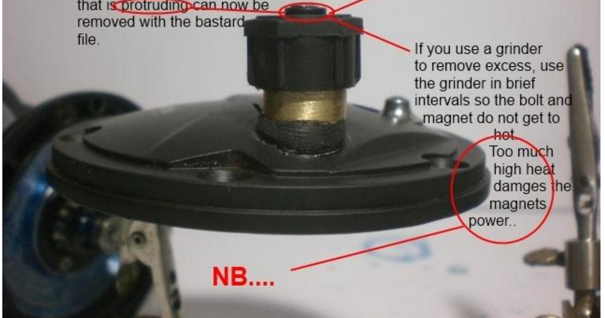
HOMESTRETCH - At this point the knobby should be secure, but when turned out to its max off position it will lock at the spring point inside the reel allowing the unsecured spacer thread on the stainless bolt shaft to turn off.
