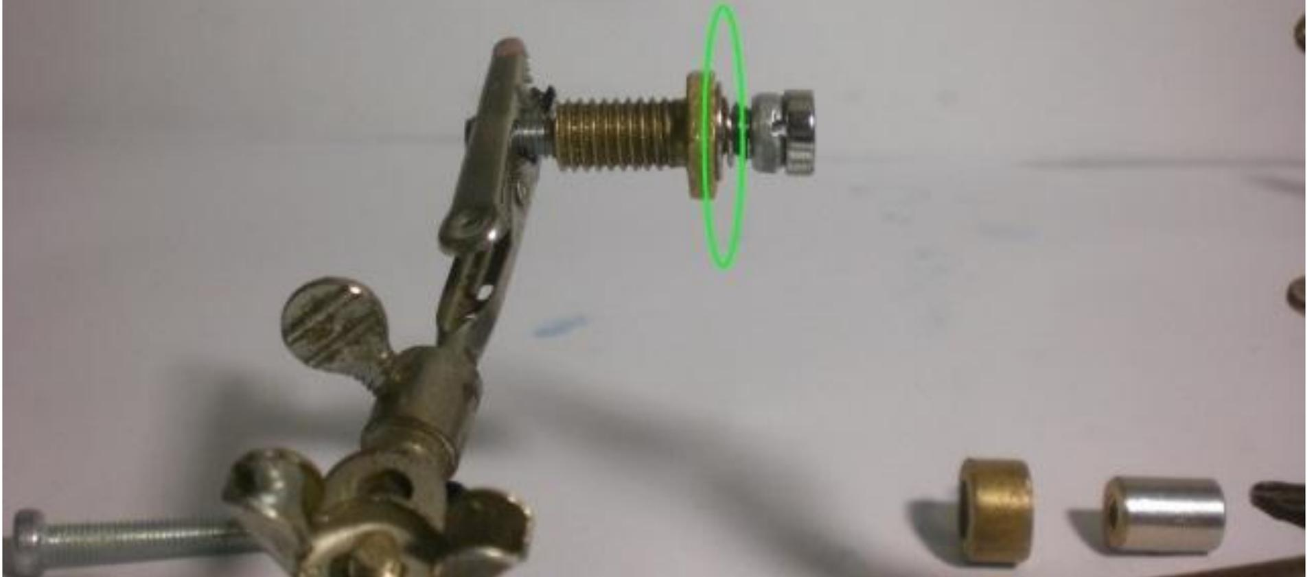
With the magnet in place run the bolt back into the MCC unit and place the sideplate onto the reel frame.
