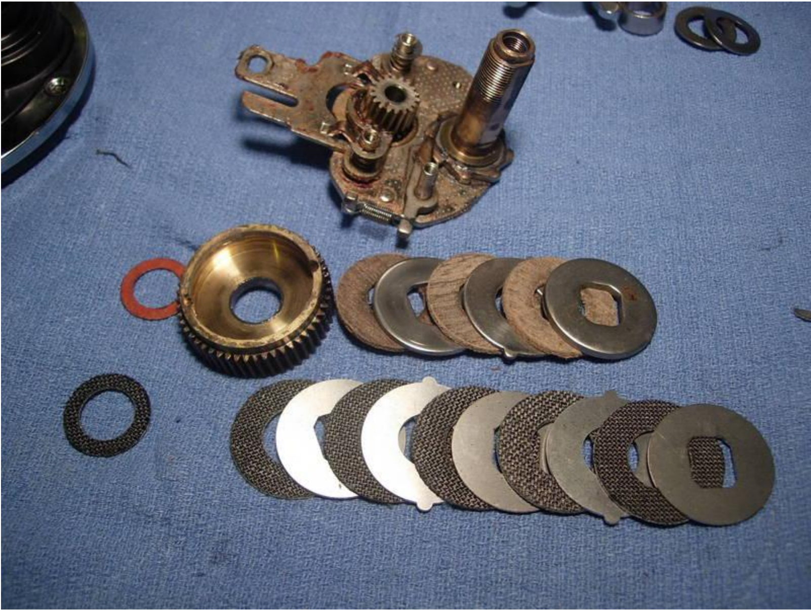
here's the old stack of drag washers compared to the new stack.
