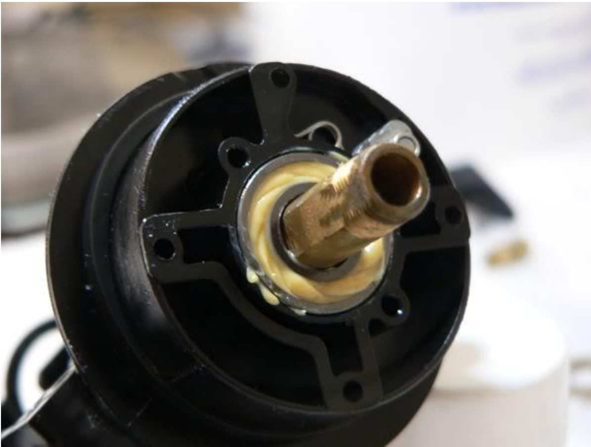
Reattach the clutch bearing
