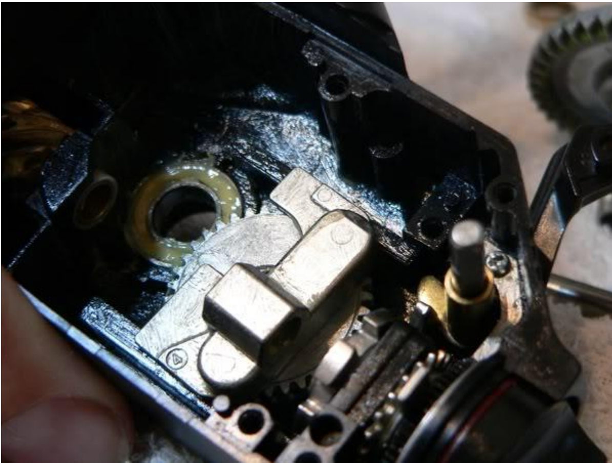
Slide the main shaft back into the reel, securing it with the c-clips on either side of the oscillating slider
