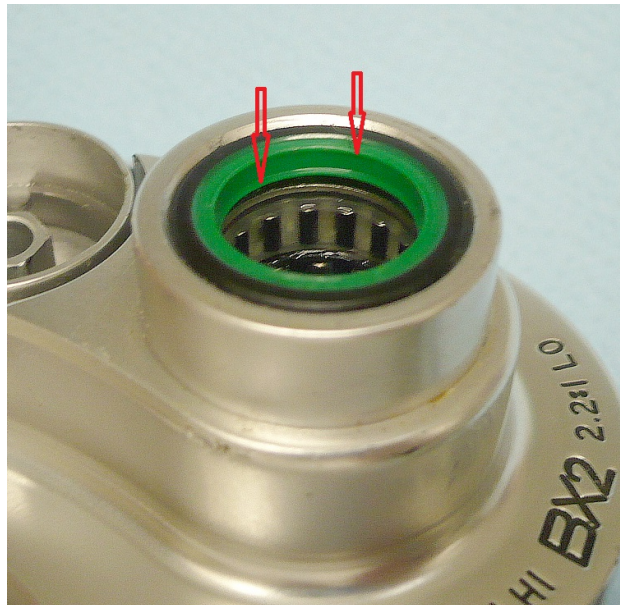
HFL Bearing 14x20x26MM The integrated ball bearings at both ends are clearly visible
