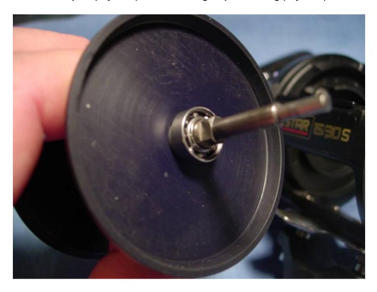
This bearing is 6x12x4 mm. W clean it with carb cleaner and compressed air, then lube it with Corrosion X.
