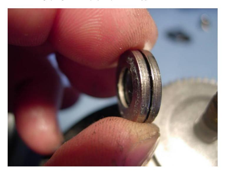
Install the bearing thrust washer (key #91).
