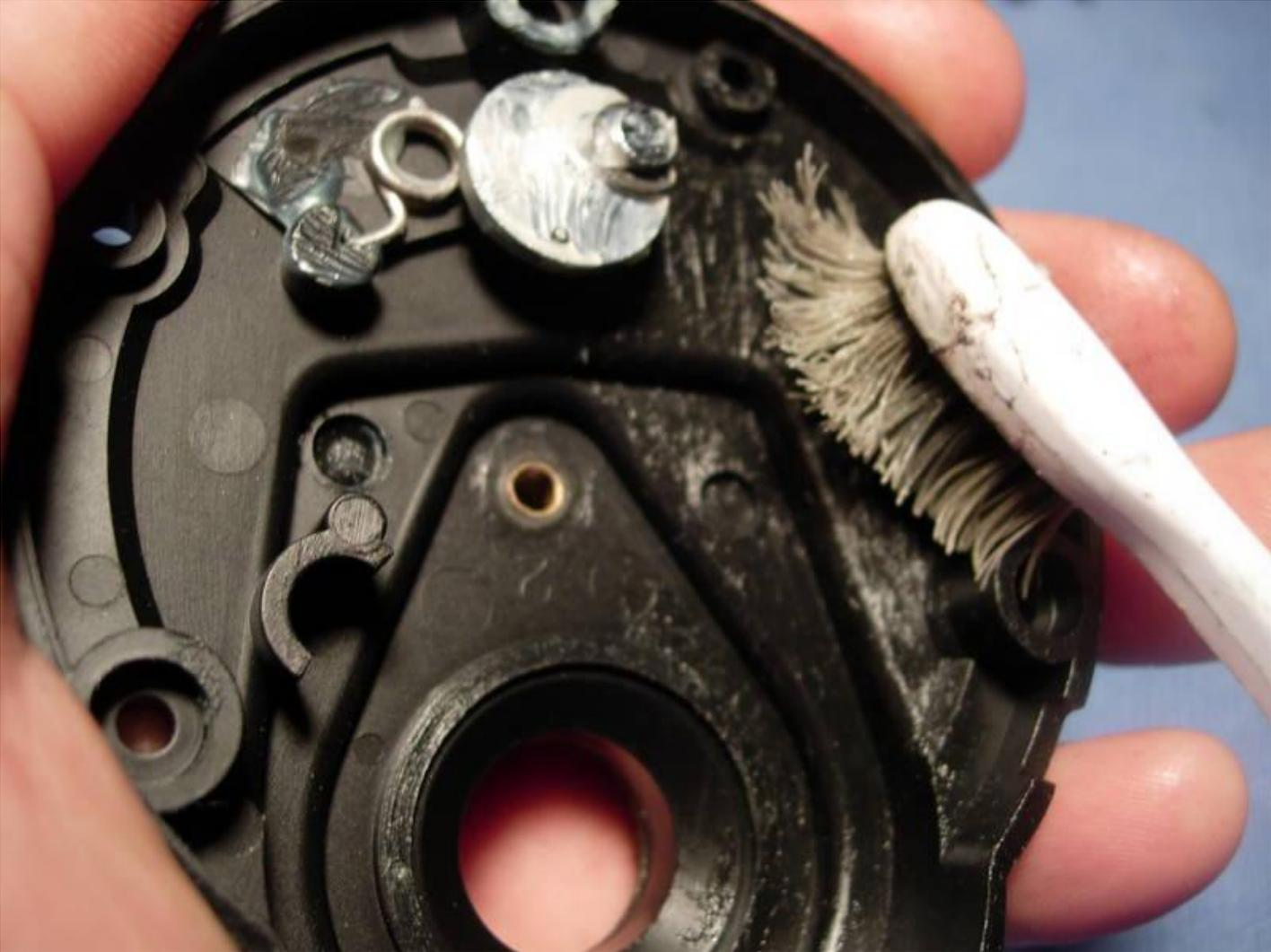
Install the right side plate, noting the "up" position of the yoke plate (key #259) and "forward" position of the clutch lever (key #132).
