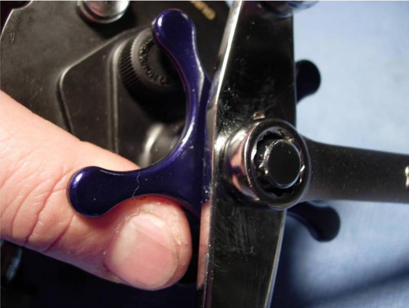
**Install the handle nut plate (key #2) and screw (key #128).**
