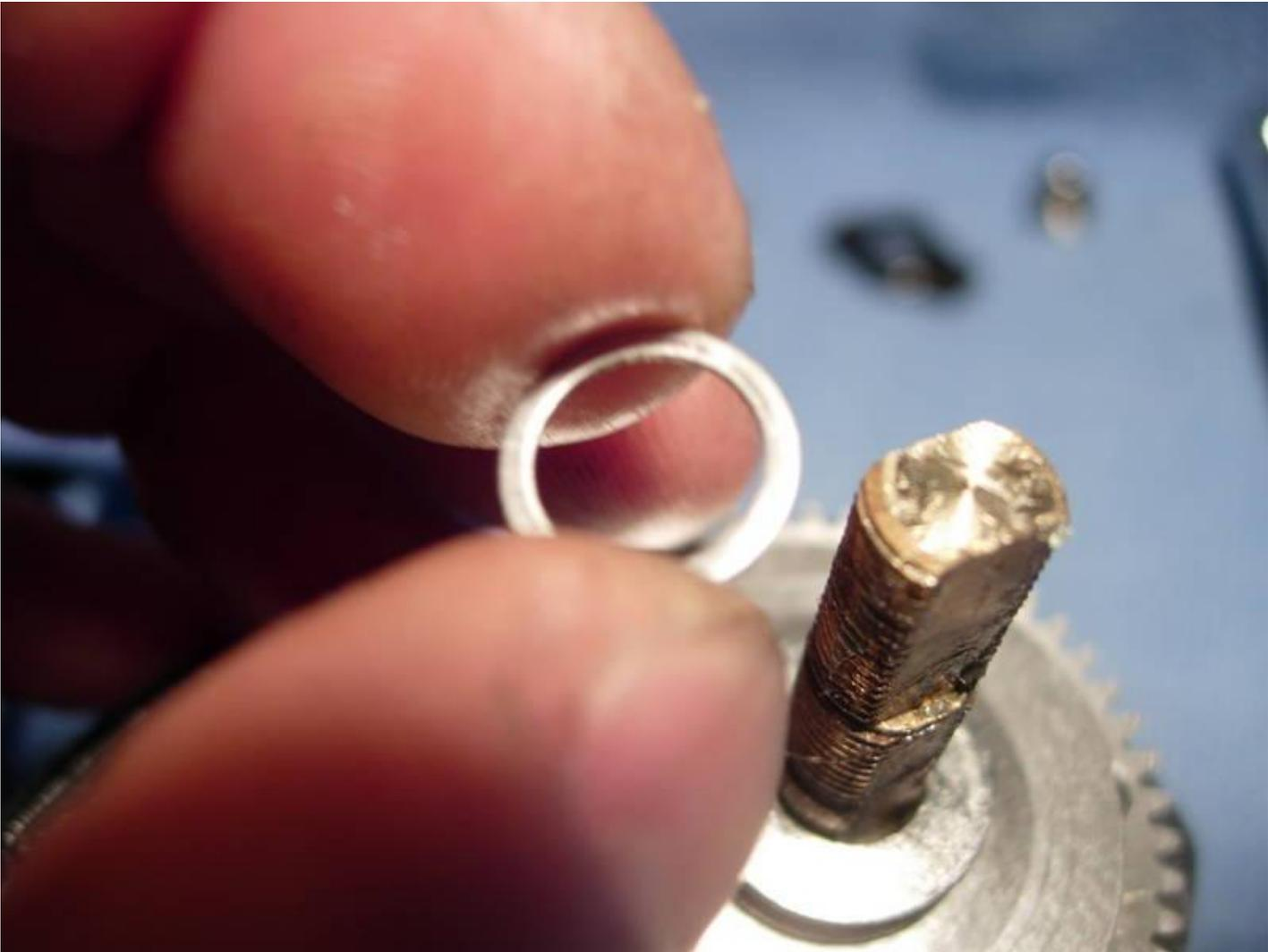
**Grease and install the drive shaft bearing (key #483).**
