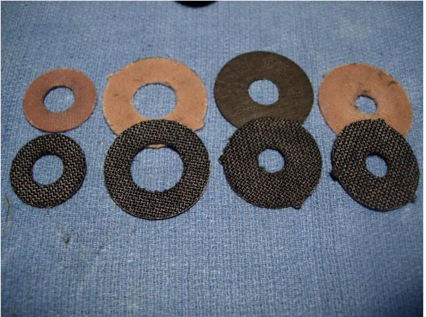
**Apply a coat of cal's drag grease to all four of the carbon fiber drag washers.**
