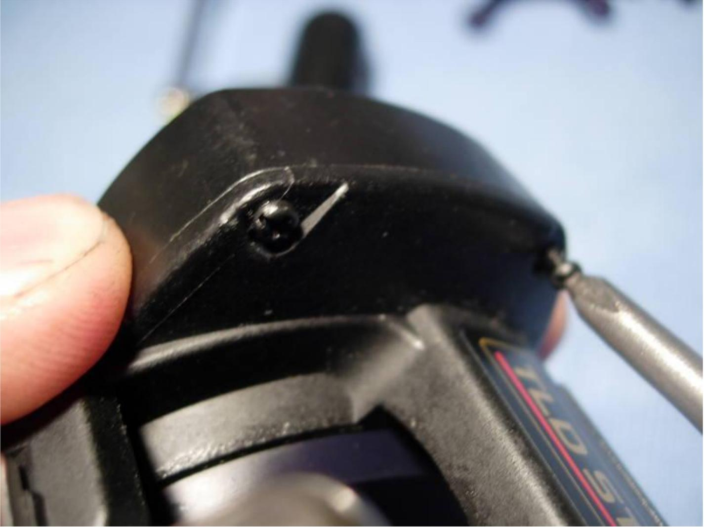
Remove the four right side plate screws "a" (key #81).
