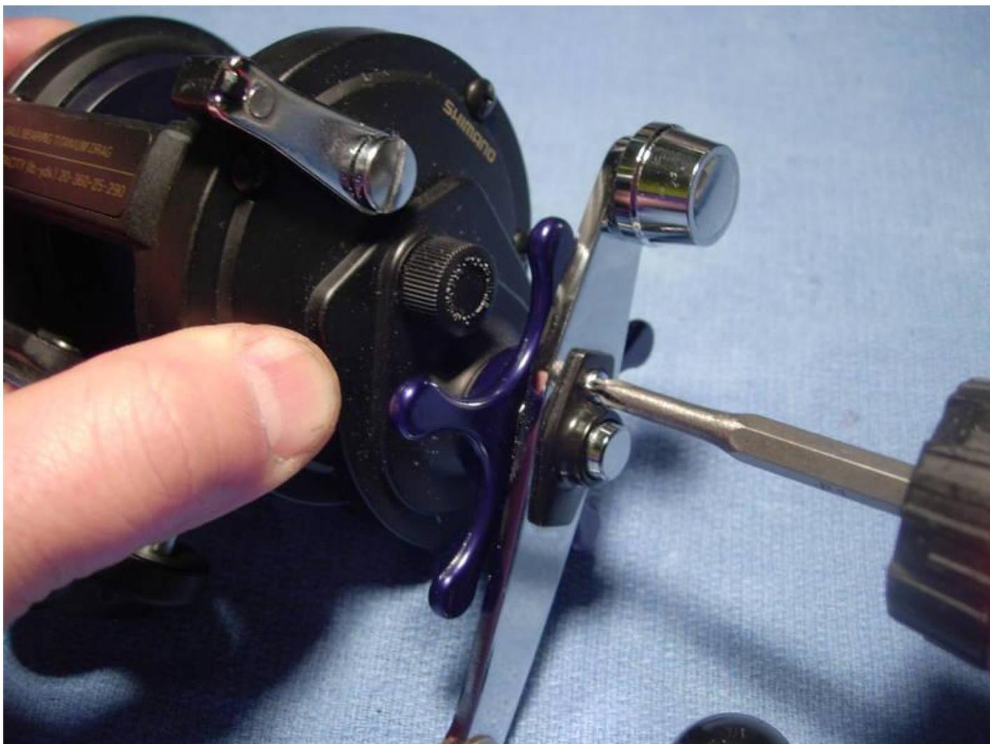
Remove the handle nut (key #129) with a 10mm wrench.
