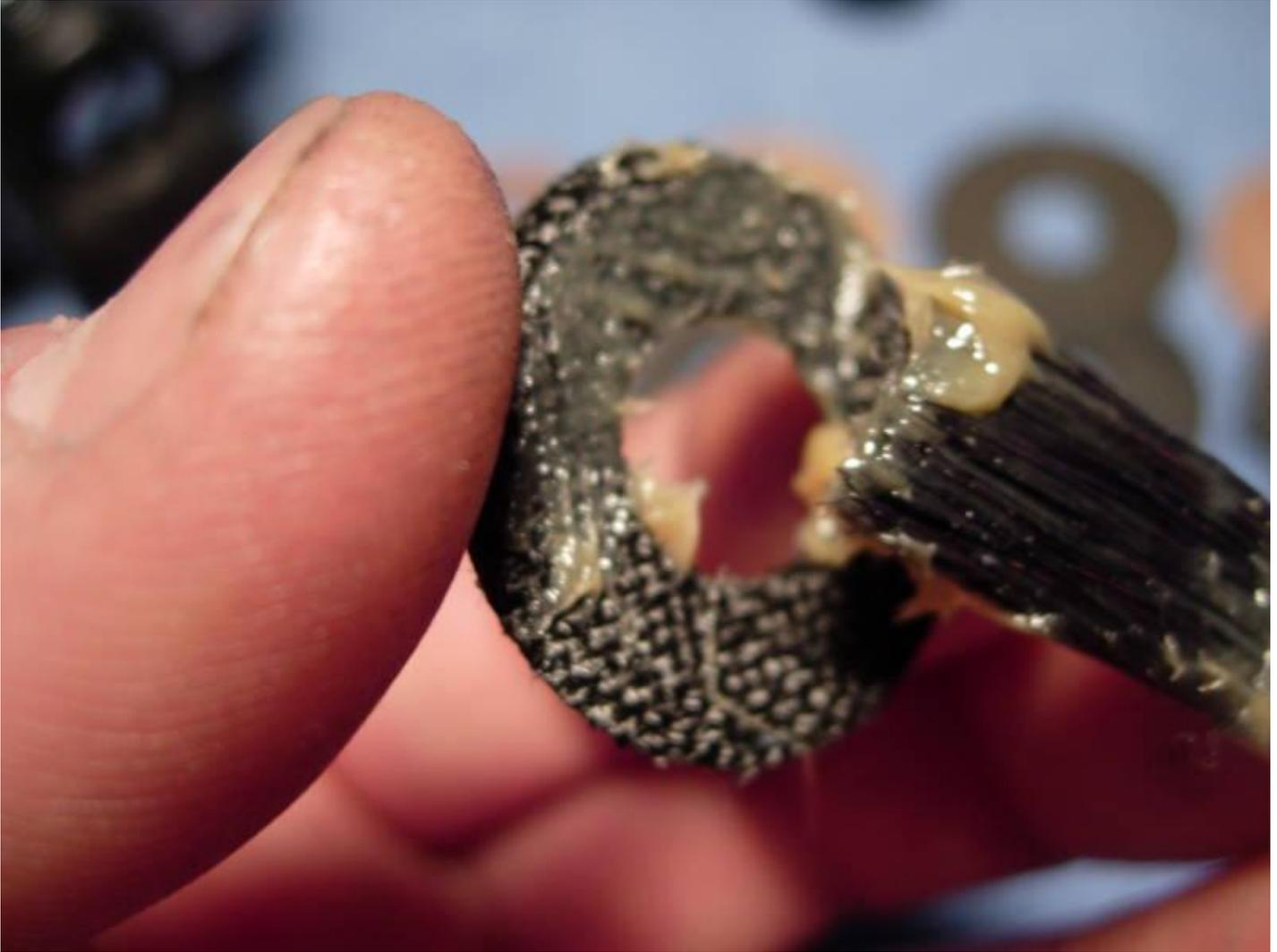
**Use an old toothbrush to apply a light coat of grease to the carbon fiber base-plate. Install the #6-309 drag washer and the drive gear (key #133).**
