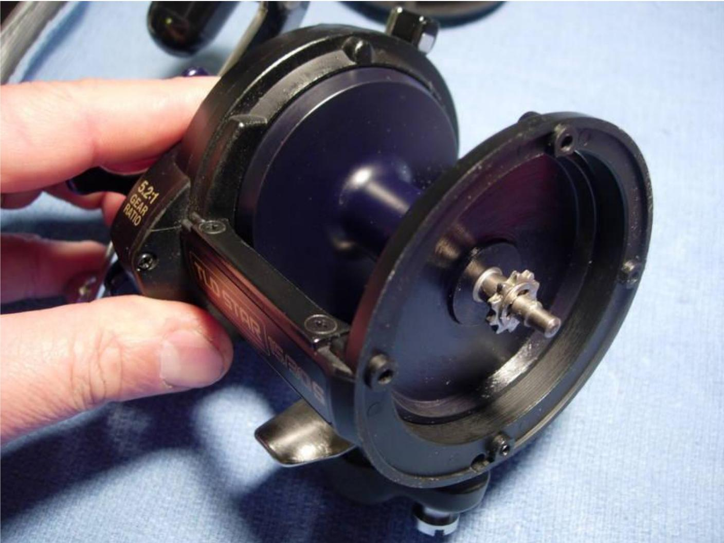
Install the left side plate assembly (key #211) and left side plate screws (key #114). These few steps are all that are required for routine maintenance of this reel.
