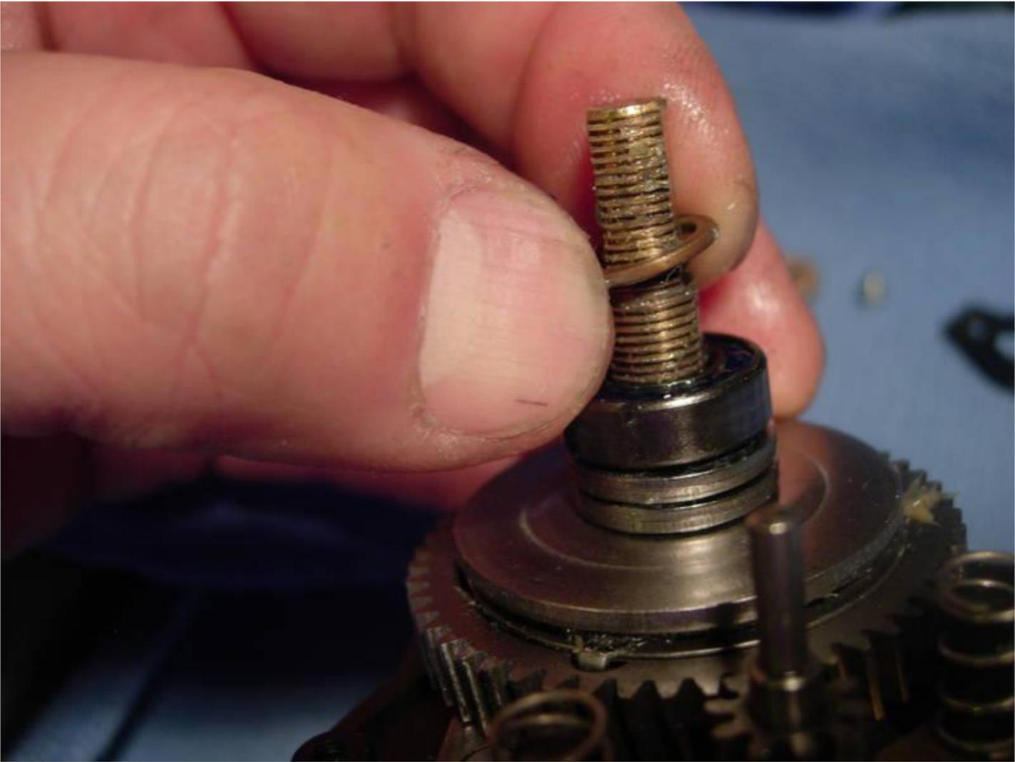
**Apply a light coat of grease to the inside of the right side plate assembly (key #209).**
