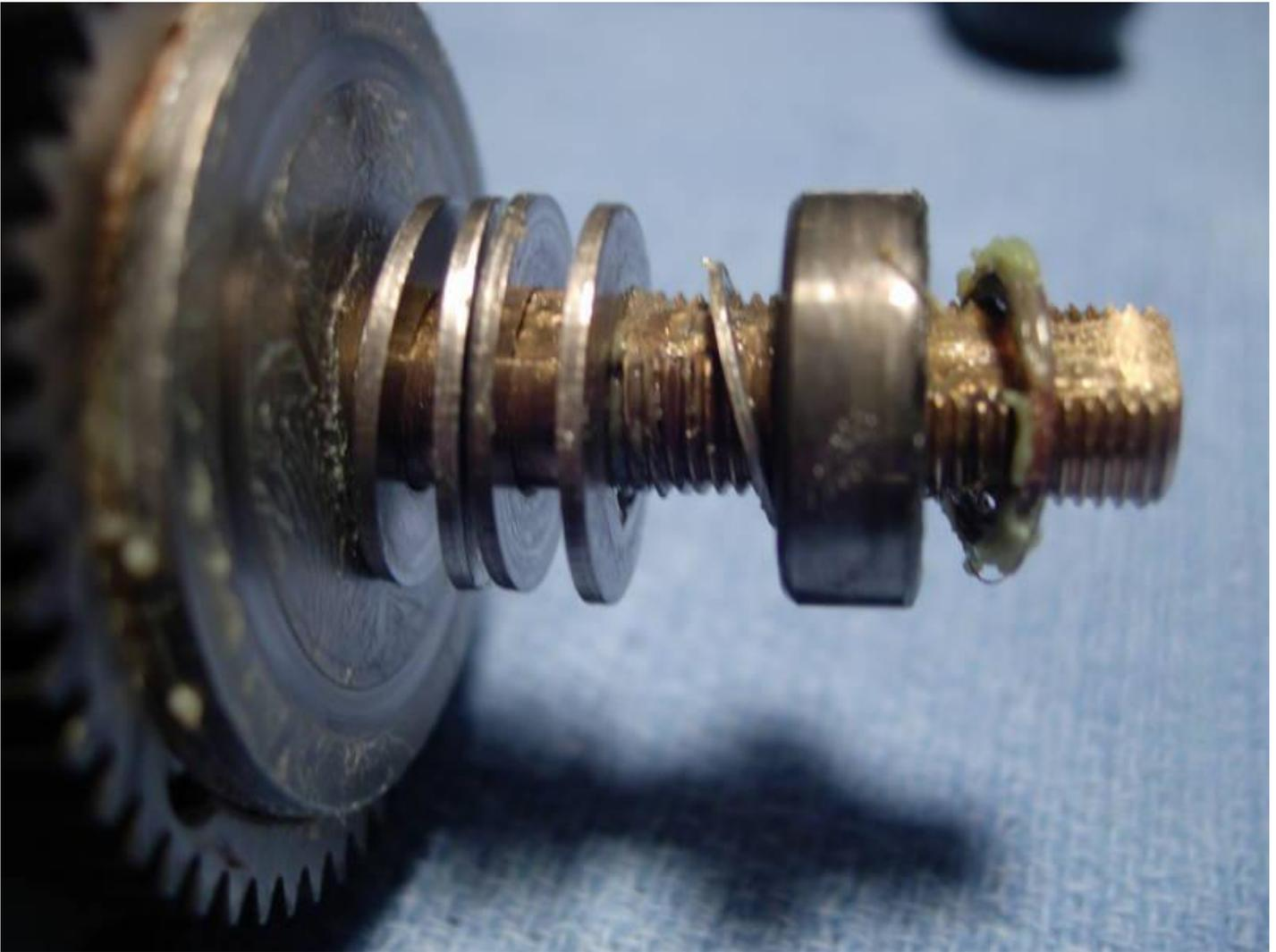
Now, carefully, remove the stainless steel and canvas drag washers, one at a time. I've cleaned them and lined them up for the photo. From left to right is the drive shaft washer (key #100), the drive gear (key #133), the eared washer "b" (key #98), key washer "c" (key #97), drag washer "i" (key #96), eared washer "e" (key #95), drag washer "d" (key #94), and key washer "f" (key #93).
