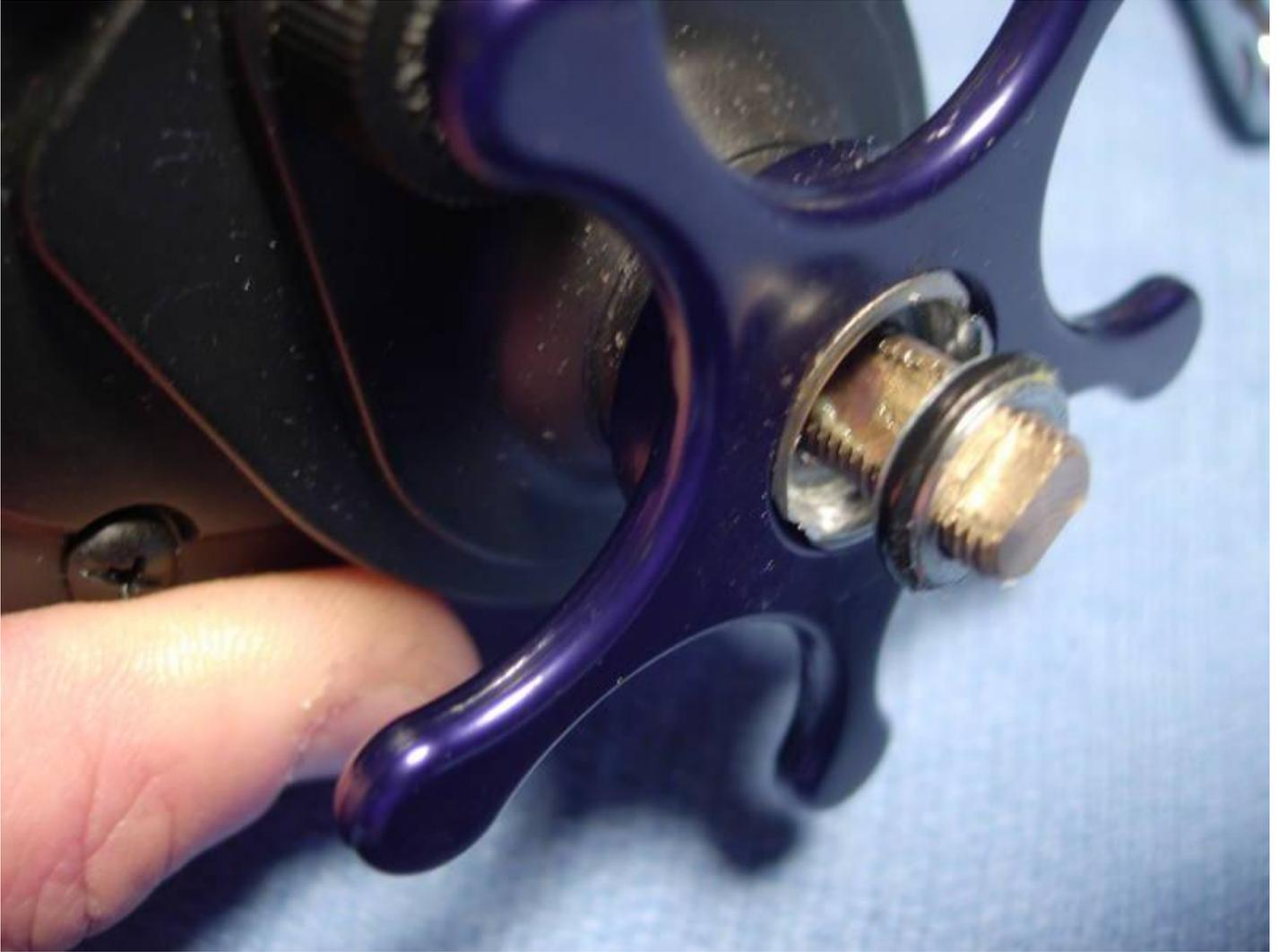
Remove the two right side plate screws "b" (key #109).
