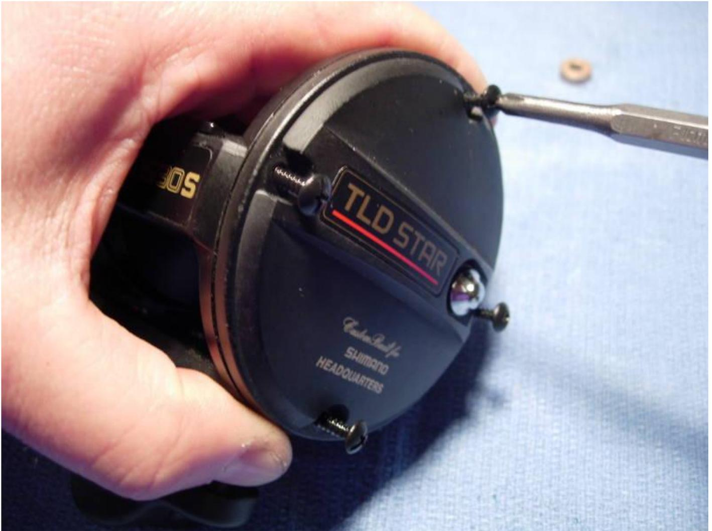
Now for the right side. Remove the handle nut plate screw (key #128) and handle nut plate (key #2).
