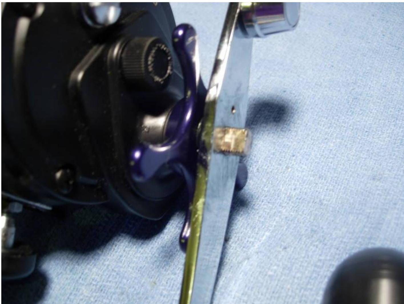
**Install and properly align the 10mm handle nut (key #129).**
