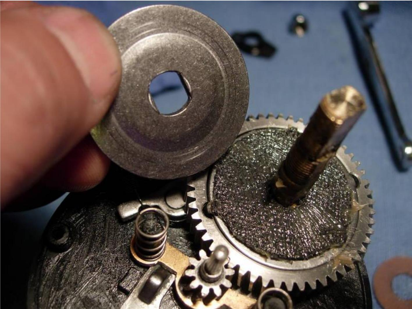
Install the drag spring washers (key #92) oriented "()
