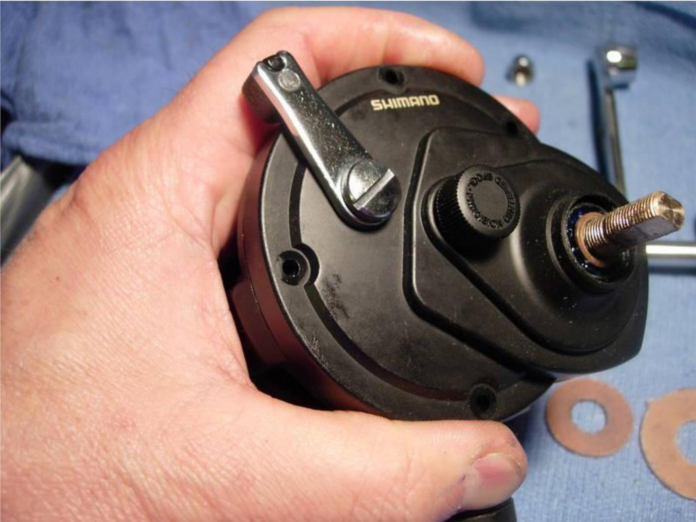
**Install the four right side plate screws "a" (key #81).**
