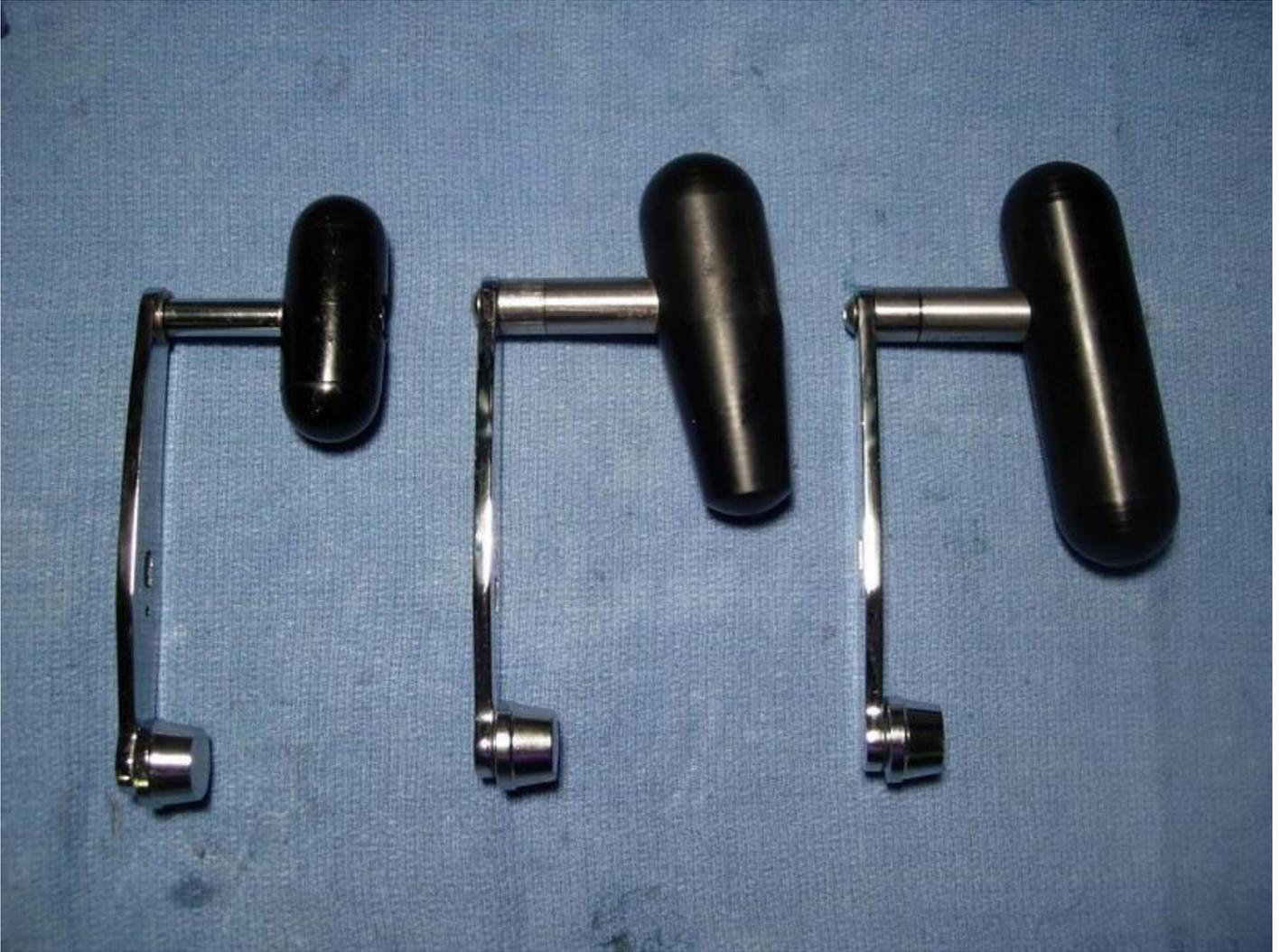
**Install the star drag (key #79), the handle washer (key #78), and the new handle (key #414L). Put a little grease on the handle arm around the drive shaft.**
