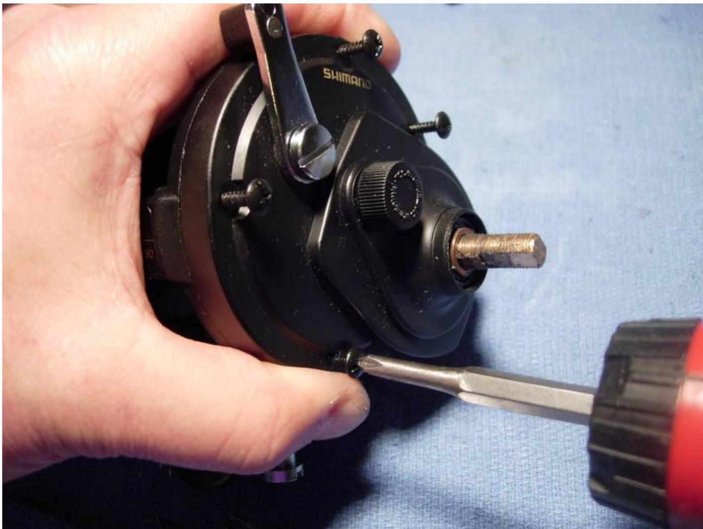
Install the two right side plate screws "b" (key #109).
