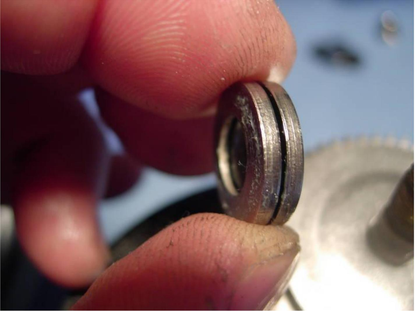
**Install the bearing thrust washer (key #91).**
