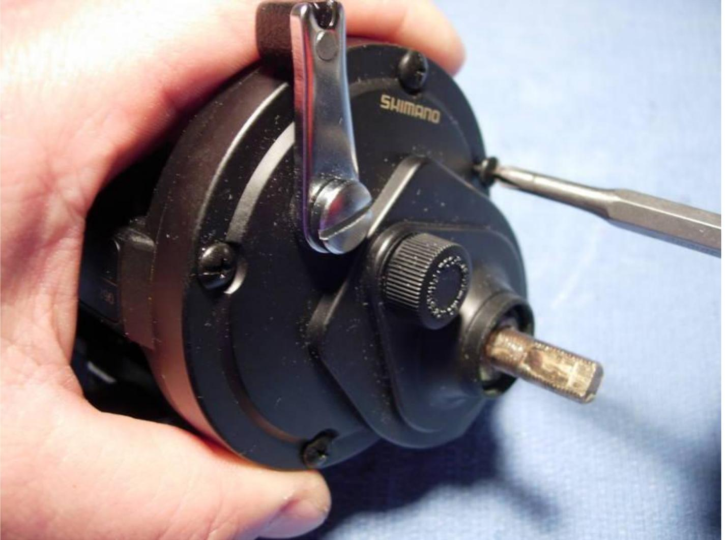
Remove the right side plate assembly (key #209).
