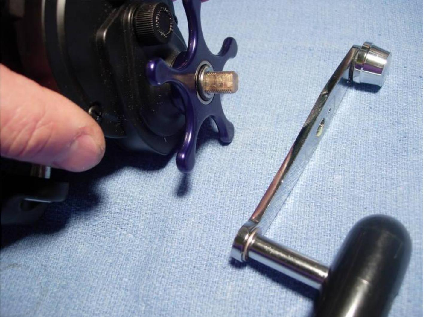
**Remove the handle washer (key #78) and star (key #79).**
