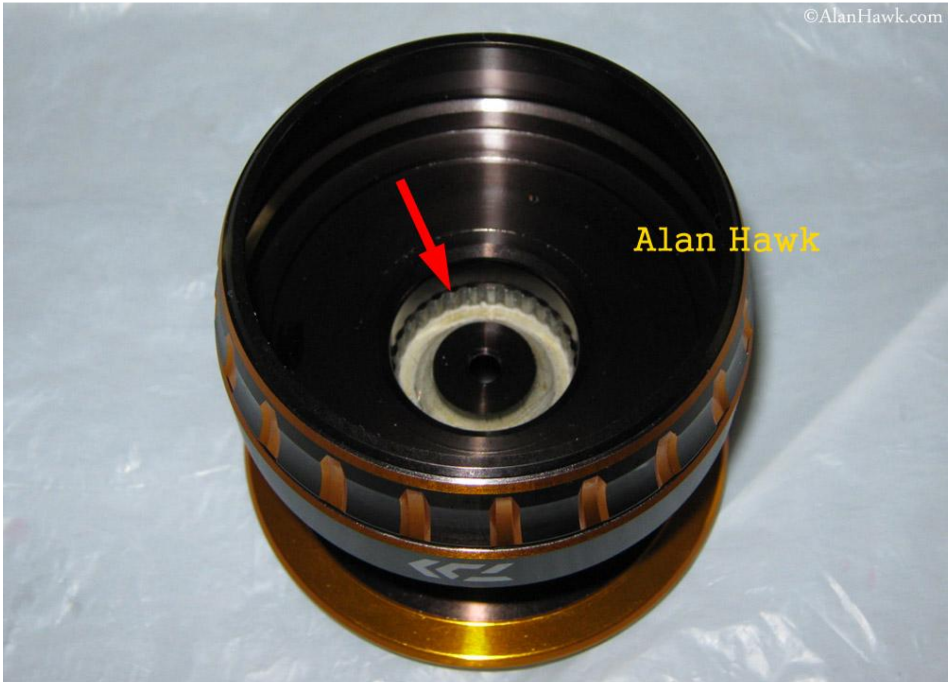
Behind the spool the drag clicker grooves are the familiar design found in Daiwa's top saltwater and freshwater reels.
