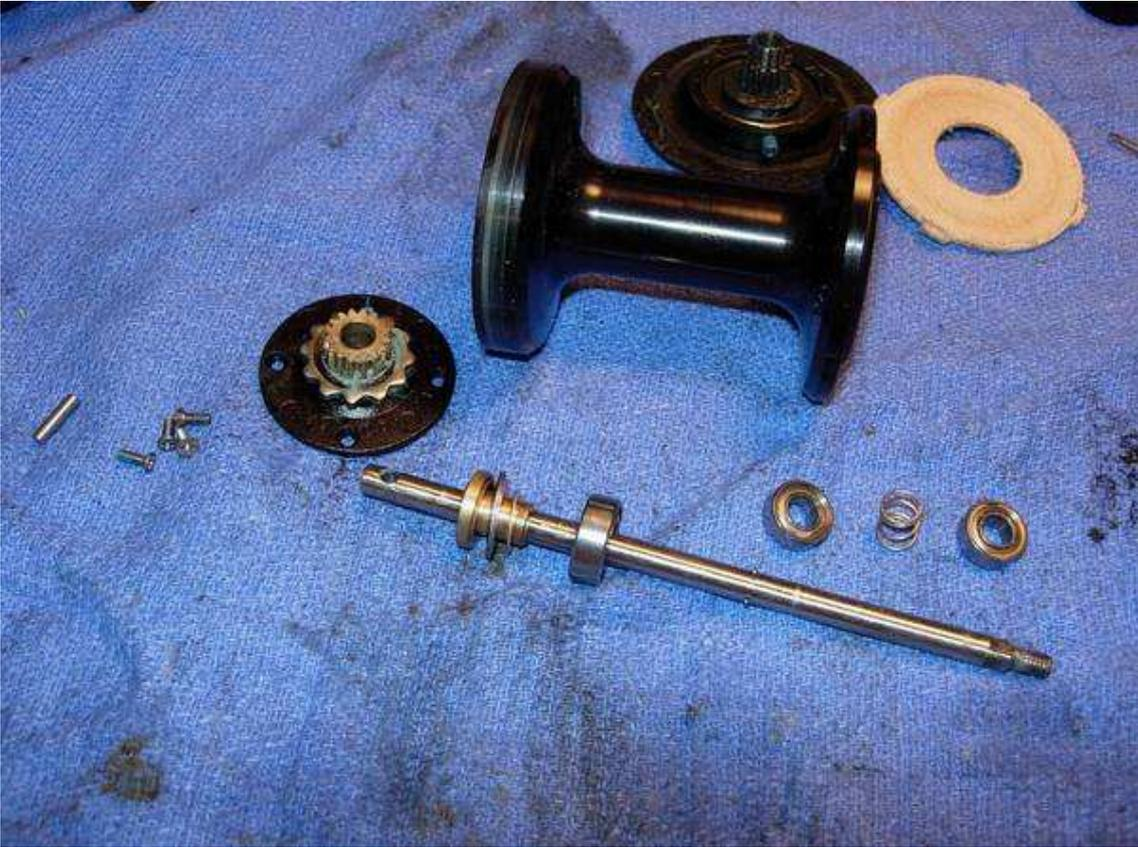
the shields of the three spool bearings can be removed and you can see the dried grease inside.
