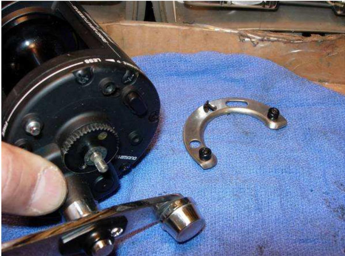
back out the five side plate screws (key #122) and remove the right side plate as a unit.
