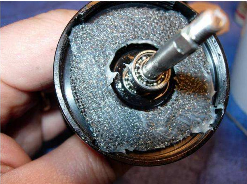
wipe off all the excess drag grease until drag washer basically looks dry.
