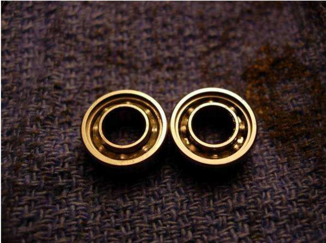
after cleaning out the grease with carb cleaner and compressed air, the bearings can be lubed with corrosion x or reel x.
