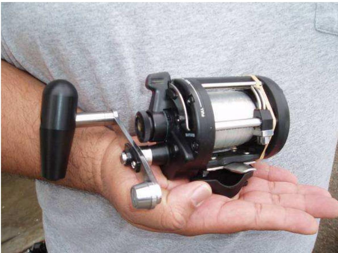
the spools of both reels will now spin easily. both of these reels have only 5 seconds of freespool, but that is because of levelwind mechanism. without the levelwind assembly, the spools probably would spin for 30 seconds. both now have a max drag at strike of 15 pounds before losing freespool. and both have a smooth drag from 1 pound up to 15 pounds. the total time required for service, including time to clean out the bearings, was an hour.
