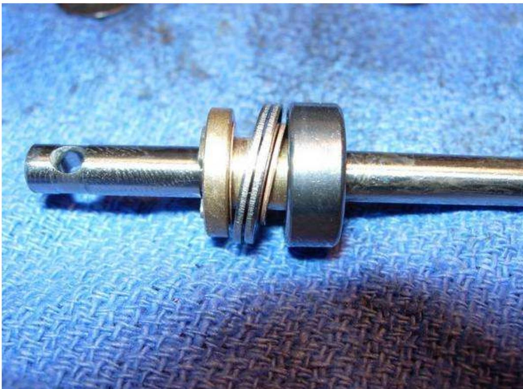
those of you that prefer a dry drag can either re-install a new canvas washer (part #tld-0129) or use a the penn ht-100 without grease. my preference remains to grease this washer using shimano or cal's drag grease, applying a thick coat to both sides of the drag washer.
