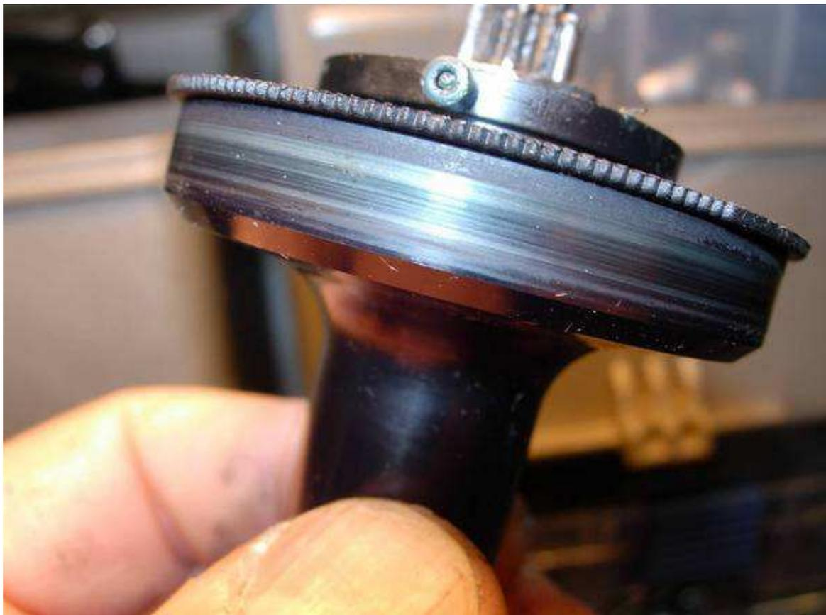
it is a common problem for these graphite frames to "swell." i use a dremel and the cutting bit #117 to cut away at the inside of the graphite frame, just enough so that the spool doesn't rub.
