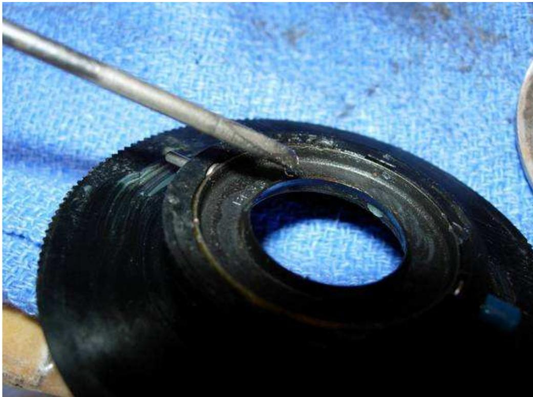
and the metal lip on the drag pressure plate assembly.
