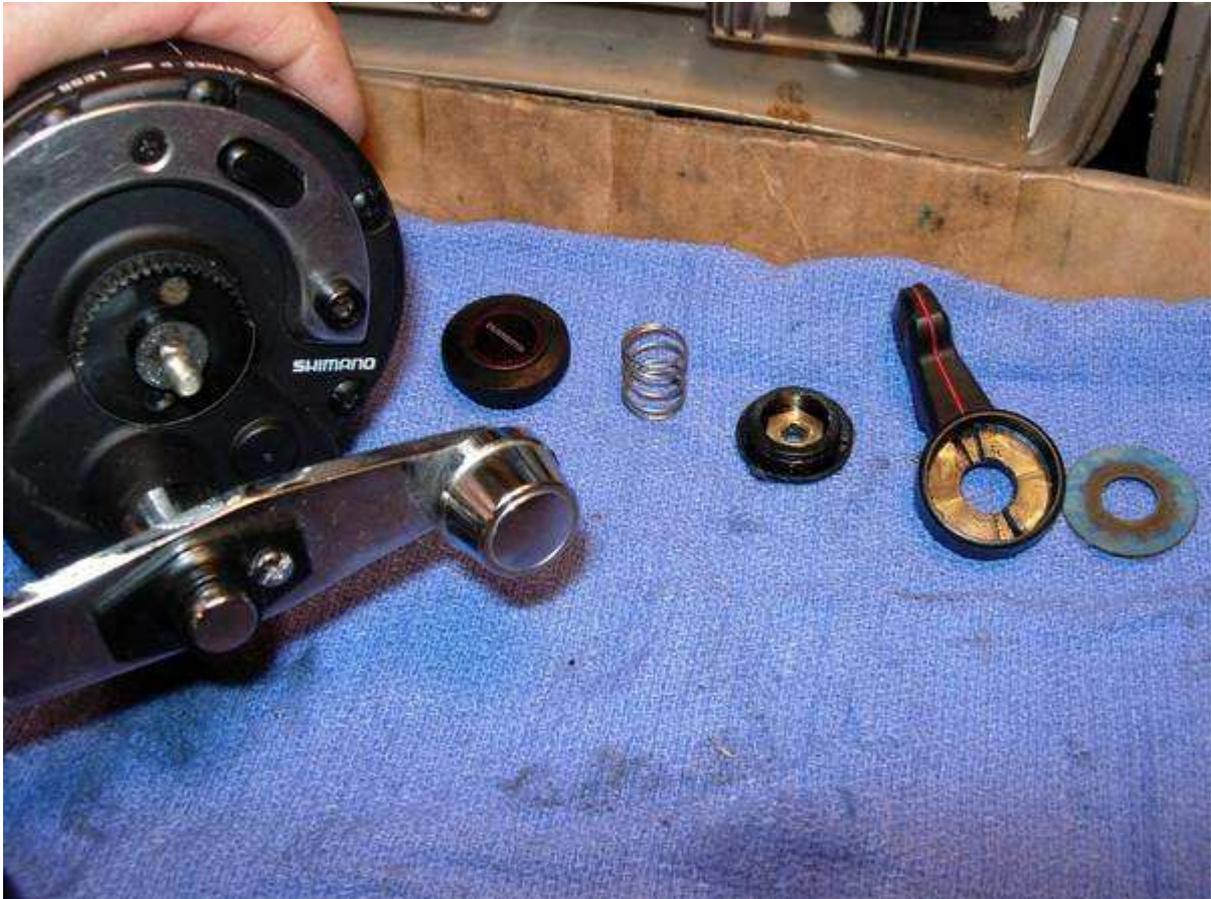
remove the lever quadrant (key #121) and screws (keys #19, 20 and 21).
