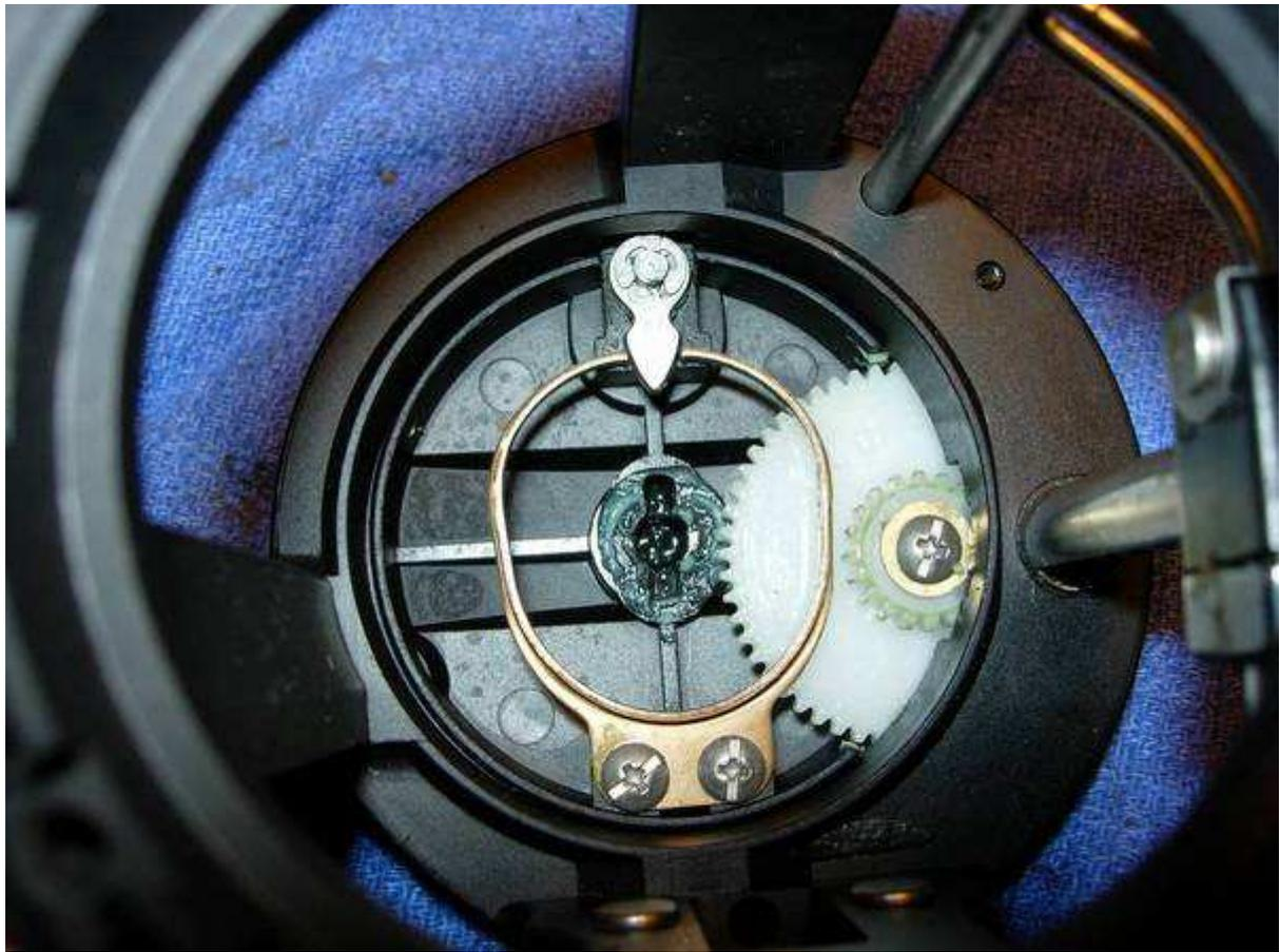
remove the spool cap and drag pressure plate as a unit. note the reverse threads.
