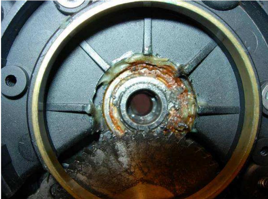
remove the handle lock screw (key #1), the handle lock (key #2), the handle nut (key #3), the gear shaft shield (key #5), the gear shaft thrust washer (key #6) and the main gear (key #8). the dog (key #26) and the brake collar (key #190) will fall out as well.
