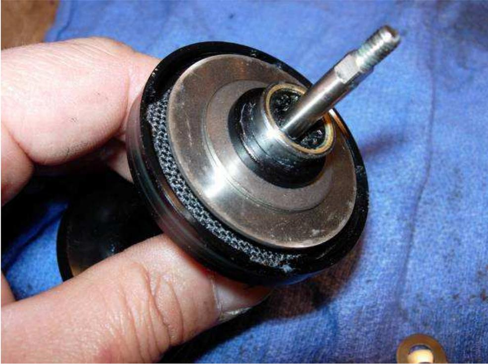
install the spool cap and pinion gear.
