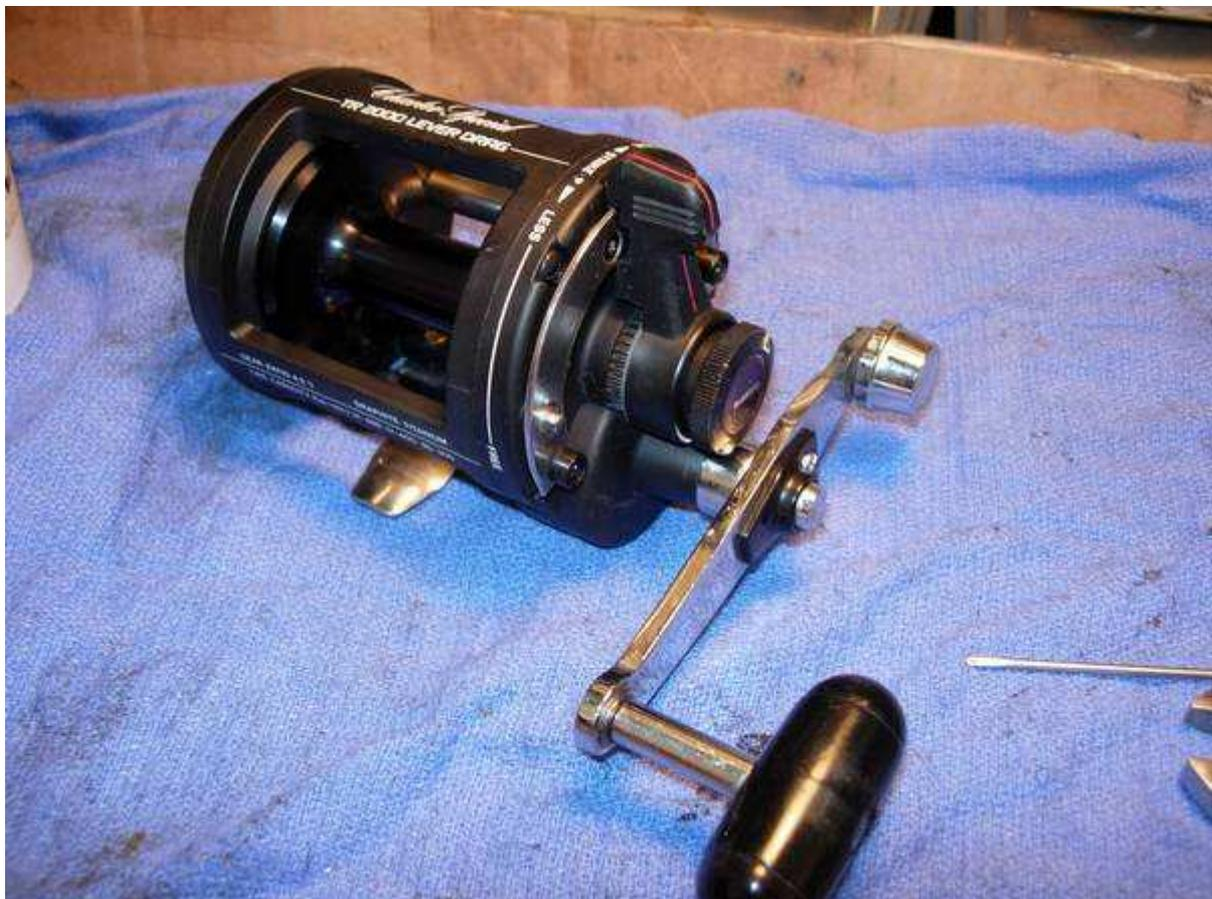
the first thing to come off is the lever assembly, including the pre-program dial (key #115), the dial spring (key #82), the lever shaft body and "O" seal (keys #116 and 10), the drag control lever (key #117) and the lever thrust ring (key #84).
