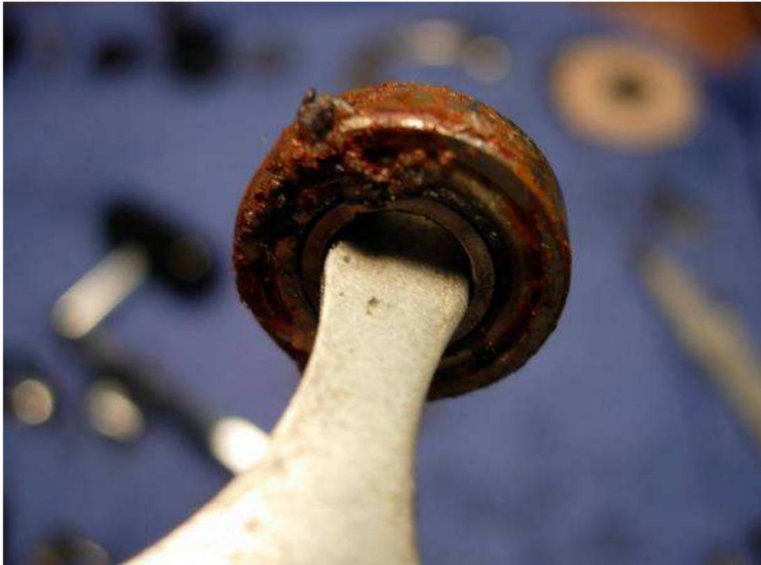
the old bearing was too badly rusted, so i pulled out a new one....
