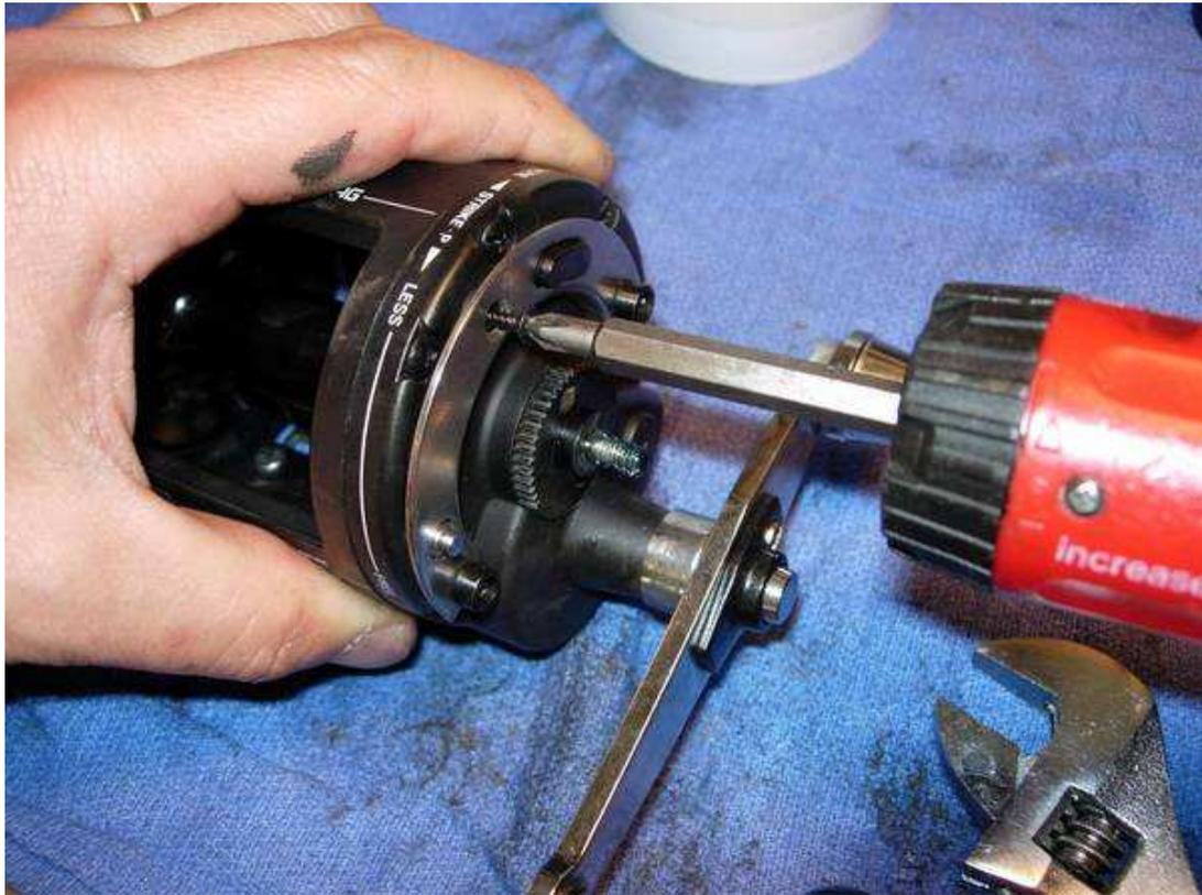
install the lever and pre-set dial. make sure the lever is in the free position and drop the lever shaft body into the lever so that they mate up.
