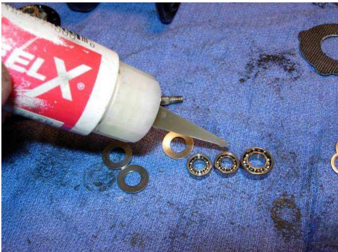
switching out thin pre-load washers (bellevilles) for thicker ones will ramp up the drag pressure more quickly and give you a higher drag at strike before you lose freespool. the thin preload washer B's (key #44) on the right will be switched out for the thicker preload washers from the shimano tld 20/30 two speed reels (part # tt-0040A). the orientation of these belleville pressure washers remains "()".
