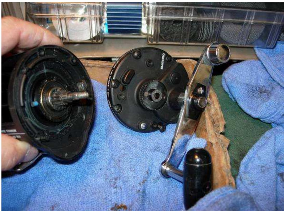
remove the spool assembly as a unit.
