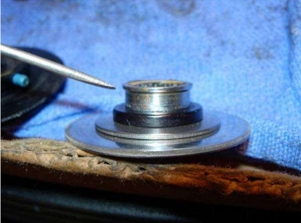
when the drag lever is at strike and the reel is engaged, this metal lip mates up with the rubber gasket and seals up the drag chamber to keep water out. the take home message is this. rinsed off your shimano lever drag reels in the "strike" position. all other lever drag reels should be rinsed in "free."
