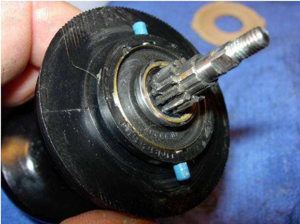
install cross pin B (key #50) and place the spool assembly back into the frame. the spool should slide easily back into the frame.
