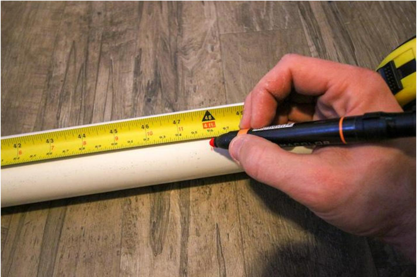
Cut your 4" PVC pipe to 18" inches (foot and a half) in length, and your 2" PVC pipe to four feet. Take care to ensure your cuts are clean and square so that the fittings will seat flush to the end of the pipe. If you have lots of extra frayed bits of PVC after your cut, use some sandpaper to smooth them out. You can also often get your pipes pre-cut at hardware stores.
