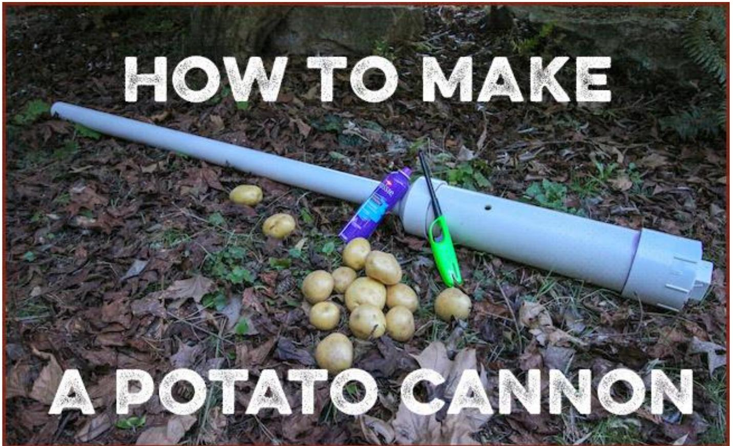
Made out of a few simple PVC fittings and lengths of pipe, potato cannons can launch spuds up to 300 yards. They're cheap and fun to make, and they're also a great way to get introduced to the basics of cutting, priming, and gluing PVC together. If you've been hesitant about DIY plumbing, making a potato cannon is a pretty low-risk intro course.
