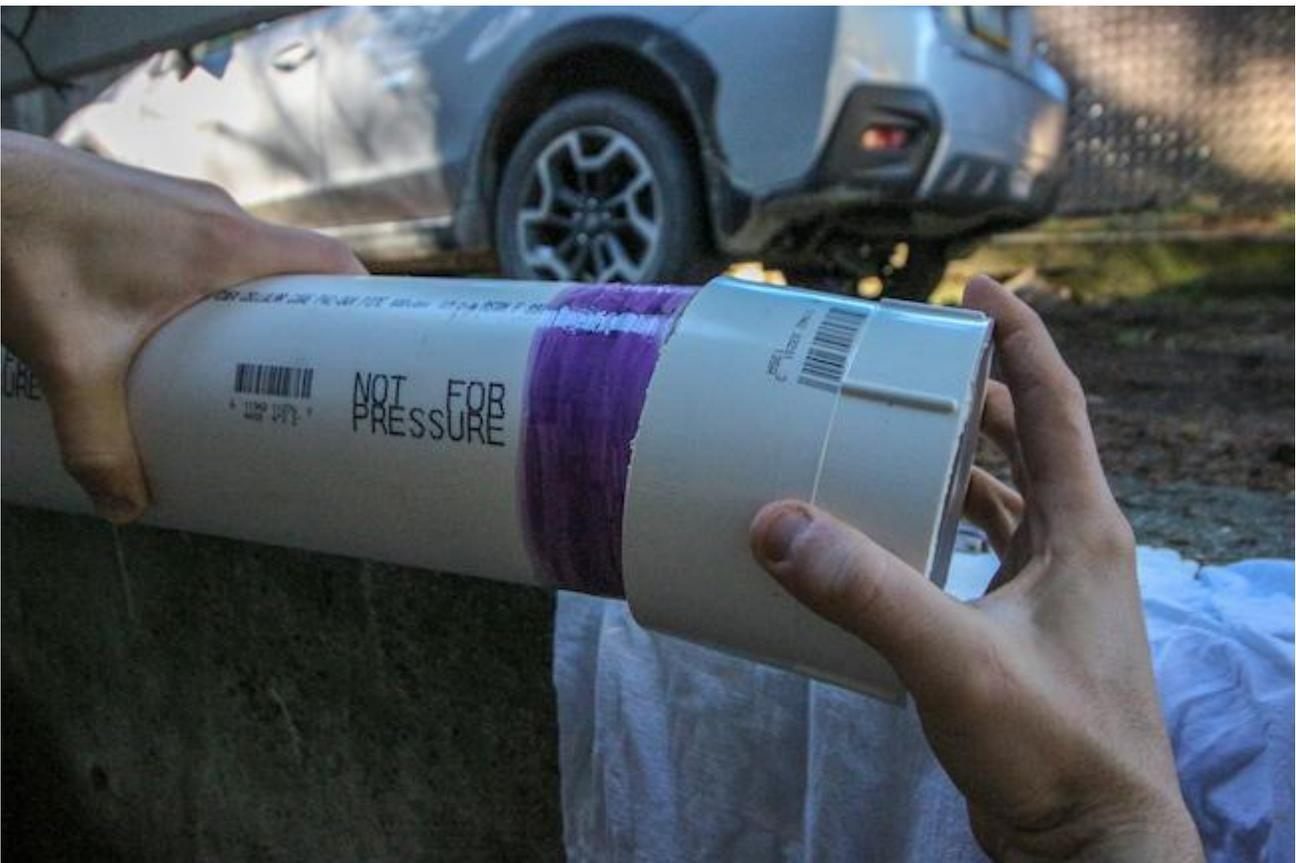
Attach the 4" threaded coupler onto the other end of your 4" pipe, and attach your 2" PVC pipe to the adapter to complete your barrel.
