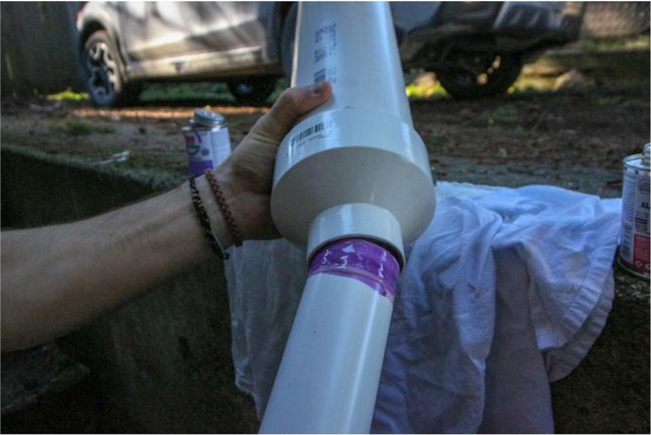
**Step 4: Screw on the 4" cleanout cap to the end of your combustion chamber.**
