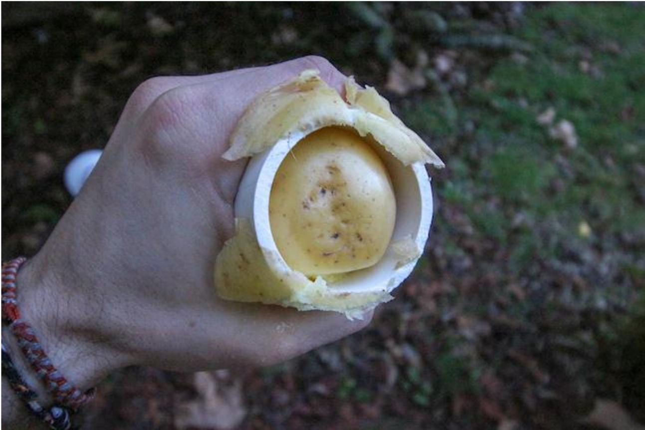
Use a broomstick or smaller diameter piece of PVC to jam it down into the barrel, like a muzzleloader. You do want the potato to fit fairly tightly; if loose, it will probably still launch, just with far less gusto.
