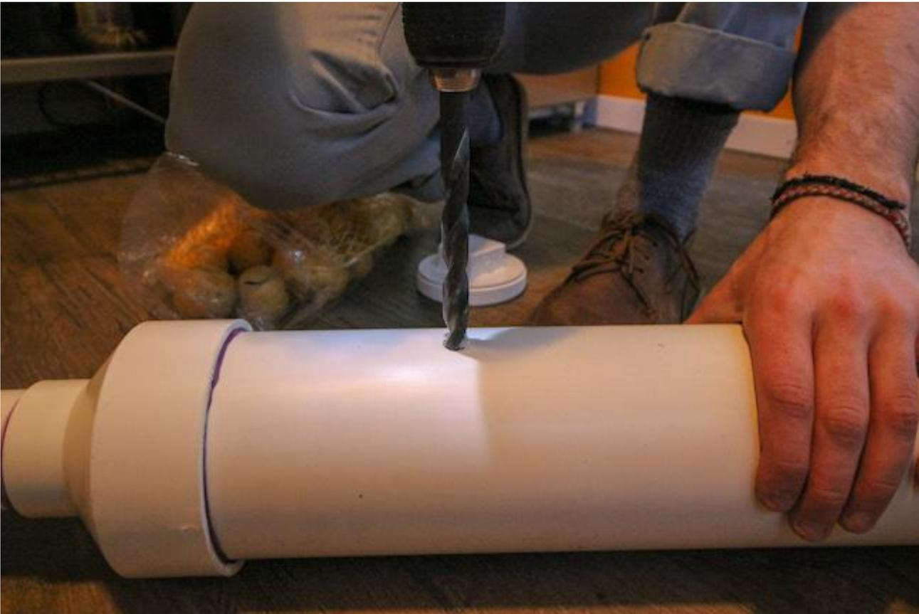
The placement of the hole doesn't really matter. Somewhere in the middle third or so of the chamber works just fine.
