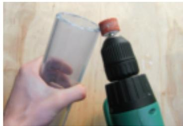
When PVC gets hot, it releases poisonous chlorine gas. Perform this step in a well-ventilated area.
