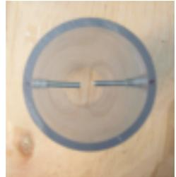
This is the spark gap that will ignite the fuel, firing the cannon.
