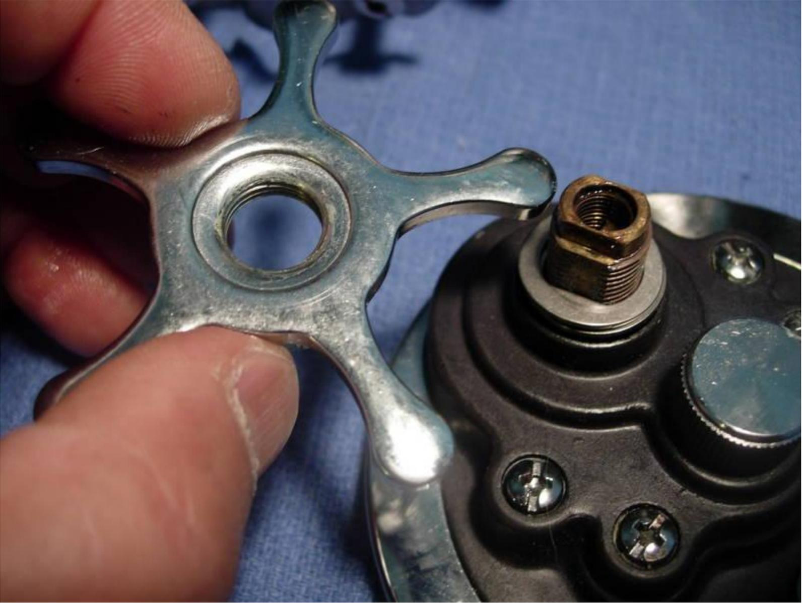
remove the tension springs (key #56). note that they are cupped "()".
