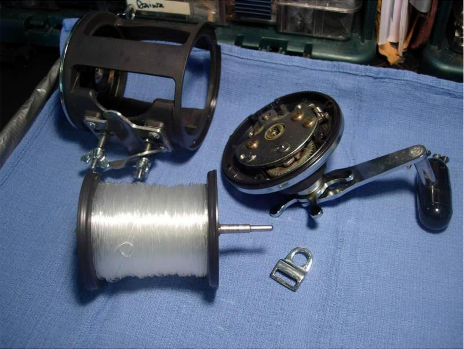
aluminum frames tend to corrode. take an old toothbrush and spread the old grease around a little, then wipe off all the excess.
