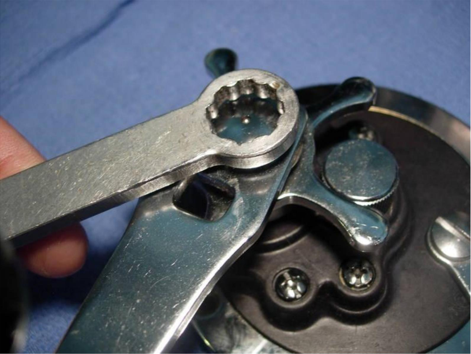
remove the handle (key #59) and handle washer (key #58).
