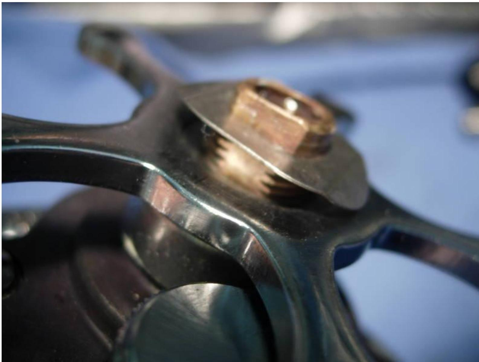
at this point, we're going to install a new handle grip. I'll drill out the back of the rivet for the old grip, then remove the grip and throw it away. I'll need the arm only.
