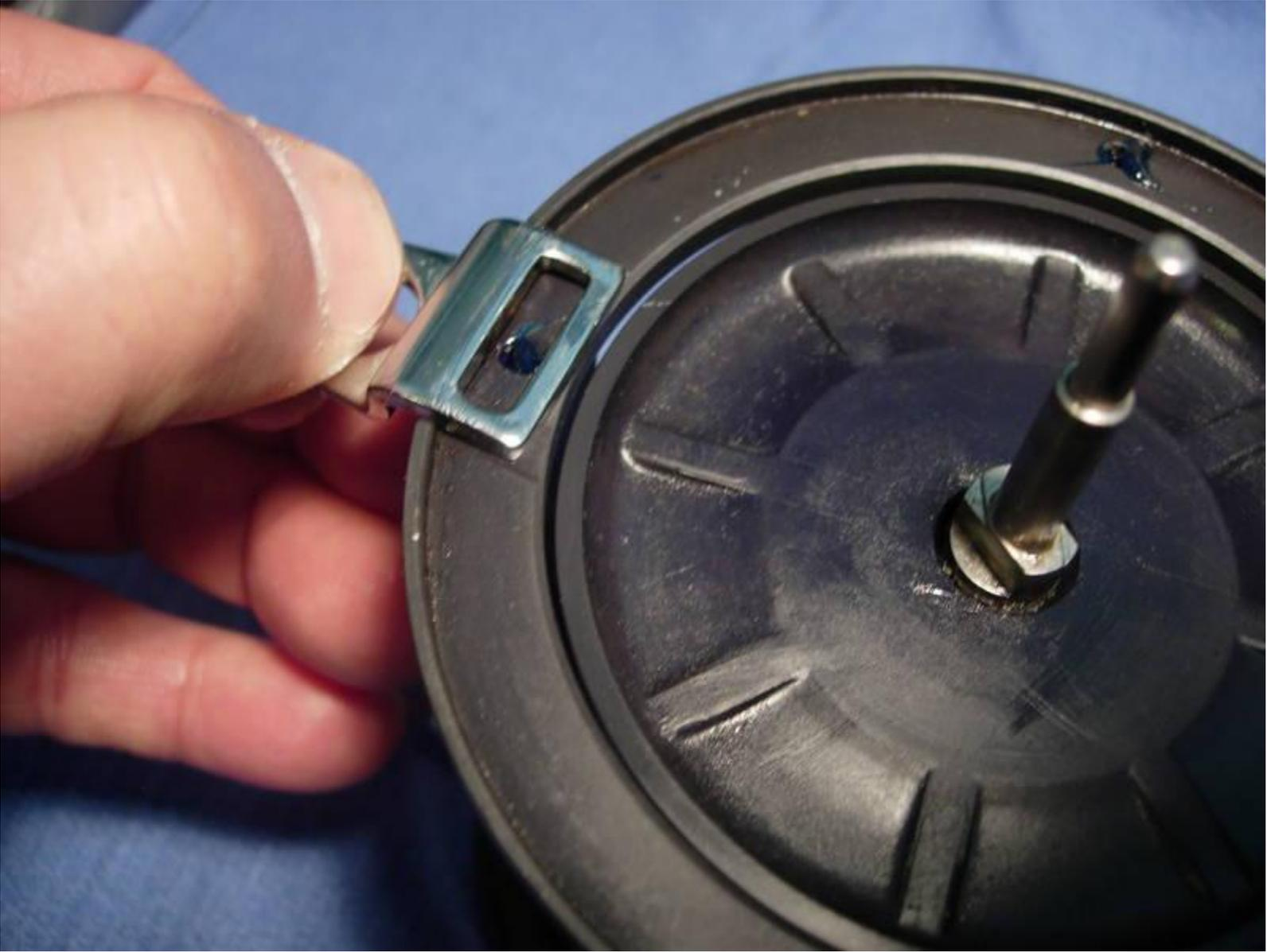
install the right side plate assembly (key #36).
