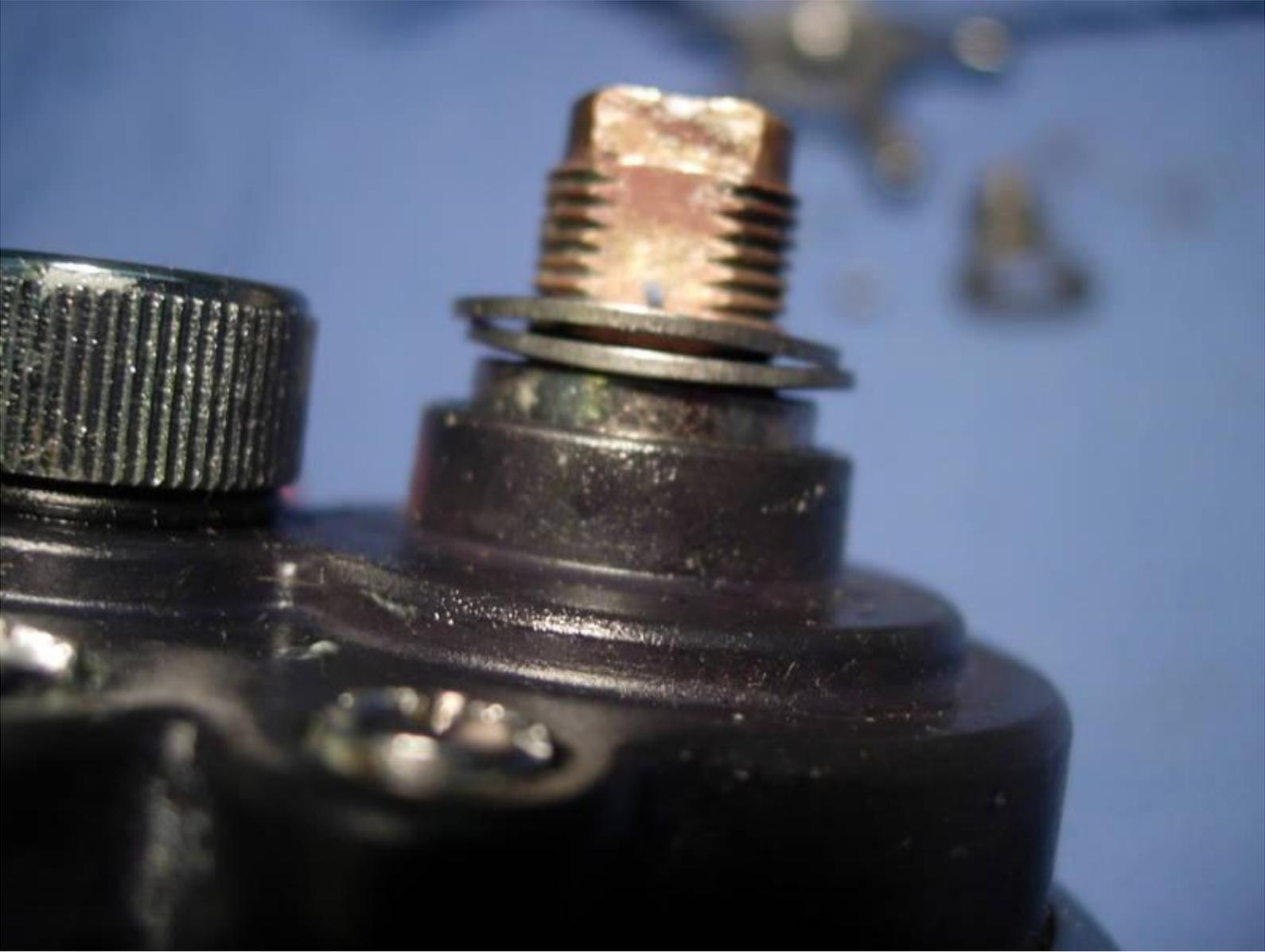
install the star drag (key #57). turn it down until it won't turn any more. you should be clear of the shoulder of the set plate drive shaft and still be able to turn the star without banging into the spool adjusting cap (key #46).
