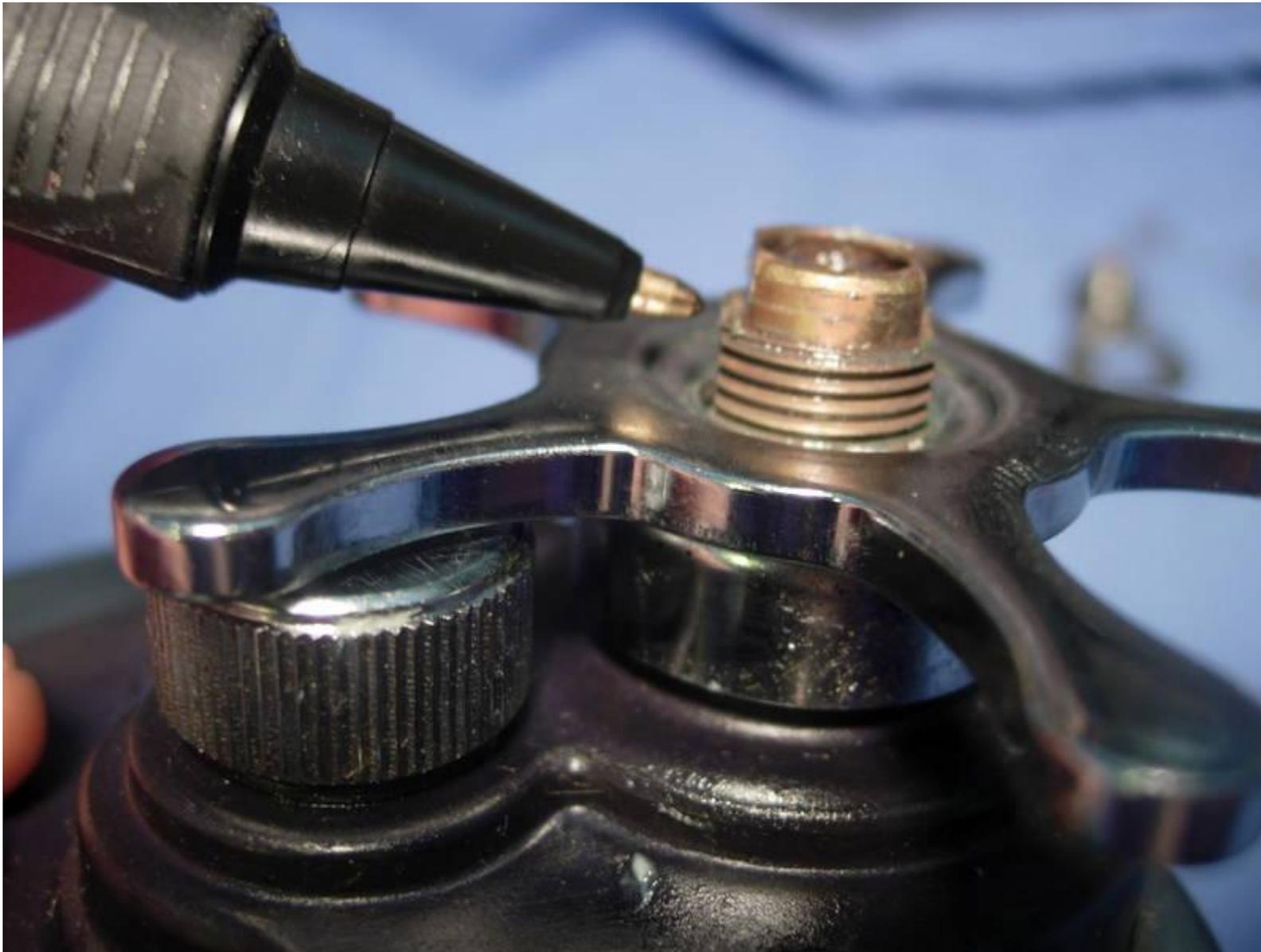
install the handle washer (key #58).
