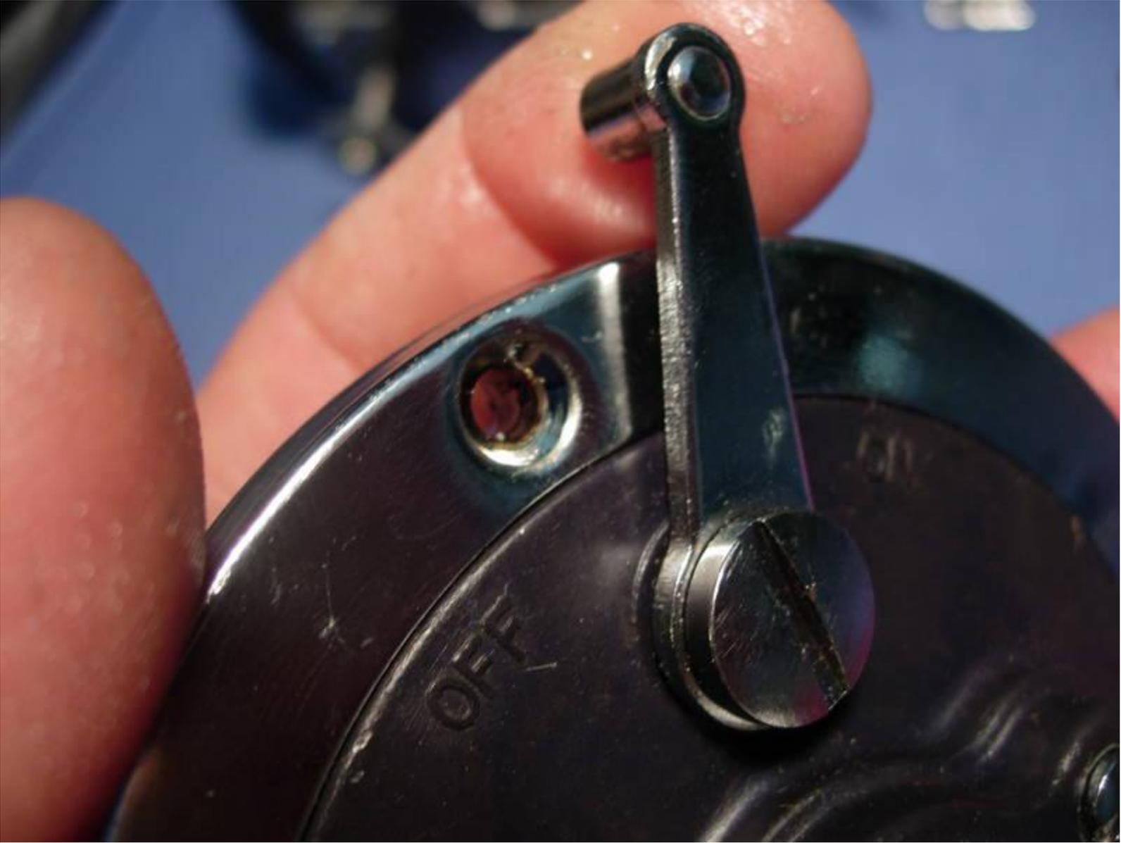
grease the screw holes on the right side of the frame (key #16).
