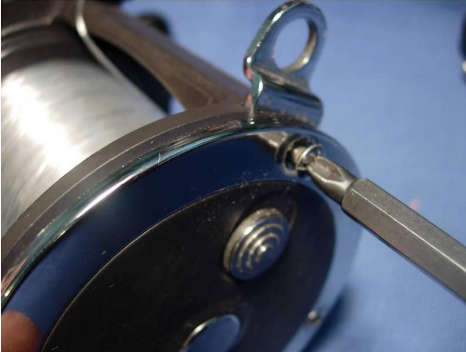
now back out the three right side plate screw A's (key #48) and two right side plate screw B's (key #49).
