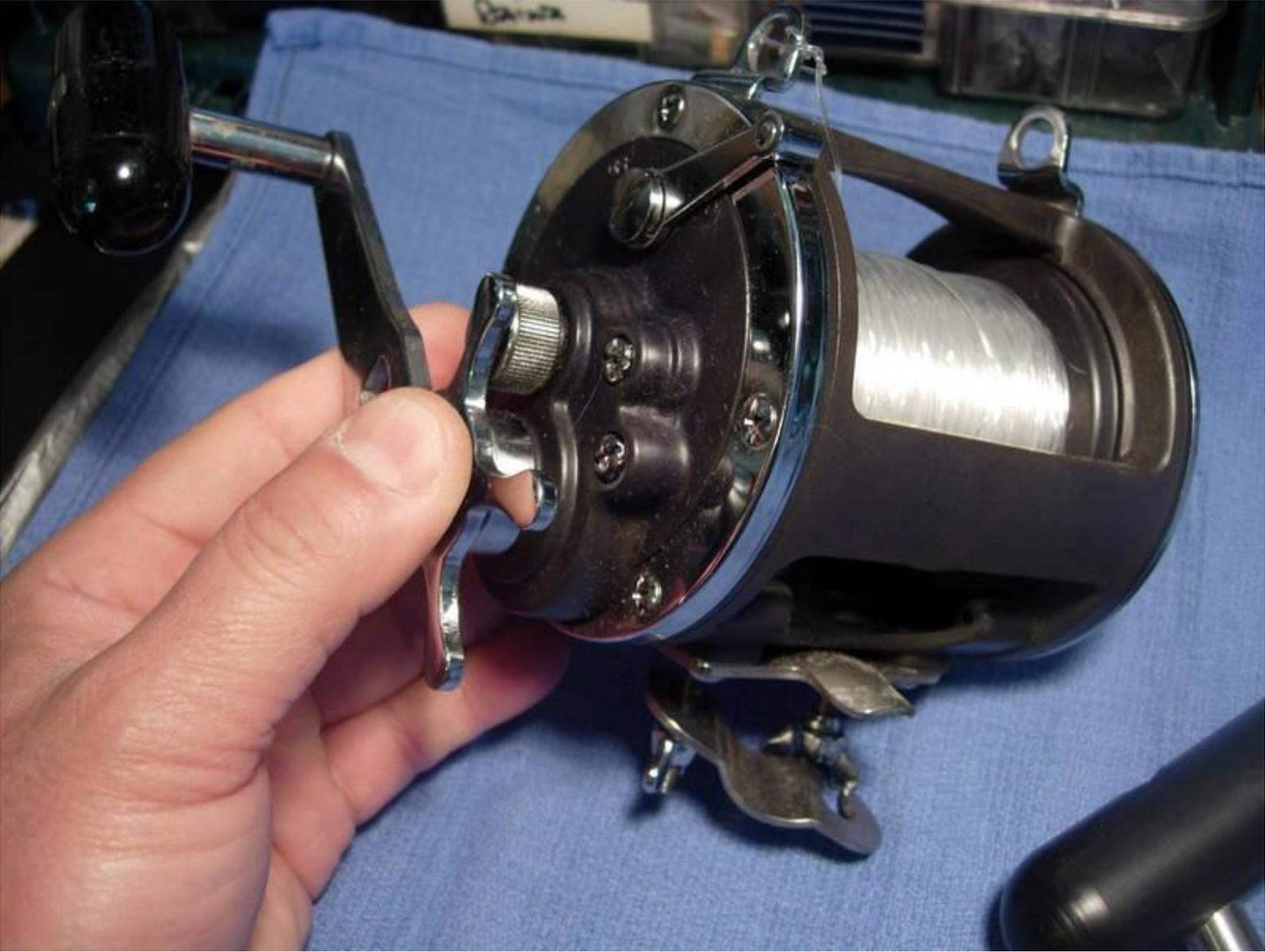
let's start with the left side plate. back out the three left side plate screw A's (key #2) and the two left side side plate screw B's (key #3) one at a time, grease the screw holes and re-install the screws.
