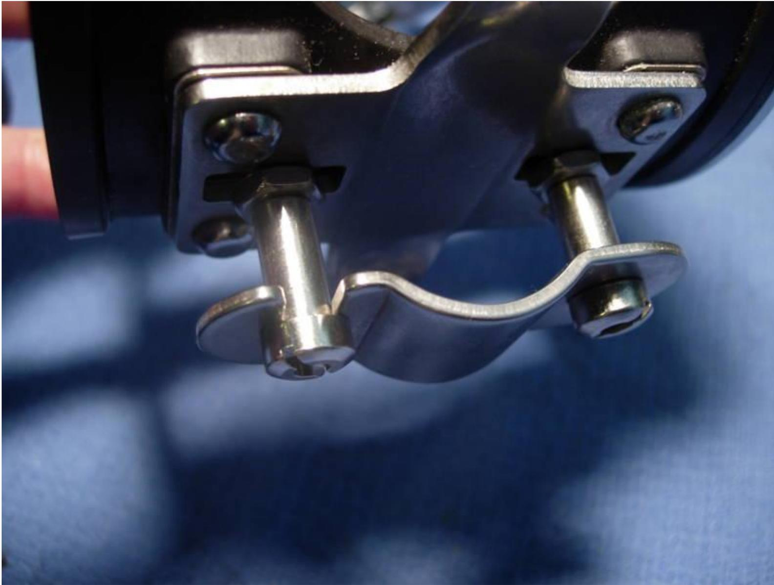
install the spool (key #24) into the frame assembly (key #16) and set both aside.
