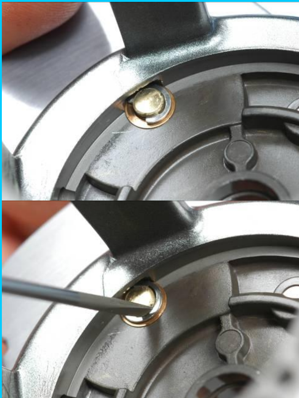
Step 8: Removal of drive shaft retainer clip for Torium reels The drive shaft retainer clip is located on the frame and is exposed when the spool assembly is removed.
