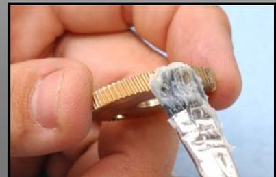
Use Shimano® Drag Grease to lubricate drive gear. Fill the threads half way around with grease.
