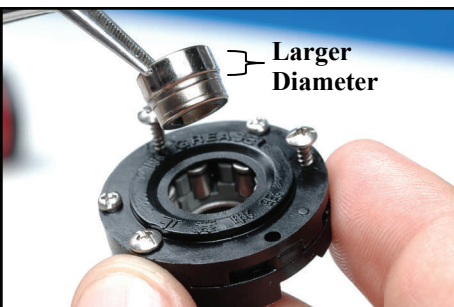
Make sure that the roller clutch sleeve is positioned with the larger diameter area towards the top of the roller clutch assembly as shown above.
