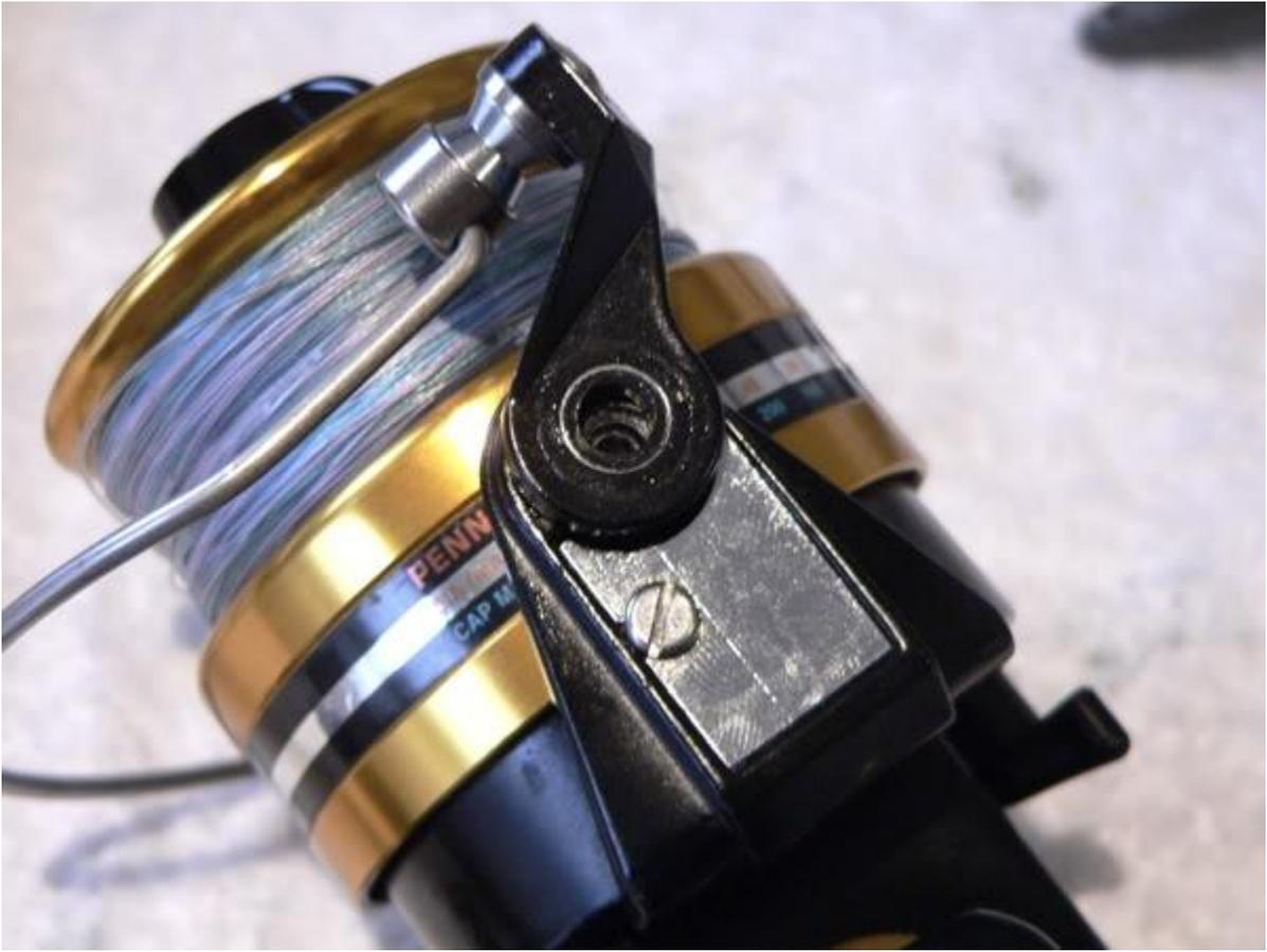
**You'll need to carefully apply pressure while holding the assembly, to align the holes so that the bail arm screw can be replaced.**
