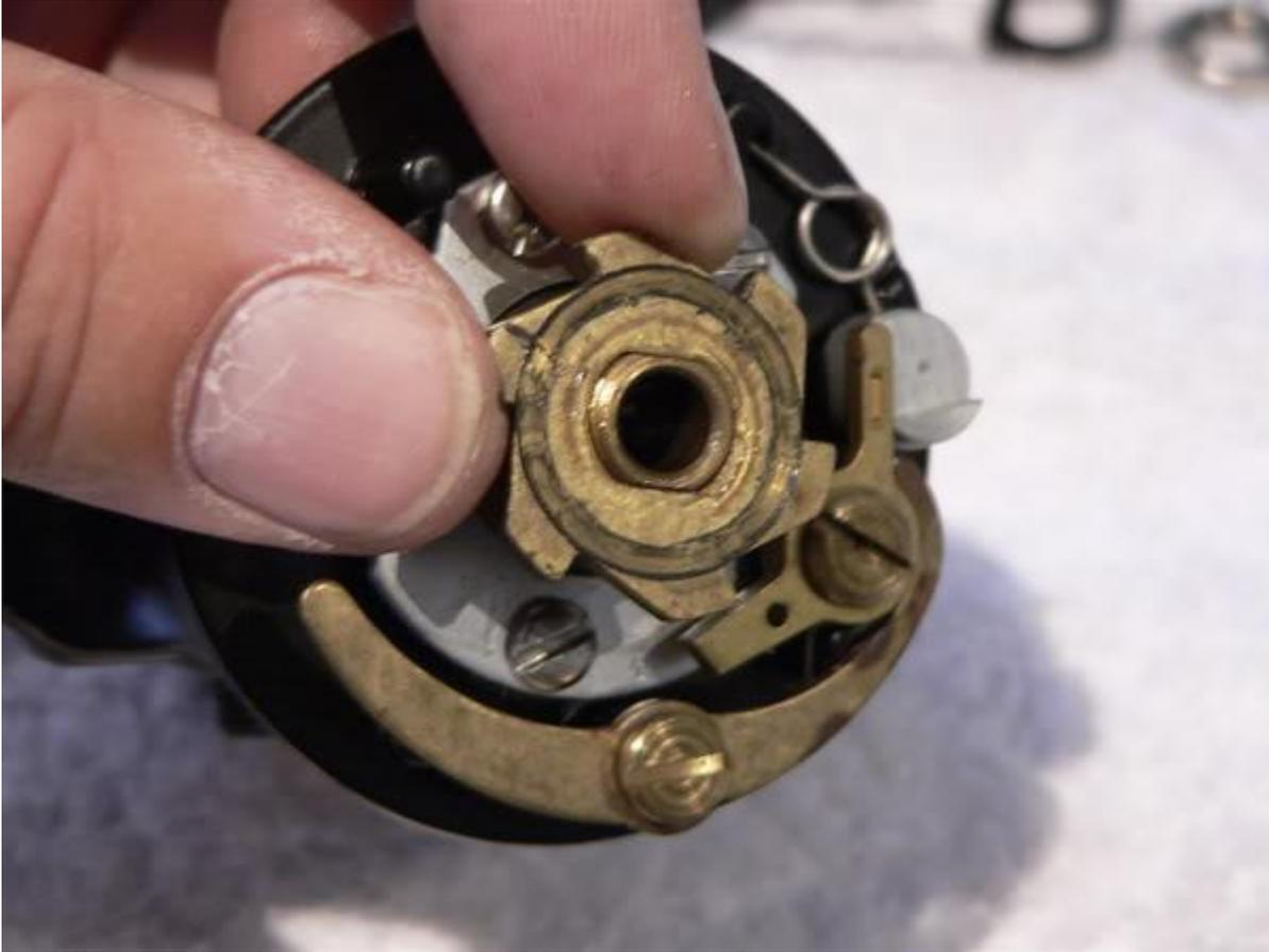
The long transfer lever (key #224) can be unscrewed and removed and now you'll be able to access the bearing retaining plate (key #21), which can be unscrewed and removed. (There's no need to remove the remaining ratchet dog (key #4) this time so lets leave those springs and things alone... no need to tempt fate)
