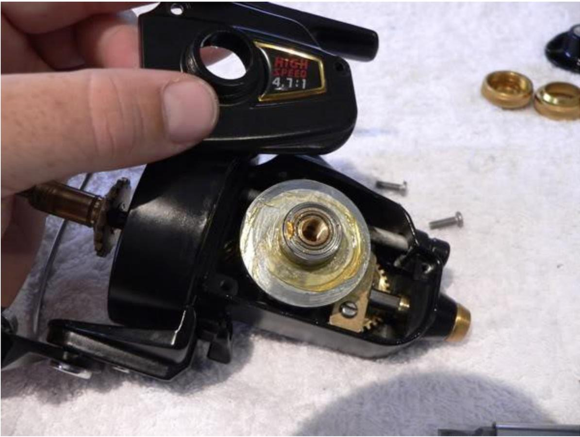
Remove the left side bearing (key #20A), open it up by removing the retaining clip from the shields using the 'Alan Tani' approved fish hook method 🐟
