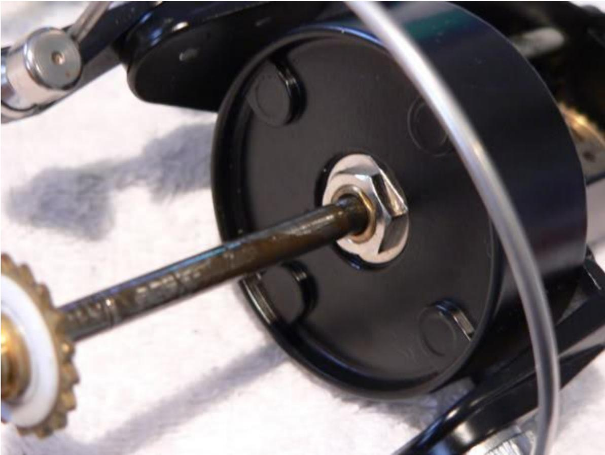
Take out the oscillating slider and the oscillating gear (key #231) beneath
