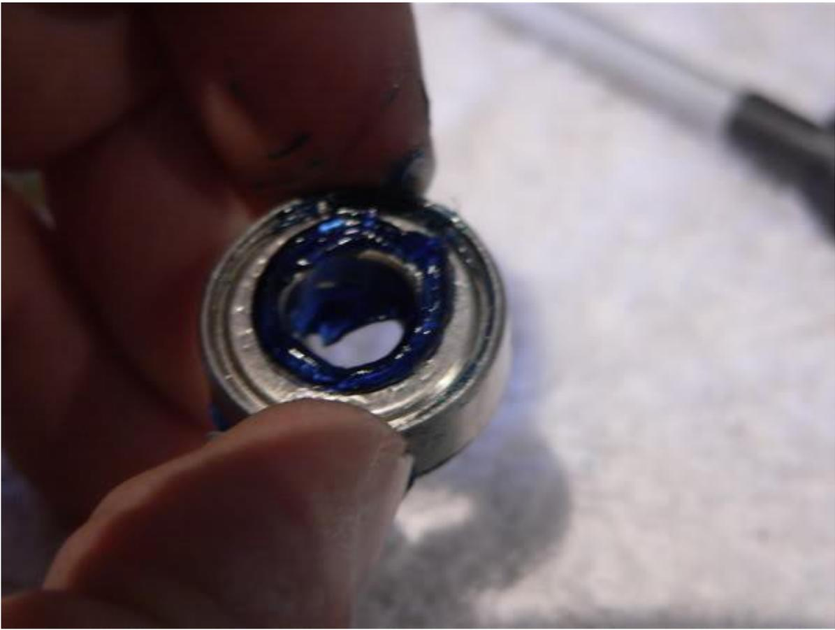
A bead of grease can be run around the main shaft bearing recess
