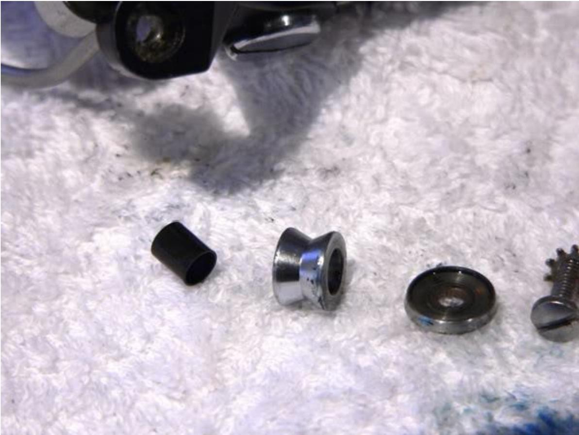
There was some grunge between the roller (key #35) itself, the roller washer (key #132) and the spindle. Along with some minor corrosion beneath the line roller screw.
