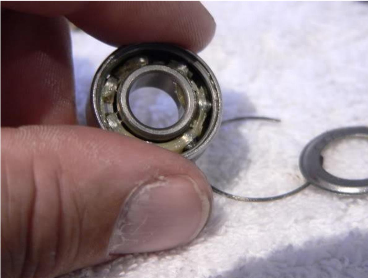
The cleaned bearings can all be packed with grease (Evinrude outboard grease in this case). To make sure there are no air pockets in the grease, pack one side first then replace the shield on that side. Pack the other side and press down on it hard with the heel of your palm. If grease squeezes evenly out through the opposite shielded side, it's good to go.
