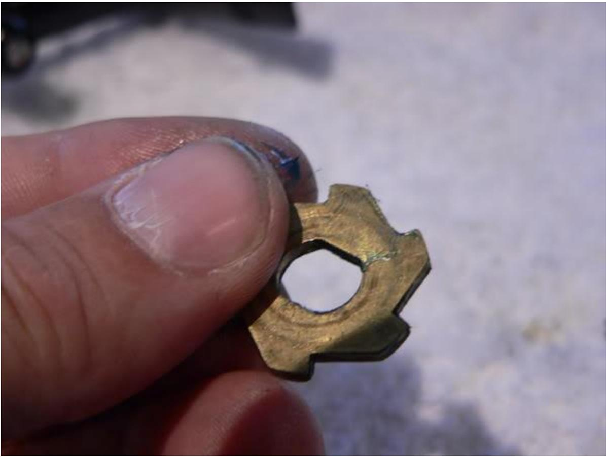
**When reinstalling the anti-reverse trip cam (key #236), make sure the spring (key #6D) engages with its retaining mount.**
