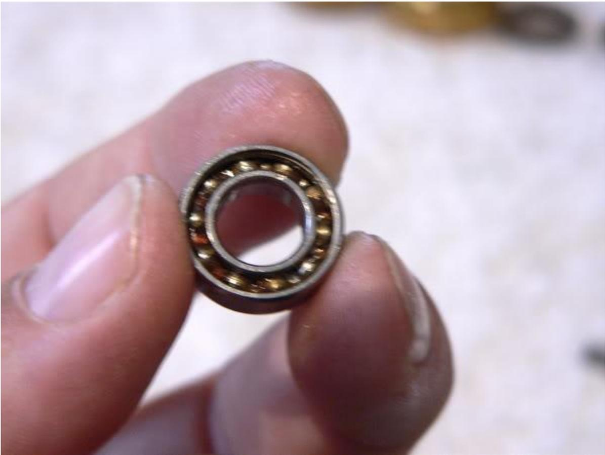
and give it a good clean to clear out all the old lube... I did this before converting to Alan's Carb Cleaner method, so used white spirit. Put the clean bearing to one side... we'll get back to that in a minute.
