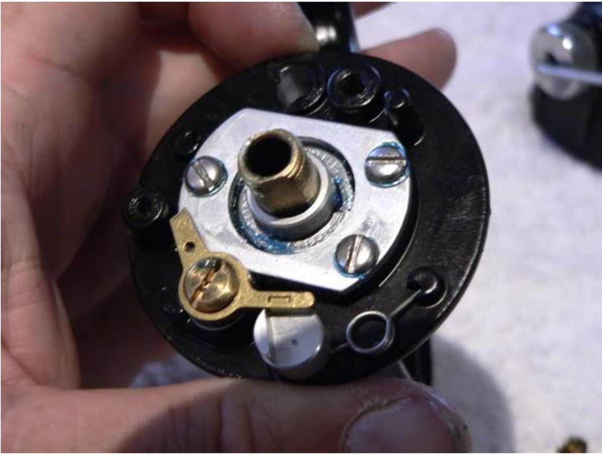
There was a little minor surface corrosion evident on the transfer lever (key #224) so let's give all of the individual parts in the sub rotor assembly a smear of grease using greasy fingers.
