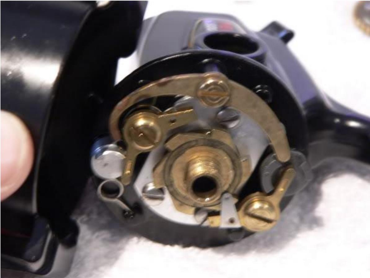
To disassemble the next stage and get at the main bearing, first unscrew and remove the anti-reverse lever (key #6E) from the rear of the reel
