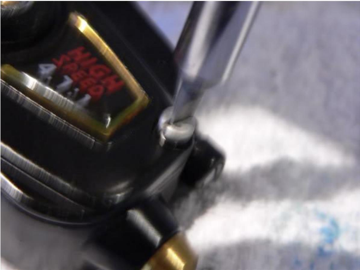
The screw thread and elbow of the handle (key #15) get a smear of grease
