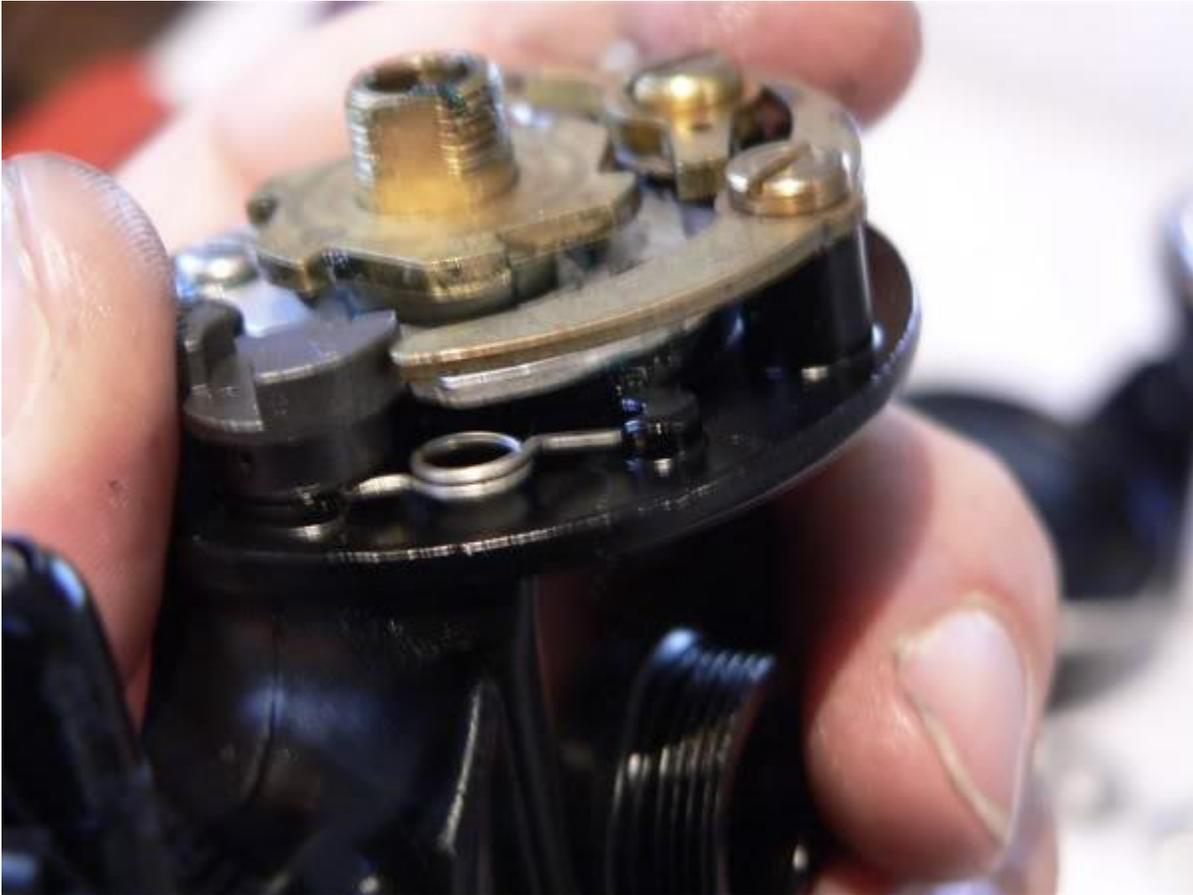
And finally, a coat of grease on the mounting plate will help resist corrosion (this should probably have been done before reinstalling all those bits but go figure!)
