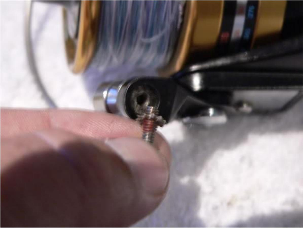
and the line roller assembly (key #'s 132, 35, 35A) can be removed.
