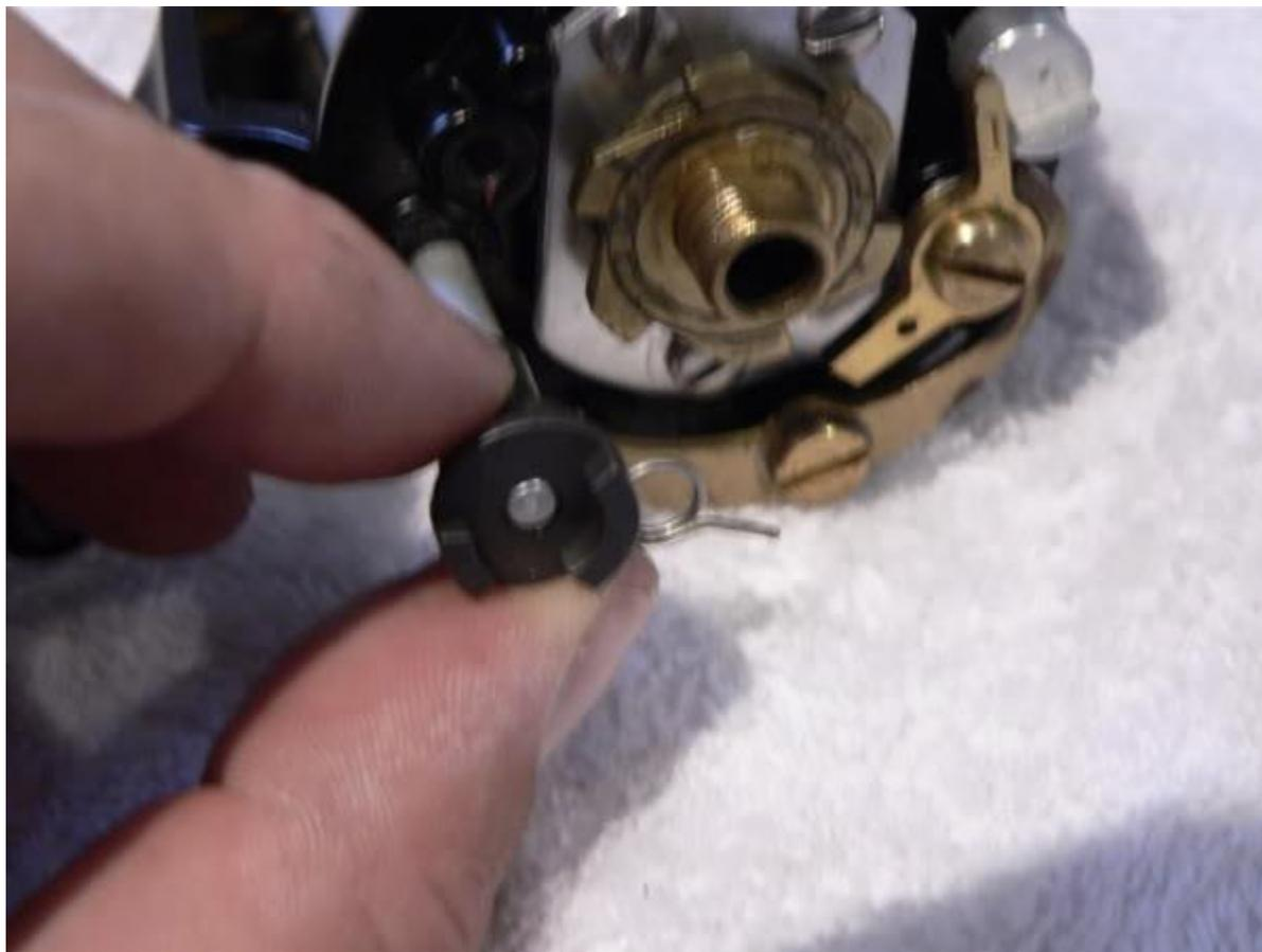
The ratchet gear (key #10) just lifts out (make sure you remember which way the gears are facing!)
