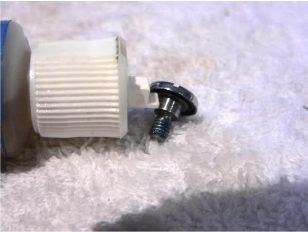
To reattach the bail arm and wire, start with the screw-in mount...
