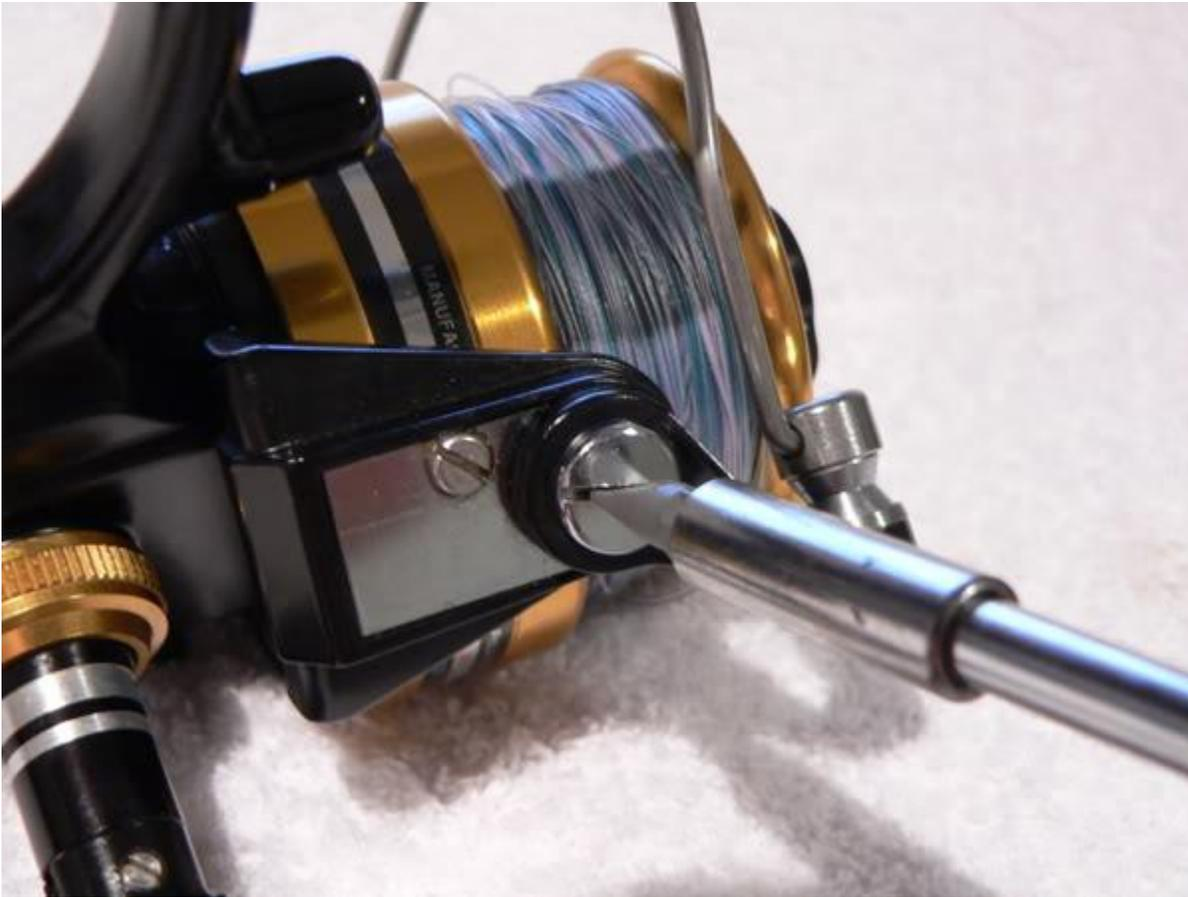
and undoing the screw-in mount (this is integrated with the bail wire key #24) on the opposite side... you'll need to start this off with a pair of vise grips or multi-grips.
