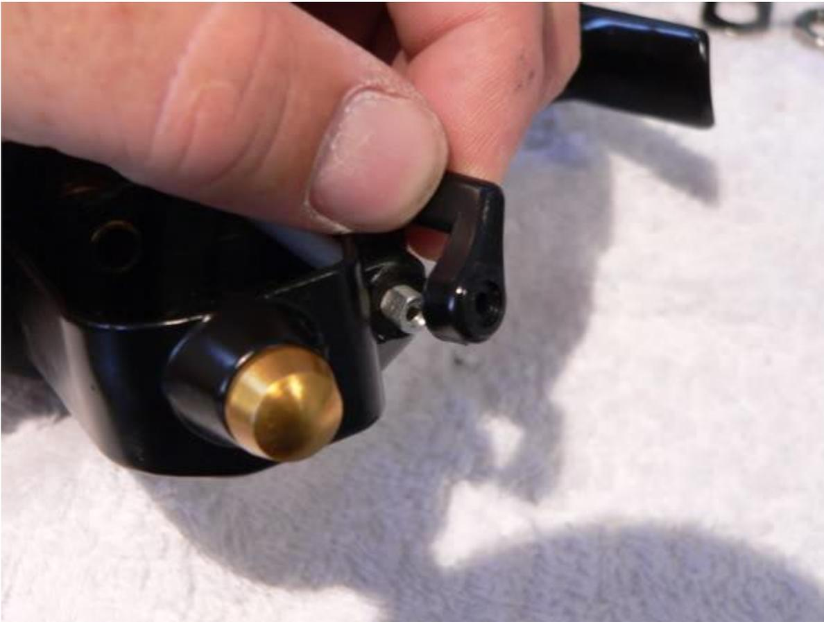
then unscrew and remove the anti-reverse dog (key #4A) (this is how spin reels did it before clutch bearings... we now get infinite anti reverse but at a higher risk of the anti reverse failing under load.
