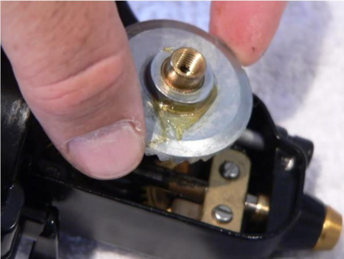
There are 2 screws (key #44) holding the shaft retaining plate (key #43A) on the oscillating slider (key #43)... these come out so the plate can be removed.
