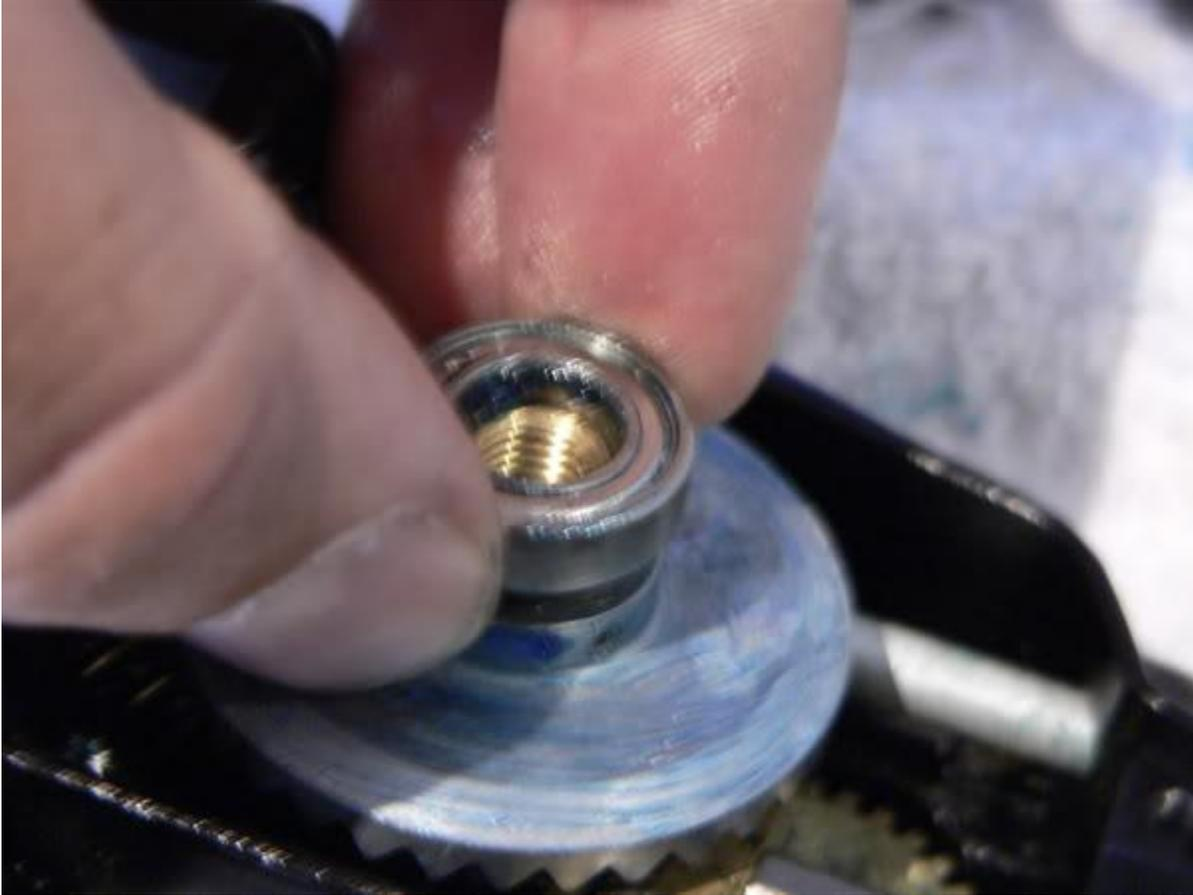
Give the inside of the left side plate (key #45N) a coat of grease and add a dab of grease to the screw holes (I really have to get myself one of the modified mini grease guns Alan uses) before screwing the plate back on.
