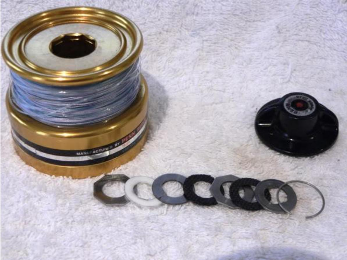
Give the HT-100 washers (key #6)... there are 2 of them... a rub with a clean cloth to remove any accumulated crud and to drive any old grease into the washer and out of the way, before reapplying fresh drag grease.
