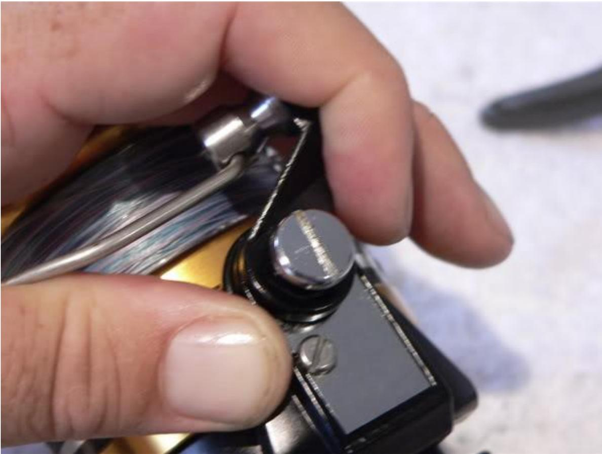
A drop of oil on the bail wire where it enters the screw-in mount.
