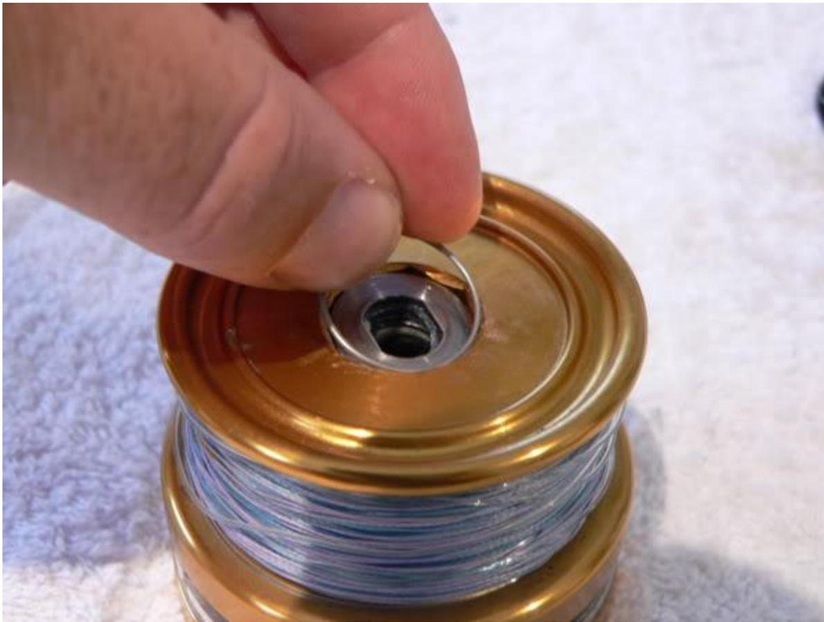
While we've got the spool in hand, flip it over and apply a coat of grease to the clicker and spring.
