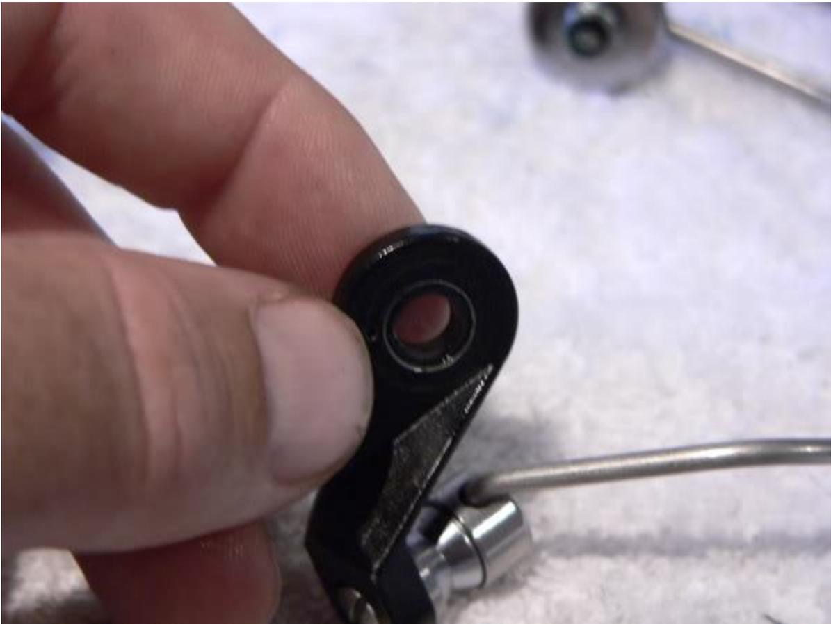
**Add a smear of grease to the threads of the bail arm screw and screw in mount... and a drop of oil to the spindle section of the bail arm screw.**
