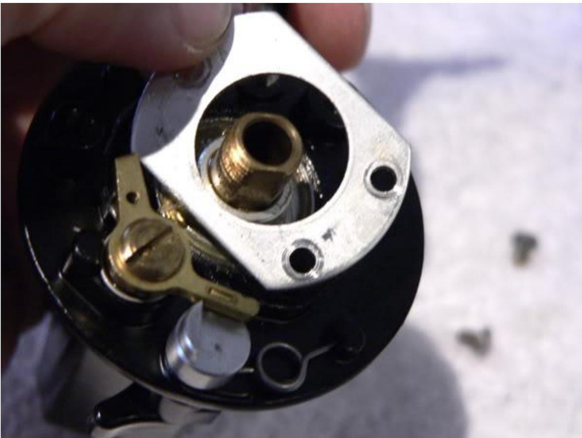
With the retaining plate out of the way, the pinion gear (key #19N) and main shaft bearing (key #20) simply lift out.
