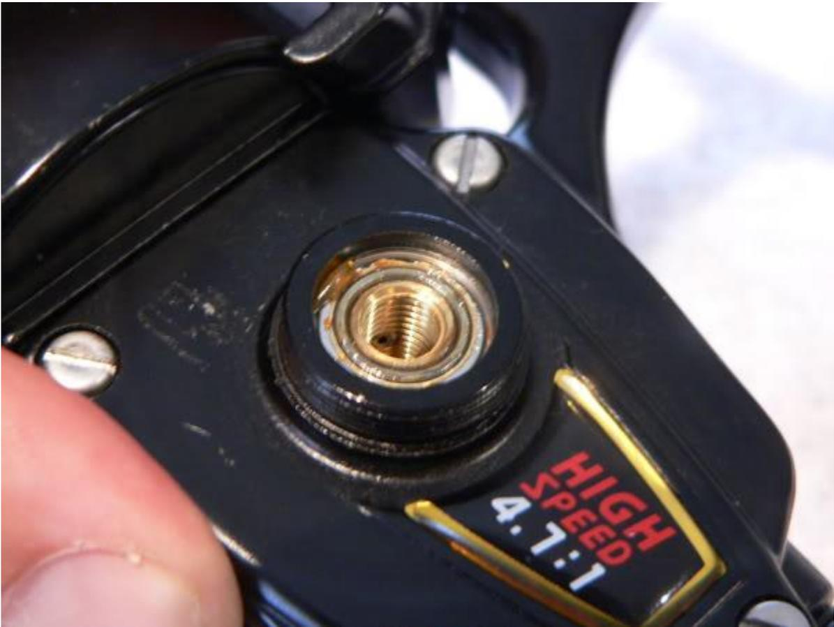
Back out the 3 screws (key #46) so you can remove the left side plate (key #45N)
