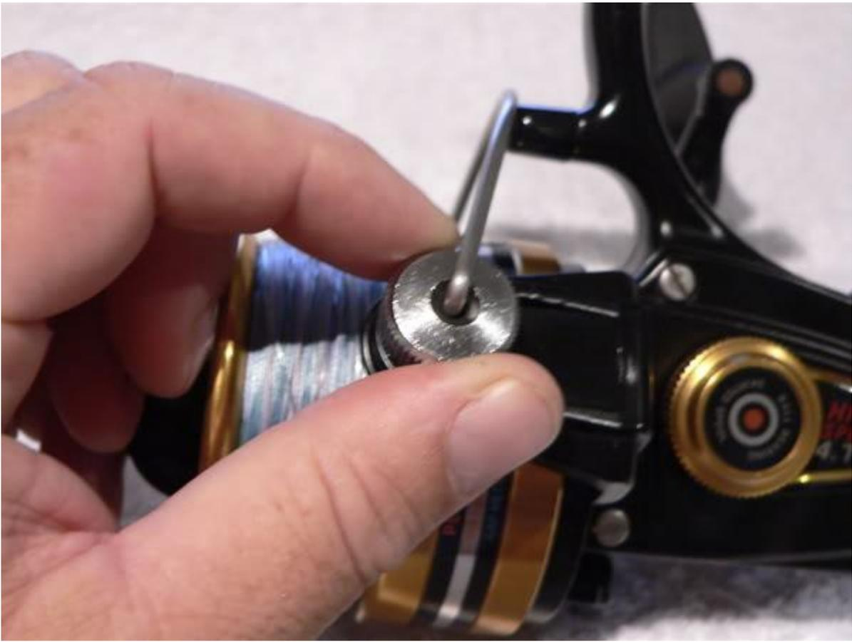
then the bail arm (key #34) and wire (key #24) can be removed... be careful to pull the bail arm assembly carefully off the bail arm spring (key #32) so as not to bend it. The spring is under a fair degree of tension.
