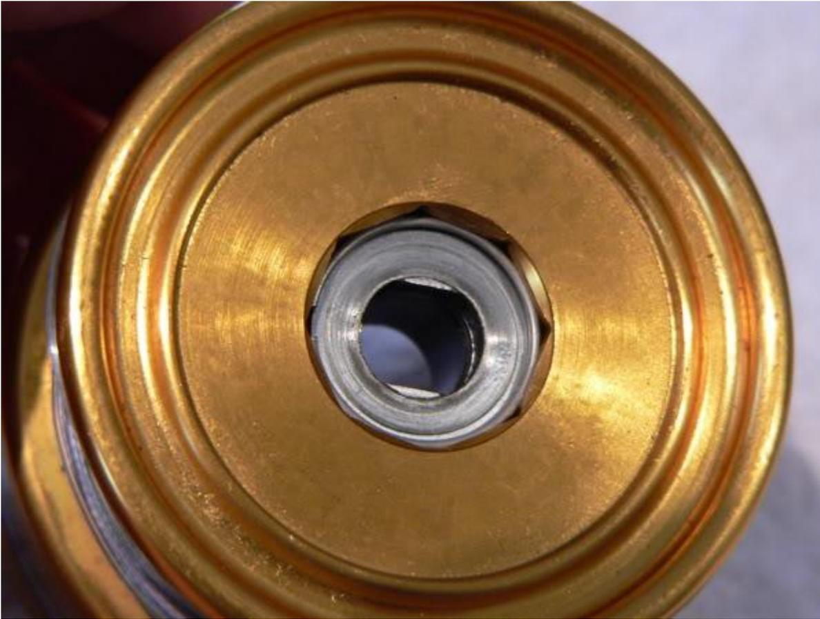
Remove the retaining spring (key #51) carefully so it doesn't go flying...
