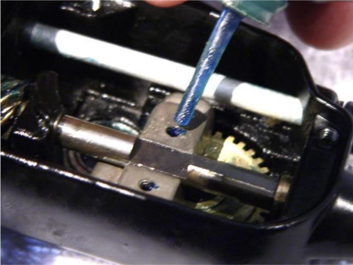
The drive gear (key #8N) can now be greased and slipped back into position
