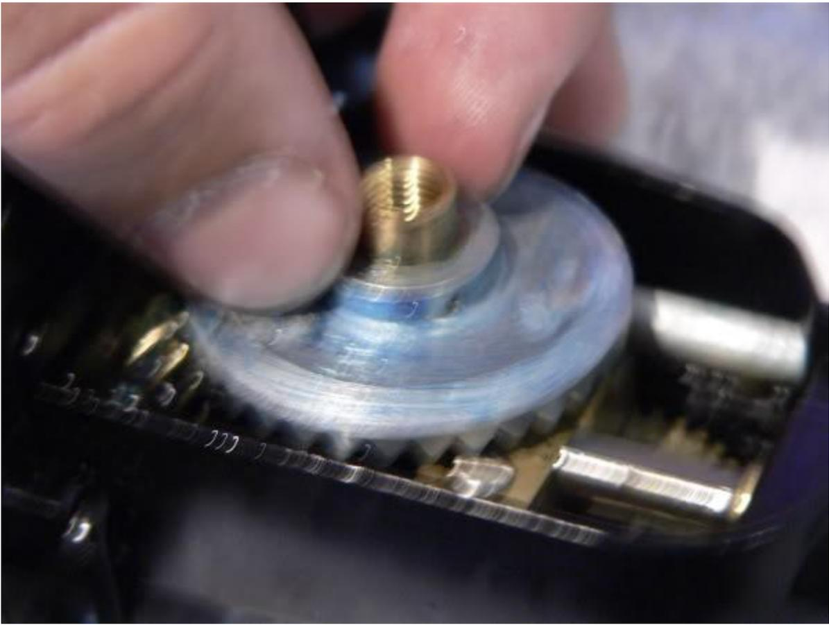
And the left side bearing (key #20A), having been packed with grease, replaced.
