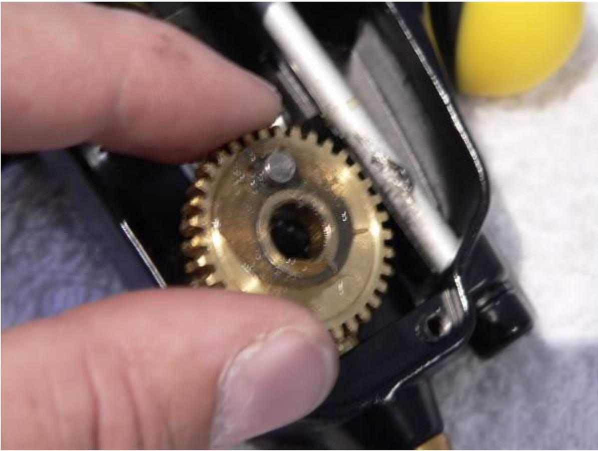
The right side bearing (key #20A) is now accessible and can be pushed out from behind. It too gets opened up and cleaned.
