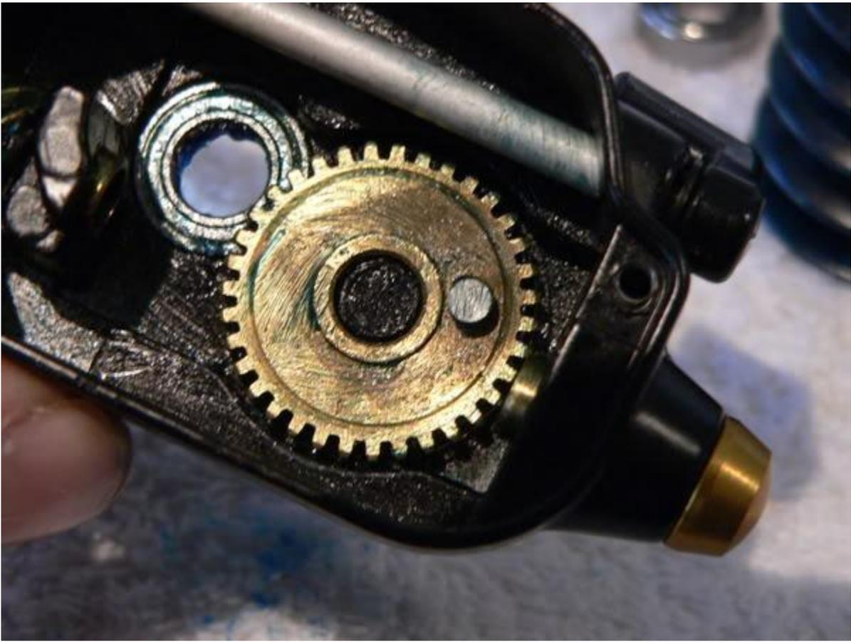
With the oscillating slider (key #43) reinstalled, add a drop of oil to the shaft recess in the slider and to the shaft (key #39) itself before slipping it back in.
