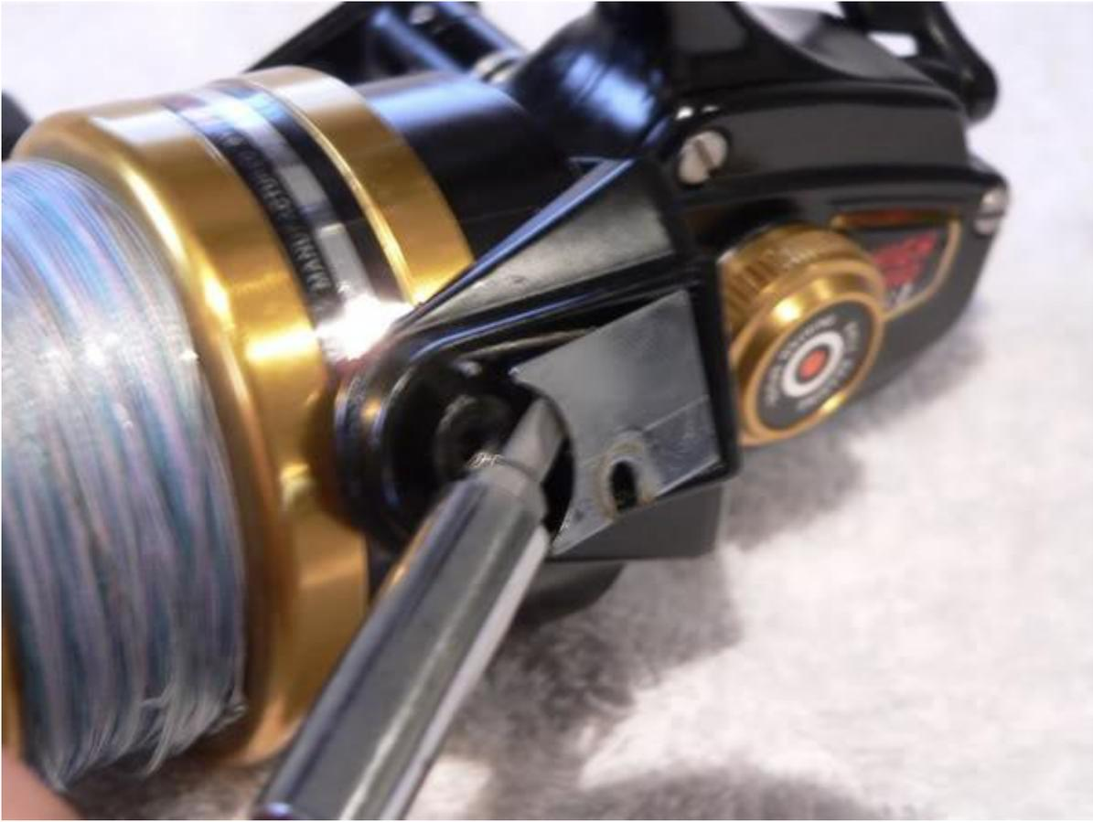
You'll now be looking at the bail spring (key #32), which needs to be removed. It's under enough tension to really need a pair of needle nose pliers. And there's always the risk when dealing with loaded springs that they'll fly off into the nearest deep-pile carpet... so hang on.
