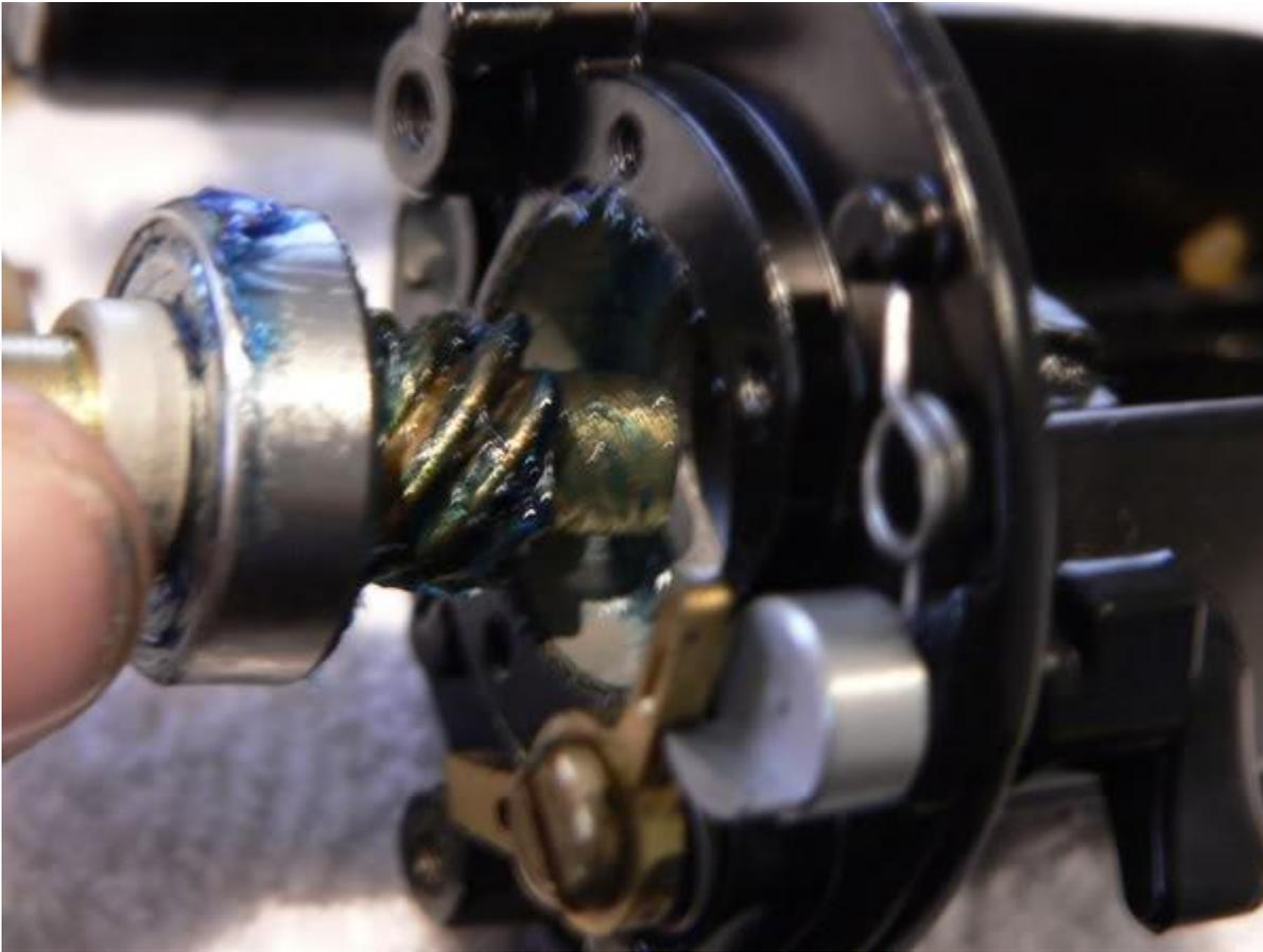
**Before replacing the bearing retaining plate (key #21), give it a thin coat of grease and lightly grease the screw holes**
