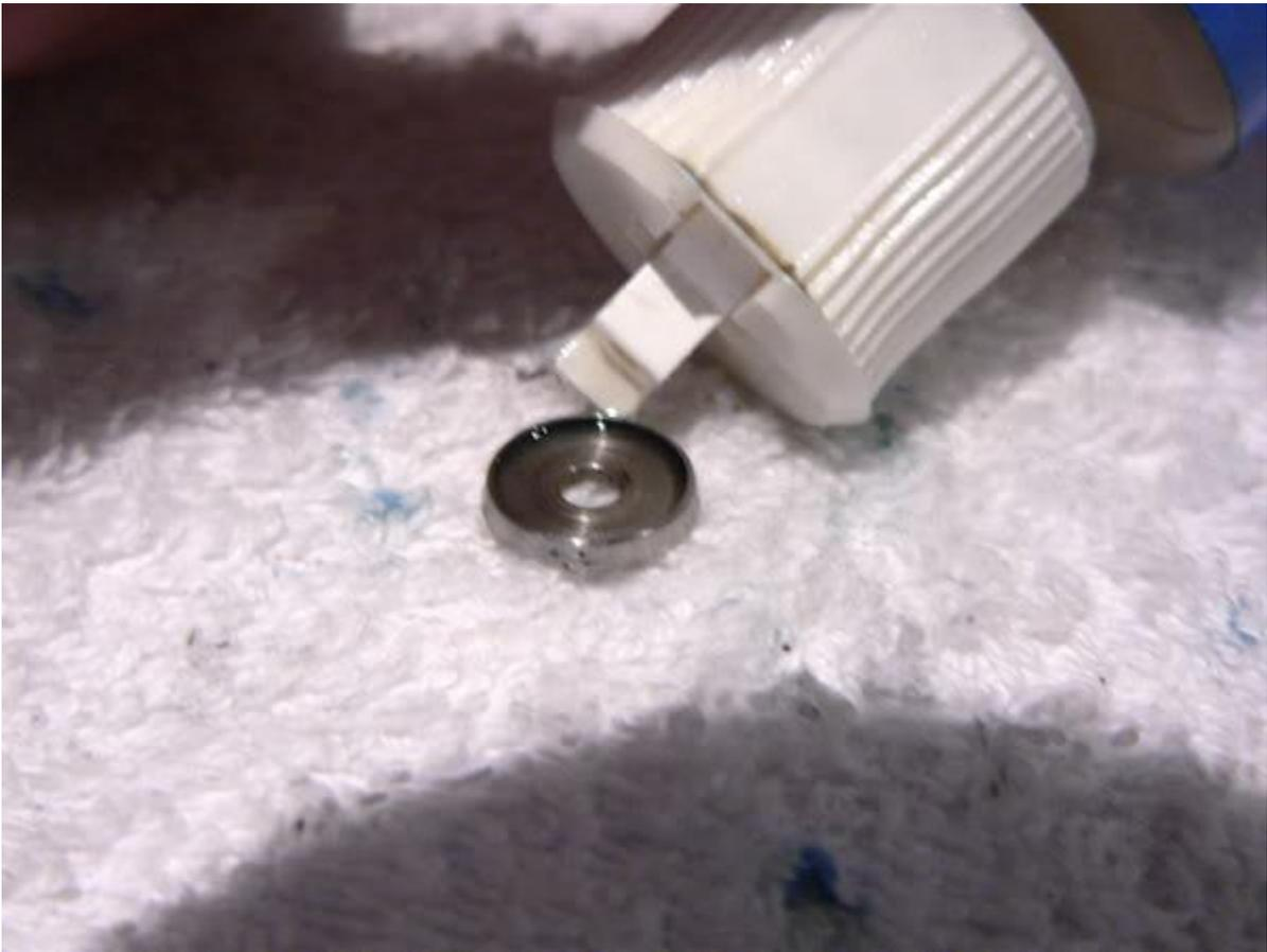
Let's not forget the bail arm assembly. Begin by backing out the bail arm screw (key #31)
