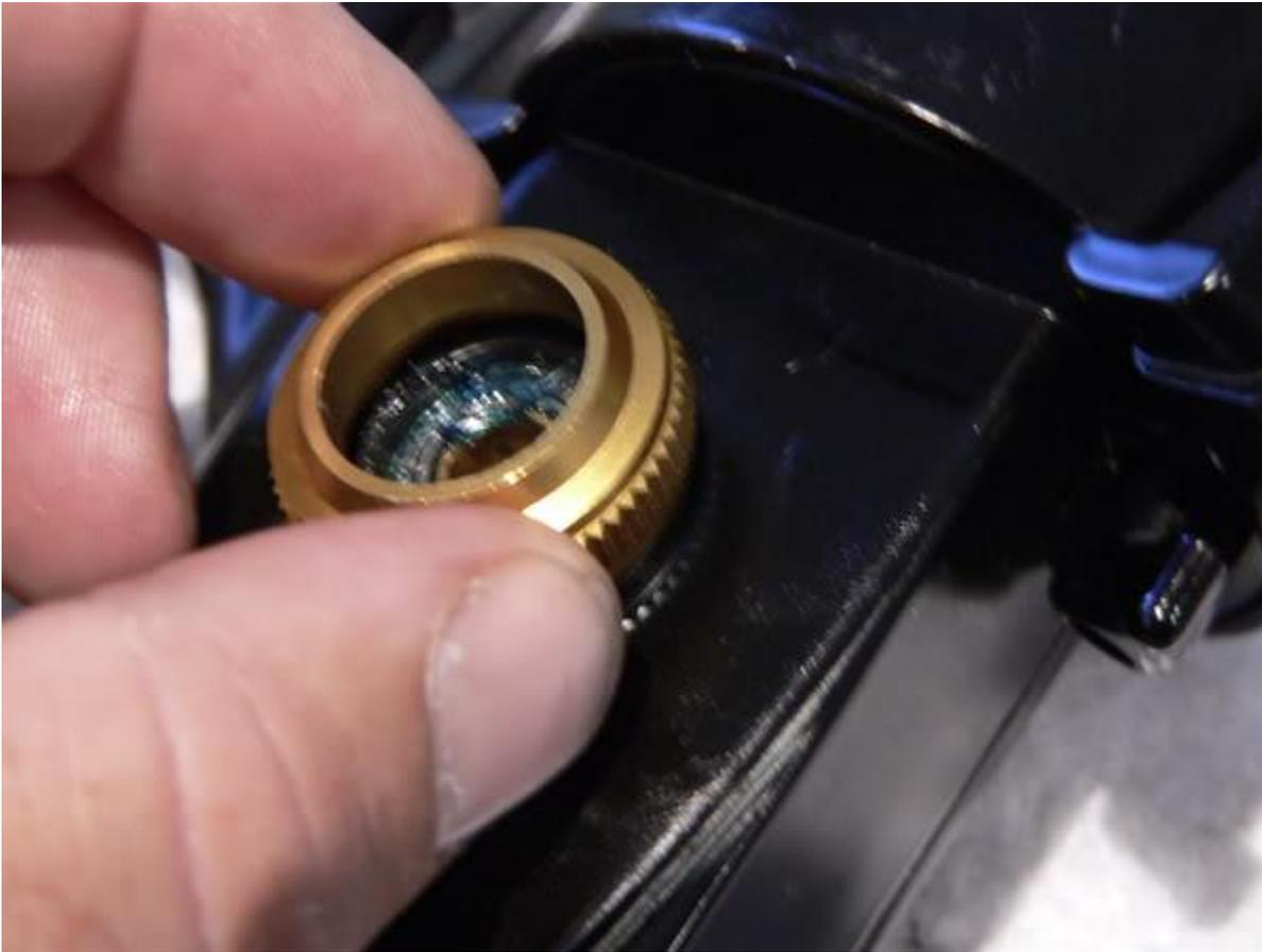
note that there's a felt washer (key #17N) that lives beneath the handle that serves as a rudimentary seal. If left dry, I can only imagine this would actually hold and retain water... not ideal! So it gets thoroughly soaked with Evinrude grease first (where I can I try to keep different types of lubricants from coming into direct contact, otherwise I would probably have used drag grease)
