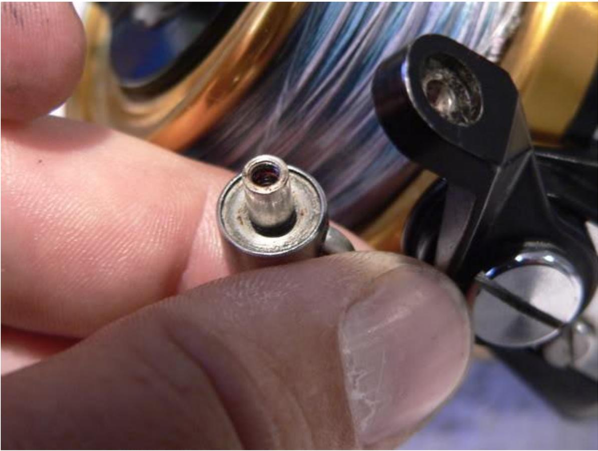
After cleaning, the screw recess gets a coating of grease while the parts of the roller assembly and spindle, get a drop of oil before reassembling.
