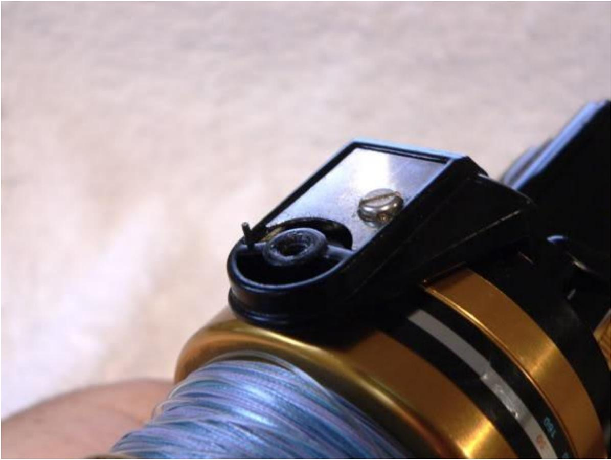
Next back the screw (key #50) out to allow the removal of the bail spring cover (key #227).
