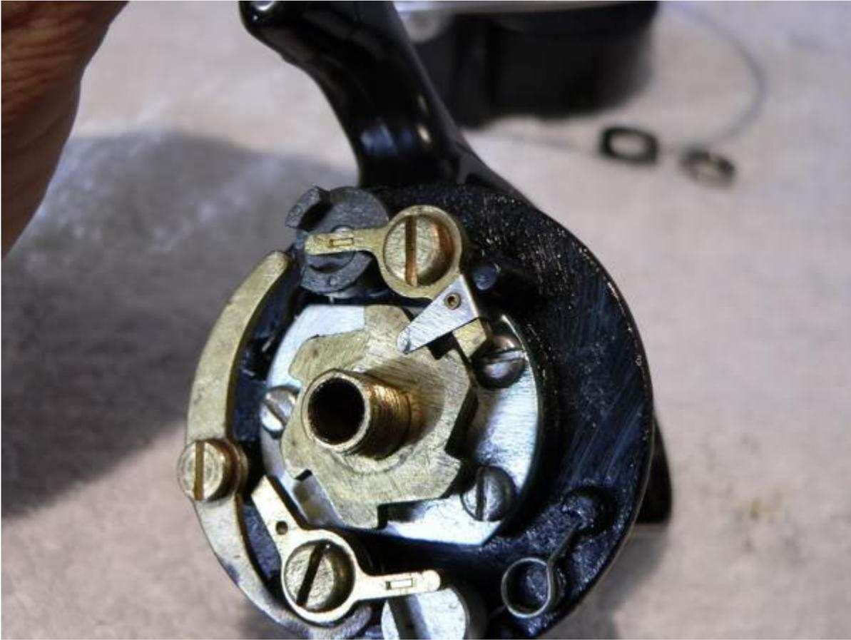
Screw the anti-reverse lever (key #6E) back on and this bit's finished.
