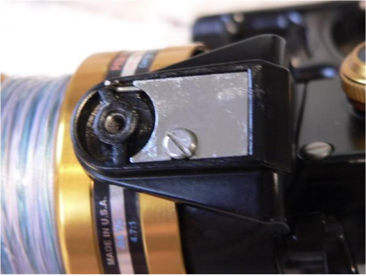
Now let's clean up the bail arm and mounts... remove the bushing (key #34A) from inside the bail arm, clean it, add a drop of oil and replace it.
