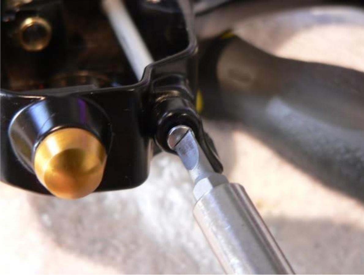
Reinstall the re-lubed right side bearing (key #20A)
