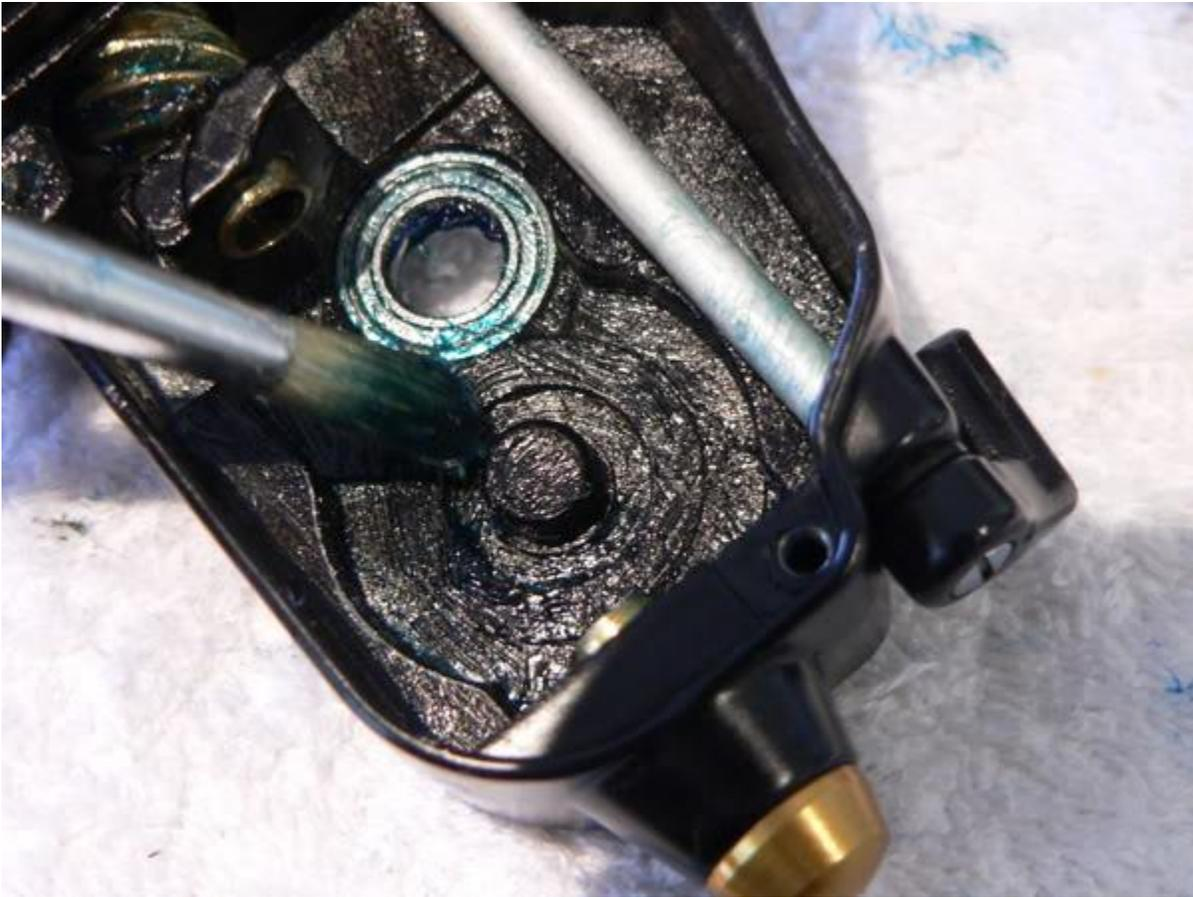
before greasing and reinstalling the oscillator gear (key #231)
