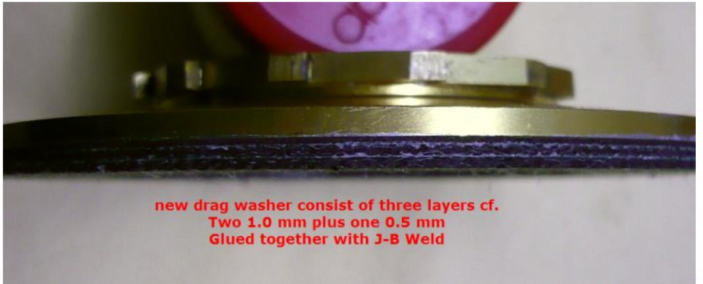
**new drag washer consist of three layers cf.**
