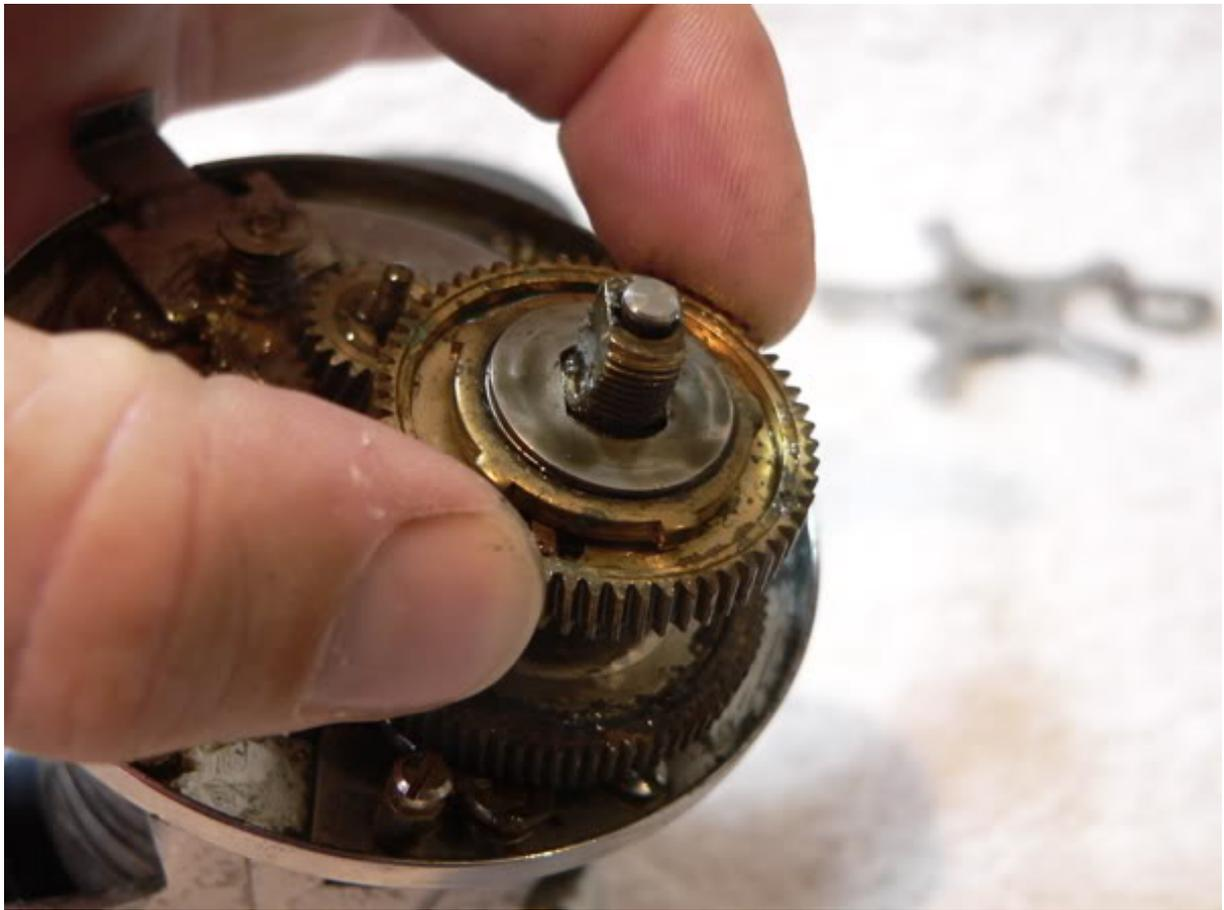
Remove the drag washers... the metal washers are stacked... and there's a washer beneath the gear too
