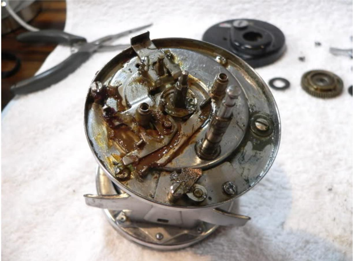
Remove the clutch cam (ref #9713) and slider (ref #9710)
