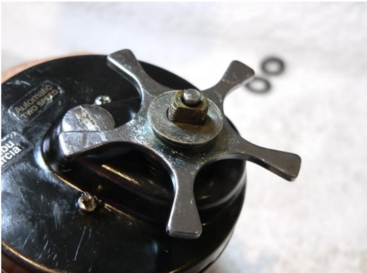
Remember me saying the handle of this reel needed attention... give the handle a coat of grease front and back where it is mounted and reinstall it. And in the case of this reel I installed a soft copper shim in the corroded locking screw hole.
