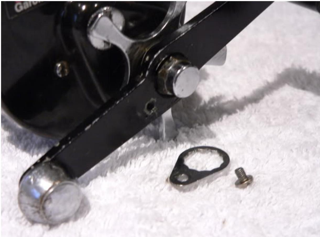
Next the handle nut (ref #6968) can be removed. There's an 'e' clip to remove carefully before the handle can come off.
