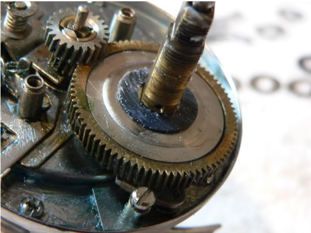
Then the smaller 'low speed' drive gear can be greased and reinstalled followed by installing the remaining drag washers... greased Carbontex of course.
