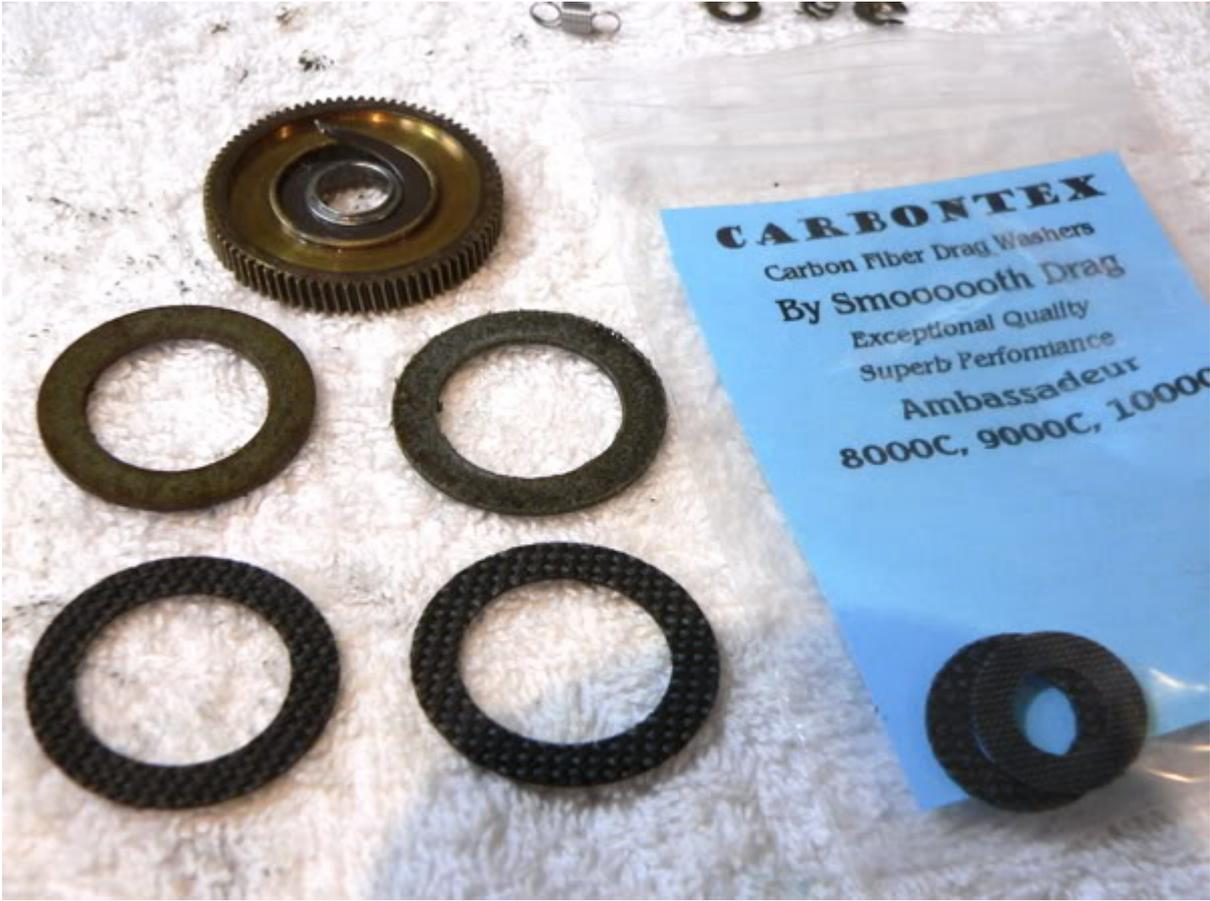
Give them and the drive gear drag recess a coat of drag grease before installing the new washers.
