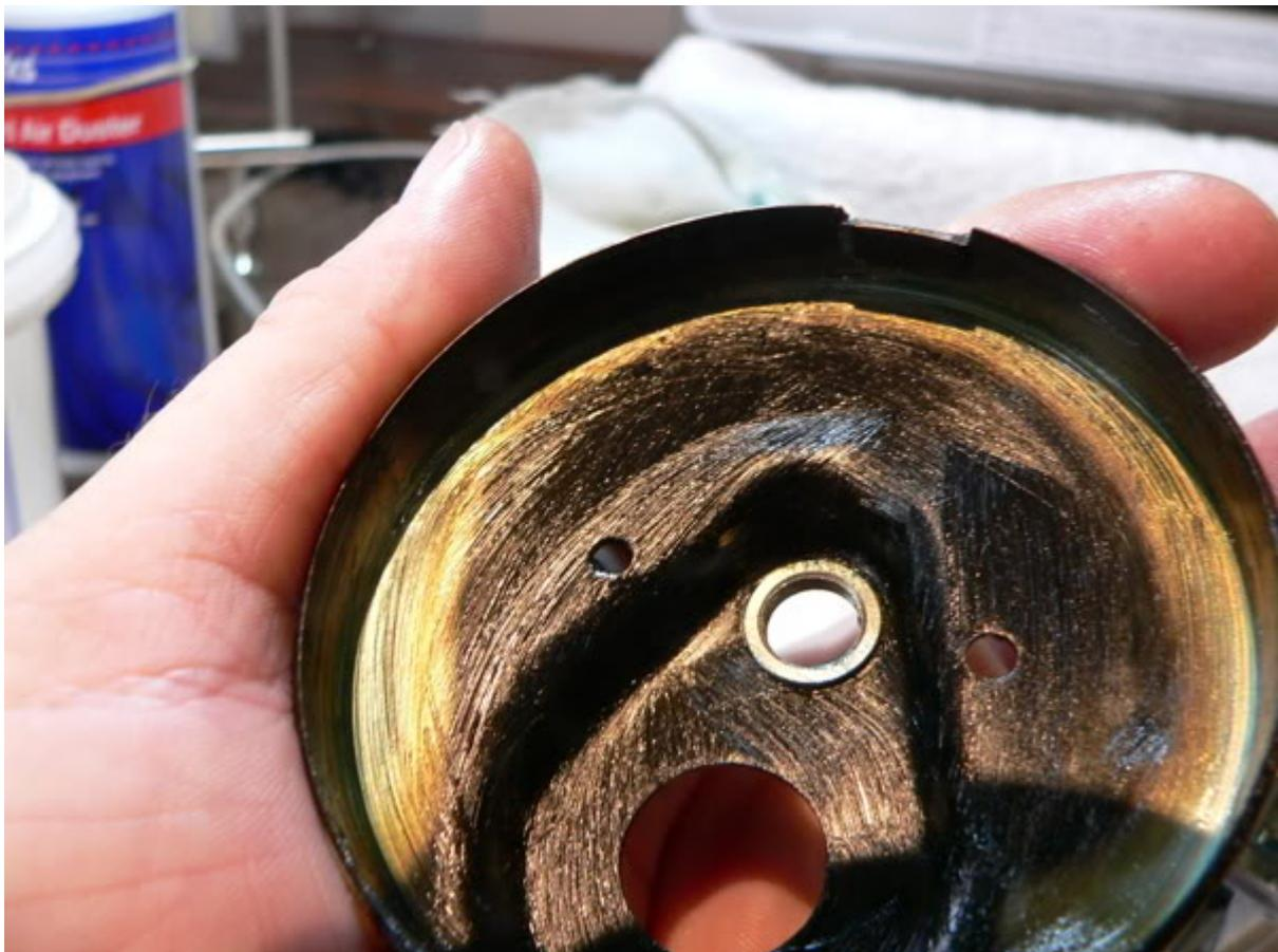
Then the side plate can be reinstalled and screwed back on... note that the seal frame has a small tab that needs to be aligned with the notch in the side plate.
