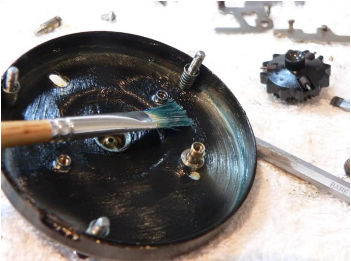
Then clean up, re-grease and reassemble the ratchet.
