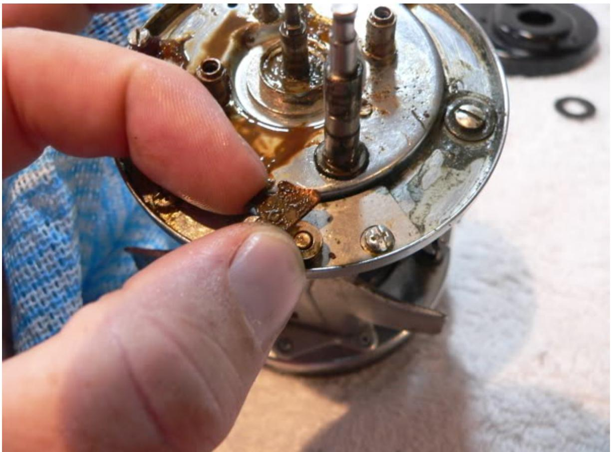
Remove the worst of your river mud (or the old grease, depending on your reel) then back out all the screws securing the right side mounting plate (ref #15018)... there are 6 screw in total, holding all the
