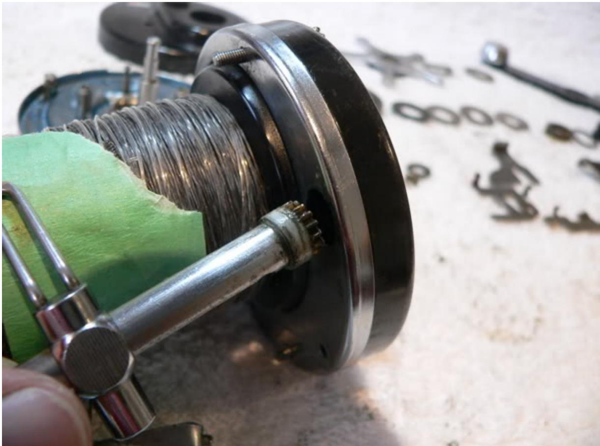
And the spool (ref #970248) can be slipped (or when there's a bit of rust involved like here... manhandled) from the left side assembly. Don't lose the spool spring (ref #4111)
