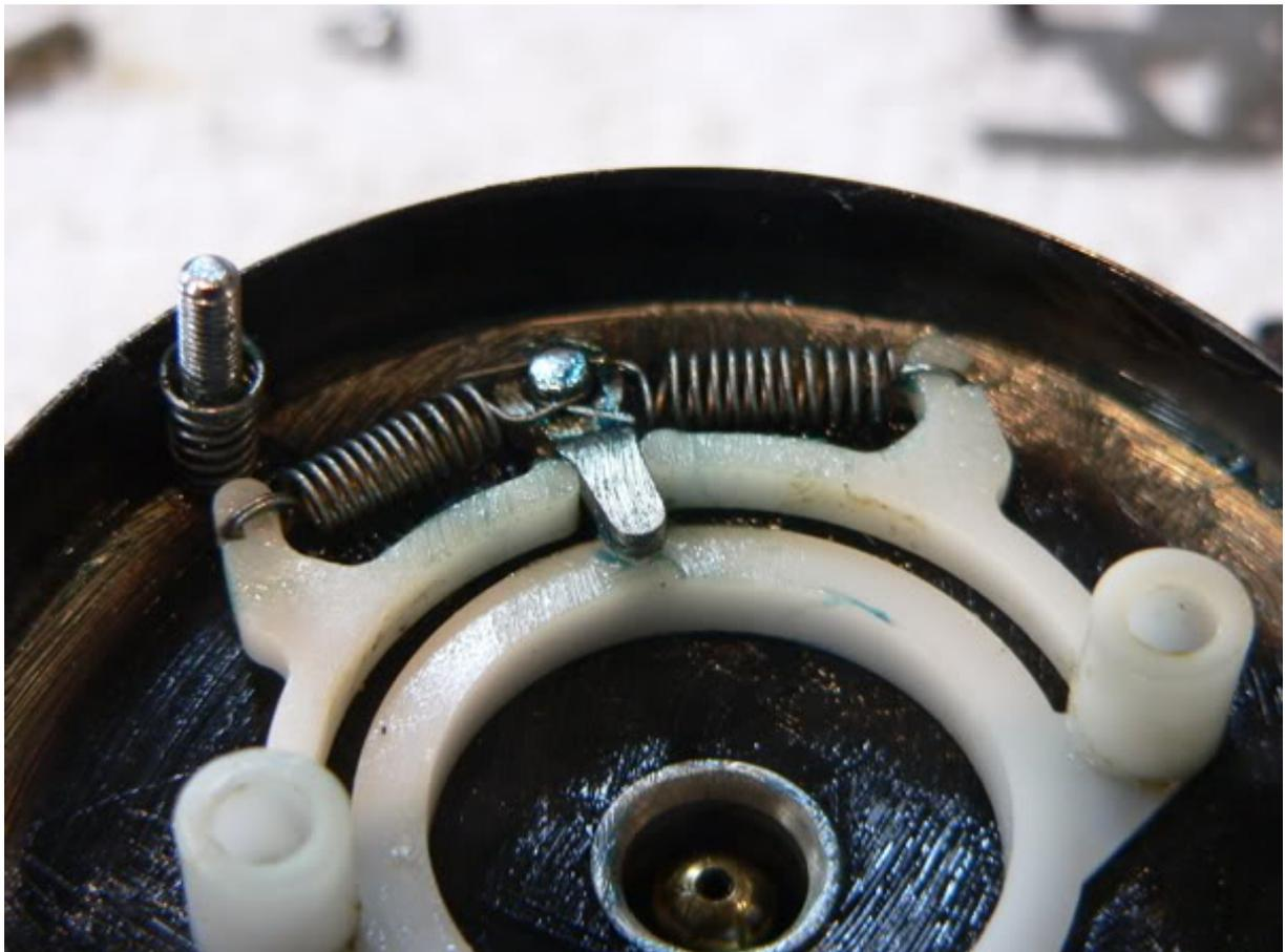
Give the idler gear a coat of grease, add some oil to the mounting point and pop the screw back in.
