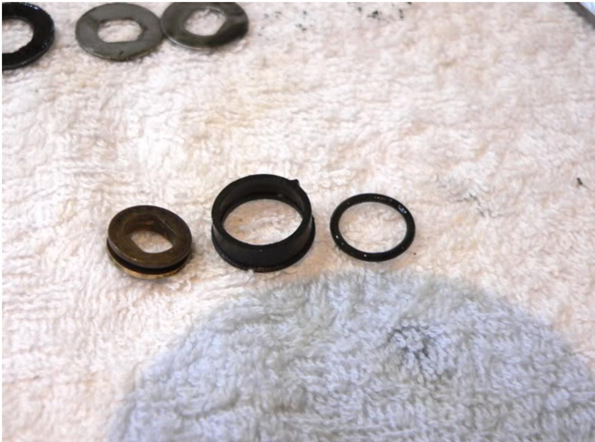
Having 2 speed gearing, there are 2 drive gears. The smaller 'low gear' drive gear slips easily off the drive shaft.
