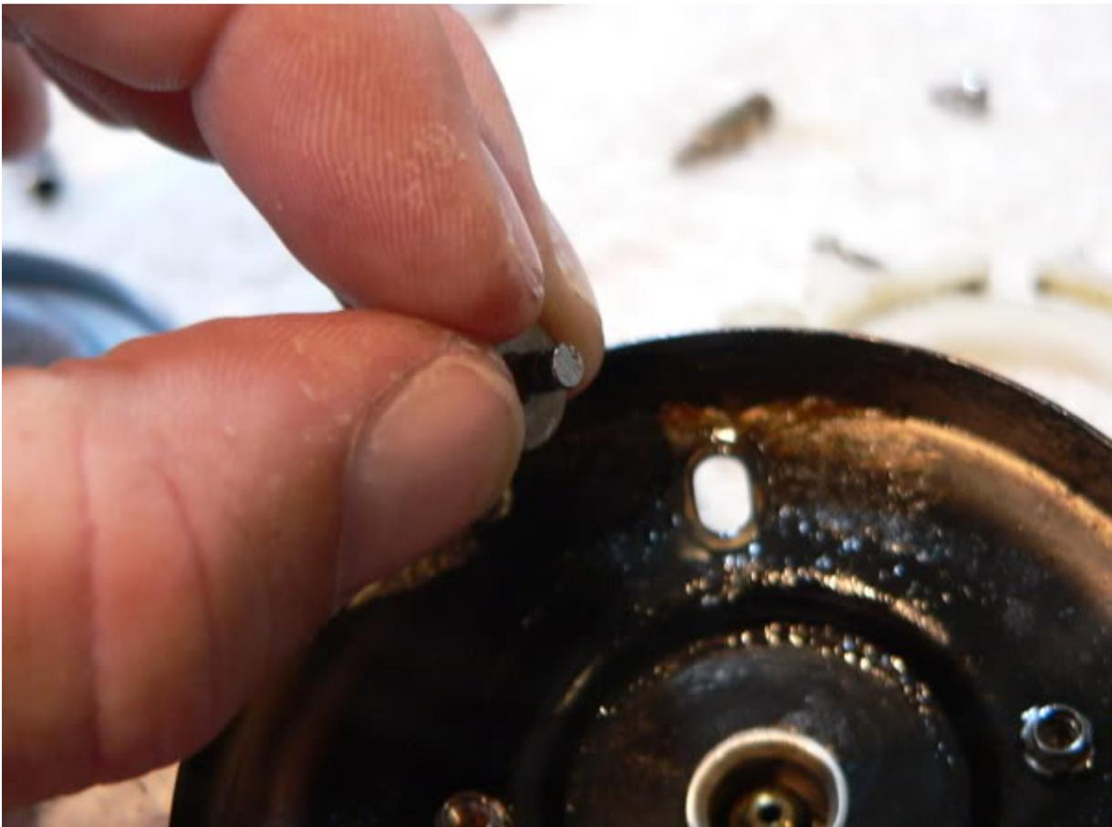
Clean up the inside of the left side plate and brush on a thin smear of fresh grease to protect everything.
