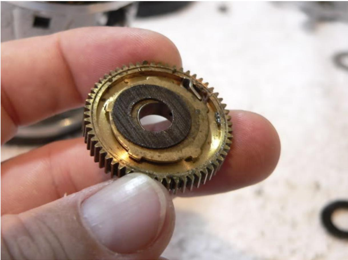
Now, to get at the larger, high speed drive gear, you'll need to partially dismantle the clutch. Begin by removing the yoke spring retainer (ref #8845), yoke spring (ref #9741) and thrust washer (ref # not shown on schematic)
