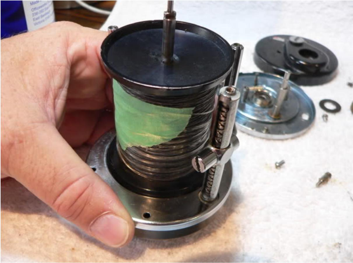
Smear the mounting plate of the reel seat with a little grease and reattach it to the left side assembly
