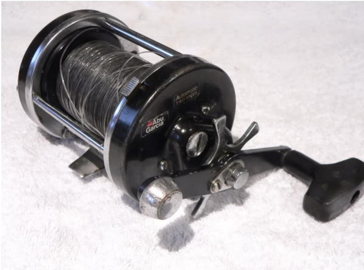
The first thing to do is remove the handle assembly. Back out the handle nut locking screw (ref #8907). Then the handle nut collar (ref #4581) slips off. Here's the first problem... the thread in the handle for the screw has been badly damaged by corrosion. We'll have to sort that out later.
