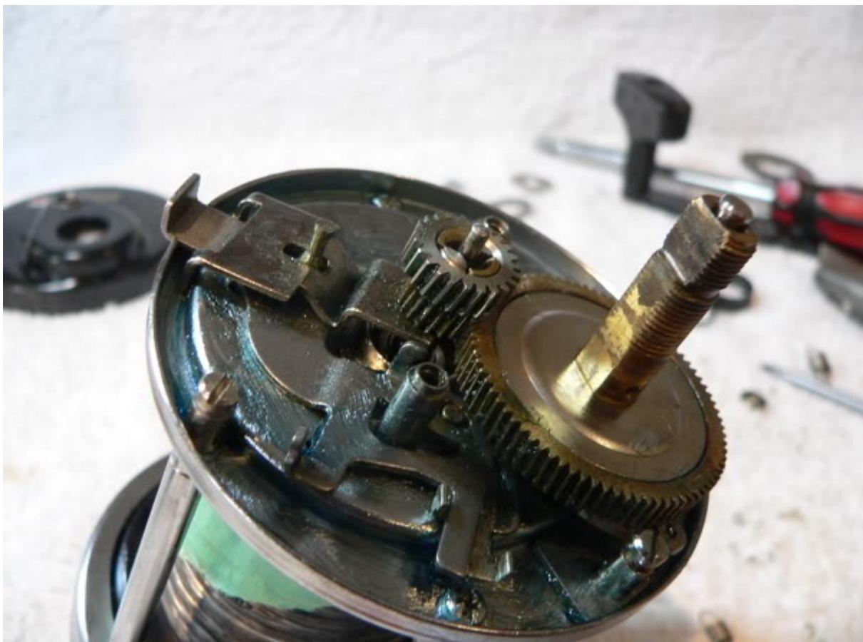
Reinstall the yoke spring and spring retainer
