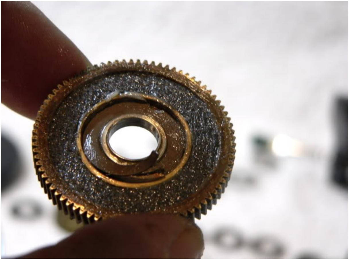
The drive gear teeth and the anti reverse gear & dog can all get a coat of blue grease.
