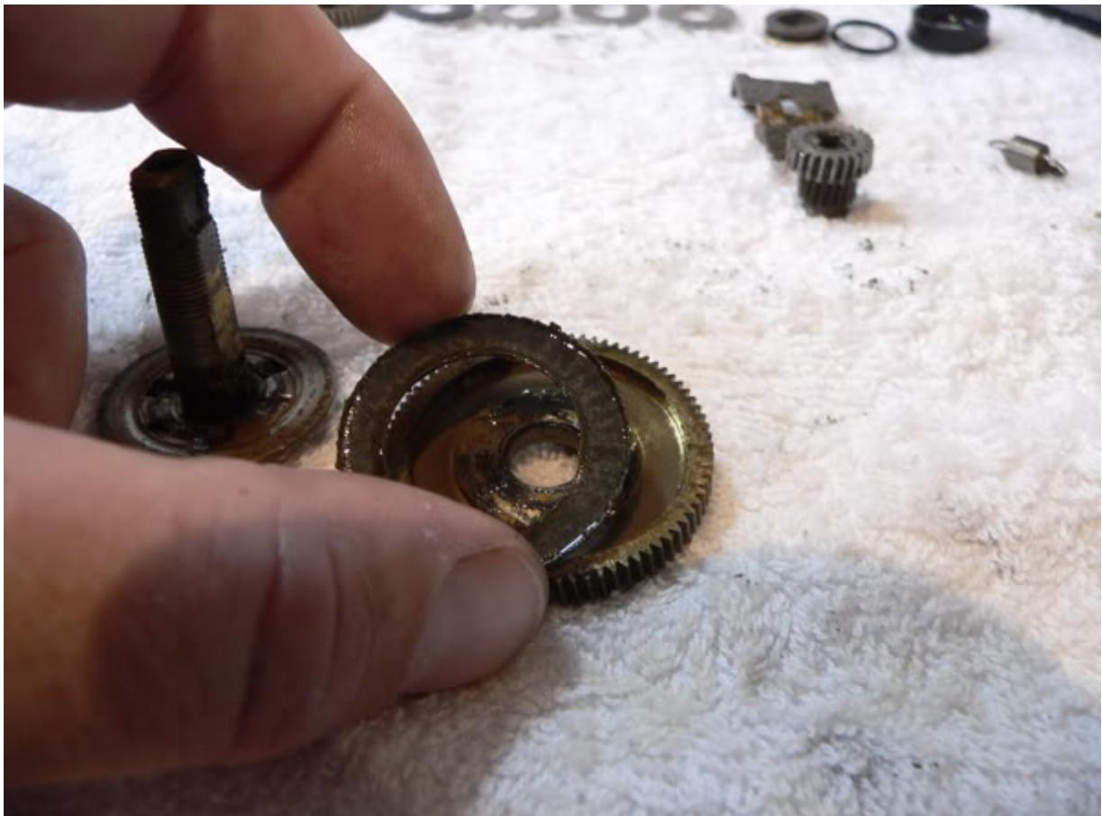
And the same with the washer beneath the drive gear (that bit that looks like torn metal is actually the drag clicker).
