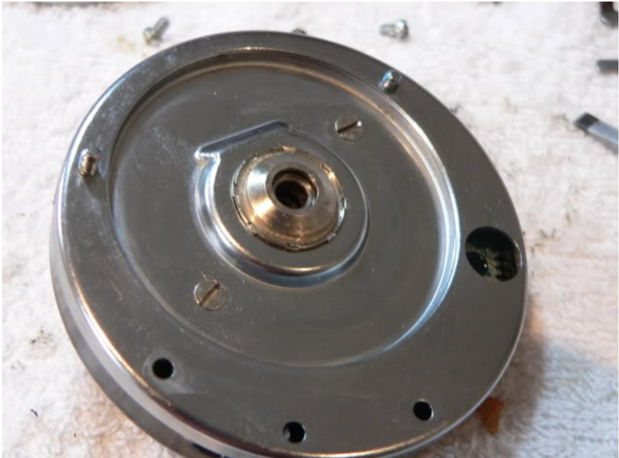
Time to give some attention to the poor, neglected levelwind assembly, starting by cleaning the gunk out of the line guide 'guide shaft' (ref #15023)
