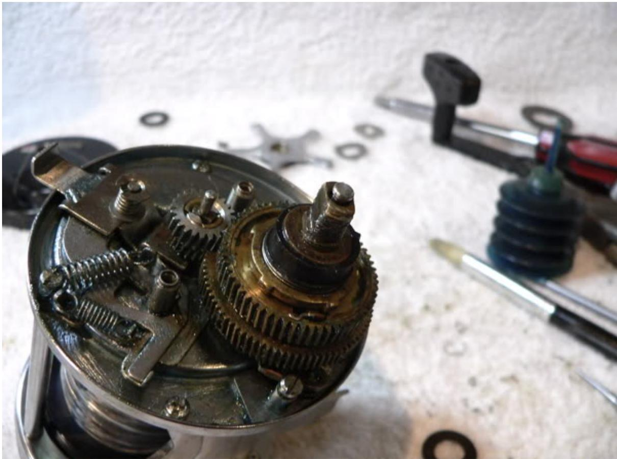
Apply a light protective smear of grease using an old paintbrush or toothbrush to the inside surface of the right side plate.
