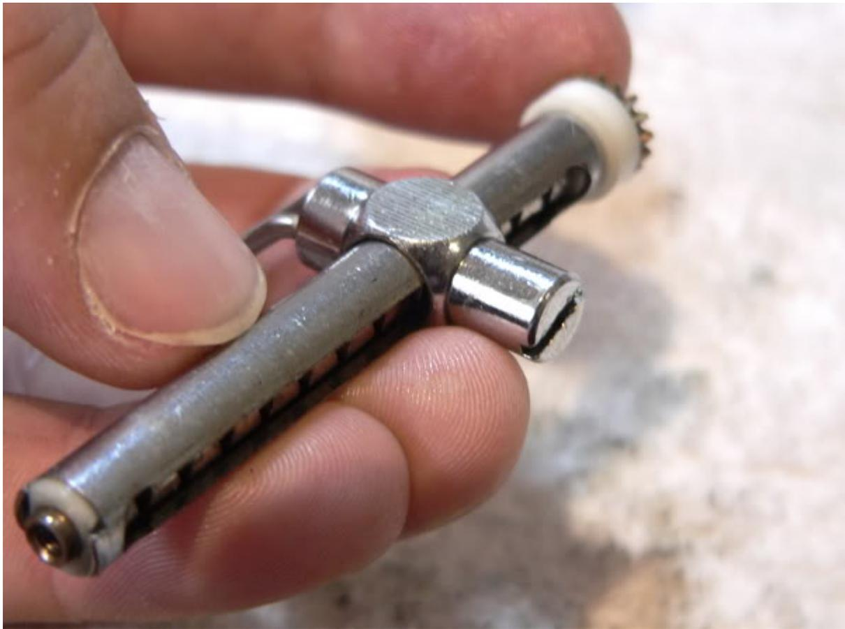
Reattach the line guide shaft adding a small dab of grease to the screw hole first, then slip the levelwind assembly back into place, making sure that the line guide is seated properly in the grooved guide shaft.
