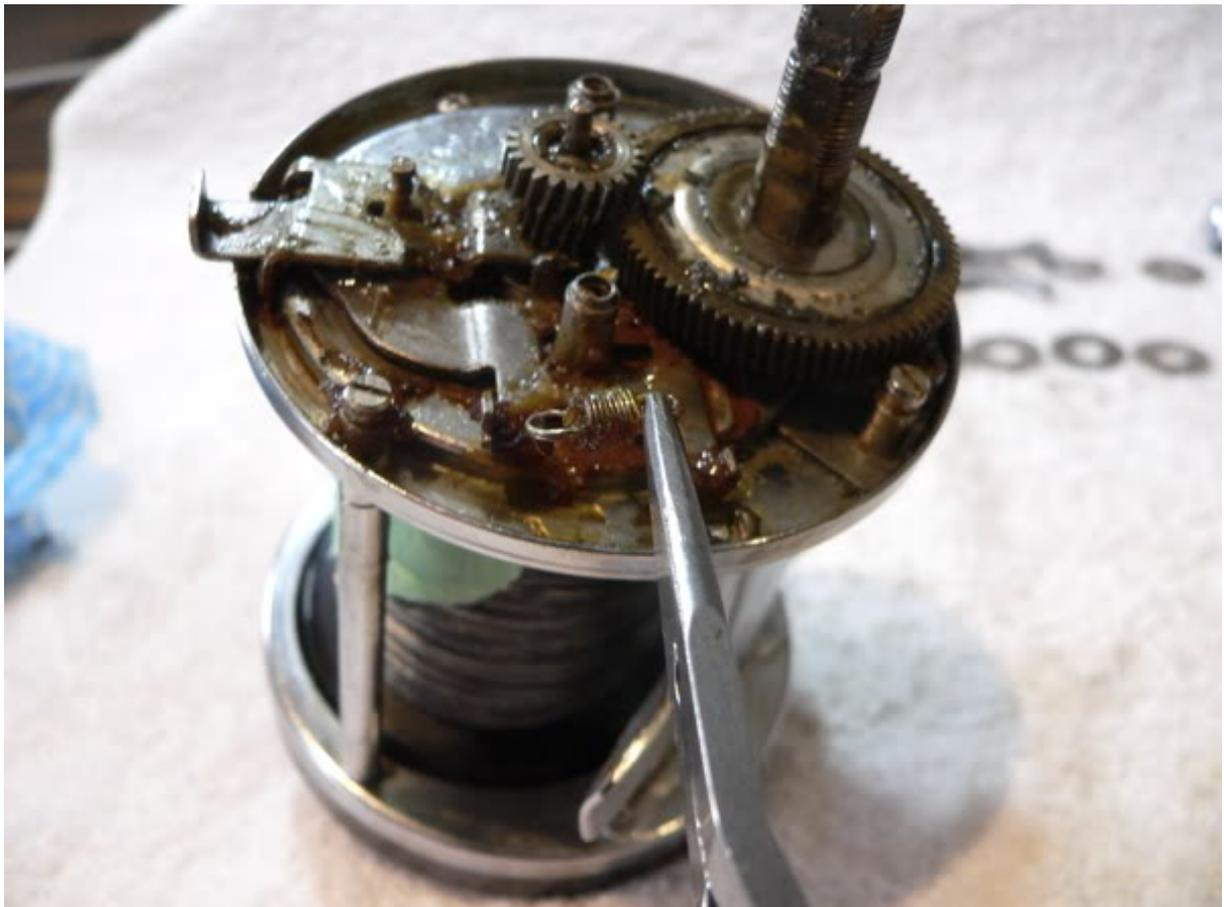
With a bit of careful manipulation, the yoke should now lift off allowing you to remove the pinion gear (ref #9737).
