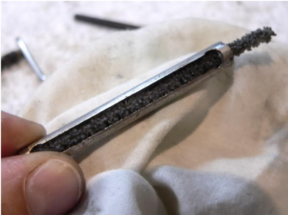
Then give all the components, including the worm screw a thin coat of oil. Add a drop of oil to the bushings at each end of the shaft and the pawl as you're reassembling the levelwind.
