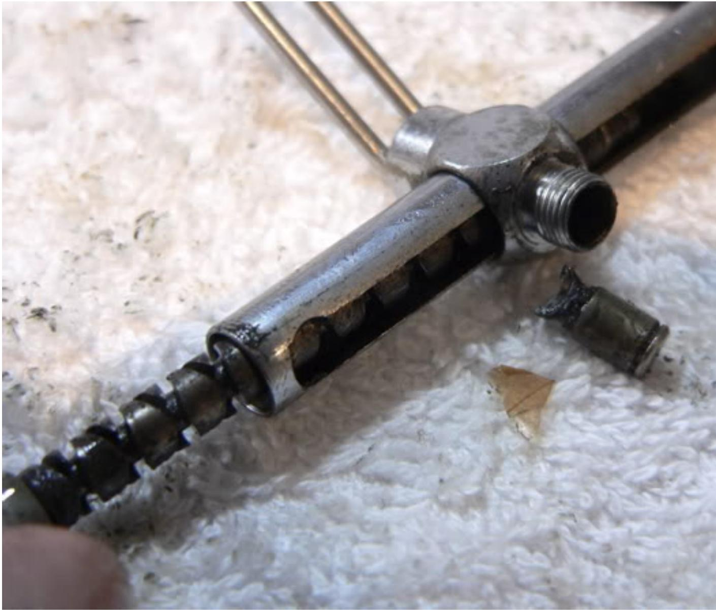
Give all the components a good clean with white spirit... pipe cleaners and Q Tips are a great accessory at this stage (that pipe cleaner started out white at the other end of the worm screw cover by the way).
