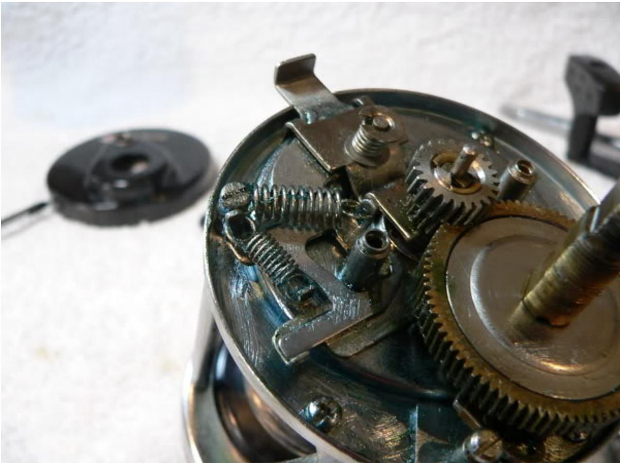
One of the Carbontex washers goes on next to separate the 2 drive gears, after a good coating of drag grease
