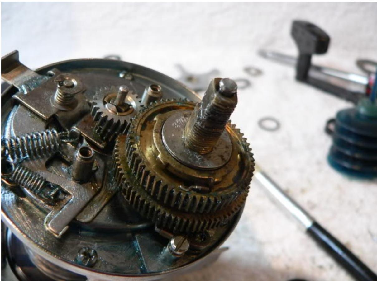
Clean out the spacer washer/seal components... including the o-ring (ref #8918, #9736 & #8868), give them a light coating of grease (drag grease might be advisable to avoid cross contaminating), reassemble and install.
