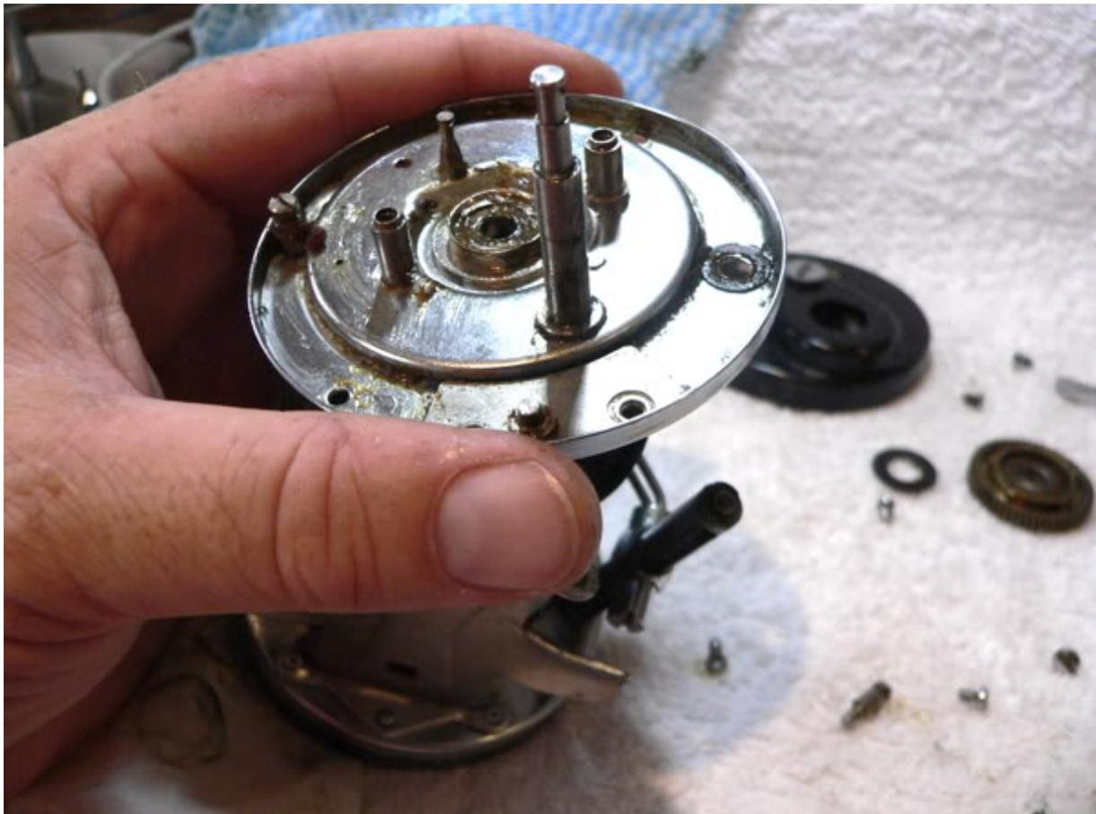
Take out the 'C' clip (ref #8816) securing the right bearing (ref #8940) and the bearing should just slip out.
