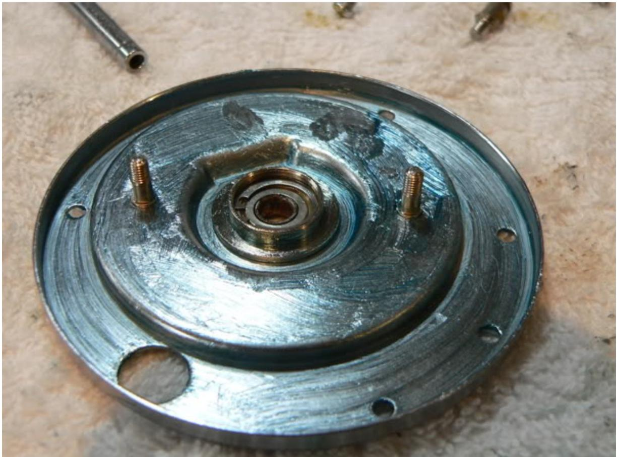
The left side plate is in much need of attention so remove the idler gear (ref #15010)
