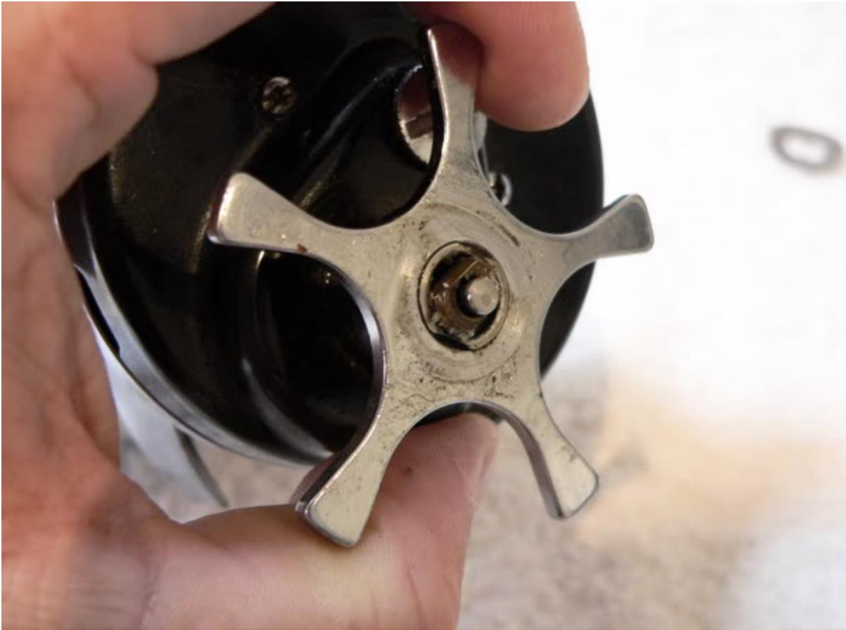
Now the 2 screws securing the right side-plate can be removed and the side plate will slip off.
