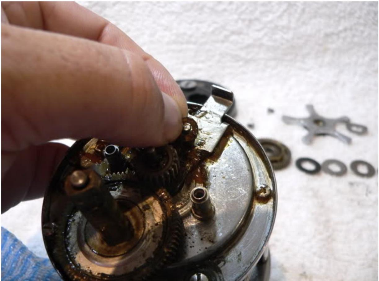
Next, detach and remove the 2 clutch slider springs (ref #9715 & 4055)... carefully so that they don't fly into the never-never.
