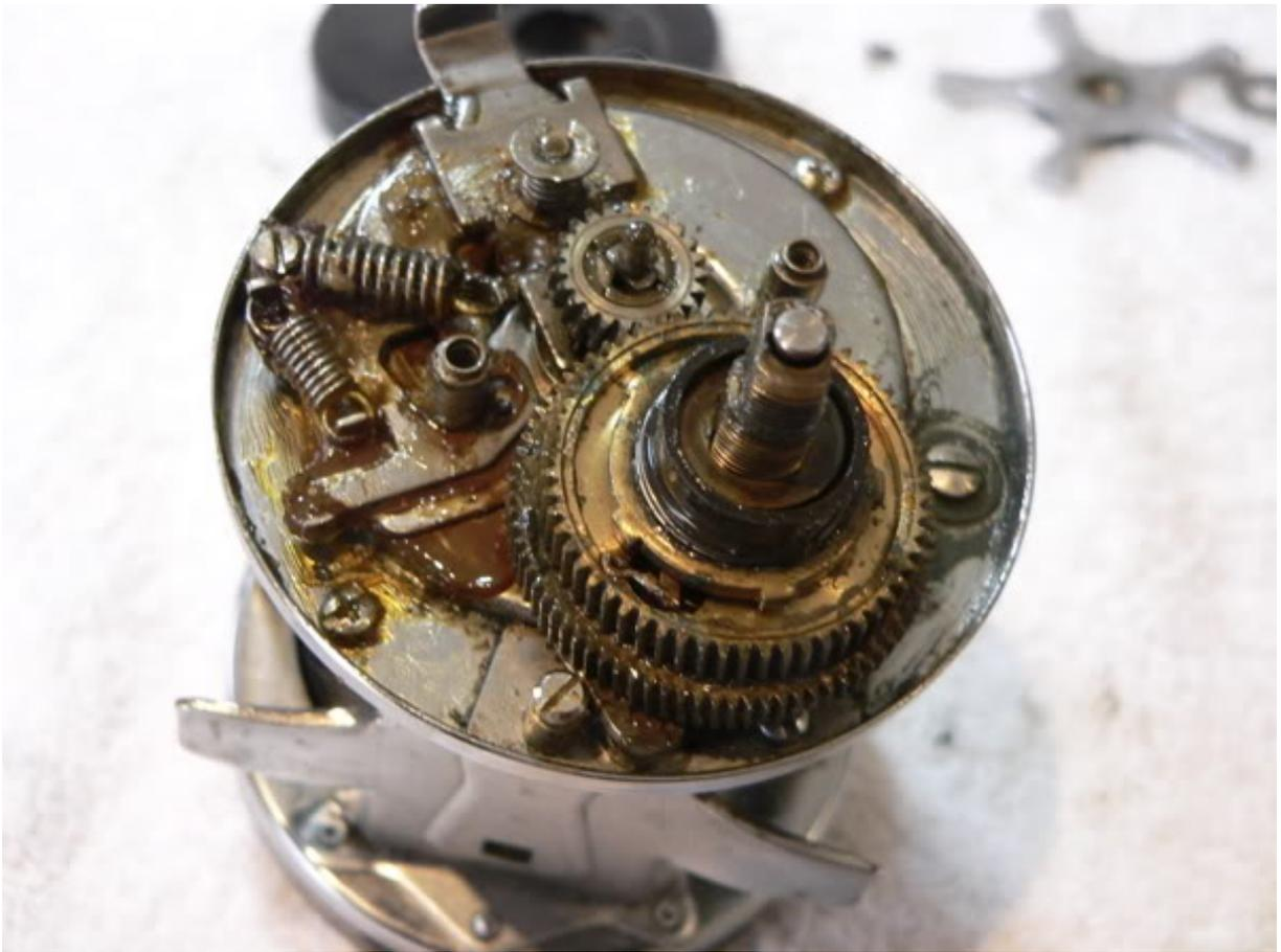
Let's start cleaning up... slip off the spacing sleeve/shield assembly and pull it apart for cleaning.
