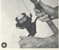
Bail automatically snaps down to retrieving position when handle is rotated for line retrieve. Rotate handle with firm motion to release bail from automatic bail lock. Line automatically is fed to line roller.
