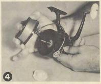
To change spools, back off drag tension knob counter-clockwise and remove. Lift spool from shaft. Keeper spring retains drag discs in position in spool body. Place new spool over shaft, heavy base down. Be sure to align drag washers in spool with shaft. Press into position. Replace drag knob, turning clockwise. Set drag tension as required.
