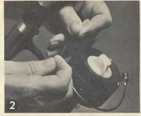
2 Thread line through rod tip, down through all rod guides to reel with bail in casting position. Be sure to secure line to spool arbor with a good knot suitable for monofilament line.
