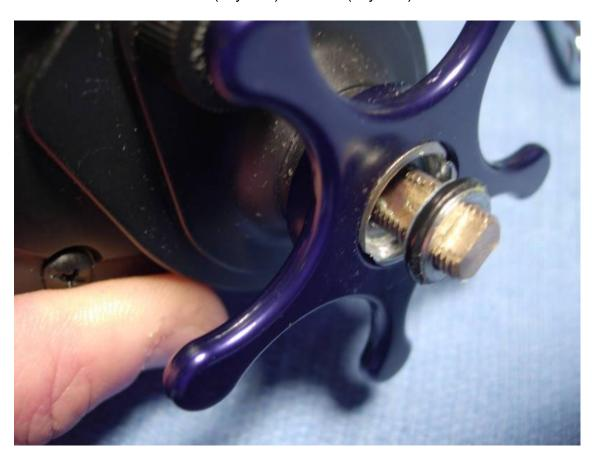
Remove the two right side plate screws "B" (key #109).
