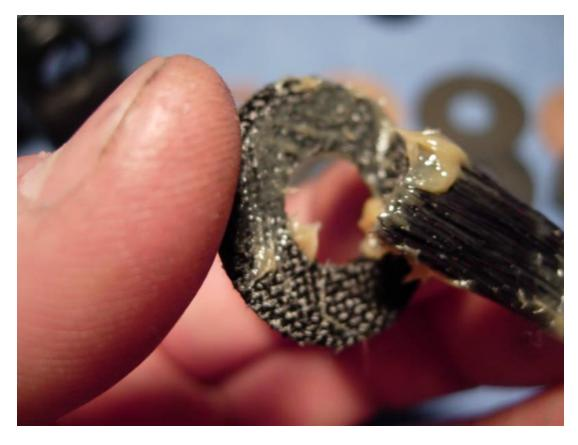
Use an old toothbrush to apply a light coat of grease to the carbon fiber base plate. Install the #6-309 drag washer and the drive gear (key #133).
