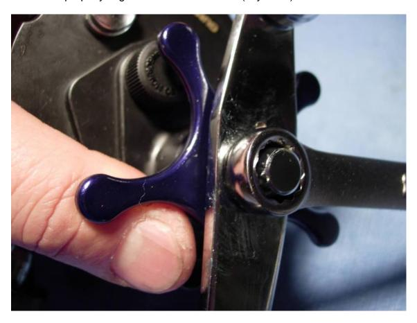
Install the handle nut plate (key #2) and screw (key #128).
