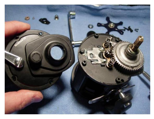
Here's a close up of the gear assembly. Take particular note of the size and strength of this stainless steel main gear and pinion gear. These are much more heavy duty than the gear sets found in equivalent size Trinidad's and Torium's.
