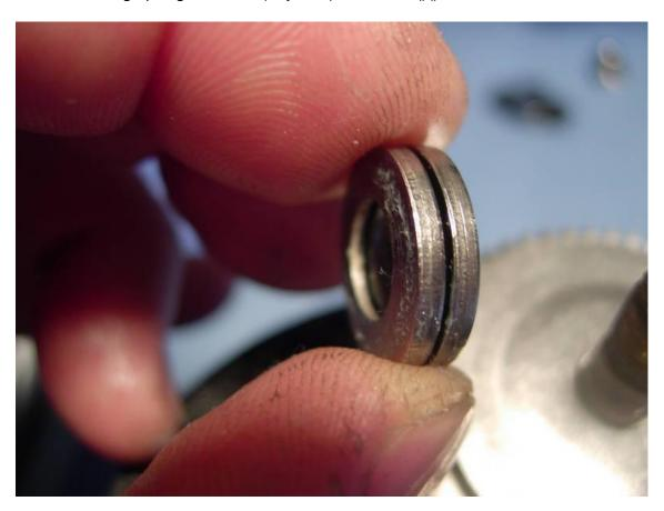
Install the bearing thrust washer (key #91).
