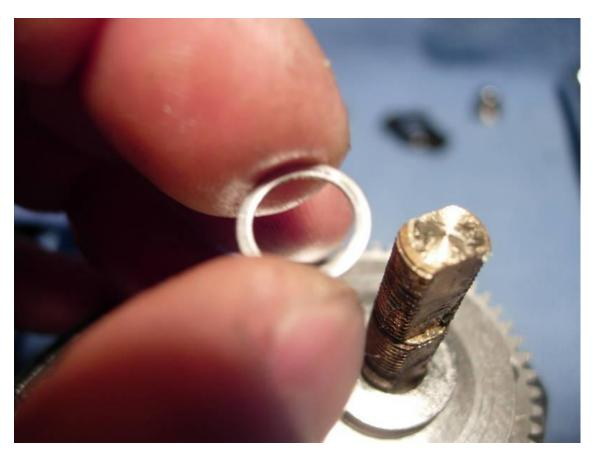
Grease and install the drive shaft bearing (key #483).
