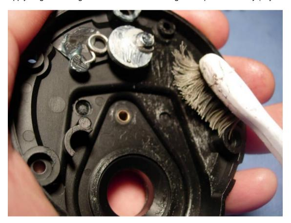
Install the right side plate, noting the "up" position of the yoke plate (key #259) and "forward" position of the clutch lever (key #132).
