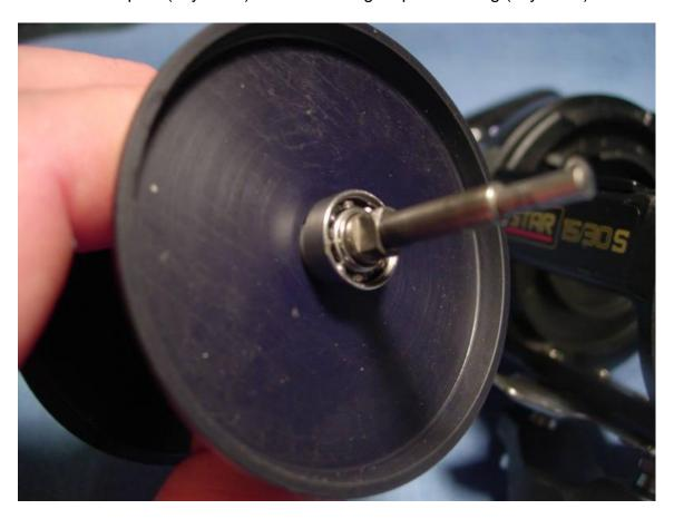
This bearing is 6x12x4 mm. we'll clean it with carb cleaner and compressed air, then lube it with corrosion x.
