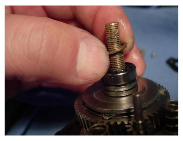
Apply a light coat of grease to the inside of the right side plate assembly (key #209).
