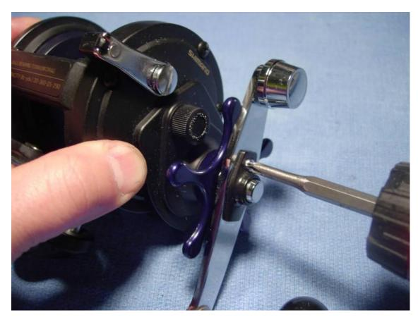
Remove the handle nut (key #129) with a 10mm wrench.
