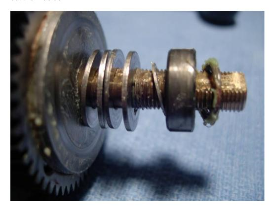
Now, carefully, remove the stainless steel and canvas drag washers, one at a time. I've cleaned them and lined them up for the photo. From left to right is the drive shaft washer (key #100), the drive gear (key #133), the eared washer "b" (key #98), key washer "c" (key #97), drag washer "i" (key #96), eared washer "e" (key #95), drag washer "d" (key #94), and key washer "f" (key #93).
