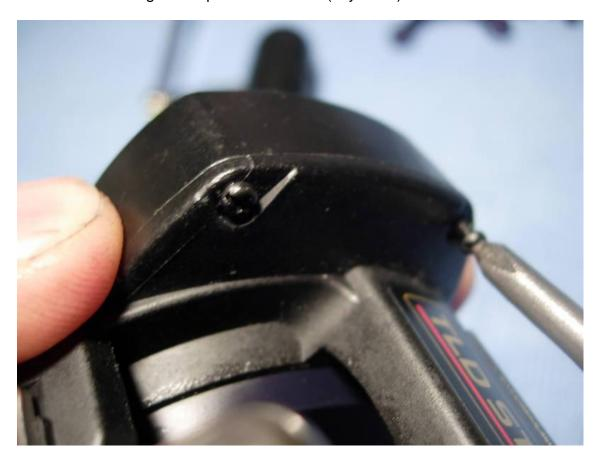
Remove the four right side plate screws "a" (key #81).
