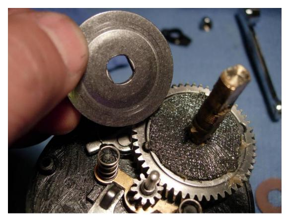
Install the drag spring washers (key #92) oriented "()()".
