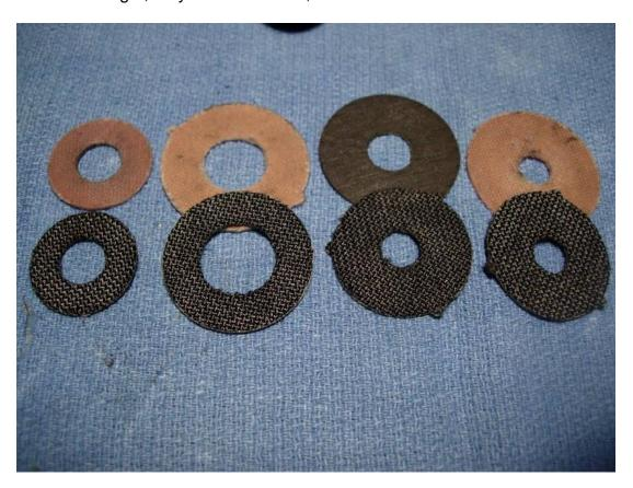
Apply a coat of Cal's drag grease to all four of the carbon fiber drag washers.
