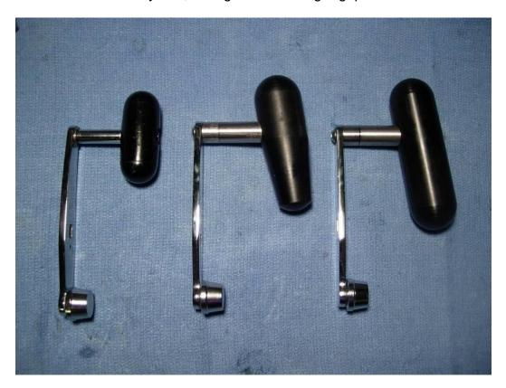
Install the star drag (key #79), the handle washer (key #78), and the new handle (key #414L). Put a little grease on the handle arm around the drive shaft.
