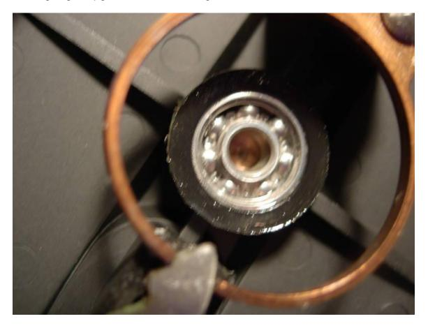
Remove the spool (key #110) and find the right spool bearing (key #482).
