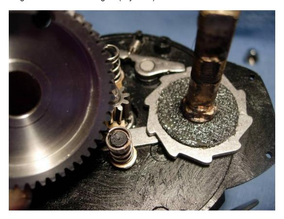
Install the remaining metal and carbon fiber drag washers.
