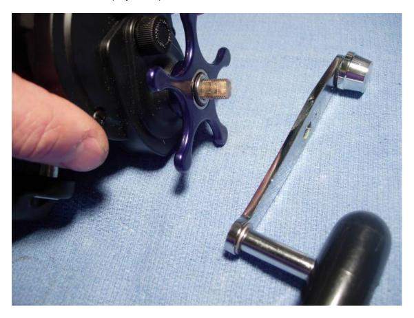
Remove the handle washer (key #78) and star (key #79).
