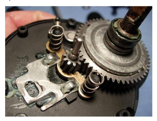
The washer stack is oriented "()()|B|", with four drag spring washers (key #92), a bearing thrust washer (key #91), an 8x16x5 mm bearing (key #483) and a star drag washer (key #80). Remove and set them aside.
