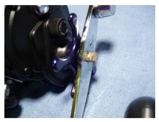
Install and properly align the 10mm handle nut (key #129).
