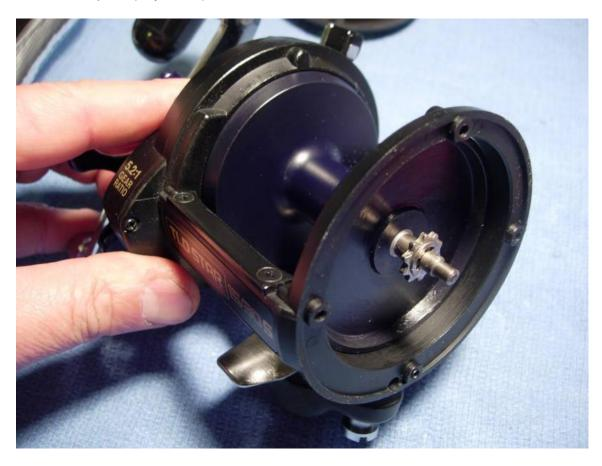
Install the left side plate assembly (key #211) and left side plate screws (key #114). These few steps are all that are required for routine maintenance of this reel.
