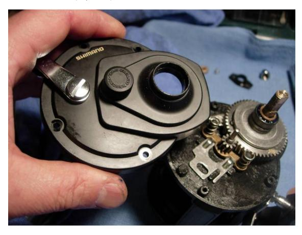
Wiggle the clutch lever back a little and the right side plate should seat properly with a snap!
