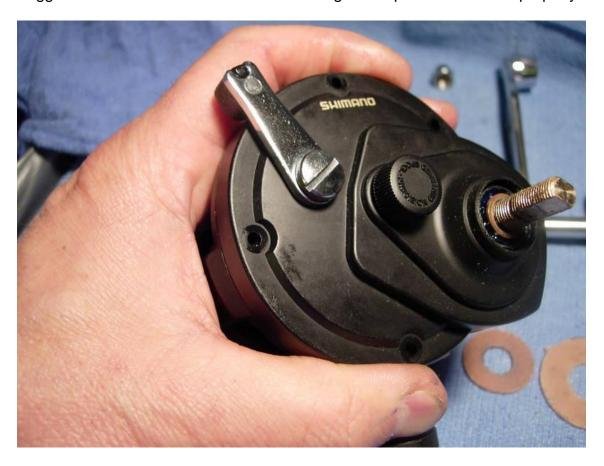
Install the four right side plate screws "a" (key #81).
