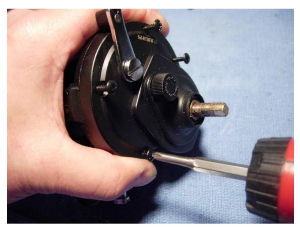
Install the two right side plate screws "b" (key #109).
