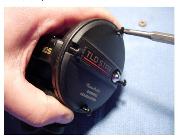
Now for the right side. Remove the handle nut plate screw (key #128) and handle nut plate (key #2).
