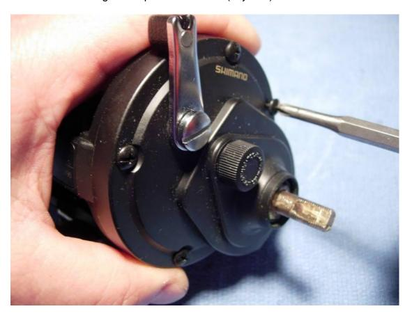
Remove the right side plate assembly (key #209).
