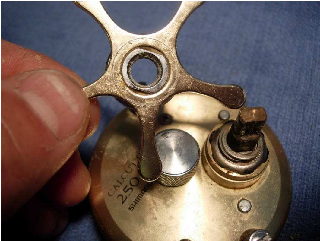
remove the star drag spacer (key #1289)
