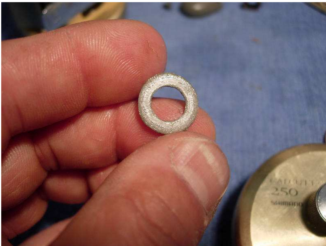
remove the drag spring washers (key # 15).
