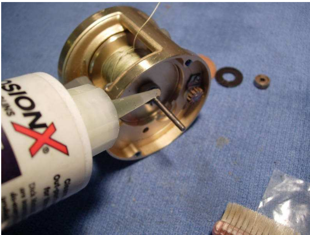
find the clutch plate (key #1233). this is the "in gear" position.
