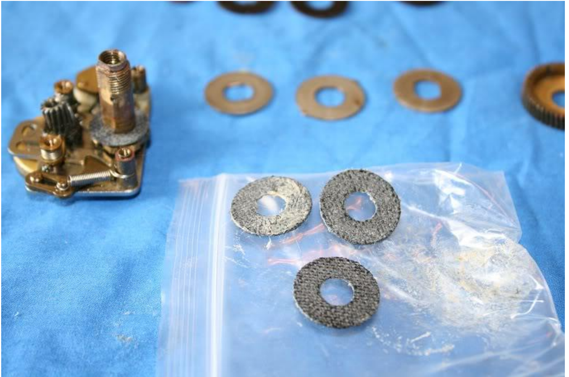
The new HT-100 drag washers that replaced the leather originals. The residue on the stainless washer is actually Cal's as I had fitted the washers then realised I hadn't taken a photo! It's actually better to use the #6-965 and grind them down to fit, but can also use #6-155.
