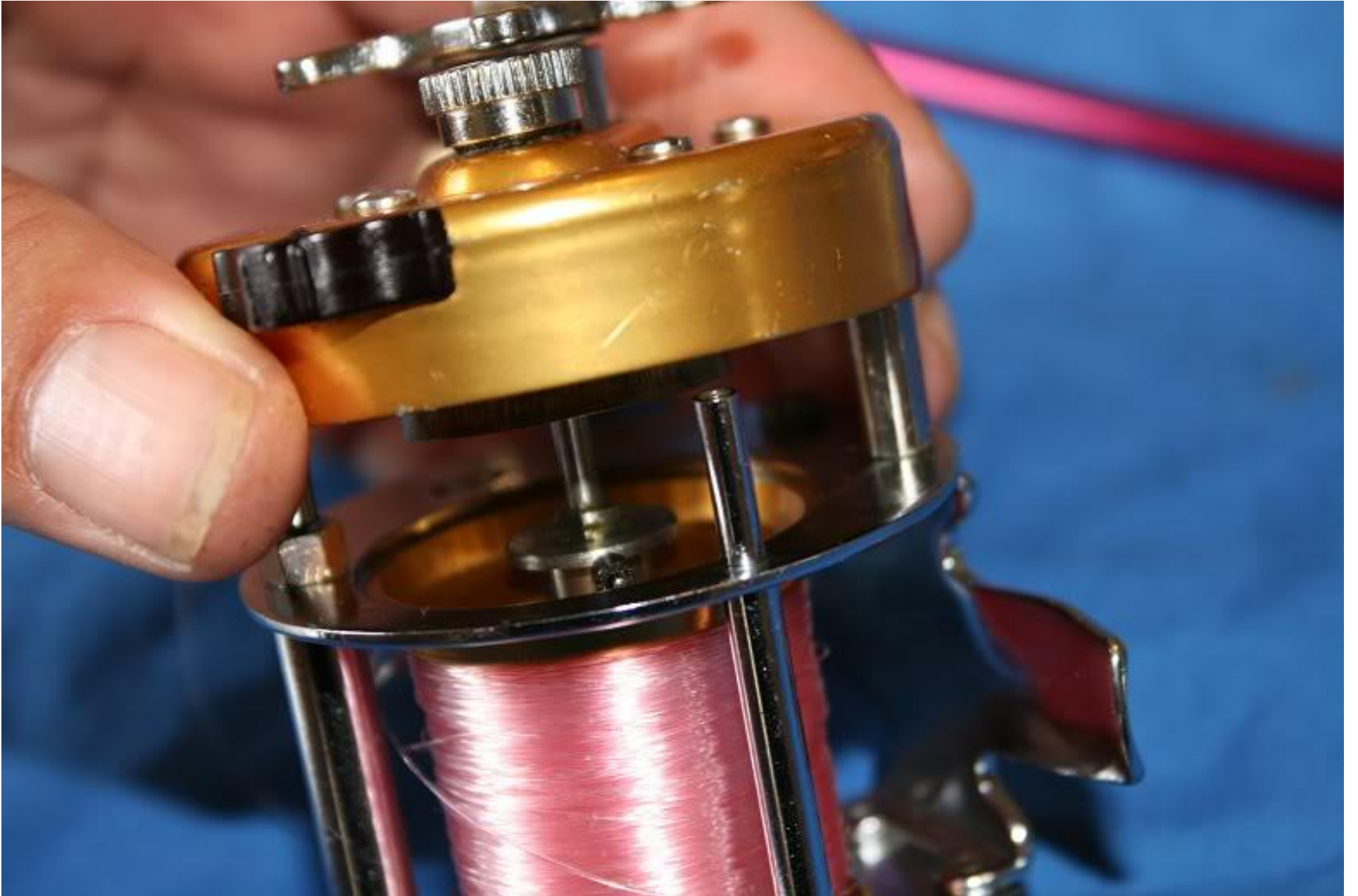
Lube and insert the side plate screws.
