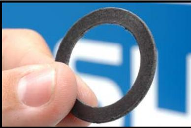
Clean drag washer of old grease. Apply a light coat of Shimano® Drag Grease.
