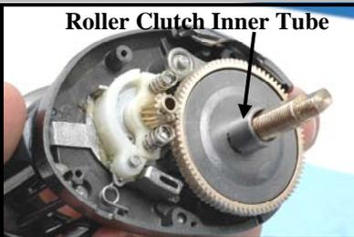
Reinstall yoke springs and roller clutch inner tube. Reinstall right side plate and side plate screws.
