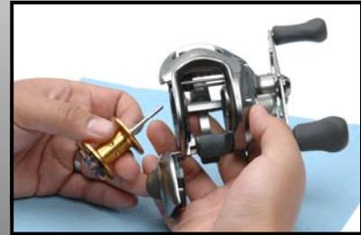
Remove spool assembly. Clean any visible dirt and debris from exterior of reel with cotton swabs or toothbrush and isopropyl rubbing alcohol. Dirt, debris, salt or sand leads to wear and tear.
