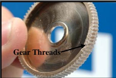
Clean drive gear and apply Shimano® Drag Grease on the threads of the gear.
