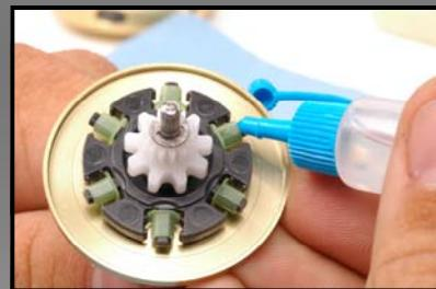
Clean and oil VBS® Brake Collars to maintain optimal casting performance. Inspect collars for wear and tear; replace accordingly.
