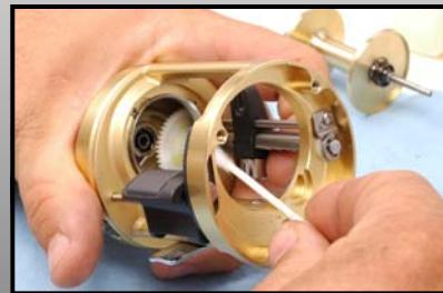
Using cotton swabs and/or a toothbrush with isopropyl rubbing alcohol, clean the exterior of the reel.
