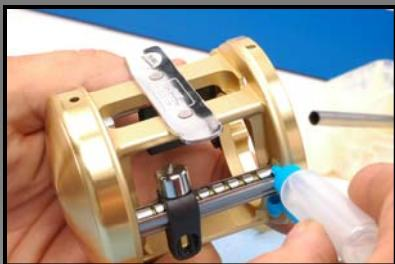
Clean levelwind system of dirt, debris and old grease. Apply 3 drops of Shimano® Bantam® Oil to levelwind. On heavily used reels, Shimano® Drag Grease may be used also.
